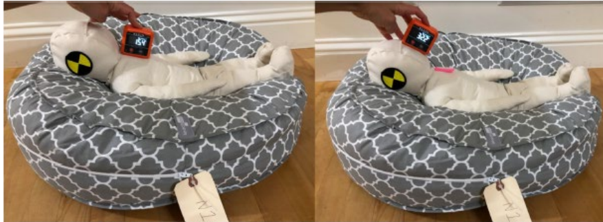
Figure 6. Photos of torso (left) and head (right) segment measurements of the newborn CAMI dummy in a normal Leachco Podster product.
