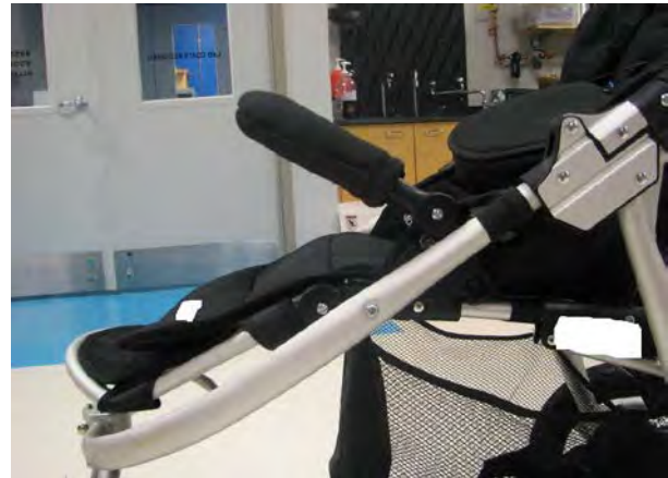
Figure 2. Grab bar in the car seat attachment position. The opening between the grab bar and seat FAILS ASTM F833-13b, Section 7.12, Passive Containment/Foot Opening Test Method .
