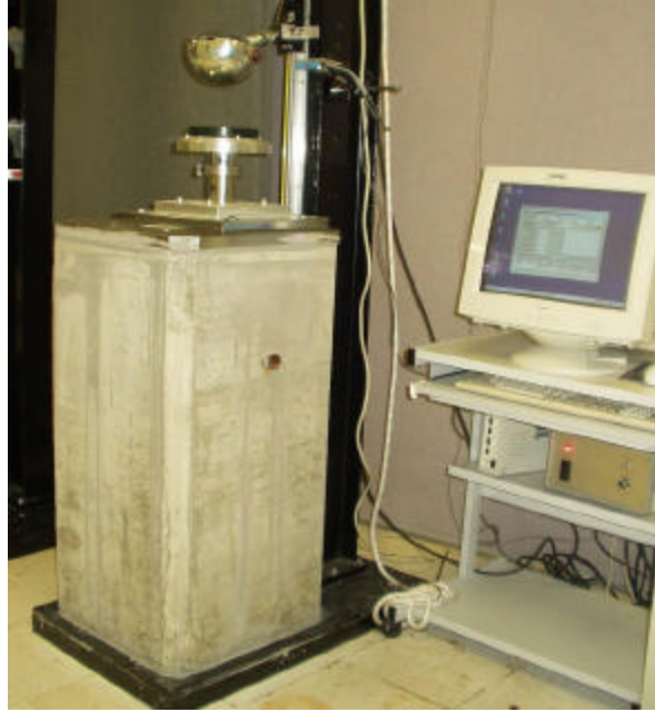
Photograph 1 – Test tower, concrete base, F1292 hemispherical impactor, and electronics.
