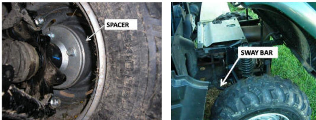
Figure 1. Modifications to ROV to improve steering characteristics.
