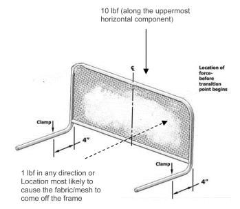
Figure 8: Determining misassembly/functional bed rail test setup
