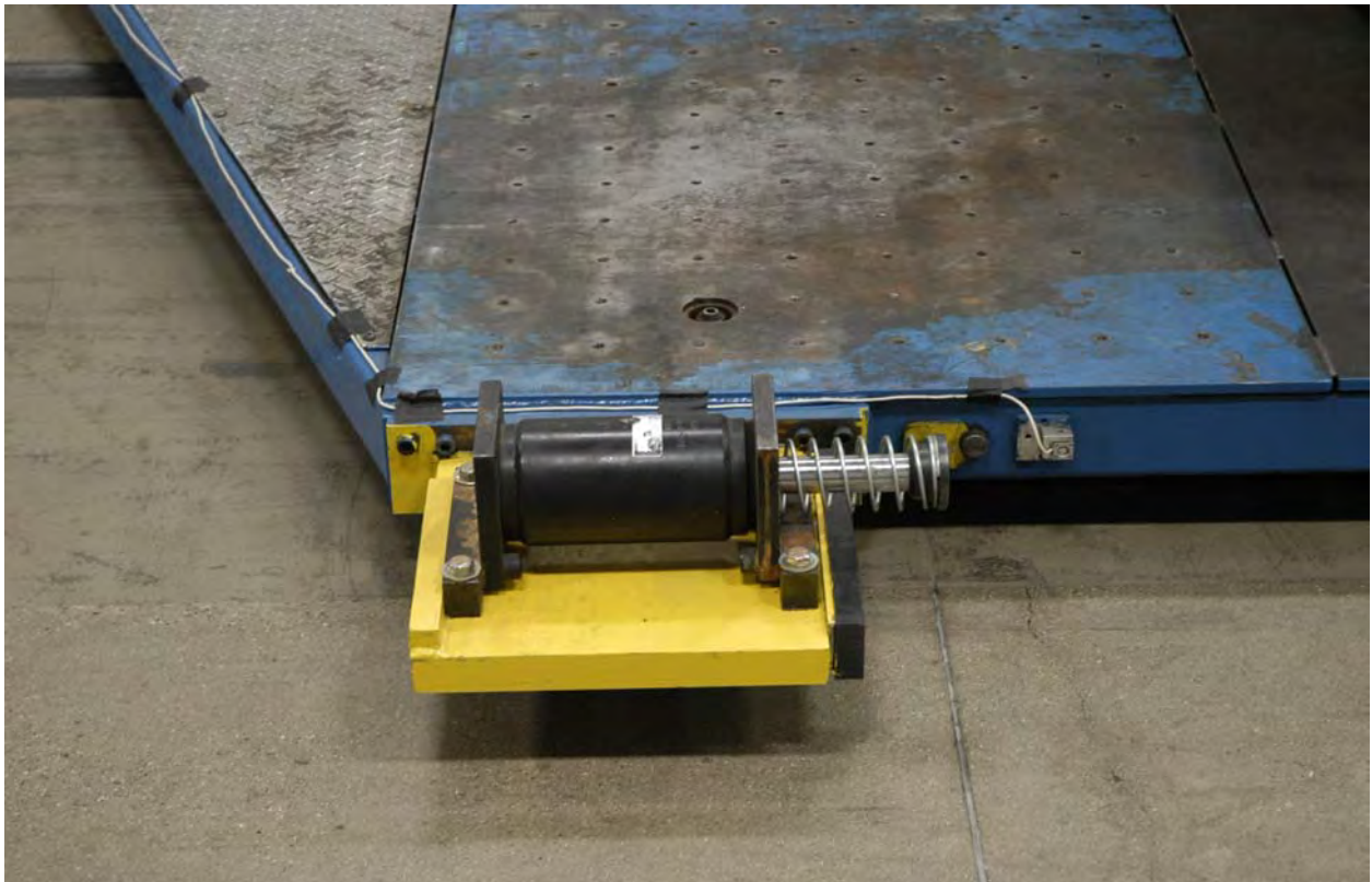
Figure 2.12 Ace Damper for Engaging Brake Caliper
