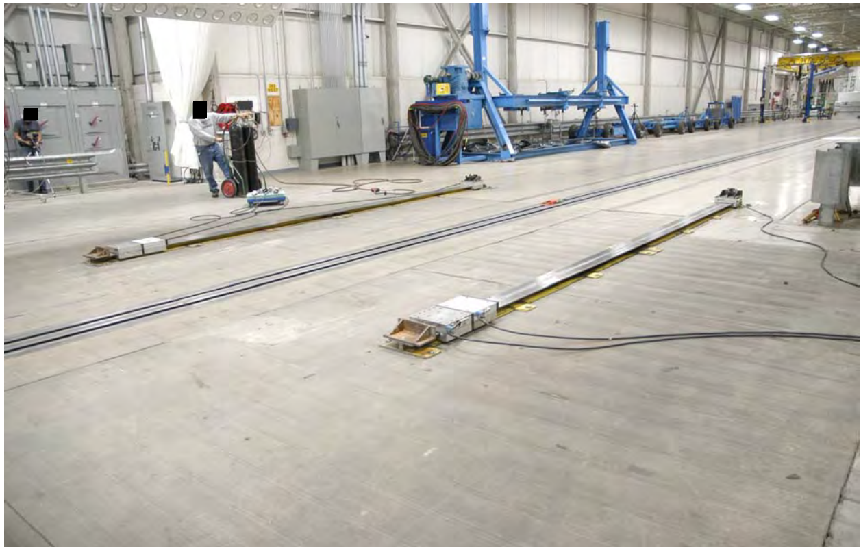
Figure 2.10 Brake Rails and Caliper System
