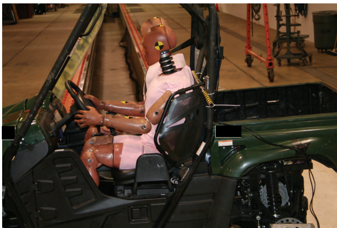
Figure 3.12 Enhanced Restraint Mounted in [REDACTED]
