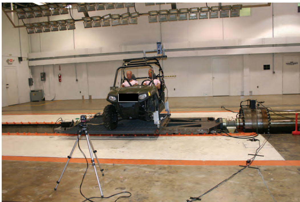
Figure 3.11 Camera Placement for Sled Testing
