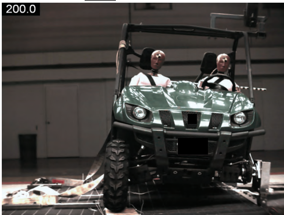
Figure 4.7 Sled Test at time = 200 msec
