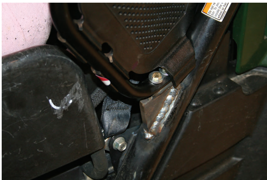
Figure 3.14 Lower Mounting of Enhanced Restraint in [REDACTED]
