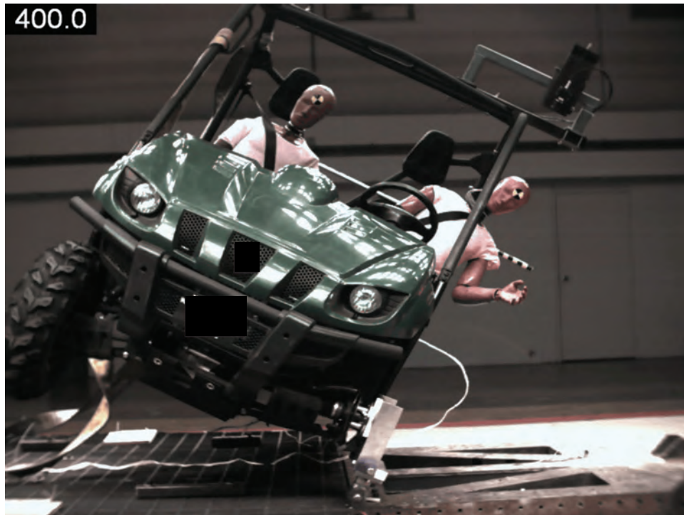
Figure 4.8 Sled Test at time = 400 msed
