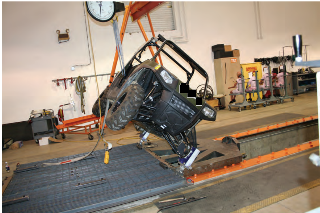
Figure 3.10 Vehicle Rotated for Tether Adjustment
