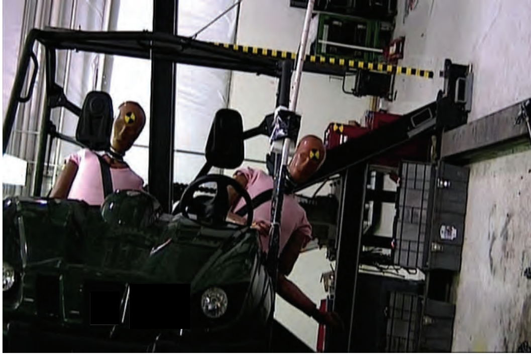
Figure 4.4 Static Test of Baseline [REDACTED] at 90 degrees Rotation
