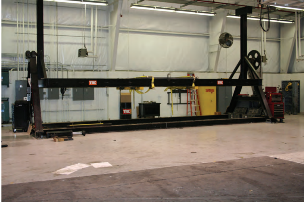
Figure 3.1 FMVSS 301 Static Roll Test Fixture
