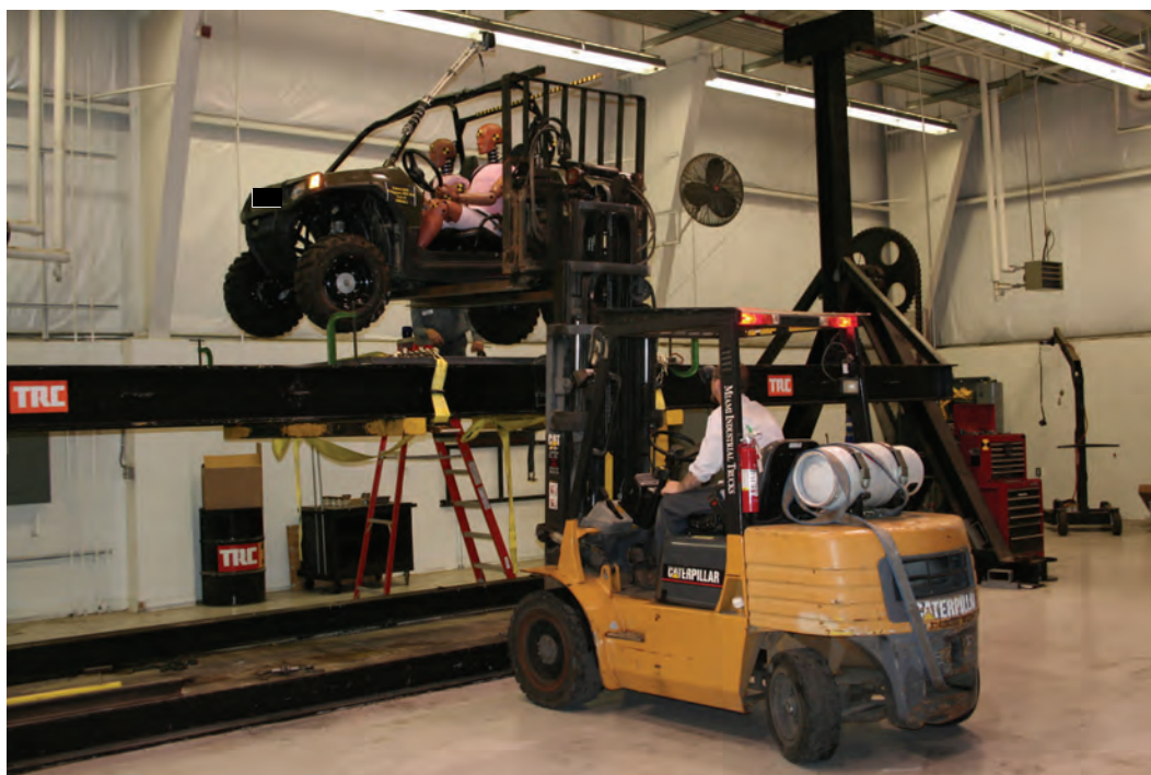
Figure 3.5 Vehicle Mounting to Static Fixture
