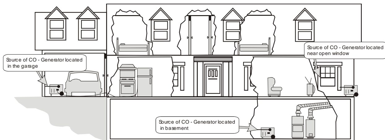
Figure 2. Portable generator located in confined spaces or near an open window
