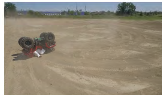
Drone Camera - End of Run - Roll Angle = 174.1°
