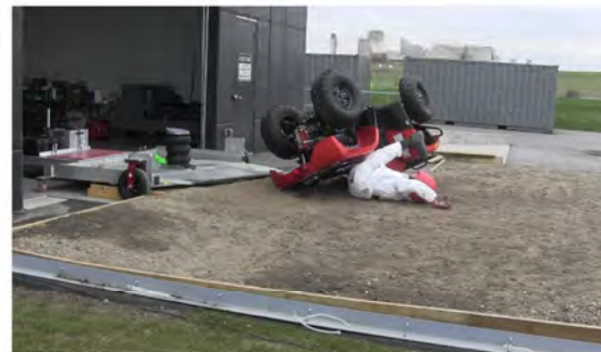
RT Camera 1 - End of Run - Roll Angle = 151.9°
