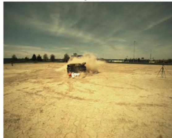
AOS Camera 1 - Roll Angle = 270° - Time = 2.46 sec
