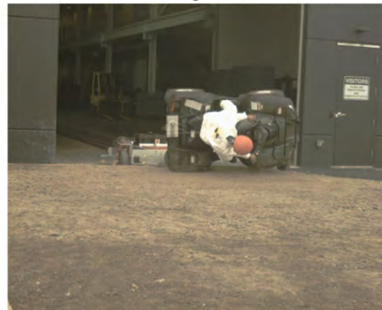
AOS Camera 1 - Roll Angle = 90° - Time = 1.03 sec
