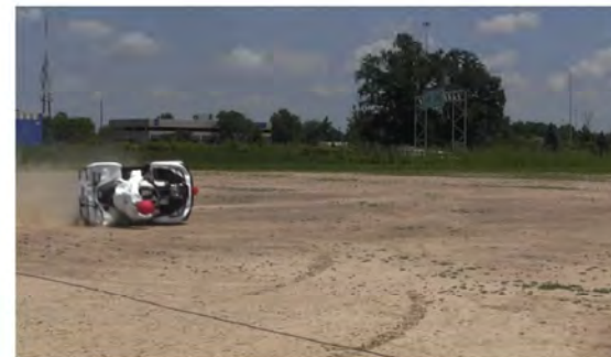
RT Camera 1 - Roll Angle = 90° - Time = 1.74 sec
