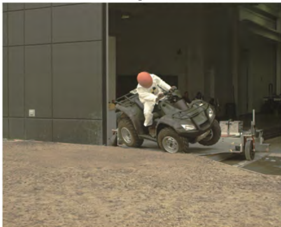
AOS Camera 2 - Roll Angle = 30° - Time = 0.69 sec
