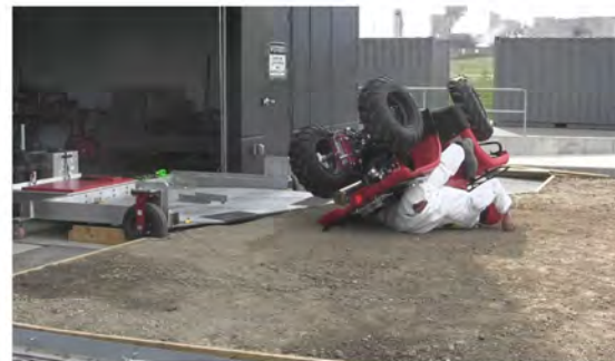
RT Camera 1 - End of Run - Roll Angle = 144.4°
