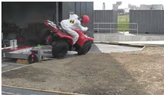
RT Camera 1 - Roll Angle = 30° - Time = 0.73 sec
