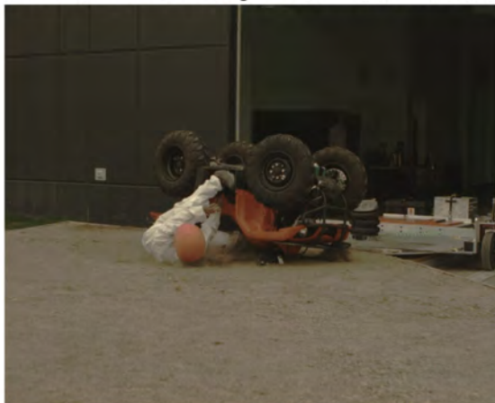
AOS Camera 2 - Roll Angle = 180° - Time = 1.15 sec
