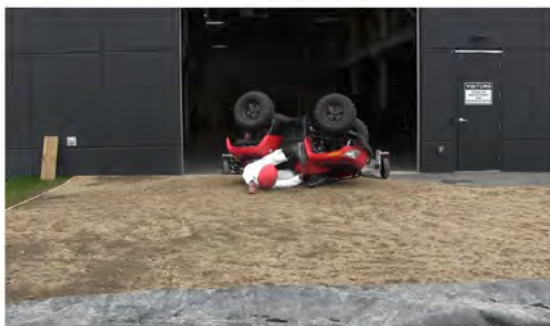
RT Camera 2 - Max Angle = 157.9° - Time = 1.7 sec
