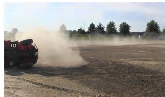
RT Camera 2 - Roll Angle = 270° - Time = 3.63 sec
