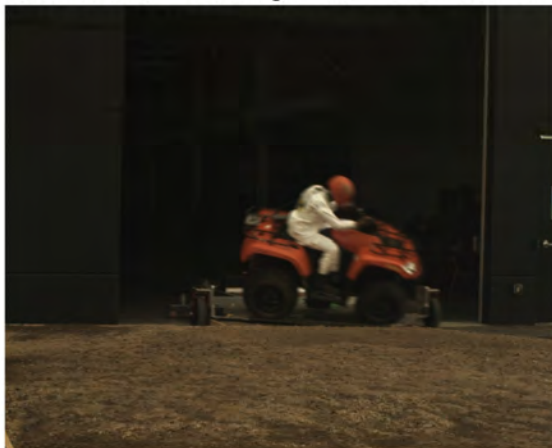
AOS Camera 1 - Roll Angle = 30° - Time = 0.53 sec
