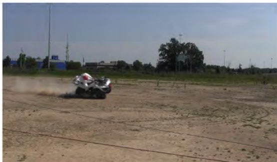
RT Camera 1 - Roll Angle = 30° - Time = 1.22 sec
