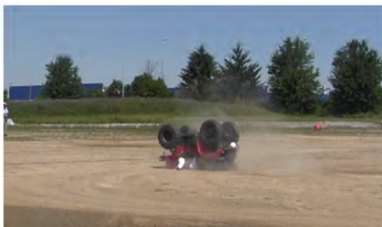
RT Camera 2 - Max Angle = 177.9° - Time = 3.24 sec
