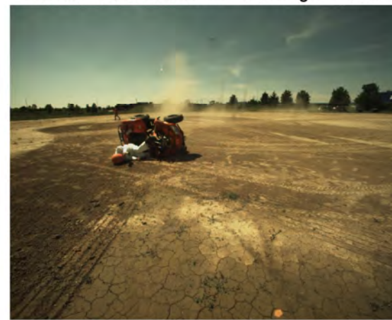
AOS Camera 2 - End of Run - Roll Angle = 102.5°
