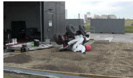
RT Camera 1 - End of Run - Roll Angle = 148.4°
