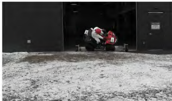
RT Camera 2 - Roll Angle = 45° - Time = 0.77 sec
