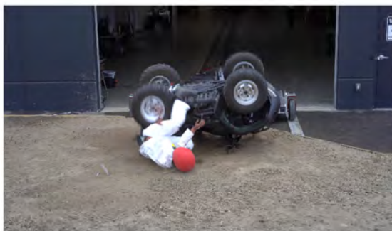
Drone Camera - Roll Angle = 180° - Time = 1.17 sec
