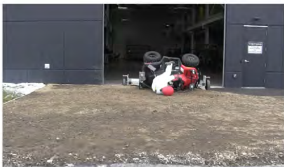
RT Camera 2 - ATD Head Strike - Time = 1.02 sec
