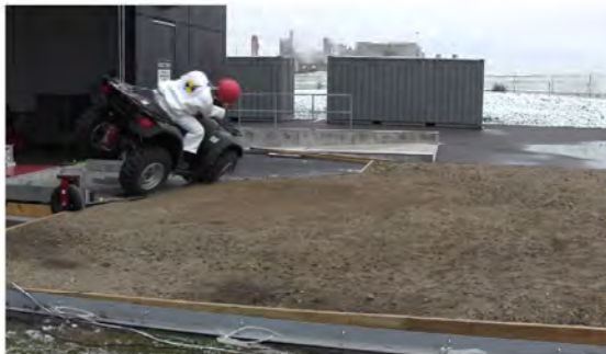
RT Camera 1 - Roll Angle = 30° - Time = 0.69 sec
