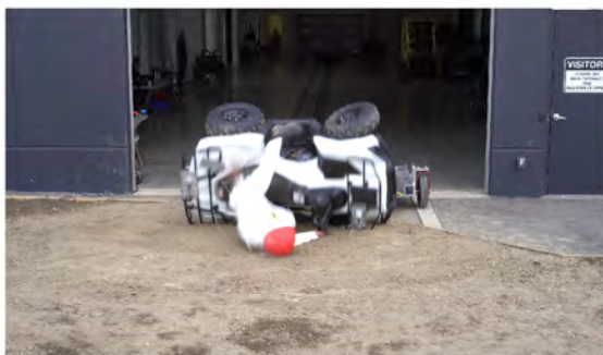
Drone Camera - ATD Head Strike - Time = 0.88 sec
