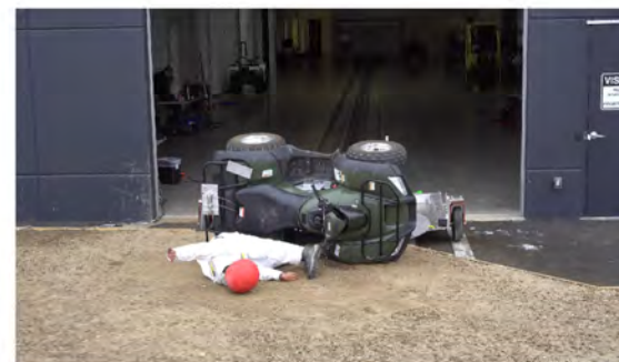
Drone Camera - End of Run - Roll Angle = 94.6°
