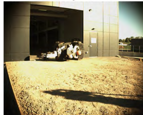
AOS Camera 1 - Roll Angle = 90° - Time = 0.79 sec
