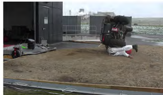
RT Camera 1 - Max Angle = 274.8° - Time = 1.98 sec
