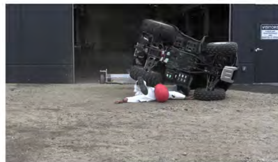
RT Camera 2 - Max Angle = 274.8° - Time = 1.98 sec
