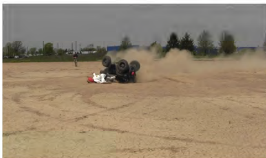
RT Camera 2 - Roll Angle = 180° - Time = 1.94 sec
