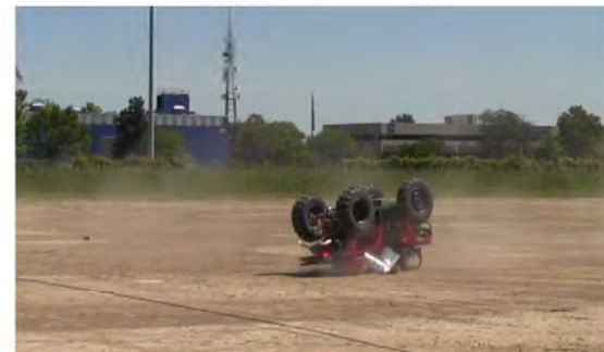
RT Camera 1 - End of Run - Roll Angle = 174.1°
