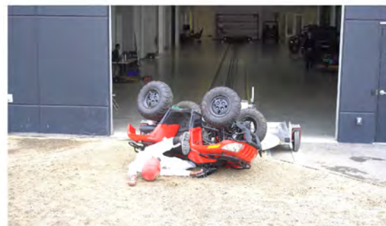
Drone Camera - End of Run - Roll Angle = 151.9°
