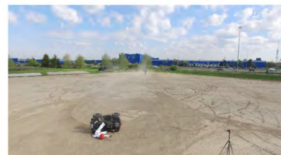
Drone Camera - End of Run - Roll Angle = 92.0°
