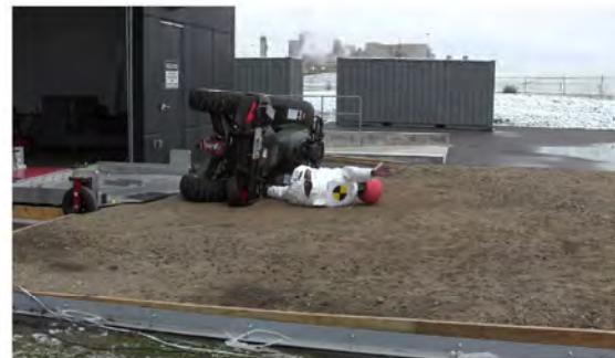
RT Camera 1 - End of Run - Roll Angle = 94.6°
