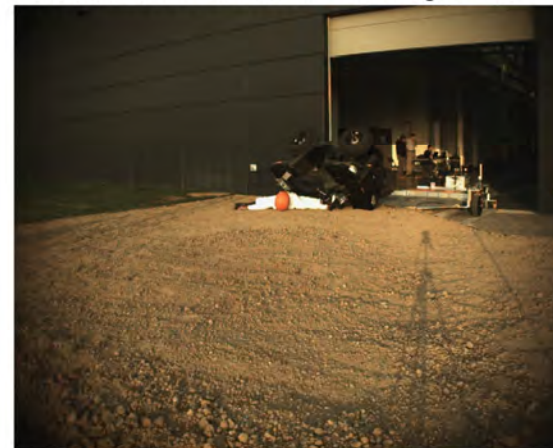
AOS Camera 2 - End of Run - Roll Angle = 135.0°
