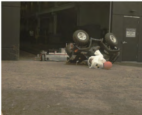
AOS Camera 1 - ATD Head Strike - Time = 1.01 sec
