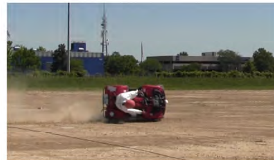
RT Camera 1 - Roll Angle = 90° - Time = 1.85 sec
