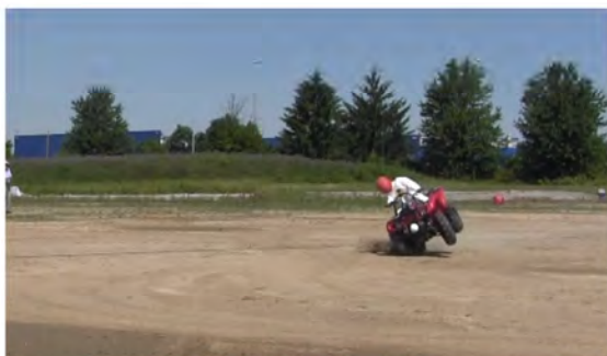
RT Camera 2 - Roll Angle = 30° - Time = 1.28 sec
