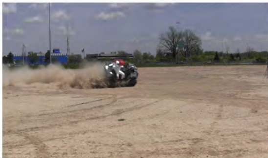
RT Camera 1 - Roll Angle = 45° - Time = 1.42 sec
