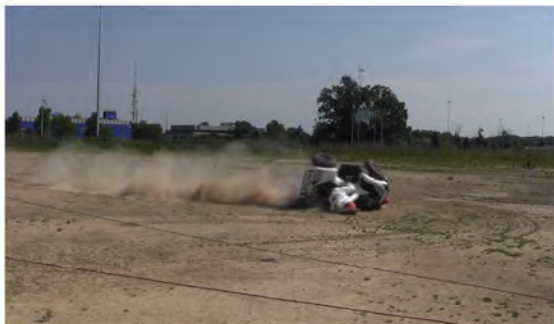
RT Camera 1 - ATD Head Strike - Time = 1.71 sec
