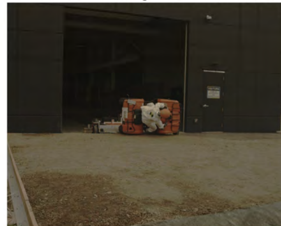
AOS Camera 1 - Roll Angle = 90° - Time = 0.85 sec
