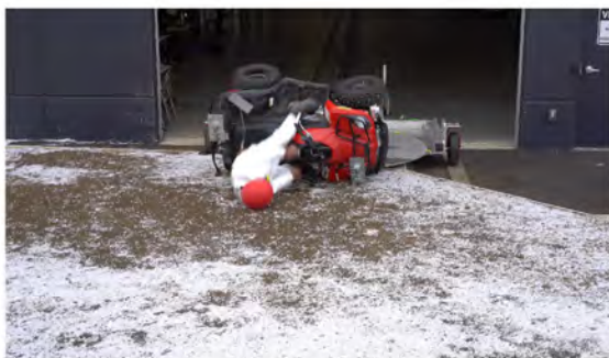
Drone Camera - ATD Head Strike - Time = 1.13 sec
