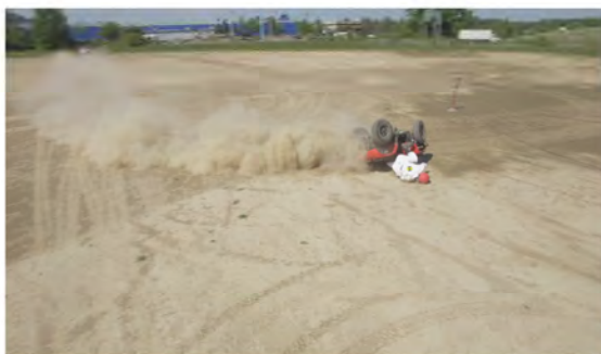
Drone Camera - ATD Head Strike - Time = 2.3 sec
