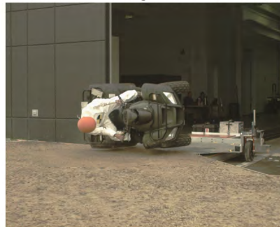
AOS Camera 2 - Roll Angle = 90° - Time = 1.03 sec
