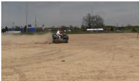
RT Camera 1 - Roll Angle = 30° - Time = 1.39 sec
