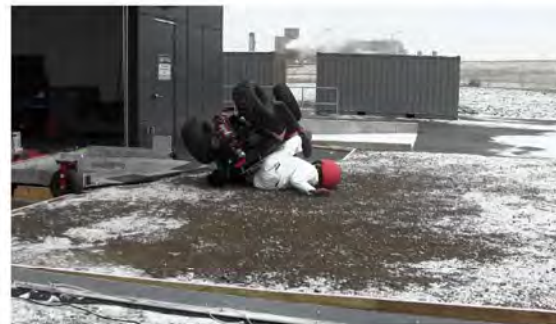
RT Camera 1 - End of Run - Roll Angle = 141.8°
