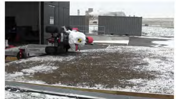
RT Camera 1 - Roll Angle = 90° - Time = 1.01 sec
