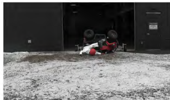
RT Camera 2 - End of Run - Roll Angle = 141.8°
