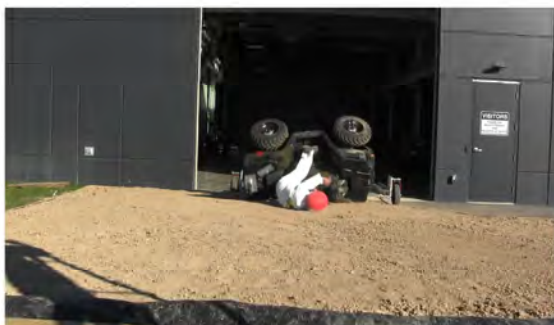
RT Camera 2 - ATD Head Strike - Time = 0.91 sec
