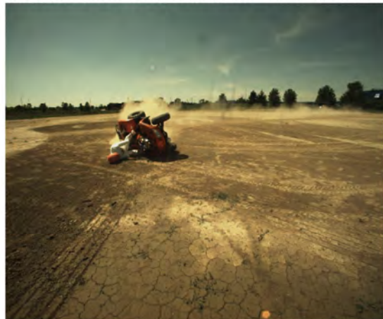
AOS Camera 2 - ATD Head Strike - Time = 2.84 sec
