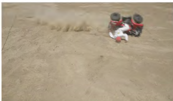
Drone Camera - ATD Head Strike - Time = 1.65 sec
