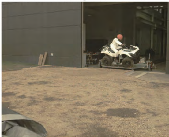
AOS Camera 2 - Roll Angle = 30° - Time = 0.41 sec
