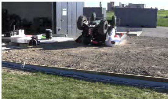
RT Camera 1 - Roll Angle = 180° - Time = 1.1 sec
