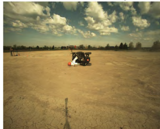
AOS Camera 2 - End of Run - Roll Angle = 92.0°
