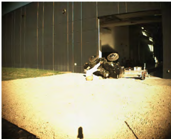
AOS Camera 2 - ATD Head Strike - Time = 0.91 sec
