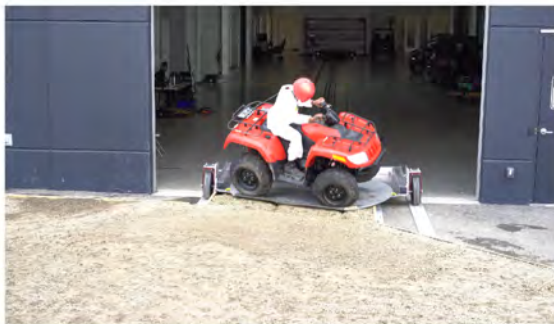
Drone Camera - Roll Angle = 30° - Time = 0.53 sec
