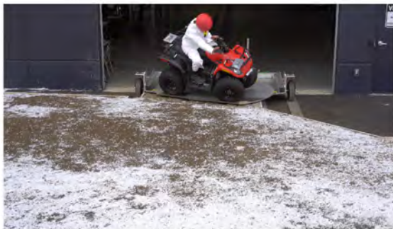
Drone Camera - Roll Angle = 30° - Time = 0.67 sec
