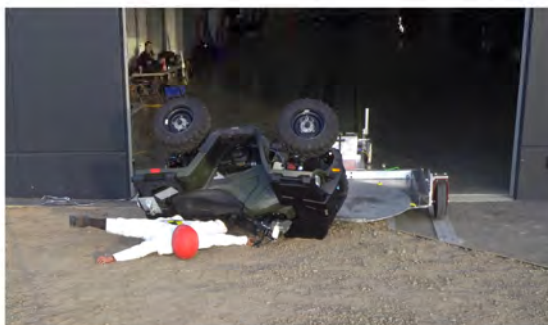
Drone Camera - Max Angle = 137.2° - Time = 2.03 sec
