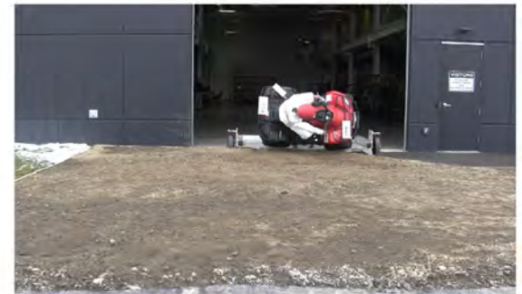
RT Camera 2 - Roll Angle = 90° - Time = 0.86 sec
