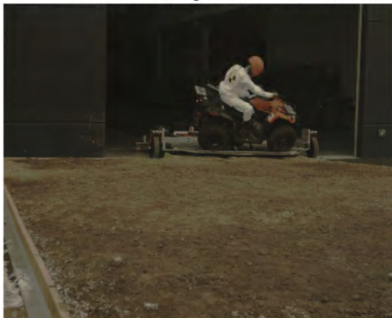
AOS Camera 1 - Roll Angle = 30° - Time = 0.53 sec
