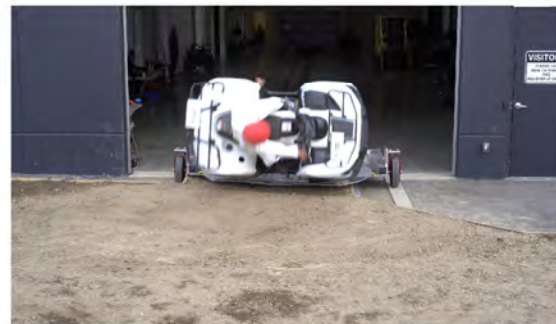
Drone Camera - Roll Angle = 90° - Time = 0.76 sec
