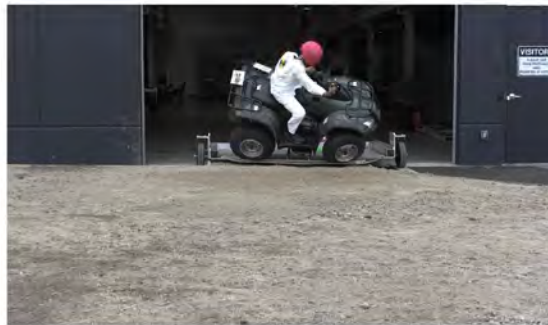
RT Camera 2 - Roll Angle = 45° - Time = 0.58 sec
