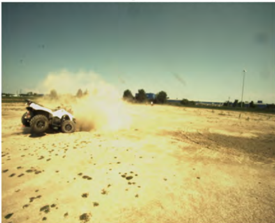
AOS Camera 1 - Roll Angle = 360° - Time = 2.51 sec
