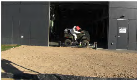
RT Camera 2 - Roll Angle = 30° - Time = 0.42 sec
