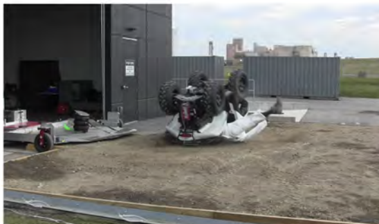
RT Camera 1 - Roll Angle = 180° - Time = 1.18 sec
