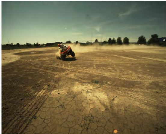
AOS Camera 2 - Roll Angle = 30° - Time = 2.18 sec
