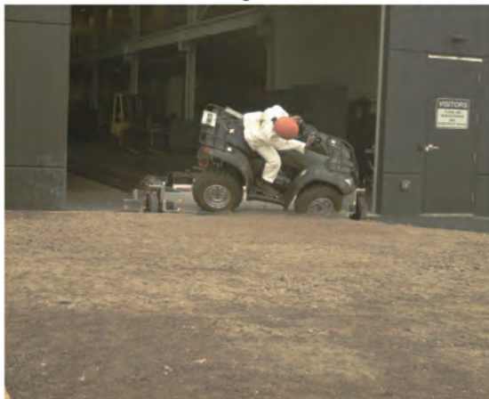
AOS Camera 1 - Roll Angle = 45° - Time = 0.78 sec
