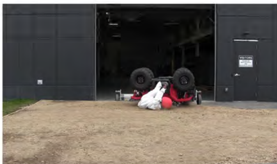
RT Camera 2 - Roll Angle = 180° - Time = 1.15 sec
