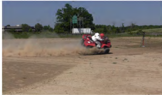
RT Camera 1 - Roll Angle = 45° - Time = 1.82 sec
