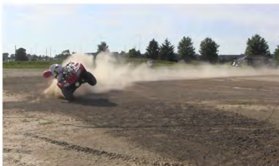
RT Camera 2 - Roll Angle = 45° - Time = 2.26 sec
