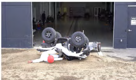
Drone Camera - Max Angle = 164.5° - Time = 1.96 sec
