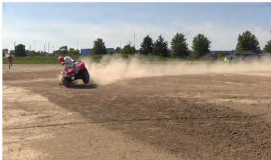
RT Camera 2 - Roll Angle = 30° - Time = 1.72 sec
