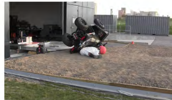
RT Camera 1 - End of Run - Roll Angle = 135.0°
