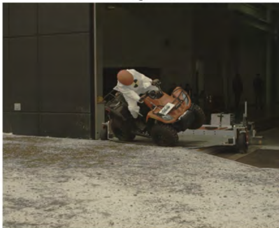
AOS Camera 2 - Roll Angle = 45° - Time = 0.77 sec
