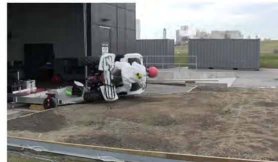
RT Camera 1 - Roll Angle = 90° - Time = 0.92 sec
