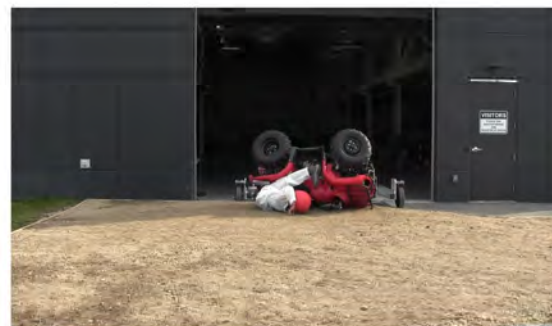
RT Camera 2 - End of Run - Roll Angle = 144.4°
