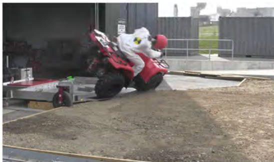
RT Camera 1 - Roll Angle = 45° - Time = 0.82 sec
