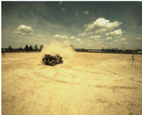
AOS Camera 1 - Roll Angle = 360° - Time = 3.08 sec
