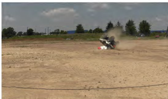
RT Camera 2 - Max Angle = 141.8° - Time = 2.42 sec
