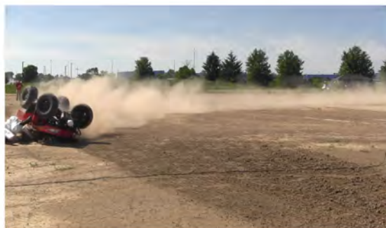
RT Camera 2 - Roll Angle = 180° - Time = 2.36 sec
