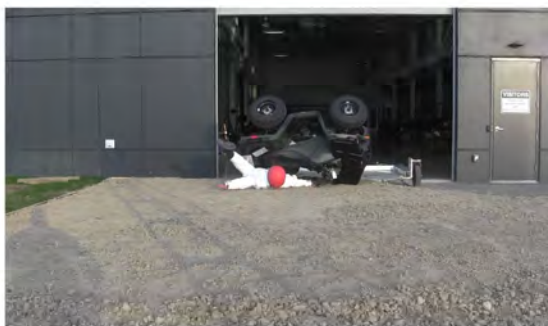
RT Camera 2 - Max Angle = 137.2° - Time = 2.03 sec
