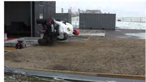
RT Camera 1 - Roll Angle = 90° - Time = 1.03 sec
