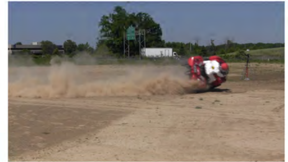
RT Camera 1 - Roll Angle = 90° - Time = 2.02 sec
