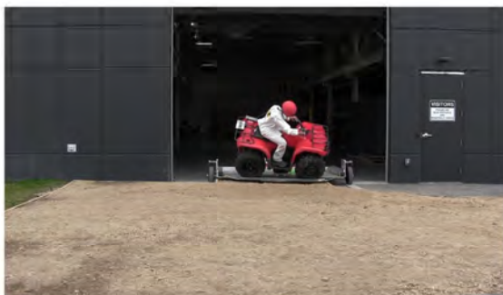
RT Camera 2 - Roll Angle = 30° - Time = 0.51 sec
