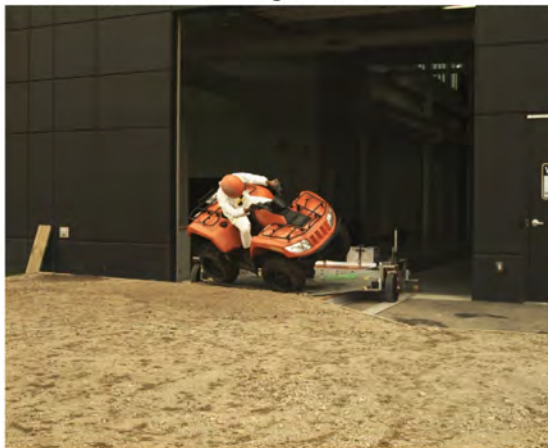
AOS Camera 2 - Roll Angle = 45° - Time = 0.66 sec
