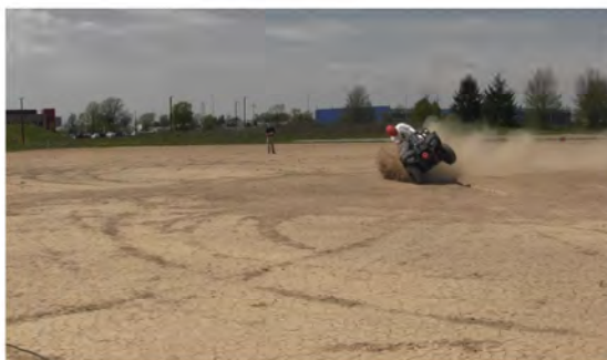
RT Camera 2 - Roll Angle = 45° - Time = 1.48 sec
