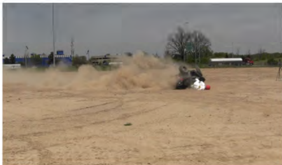
RT Camera 1 - ATD Head Strike - Time = 1.95 sec
