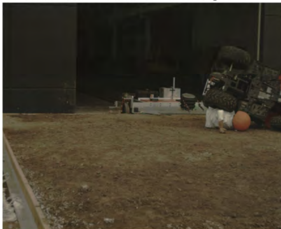
AOS Camera 1 - End of Run - Roll Angle = 253.1°
