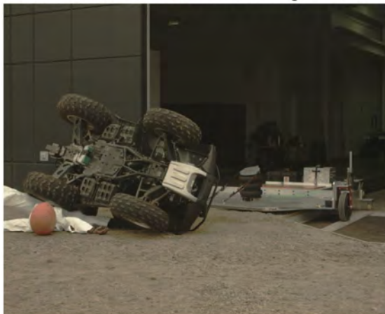
AOS Camera 2 - End of Run - Roll Angle = 241.0°
