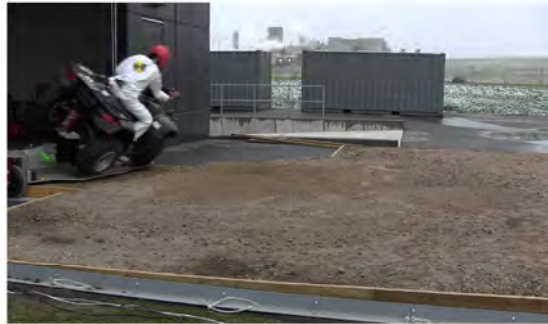
RT Camera 1 - Roll Angle = 45° - Time = 0.58 sec
