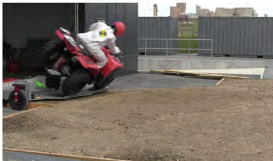
RT Camera 1 - Roll Angle = 45° - Time = 0.62 sec
