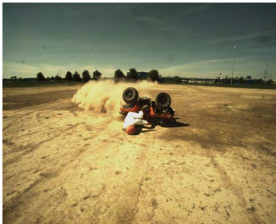
AOS Camera 1 - ATD Head Strike - Time = 2.3 sec
