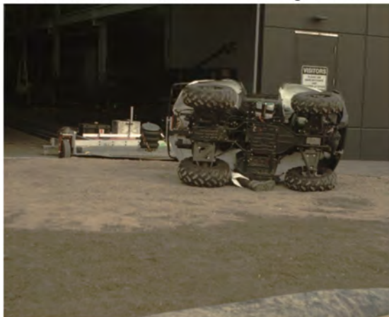
AOS Camera 1 - End of Run - Roll Angle = 277.1°
