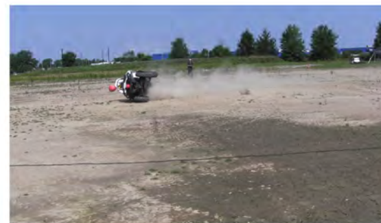
RT Camera 2 - Roll Angle = 90° - Time = 1.59 sec
