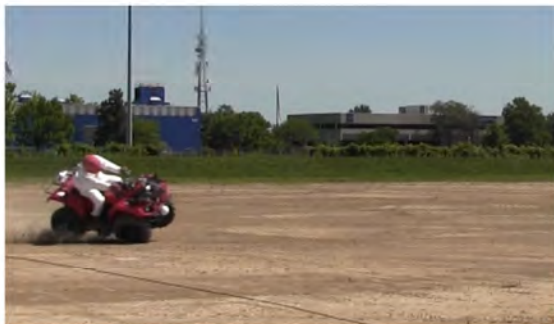
RT Camera 1 - Roll Angle = 30° - Time = 1.28 sec
