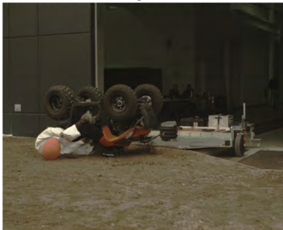
AOS Camera 2 - Roll Angle = 180° - Time = 1.18 sec
