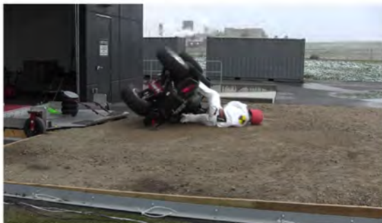
RT Camera 1 - ATD Head Strike - Time = 1.01 sec
