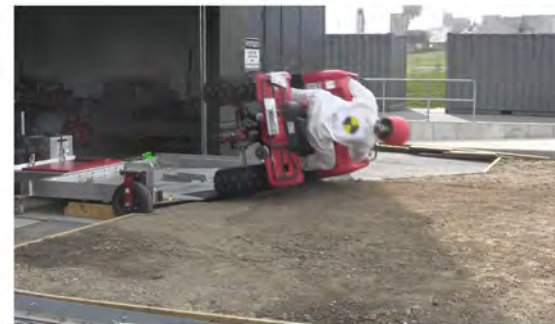
RT Camera 1 - Roll Angle = 90° - Time = 1.07 sec
