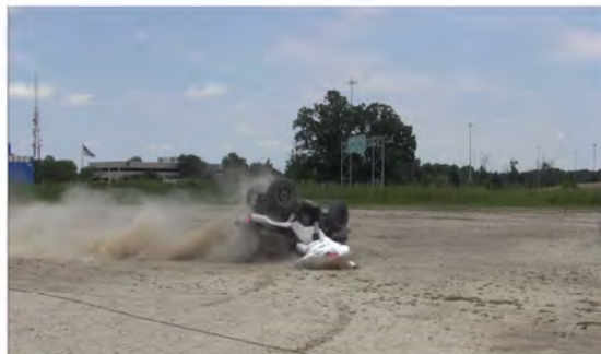
RT Camera 1 - Roll Angle = 180° - Time = 1.69 sec
