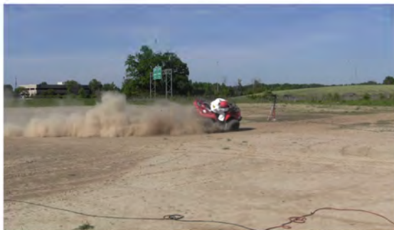
RT Camera 1 - Roll Angle = 30° - Time = 2.05 sec
