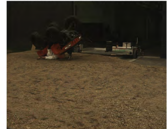
AOS Camera 2 - Max Angle = 202.3° - Time = 2.16 sec
