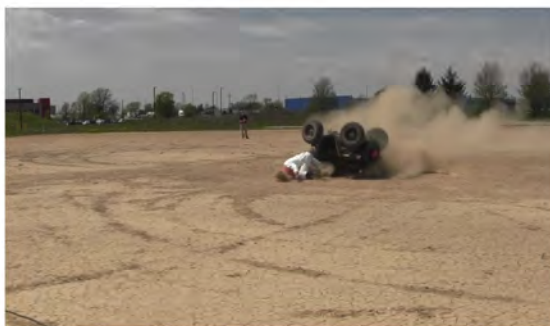
RT Camera 2 - Roll Angle = 180° - Time = 2.09 sec
