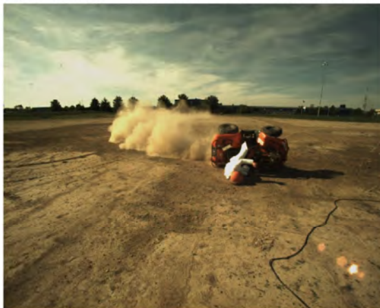
AOS Camera 1 - ATD Head Strike - Time = 2.62 sec
