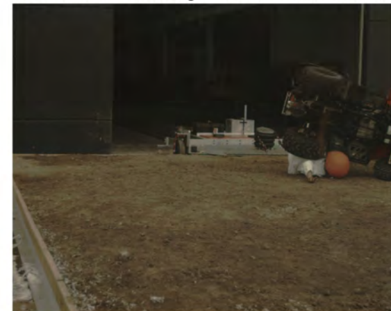
AOS Camera 1 - Max Angle = 281.6° - Time = 2.48 sec
