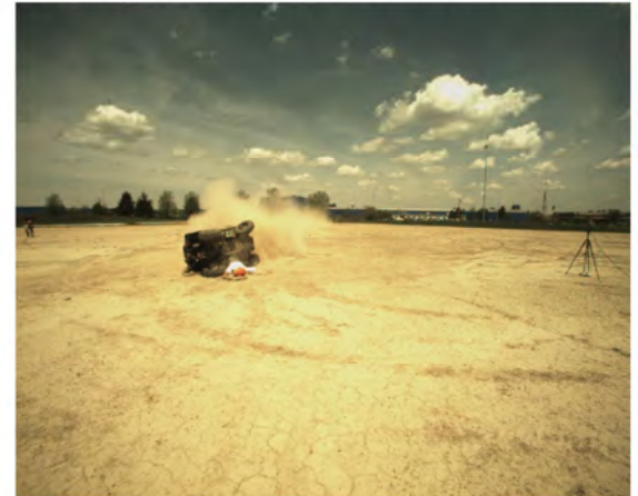
AOS Camera 1 - Roll Angle = 270° - Time = 2.47 sec
