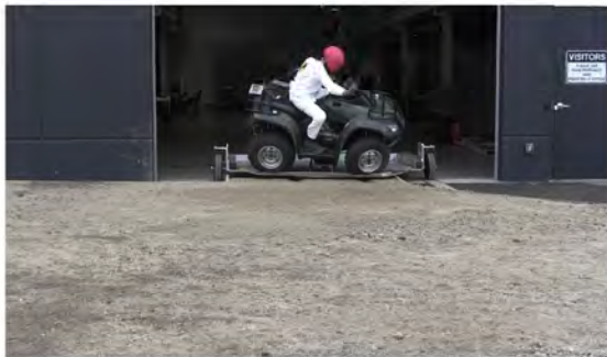
RT Camera 2 - Roll Angle = 30° - Time = 0.46 sec
