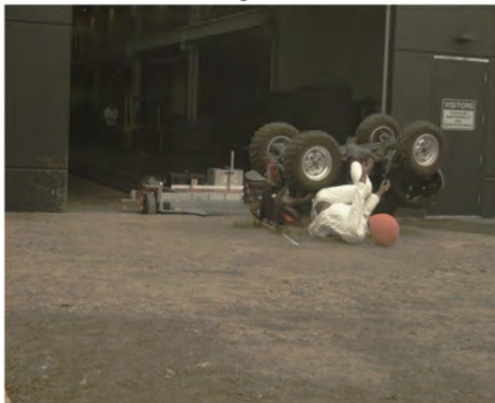
AOS Camera 1 - Roll Angle = 180° - Time = 1.17 sec
