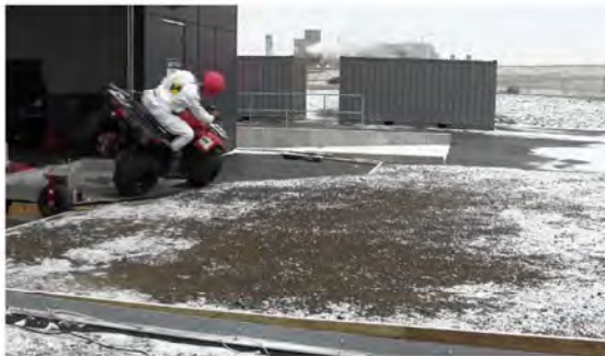
RT Camera 1 - Roll Angle = 30° - Time = 0.67 sec
