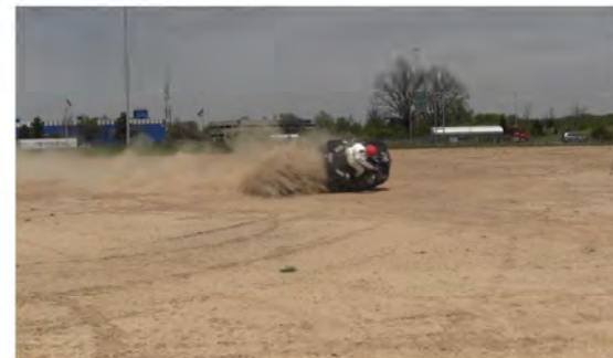
RT Camera 1 - Roll Angle = 90° - Time = 1.67 sec
