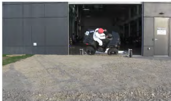
RT Camera 2 - Roll Angle = 45° - Time = 0.86 sec
