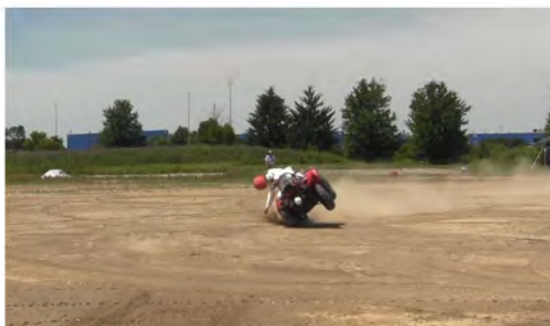
RT Camera 2 - Roll Angle = 45° - Time = 1.3 sec
