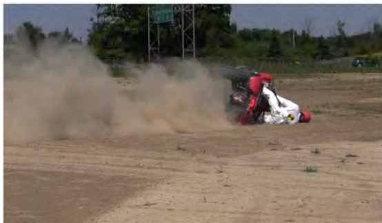
RT Camera 1 - ATD Head Strike - Time = 2.84 sec
