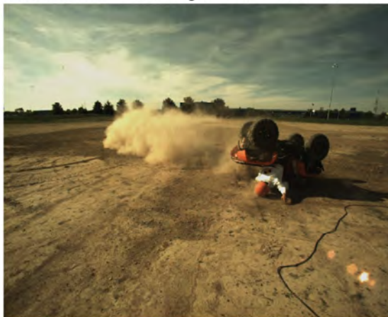
AOS Camera 1 - Roll Angle = 180° - Time = 2.97 sec
