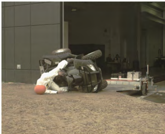
AOS Camera 2 - ATD Head Strike - Time = 1.15 sec
