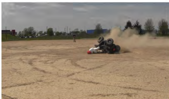
RT Camera 2 - ATD Head Strike - Time = 1.95 sec
