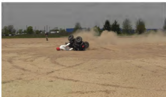
RT Camera 2 - ATD Head Strike - Time = 1.84 sec
