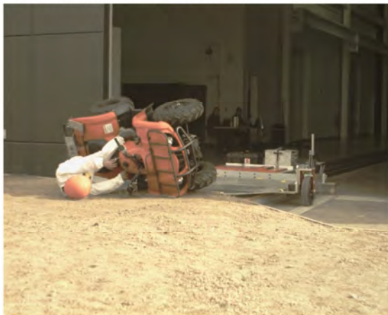
AOS Camera 2 - ATD Head Strike - Time = 1.23 sec
