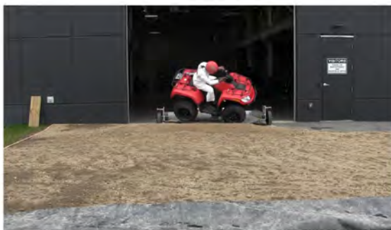
RT Camera 2 - Roll Angle = 30° - Time = 0.53 sec
