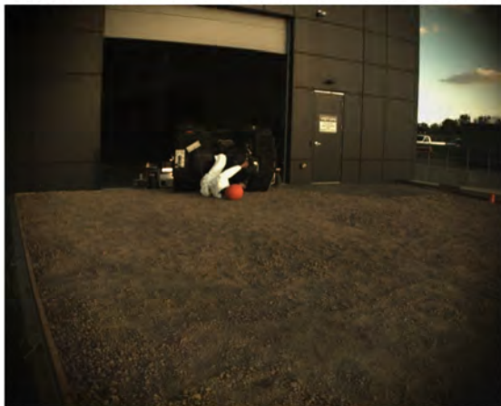
AOS Camera 1 - ATD Head Strike - Time = 1.28 sec
