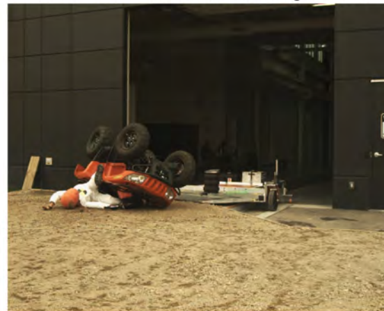
AOS Camera 2 - End of Run - Roll Angle = 151.9°
