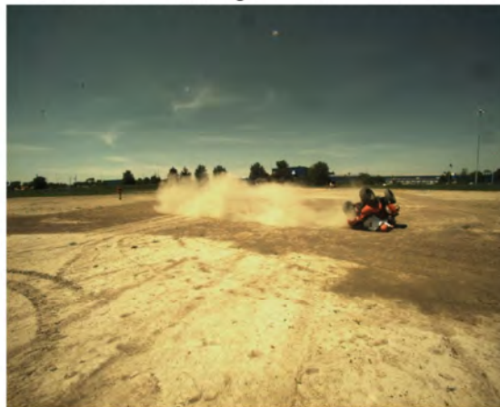
AOS Camera 1 - Max Angle = 148.3° - Time = 3.44 sec
