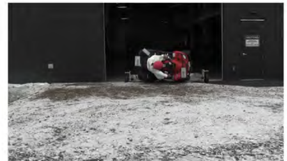
RT Camera 2 - Roll Angle = 90° - Time = 1.01 sec
