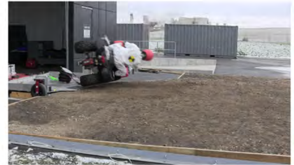
RT Camera 1 - Roll Angle = 90° - Time = 0.86 sec
