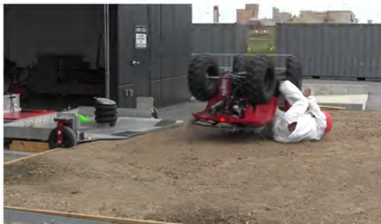
RT Camera 1 - Roll Angle = 180° - Time = 1.15 sec
