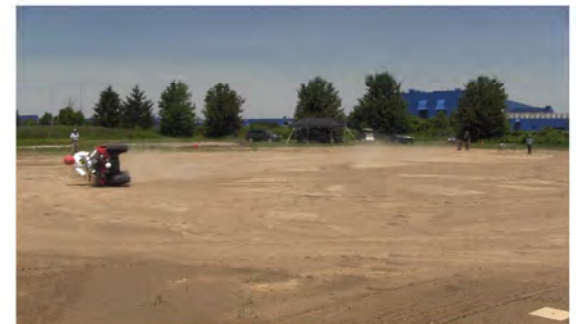
RT Camera 2 - Roll Angle = 90° - Time = 1.27 sec
