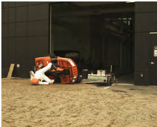
AOS Camera 2 - ATD Head Strike - Time = 0.99 sec
