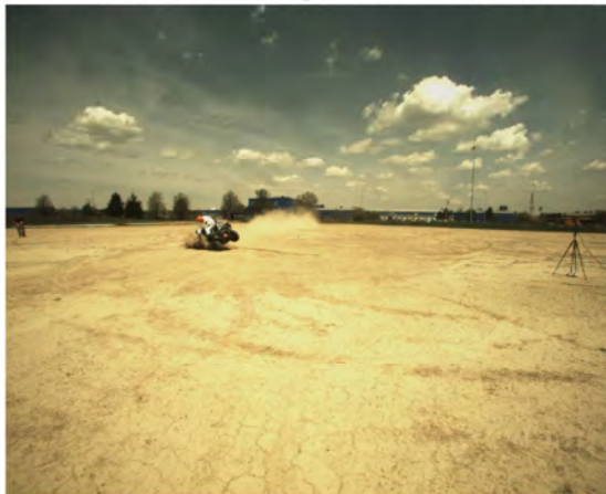
AOS Camera 1 - Roll Angle = 45° - Time = 1.42 sec
