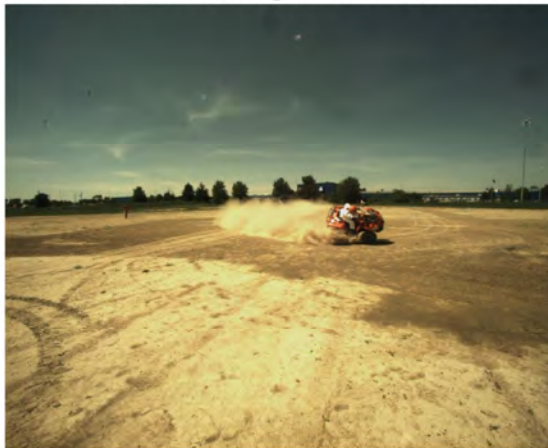
AOS Camera 1 - Roll Angle = 45° - Time = 2.38 sec
