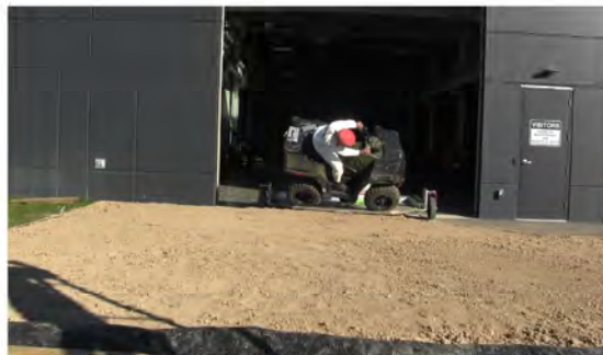
RT Camera 2 - Roll Angle = 45° - Time = 0.56 sec
