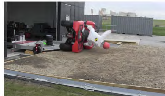
RT Camera 1 - Roll Angle = 90° - Time = 0.91 sec
