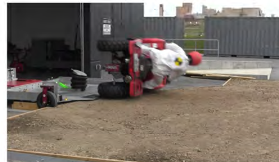
RT Camera 1 - Roll Angle = 90° - Time = 0.85 sec
