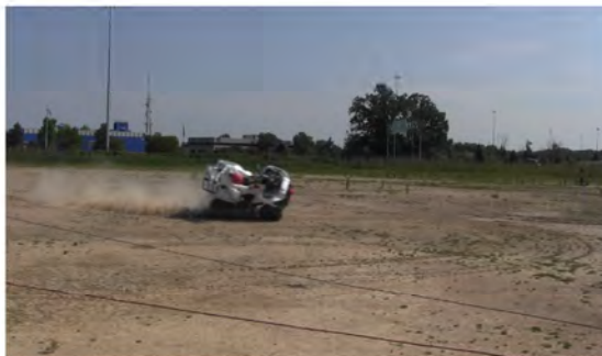
RT Camera 1 - Roll Angle = 45° - Time = 1.33 sec
