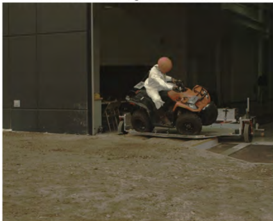
AOS Camera 2 - Roll Angle = 30° - Time = 0.53 sec
