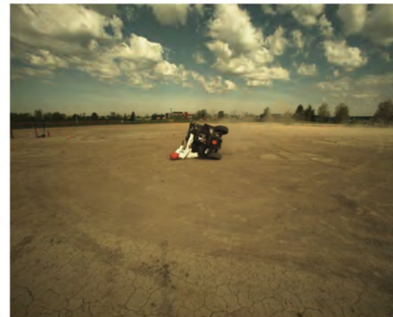
AOS Camera 2 - ATD Head Strike - Time = 2.72 sec
