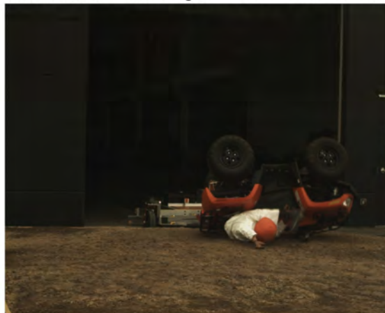
AOS Camera 1 - Max Angle = 157.9° - Time = 1.7 sec
