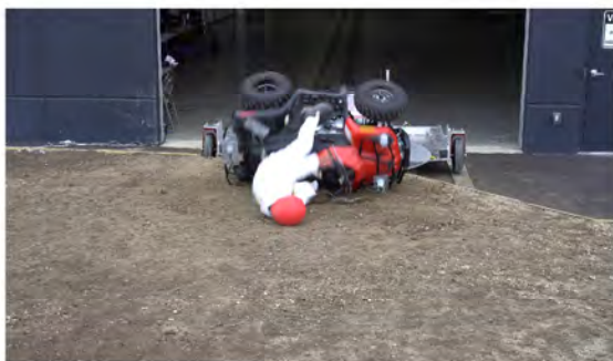
Drone Camera - ATD Head Strike - Time = 1.02 sec
