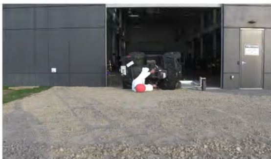
RT Camera 2 - ATD Head Strike - Time = 1.28 sec
