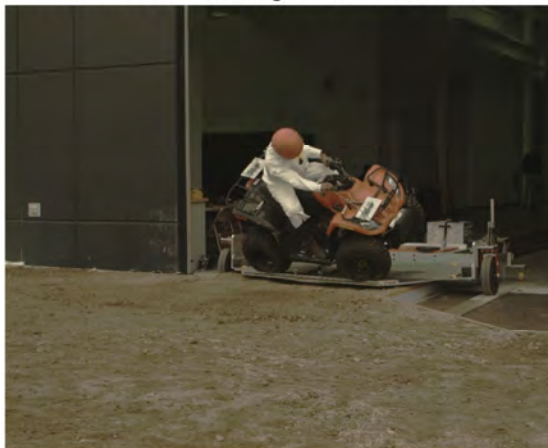
AOS Camera 2 - Roll Angle = 45° - Time = 0.64 sec
