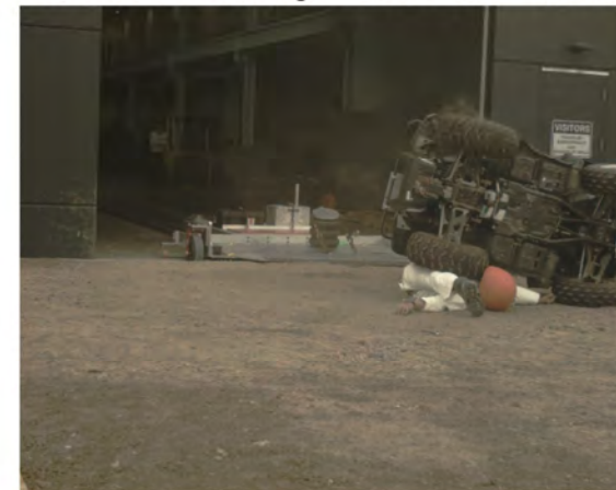
AOS Camera 1 - Max Angle = 274.8° - Time = 1.98 sec
