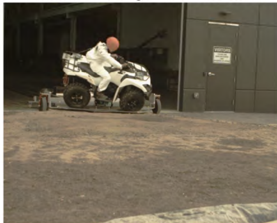
AOS Camera 1 - Roll Angle = 30° - Time = 0.55 sec
