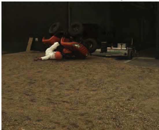
AOS Camera 2 - End of Run - Roll Angle = 139.2°
