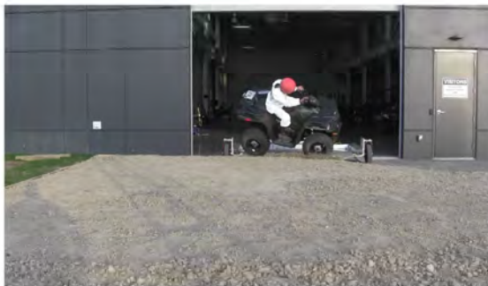
RT Camera 2 - Roll Angle = 30° - Time = 0.76 sec
