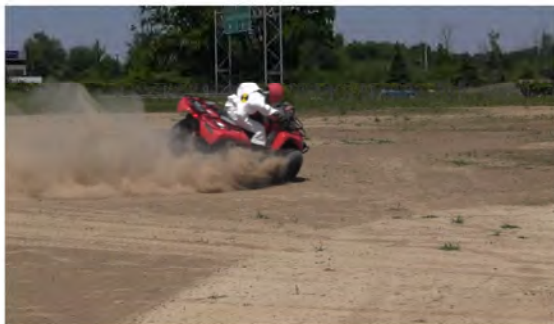
RT Camera 1 - Roll Angle = 30° - Time = 2.18 sec
