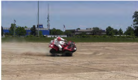
RT Camera 1 - Roll Angle = 30° - Time = 0.97 sec
