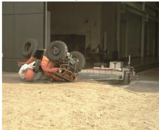
AOS Camera 2 - Max Angle = 154.8° - Time = 1.85 sec
