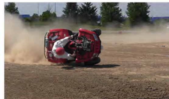
RT Camera 2 - Roll Angle = 90° - Time = 2.72 sec
