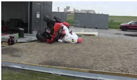
RT Camera 1 - ATD Head Strike - Time = 1.04 sec
