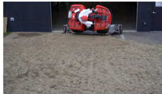
Drone Camera - Roll Angle = 90° - Time = 0.88 sec
