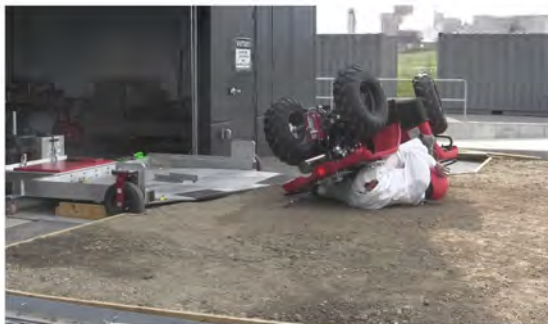
RT Camera 1 - Max Angle = 154.8° - Time = 1.85 sec
