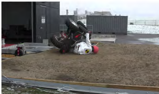
RT Camera 1 - Max Angle = 131.9° - Time = 1.77 sec
