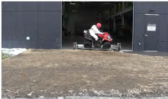
RT Camera 2 - Roll Angle = 30° - Time = 0.53 sec
