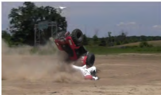
RT Camera 1 - Roll Angle = 180° - Time = 2.01 sec
