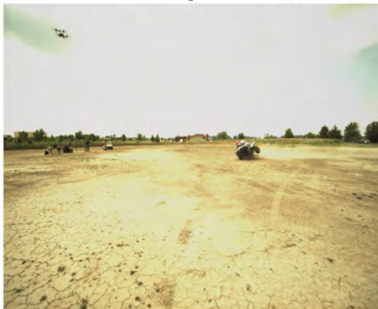
AOS Camera 2 - Roll Angle = 45° - Time = 1.14 sec
