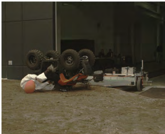
AOS Camera 1 - Roll Angle = 180° - Time = 1.18 sec
