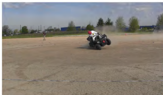
RT Camera 2 - Roll Angle = 30° - Time = 2.01 sec
