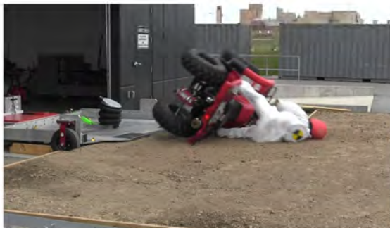
RT Camera 1 - ATD Head Strike - Time = 0.97 sec
