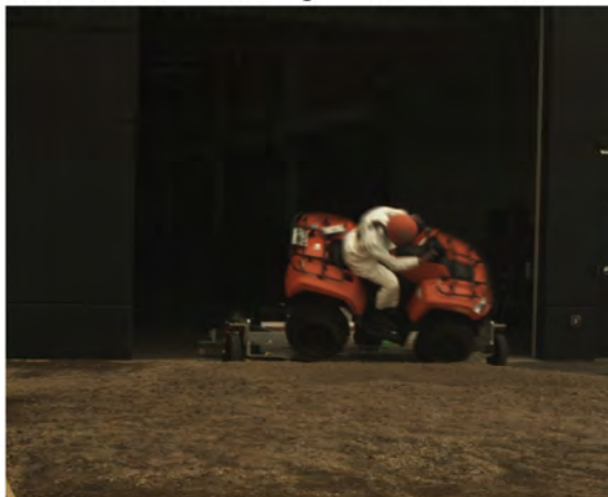
AOS Camera 1 - Roll Angle = 45° - Time = 0.66 sec
