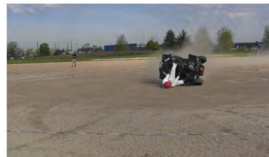
RT Camera 2 - ATD Head Strike - Time = 2.72 sec
