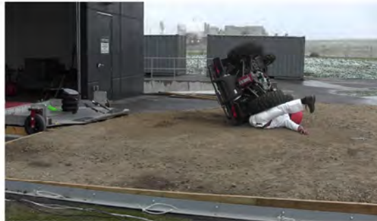
RT Camera 1 - End of Run - Roll Angle = 241.0°
