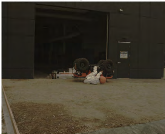
AOS Camera 1 - Roll Angle = 180° - Time = 1.15 sec
