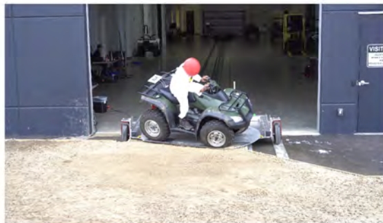
Drone Camera - Roll Angle = 30° - Time = 0.69 sec
