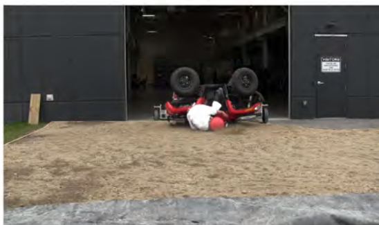
RT Camera 2 - Roll Angle = 180° - Time = 1.25 sec
