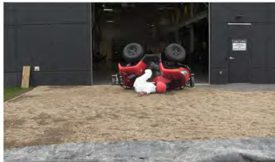
RT Camera 2 - End of Run - Roll Angle = 139.2°
