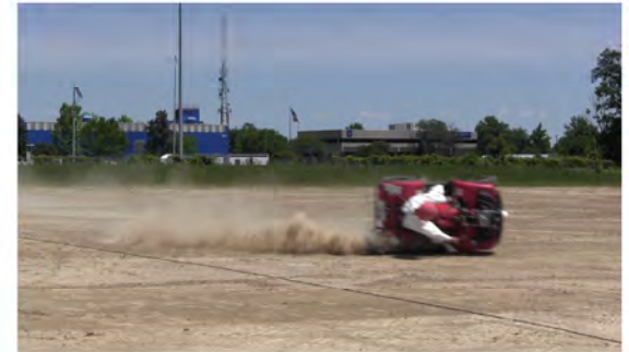
RT Camera 1 - Roll Angle = 90° - Time = 1.27 sec
