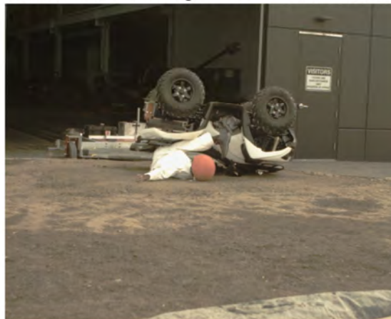
AOS Camera 1 - Max Angle = 164.5° - Time = 1.96 sec
