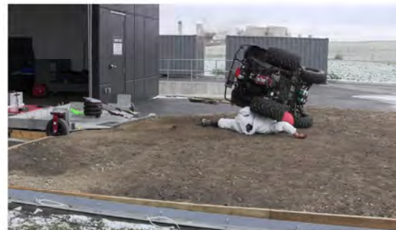
RT Camera 1 - Max Angle = 281.6° - Time = 2.48 sec
