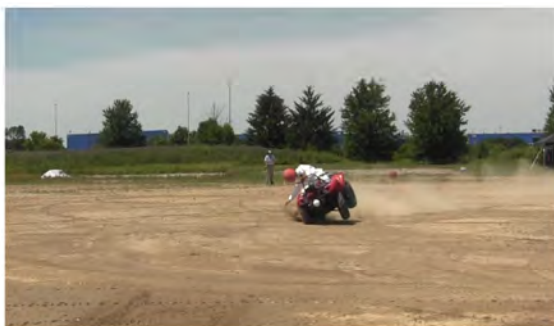
RT Camera 2 - Roll Angle = 30° - Time = 1.19 sec
