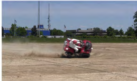
RT Camera 1 - Roll Angle = 45° - Time = 1.08 sec
