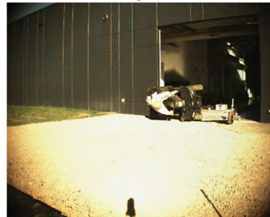
AOS Camera 2 - Roll Angle = 90° - Time = 0.79 sec
