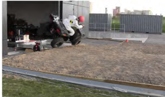
RT Camera 1 - Roll Angle = 45° - Time = 0.86 sec
