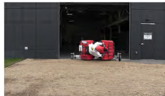
RT Camera 2 - Roll Angle = 90° - Time = 0.85 sec
