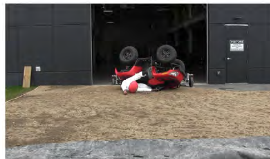
RT Camera 2 - End of Run - Roll Angle = 151.9°
