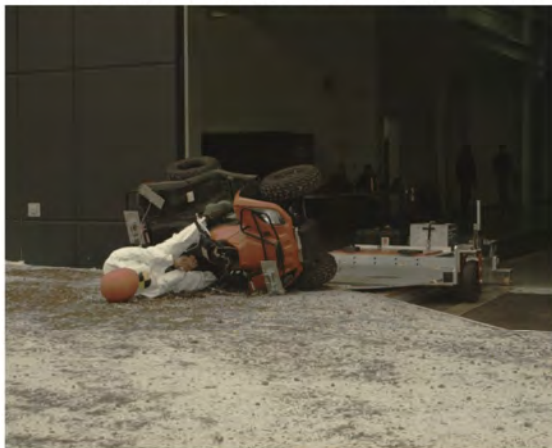
AOS Camera 2 - ATD Head Strike - Time = 1.13 sec
