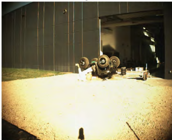
AOS Camera 2 - Roll Angle = 180° - Time = 1.1 sec
