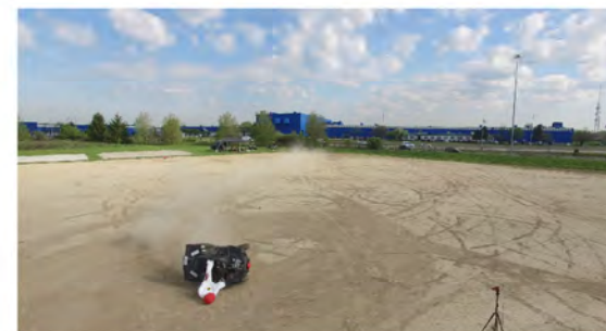
Drone Camera - ATD Head Strike - Time = 2.72 sec
