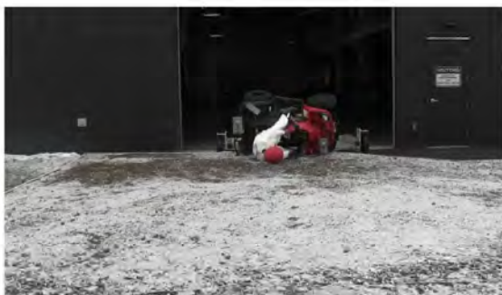
RT Camera 2 - ATD Head Strike - Time = 1.13 sec
