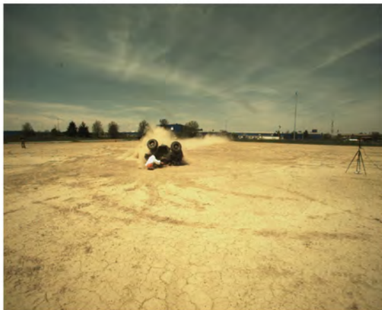
AOS Camera 1 - ATD Head Strike - Time = 1.95 sec
