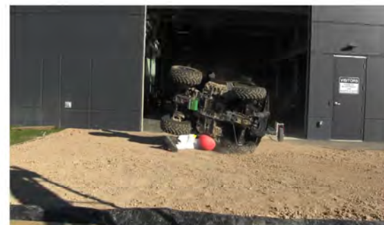
RT Camera 2 - Roll Angle = 270° - Time = 1.56 sec
