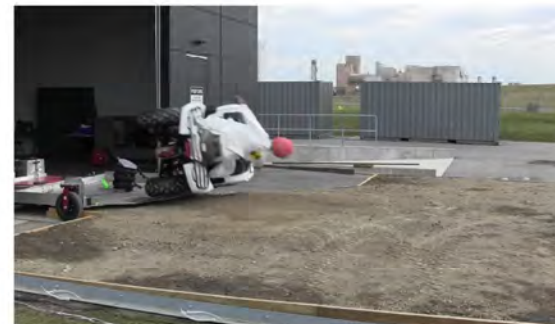
RT Camera 1 - Roll Angle = 90° - Time = 0.76 sec
