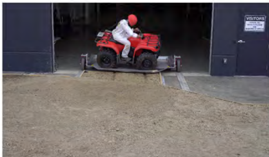
Drone Camera - Roll Angle = 30° - Time = 0.51 sec
