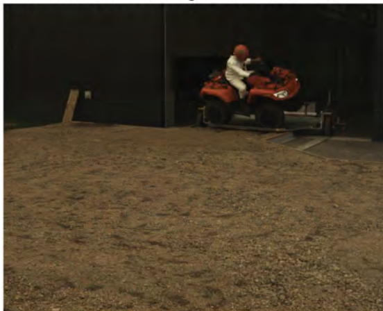
AOS Camera 2 - Roll Angle = 30° - Time = 0.51 sec
