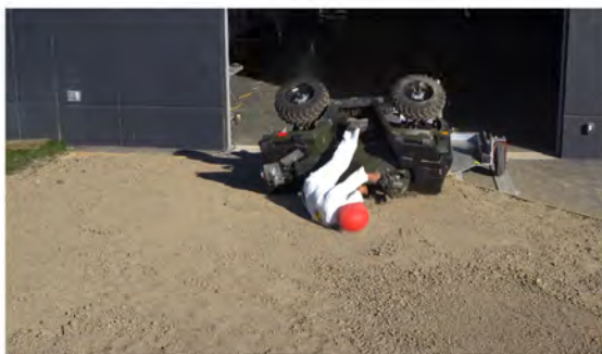
Drone Camera - ATD Head Strike - Time = 0.91 sec
