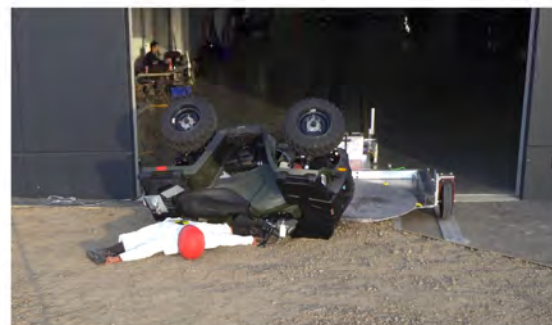
Drone Camera - End of Run - Roll Angle = 135.0°
