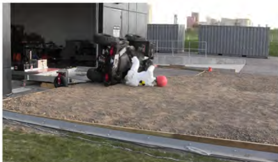
RT Camera 1 - ATD Head Strike - Time = 1.28 sec
