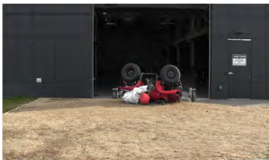
RT Camera 2 - Max Angle = 154.8° - Time = 1.85 sec
