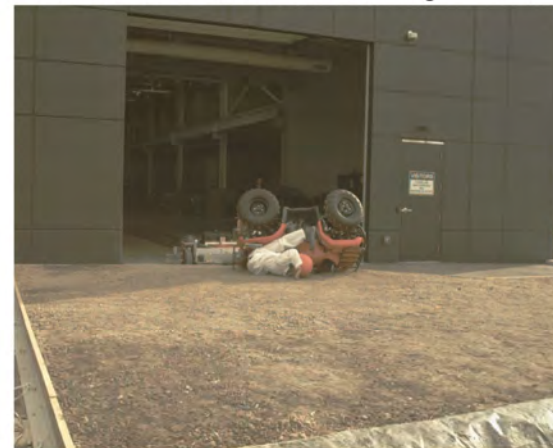
AOS Camera 1 - End of Run - Roll Angle = 144.4°
