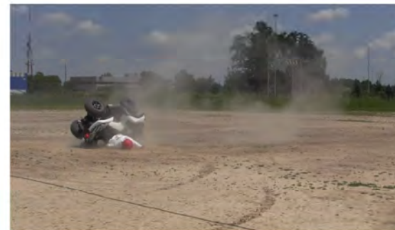
RT Camera 1 - End of Run - Roll Angle = 137.3°
