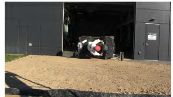
RT Camera 2 - Roll Angle = 90° - Time = 0.79 sec
