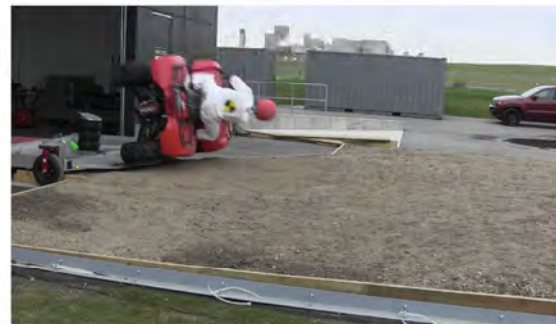
RT Camera 1 - Roll Angle = 90° - Time = 0.88 sec
