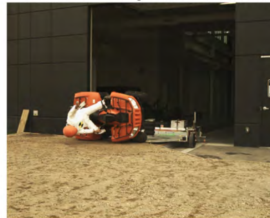
AOS Camera 2 - Roll Angle = 90° - Time = 0.91 sec
