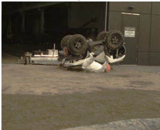
AOS Camera 1 - Roll Angle = 180° - Time = 1.18 sec
