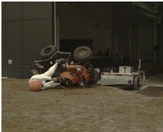
AOS Camera 2 - ATD Head Strike - Time = 1.02 sec
