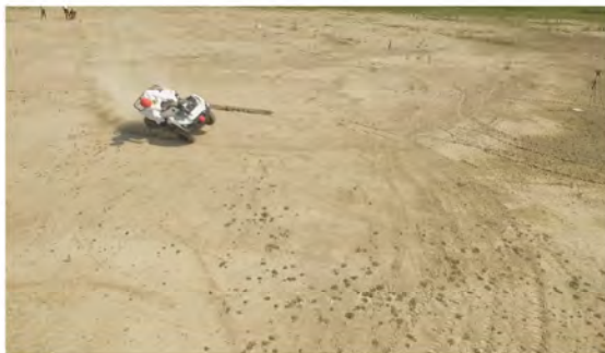
Drone Camera - Roll Angle = 30° - Time = 1.22 sec
