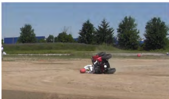
RT Camera 2 - ATD Head Strike - Time = 1.97 sec
