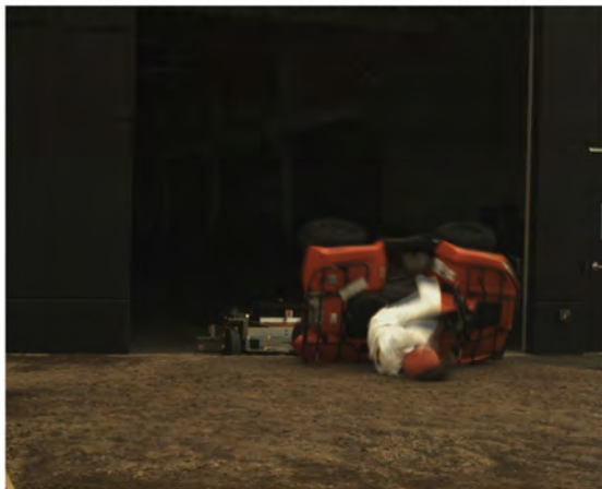
AOS Camera 1 - ATD Head Strike - Time = 0.99 sec
