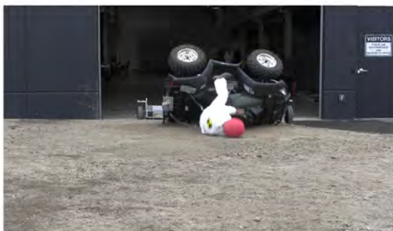
RT Camera 2 - ATD Head Strike - Time = 1.01 sec
