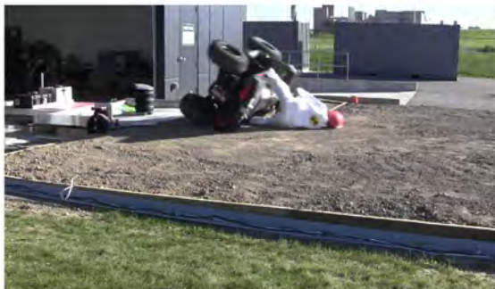
RT Camera 1 - ATD Head Strike - Time = 0.91 sec
