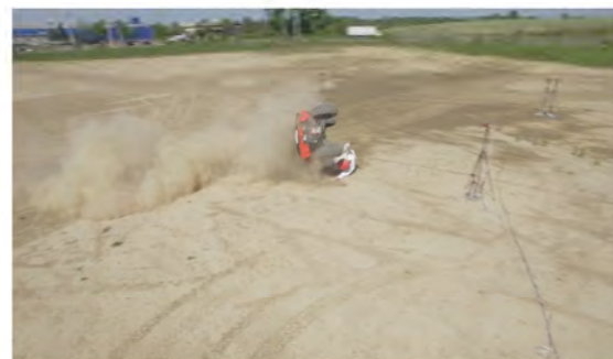
Drone Camera - Roll Angle = 270° - Time = 2.76 sec
