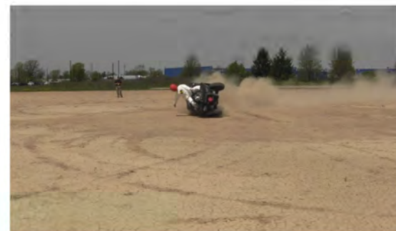
RT Camera 2 - Roll Angle = 90° - Time = 1.6 sec
