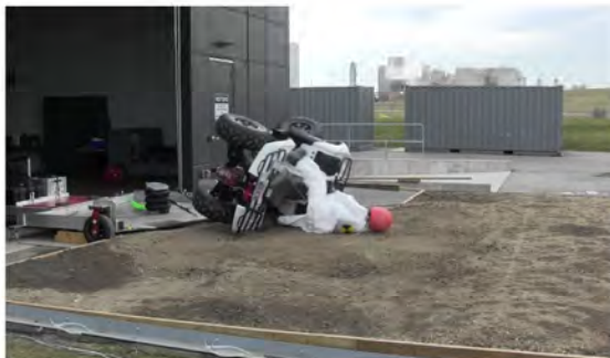
RT Camera 1 - ATD Head Strike - Time = 1.08 sec
