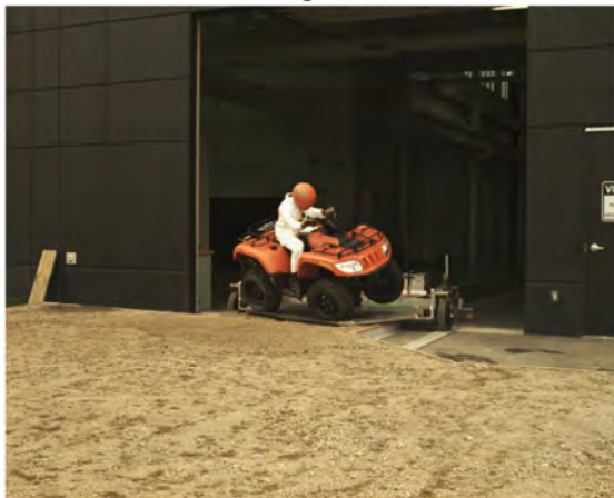
AOS Camera 2 - Roll Angle = 30° - Time = 0.53 sec
