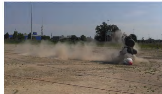
RT Camera 1 - Roll Angle = 270° - Time = 2.2 sec
