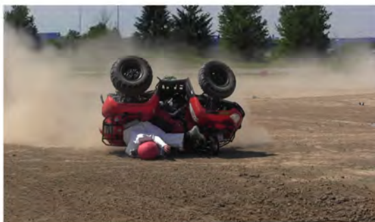
RT Camera 2 - Max Angle = 148.3° - Time = 3.44 sec
