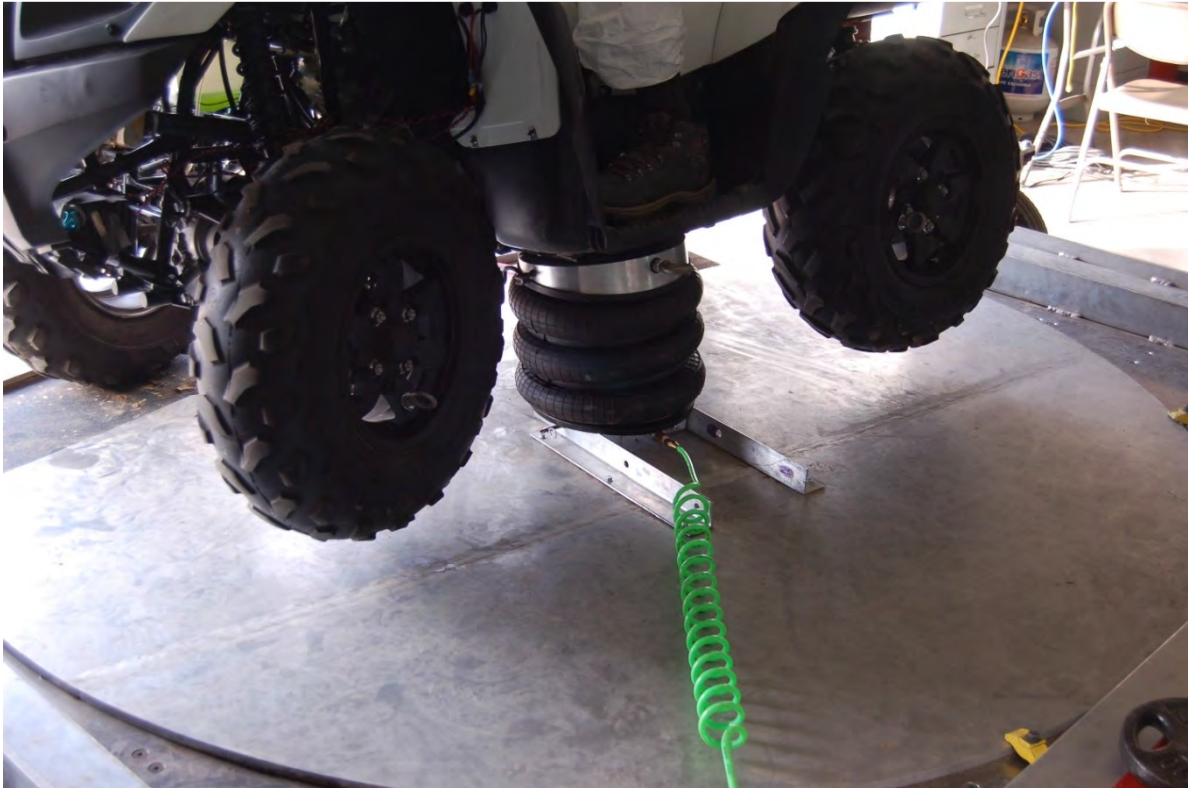
Figure F.5: Photo Showing Helper Spring used to Set ATV Initial Roll Angle
