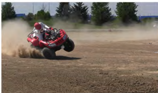
RT Camera 2 - Roll Angle = 30° - Time = 2.18 sec
