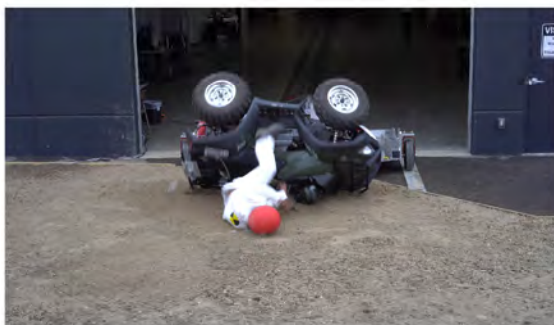
Drone Camera - ATD Head Strike - Time = 1.01 sec
