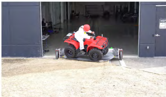
Drone Camera - Roll Angle = 30° - Time = 0.73 sec
