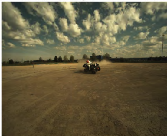
AOS Camera 1 - Roll Angle = 30° - Time = 2.01 sec
