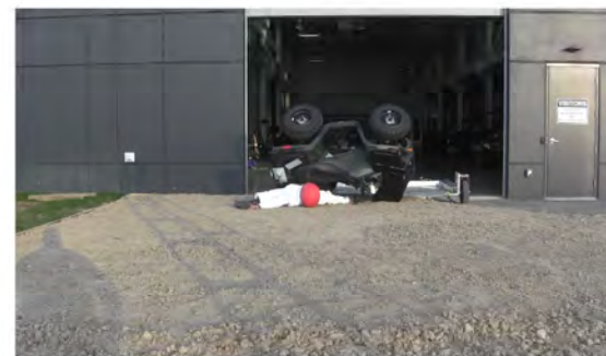
RT Camera 2 - End of Run - Roll Angle = 135.0°
