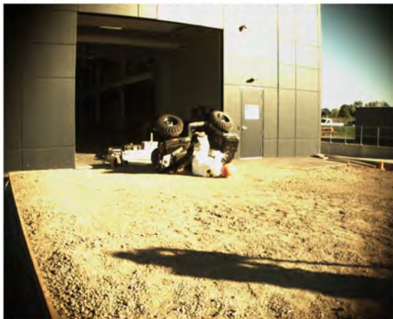
AOS Camera 1 - ATD Head Strike - Time = 0.91 sec
