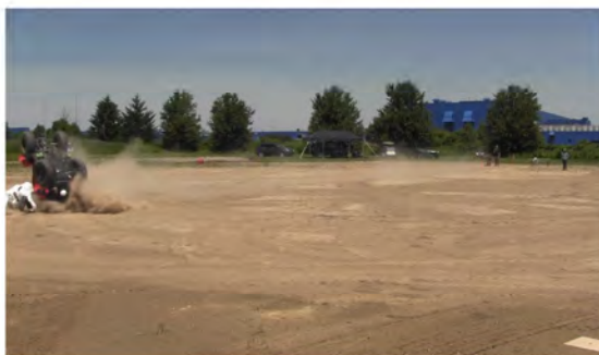
RT Camera 2 - Roll Angle = 180° - Time = 1.66 sec
