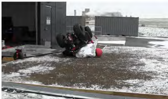
RT Camera 1 - Max Angle = 148.5° - Time = 1.7 sec
