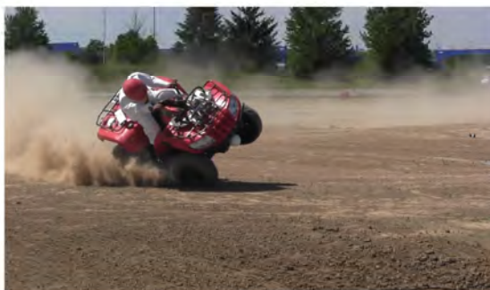
RT Camera 2 - Roll Angle = 45° - Time = 2.38 sec
