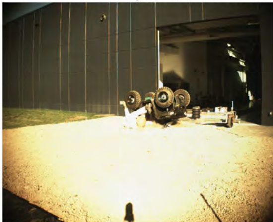
AOS Camera 1 - Roll Angle = 180° - Time = 1.1 sec
