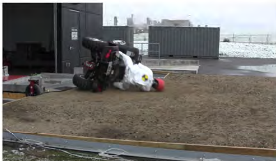
RT Camera 1 - ATD Head Strike - Time = 1.15 sec
