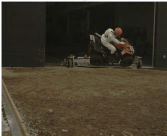
AOS Camera 1 - Roll Angle = 45° - Time = 0.64 sec
