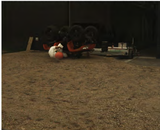
AOS Camera 2 - Roll Angle = 180° - Time = 1.25 sec
