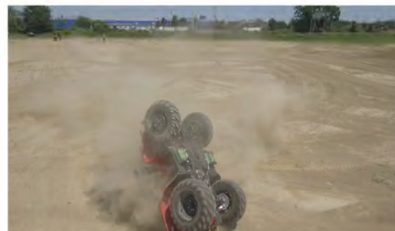
Drone Camera - Max Angle = 217.5° - Time = 2.38 sec
