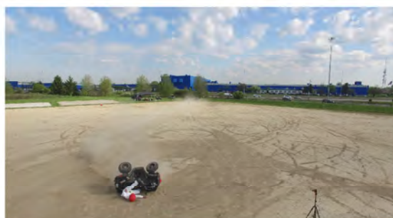
Drone Camera - Max Angle = 114.2° - Time = 3.26 sec
