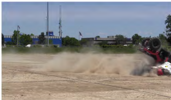
RT Camera 1 - Roll Angle = 180° - Time = 1.66 sec
