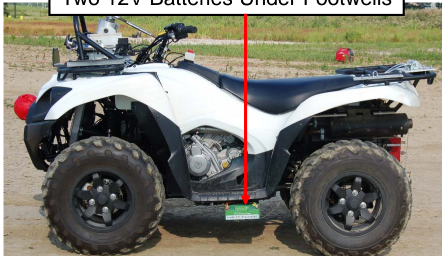
Two 12V Batteries Under Footwells
