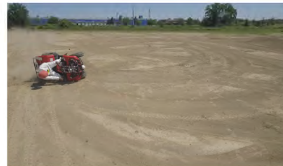
Drone Camera - Roll Angle = 90° - Time = 1.85 sec
