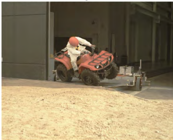
AOS Camera 2 - Roll Angle = 30° - Time = 0.73 sec
