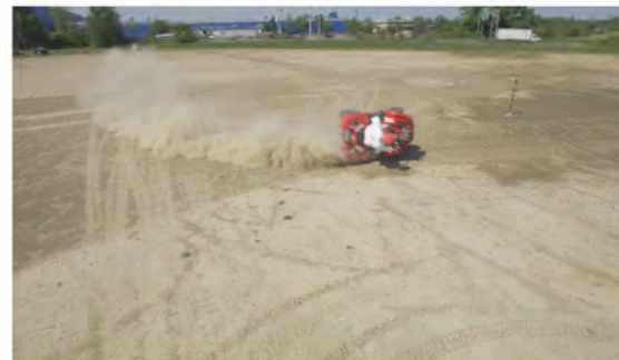
Drone Camera - Roll Angle = 90° - Time = 2.02 sec
