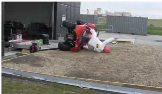
RT Camera 1 - ATD Head Strike - Time = 0.99 sec
