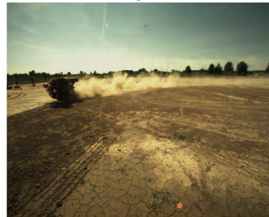
AOS Camera 2 - Roll Angle = 90° - Time = 2.02 sec
