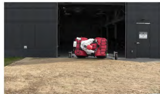
RT Camera 2 - Roll Angle = 90° - Time = 1.07 sec
