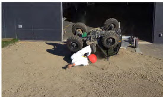
Drone Camera - Roll Angle = 180° - Time = 1.1 sec
