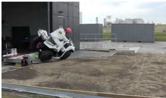
RT Camera 1 - Roll Angle = 45° - Time = 0.68 sec
