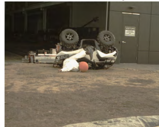
AOS Camera 1 - End of Run - Roll Angle = 148.4°
