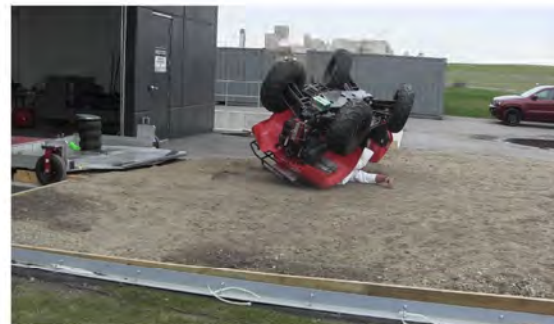
RT Camera 1 - Max Angle = 202.3° - Time = 2.16 sec
