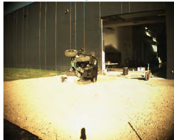
AOS Camera 2 - Roll Angle = 270° - Time = 1.56 sec
