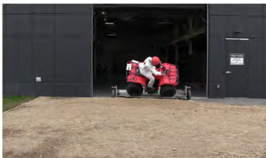
RT Camera 2 - Roll Angle = 45° - Time = 0.62 sec
