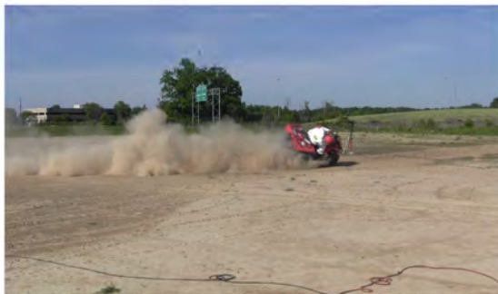
RT Camera 1 - Roll Angle = 45° - Time = 2.26 sec
