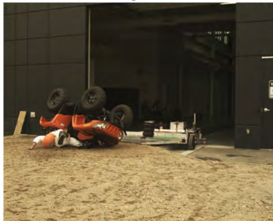
AOS Camera 2 - Max Angle = 157.9° - Time = 1.7 sec
