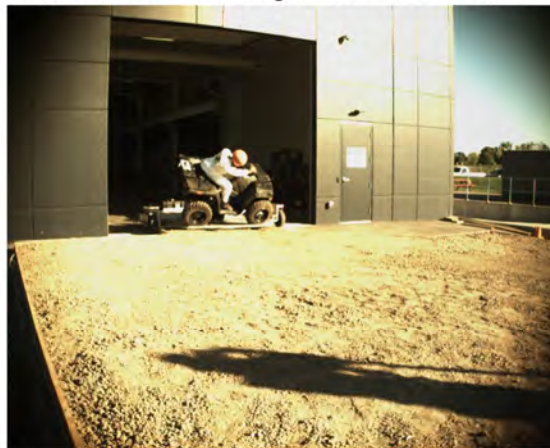
AOS Camera 1 - Roll Angle = 45° - Time = 0.56 sec
