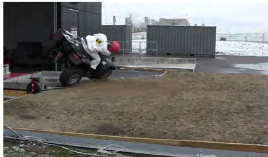
RT Camera 1 - Roll Angle = 45° - Time = 0.78 sec
