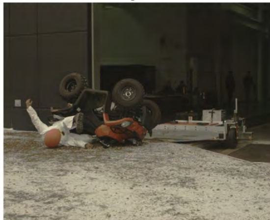
AOS Camera 2 - Max Angle = 148.5° - Time = 1.7 sec
