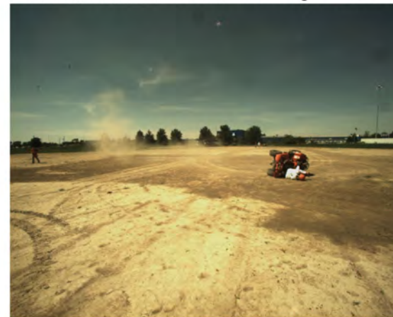
AOS Camera 1 - End of Run - Roll Angle = 102.5°
