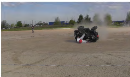
RT Camera 2 - Max Angle = 114.2^{\circ} - Time = 3.26 sec
