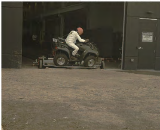
AOS Camera 1 - Roll Angle = 30° - Time = 0.46 sec
