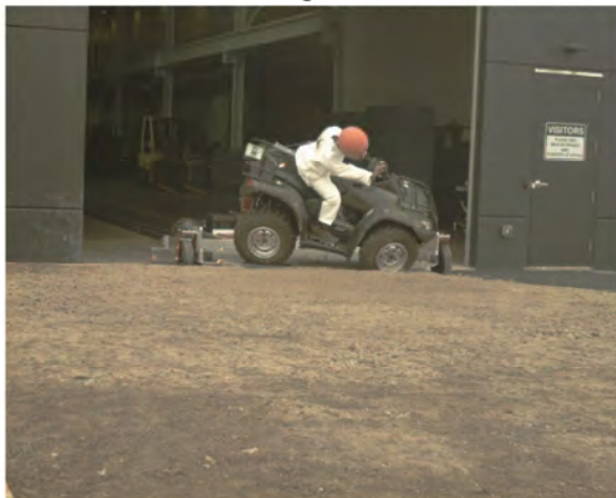
AOS Camera 1 - Roll Angle = 30° - Time = 0.69 sec
