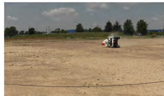
RT Camera 2 - Roll Angle = 90° - Time = 1.74 sec
