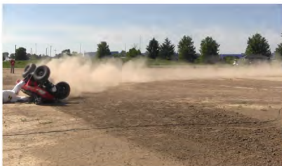
RT Camera 2 - ATD Head Strike - Time = 2.3 sec
