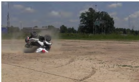
RT Camera 1 - Max Angle = 141.8° - Time = 2.42 sec
