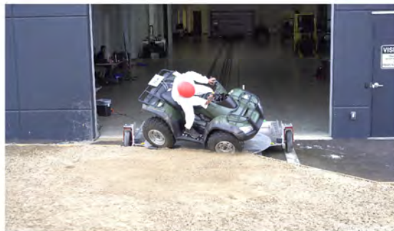
Drone Camera - Roll Angle = 45° - Time = 0.78 sec
