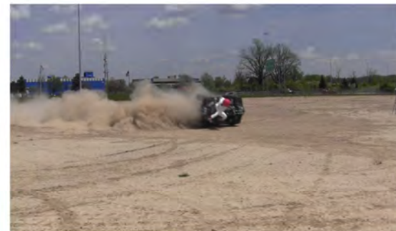
RT Camera 1 - Roll Angle = 90° - Time = 1.6 sec
