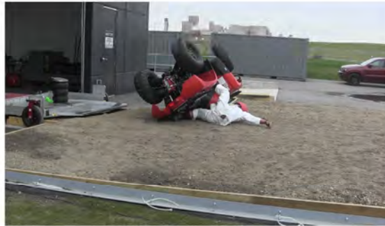
RT Camera 1 - End of Run - Roll Angle = 139.2°
