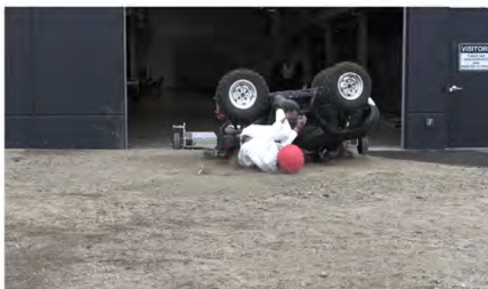
RT Camera 2 - Roll Angle = 180° - Time = 1.17 sec
