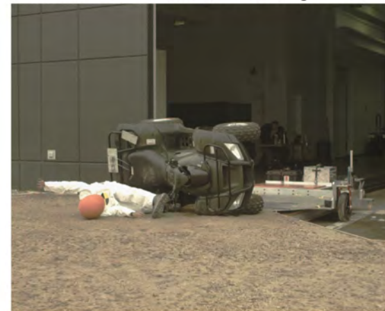
AOS Camera 2 - End of Run - Roll Angle = 94.6°
