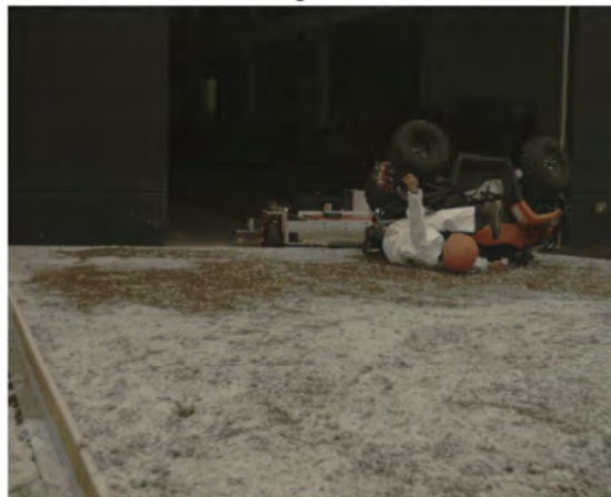
AOS Camera 1 - Max Angle = 148.5° - Time = 1.7 sec
