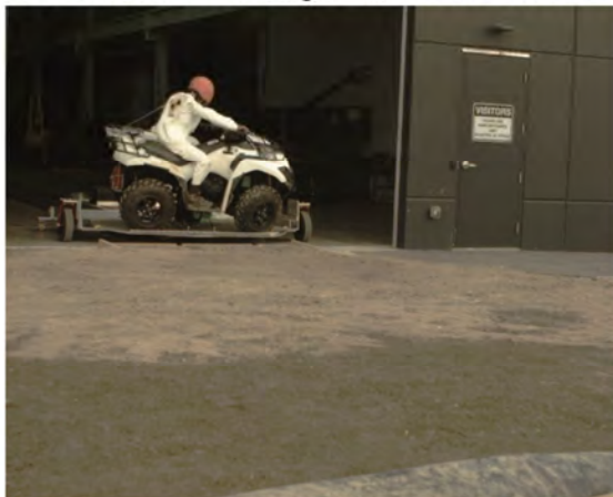
AOS Camera 1 - Roll Angle = 30° - Time = 0.41 sec
