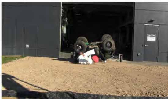
RT Camera 2 - Roll Angle = 180° - Time = 1.1 sec
