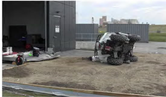
RT Camera 1 - End of Run - Roll Angle = 277.1°
