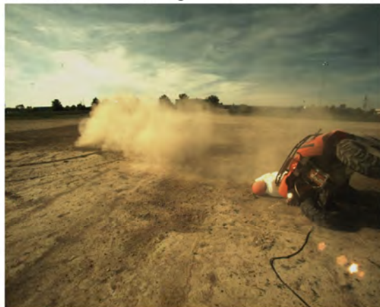
AOS Camera 1 - Max Angle = 294.4° - Time = 4.15 sec
