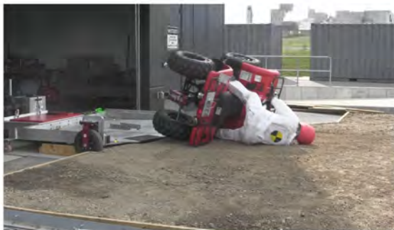
RT Camera 1 - ATD Head Strike - Time = 1.23 sec
