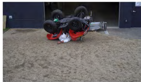
Drone Camera - Max Angle = 202.3° - Time = 2.16 sec
