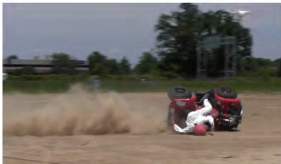
RT Camera 1 - ATD Head Strike - Time = 1.65 sec
