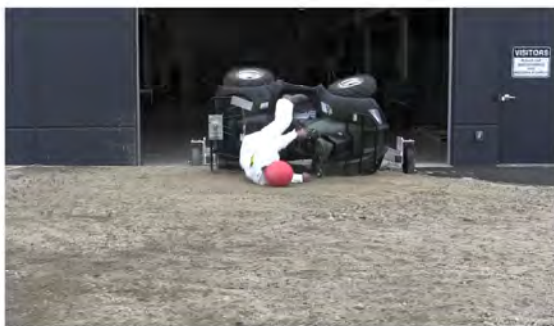
RT Camera 2 - ATD Head Strike - Time = 1.15 sec
