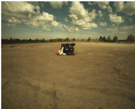
AOS Camera 2 - Roll Angle = 90° - Time = 2.8 sec
