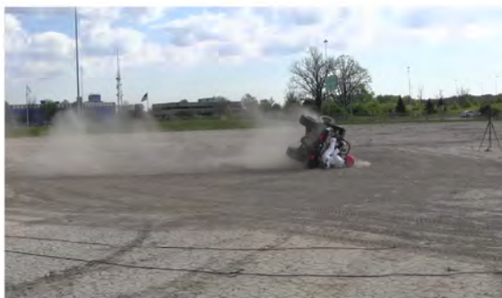
RT Camera 1 - Max Angle = 114.2^{\circ} - Time = 3.26 sec
