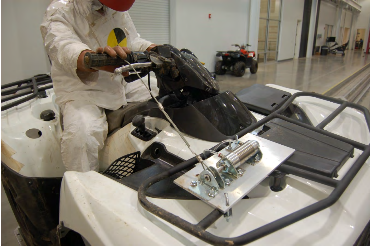
Figure E.7: Pneumatically Released Handhold used on Right Hand (Sled Vehicles F and G)
