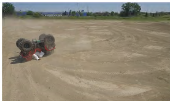
Drone Camera - Max Angle = 177.9° - Time = 3.24 sec
