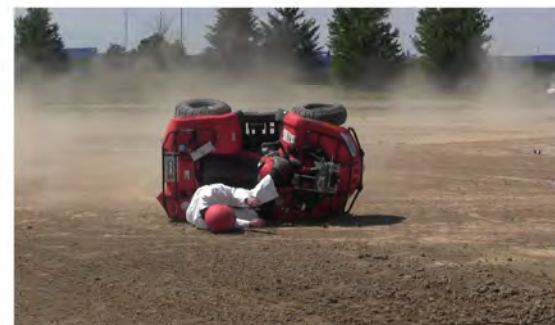
RT Camera 2 - End of Run - Roll Angle = 102.5°
