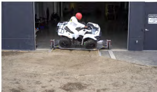
Drone Camera - Roll Angle = 45° - Time = 0.53 sec
