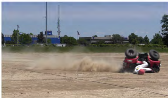
RT Camera 1 - ATD Head Strike - Time = 1.43 sec
