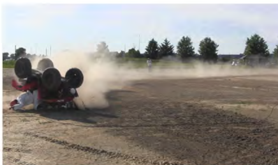
RT Camera 2 - Roll Angle = 180° - Time = 2.97 sec
