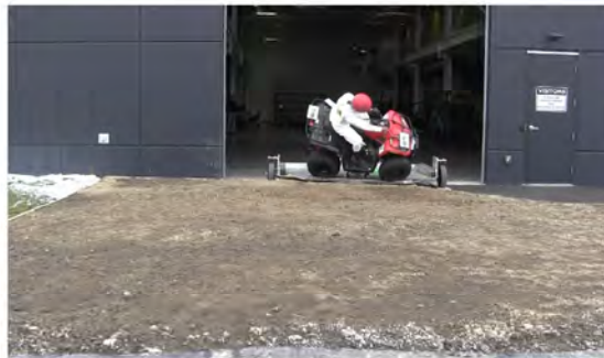
RT Camera 2 - Roll Angle = 45° - Time = 0.64 sec
