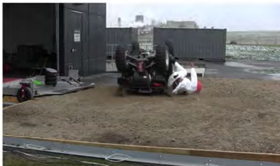
RT Camera 1 - Roll Angle = 180° - Time = 1.17 sec
