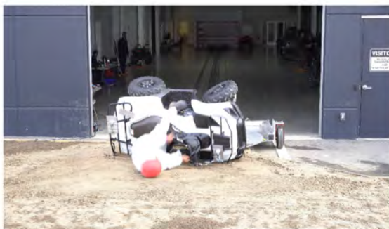
Drone Camera - ATD Head Strike - Time = 1.08 sec
