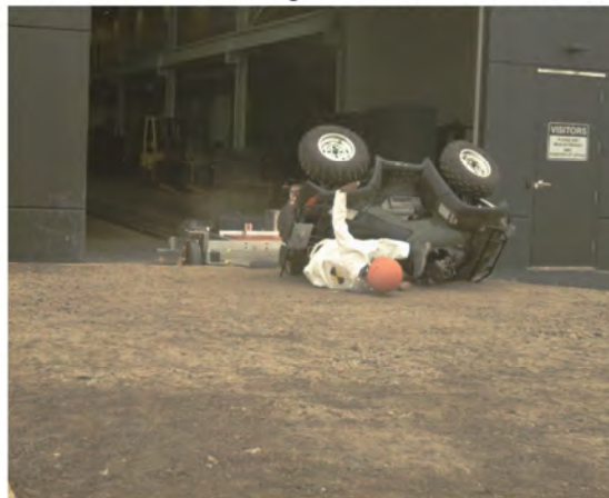
AOS Camera 1 - Max Angle = 131.9° - Time = 1.77 sec
