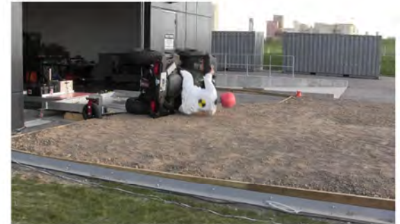
RT Camera 1 - Roll Angle = 90° - Time = 1.2 sec
