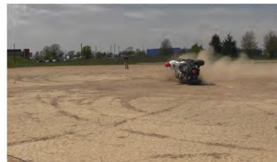
RT Camera 2 - Roll Angle = 90° - Time = 1.67 sec
