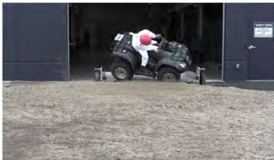
RT Camera 2 - Roll Angle = 30° - Time = 0.69 sec
