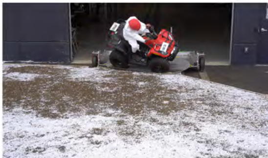
Drone Camera - Roll Angle = 45° - Time = 0.77 sec
