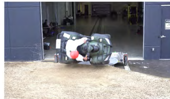
Drone Camera - Roll Angle = 90° - Time = 1.03 sec
