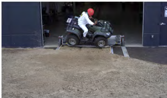
Drone Camera - Roll Angle = 45° - Time = 0.58 sec
