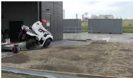
RT Camera 1 - Roll Angle = 30° - Time = 0.55 sec
