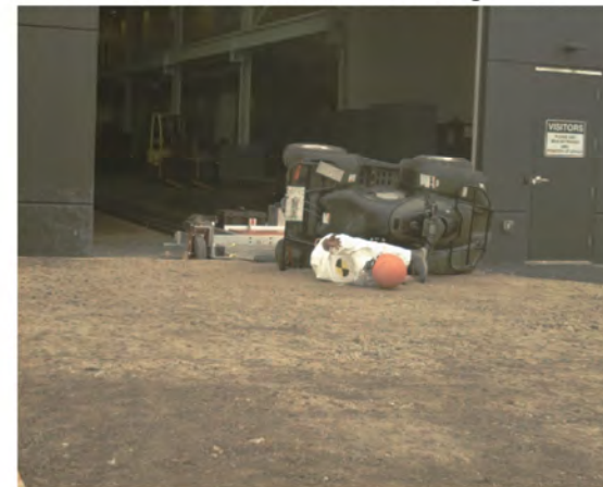
AOS Camera 1 - End of Run - Roll Angle = 94.6°
