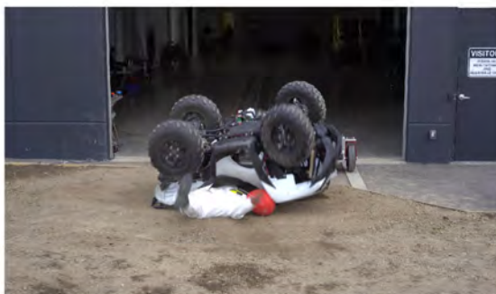
Drone Camera - Roll Angle = 180° - Time = 1.18 sec
