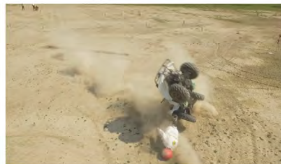
Drone Camera - Roll Angle = 270° - Time = 2.2 sec
