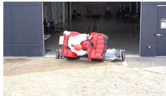
Drone Camera - Roll Angle = 90° - Time = 1.07 sec
