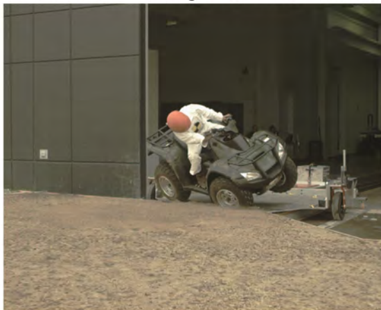
AOS Camera 2 - Roll Angle = 45° - Time = 0.78 sec
