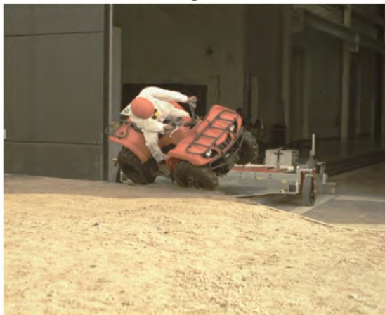
AOS Camera 2 - Roll Angle = 45° - Time = 0.82 sec
