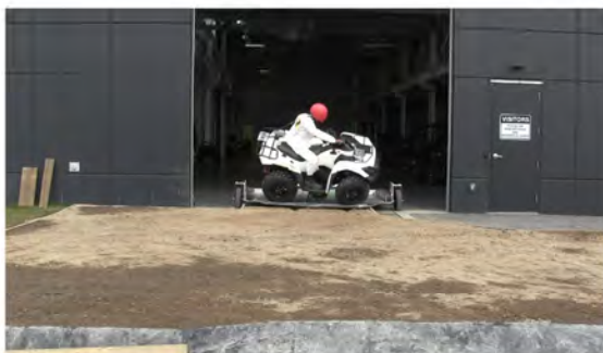
RT Camera 2 - Roll Angle = 30° - Time = 0.41 sec
