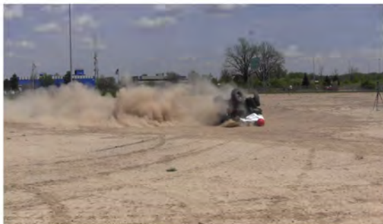
RT Camera 1 - ATD Head Strike - Time = 1.84 sec
