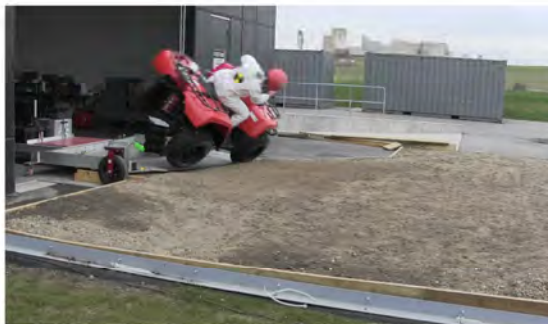
RT Camera 1 - Roll Angle = 45° - Time = 0.66 sec
