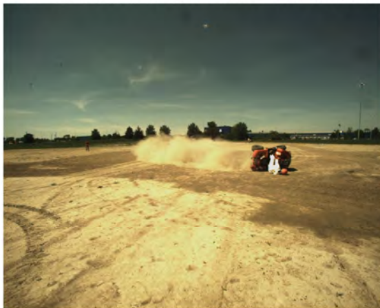
AOS Camera 1 - ATD Head Strike - Time = 2.84 sec
