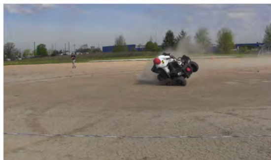
RT Camera 2 - Roll Angle = 45° - Time = 2.35 sec
