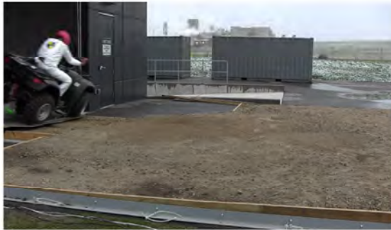
RT Camera 1 - Roll Angle = 30° - Time = 0.46 sec
