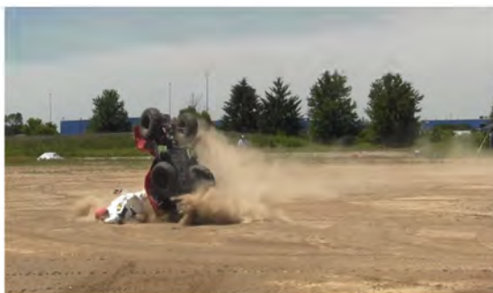
RT Camera 2 - Roll Angle = 180° - Time = 2.01 sec
