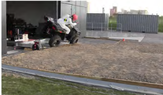
RT Camera 1 - Roll Angle = 30° - Time = 0.76 sec
