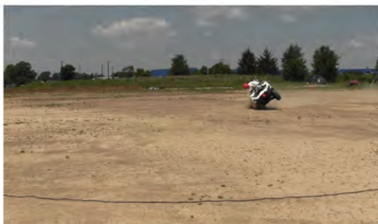
RT Camera 2 - Roll Angle = 45° - Time = 1.44 sec
