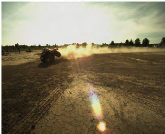
AOS Camera 2 - Roll Angle = 30° - Time = 2.05 sec
