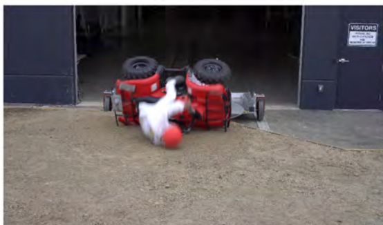
Drone Camera - ATD Head Strike - Time = 0.97 sec
