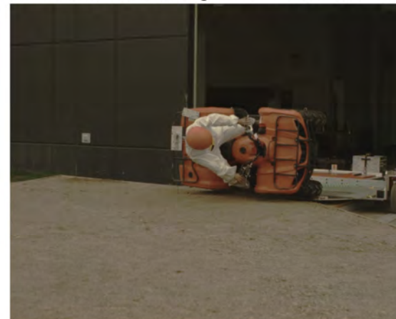
AOS Camera 2 - Roll Angle = 90° - Time = 0.85 sec
