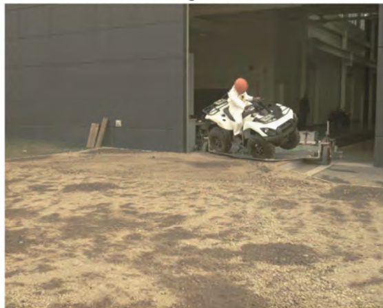
AOS Camera 2 - Roll Angle = 30° - Time = 0.55 sec
