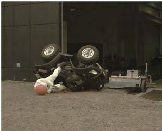
AOS Camera 2 - ATD Head Strike - Time = 1.01 sec
