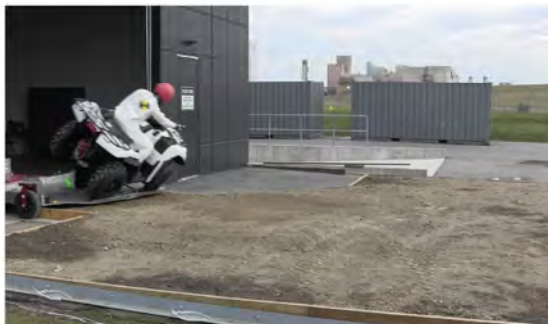
RT Camera 1 - Roll Angle = 45° - Time = 0.53 sec
