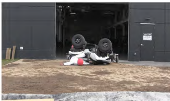
RT Camera 2 - Max Angle = 164.5° - Time = 1.96 sec
