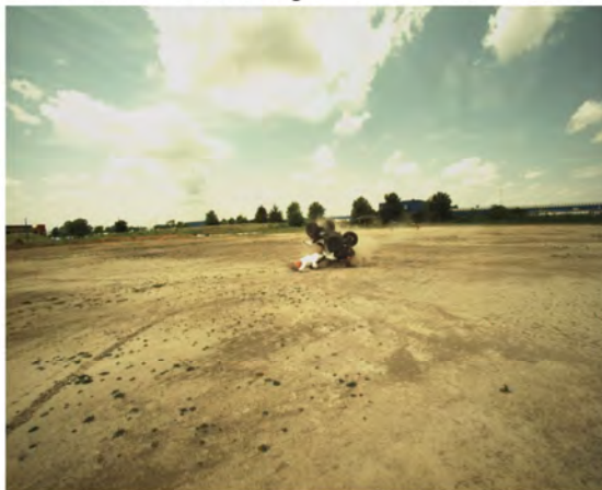
AOS Camera 1 - Roll Angle = 180° - Time = 1.69 sec
