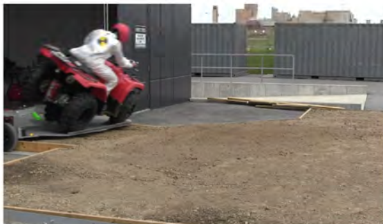
RT Camera 1 - Roll Angle = 30° - Time = 0.51 sec
