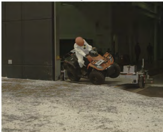
AOS Camera 2 - Roll Angle = 30° - Time = 0.67 sec
