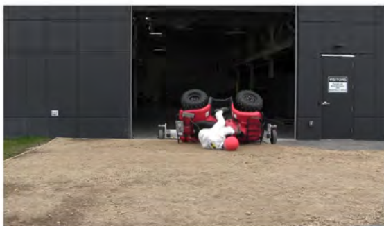
RT Camera 2 - ATD Head Strike - Time = 0.97 sec
