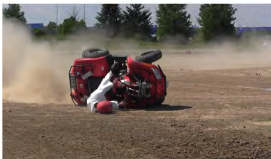
RT Camera 2 - ATD Head Strike - Time = 2.84 sec
