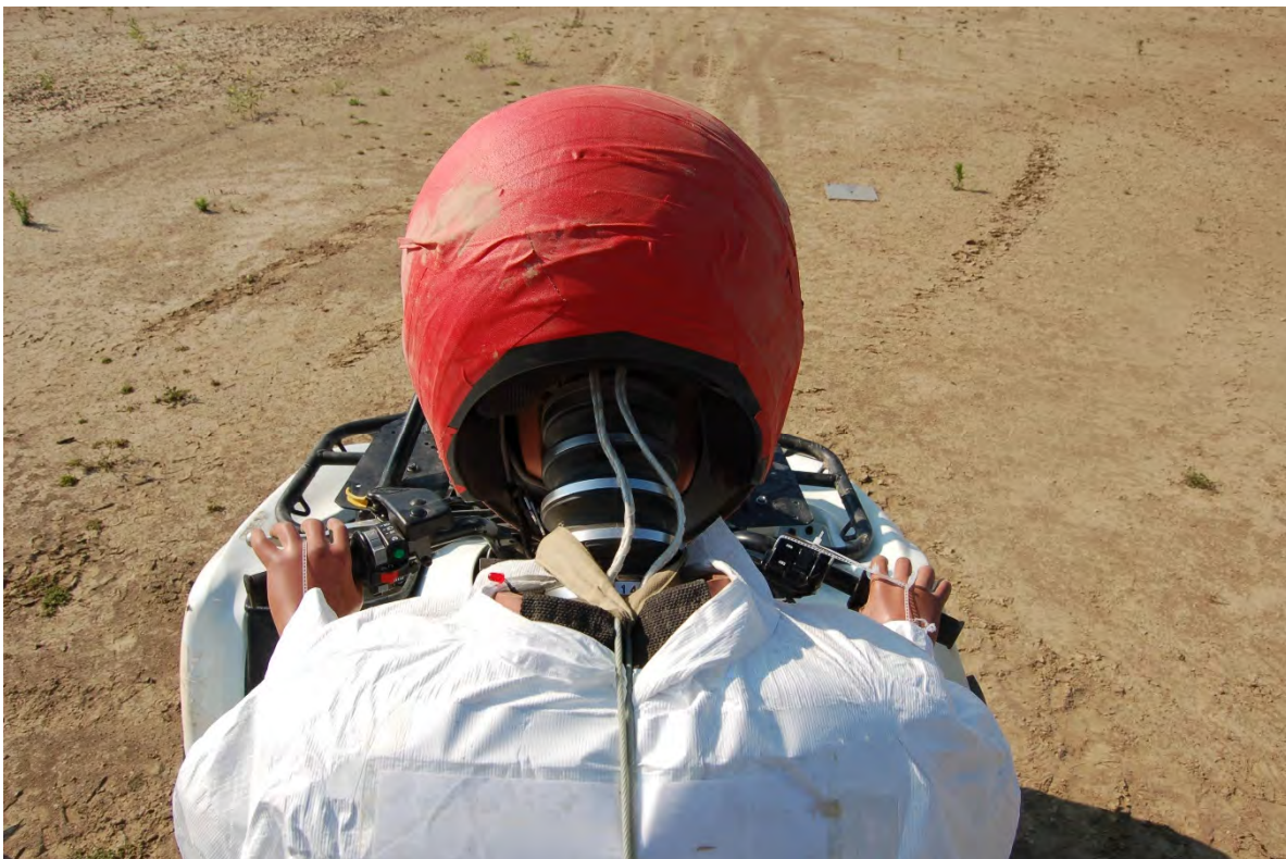
Figure E.6: Velcro Strap used for Attaching the Neck Cable to the ATD
