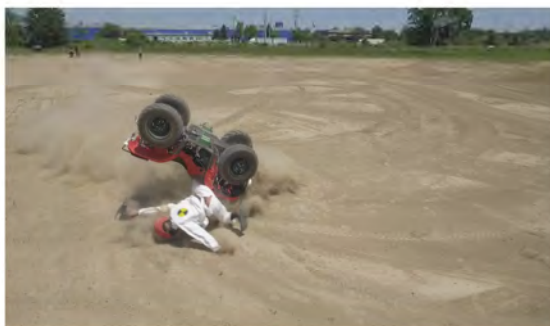
Drone Camera - Roll Angle = 180° - Time = 1.66 sec
