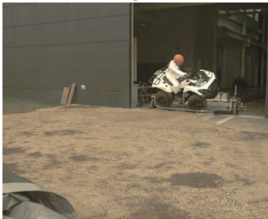
AOS Camera 2 - Roll Angle = 45° - Time = 0.53 sec
