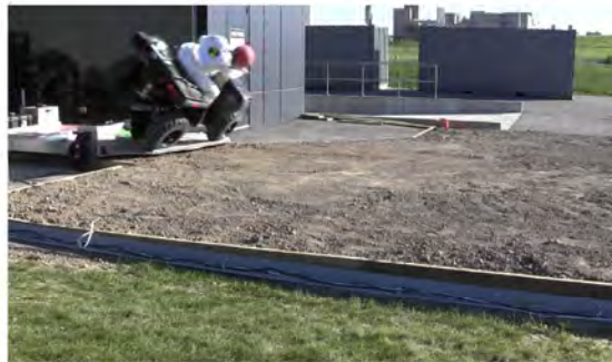
RT Camera 1 - Roll Angle = 45° - Time = 0.56 sec
