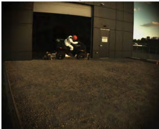
AOS Camera 1 - Roll Angle = 45° - Time = 0.86 sec
