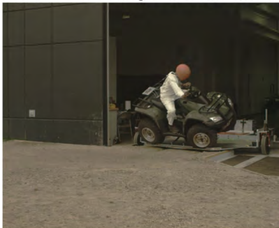
AOS Camera 2 - Roll Angle = 45° - Time = 0.58 sec
