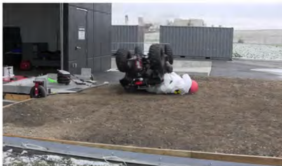
RT Camera 1 - Roll Angle = 180° - Time = 1.18 sec
