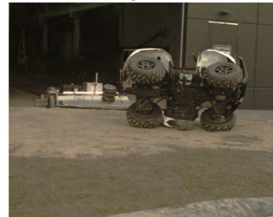
AOS Camera 1 - Max Angle = 297.7° - Time = 2.56 sec
