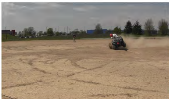
RT Camera 2 - Roll Angle = 30° - Time = 1.39 sec
