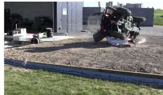
RT Camera 1 - Roll Angle = 270° - Time = 1.56 sec
