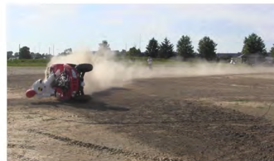
RT Camera 2 - Roll Angle = 90° - Time = 2.54 sec
