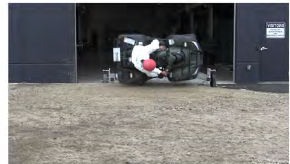
RT Camera 2 - Roll Angle = 90° - Time = 1.03 sec
