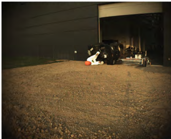
AOS Camera 2 - ATD Head Strike - Time = 1.28 sec
