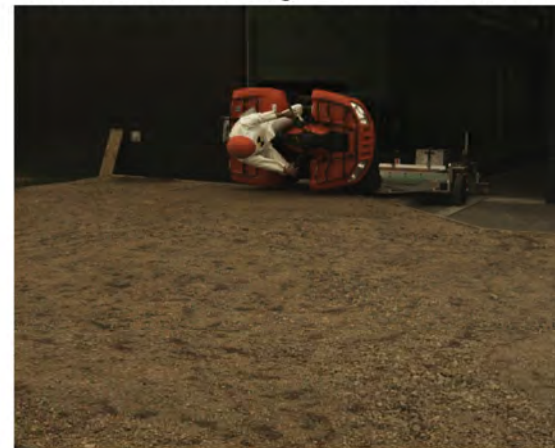
AOS Camera 2 - Roll Angle = 90° - Time = 0.88 sec
