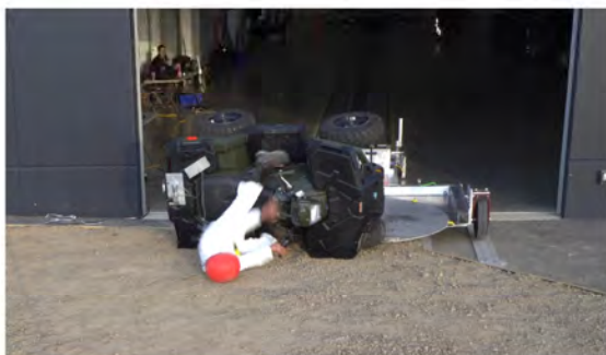
Drone Camera - ATD Head Strike - Time = 1.28 sec
