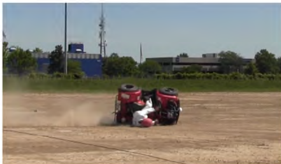
RT Camera 1 - ATD Head Strike - Time = 1.97 sec
