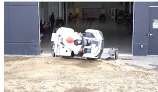
Drone Camera - Roll Angle = 90° - Time = 0.92 sec
