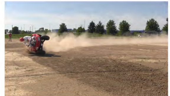
RT Camera 2 - Roll Angle = 90° - Time = 2.02 sec
