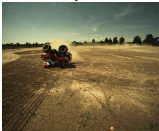
AOS Camera 2 - Max Angle = 148.3° - Time = 3.44 sec
