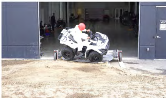
Drone Camera - Roll Angle = 45° - Time = 0.68 sec
