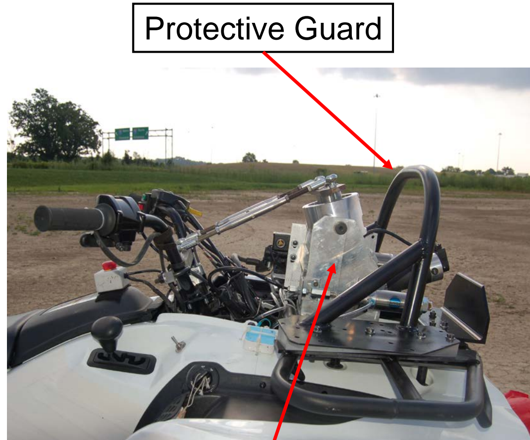
Steering Motor with 90° Gear Box and Coupler to Rods Connecting to Handlebars
