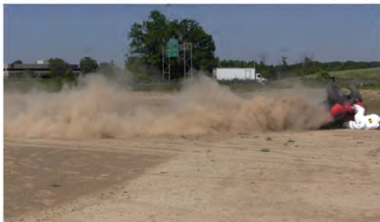
RT Camera 1 - ATD Head Strike - Time = 2.3 sec
