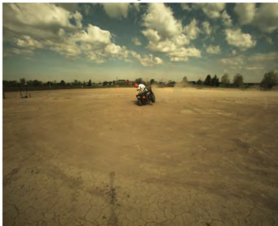
AOS Camera 2 - Roll Angle = 30° - Time = 2.01 sec
