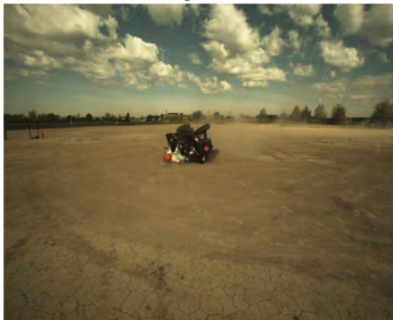
AOS Camera 2 - Max Angle = 114.2° - Time = 3.26 sec
