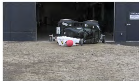
RT Camera 2 - End of Run - Roll Angle = 94.6°
