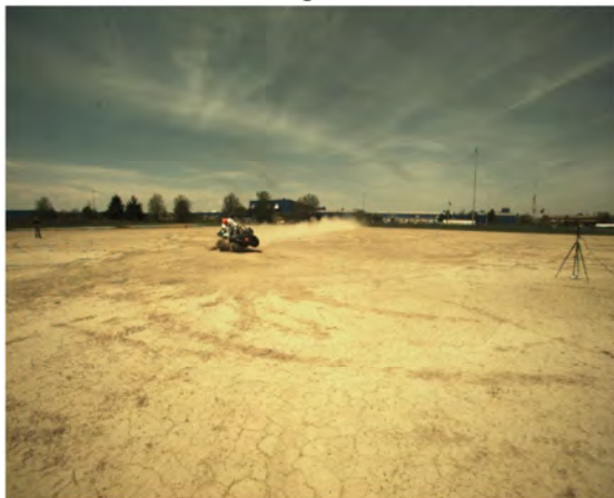
AOS Camera 1 - Roll Angle = 30° - Time = 1.39 sec
