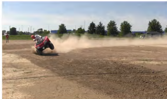
RT Camera 2 - Roll Angle = 45° - Time = 1.82 sec
