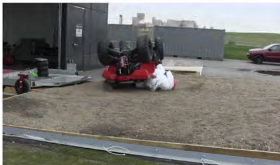
RT Camera 1 - Roll Angle = 180° - Time = 1.25 sec
