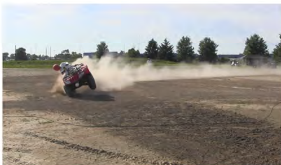
RT Camera 2 - Roll Angle = 30° - Time = 2.05 sec
