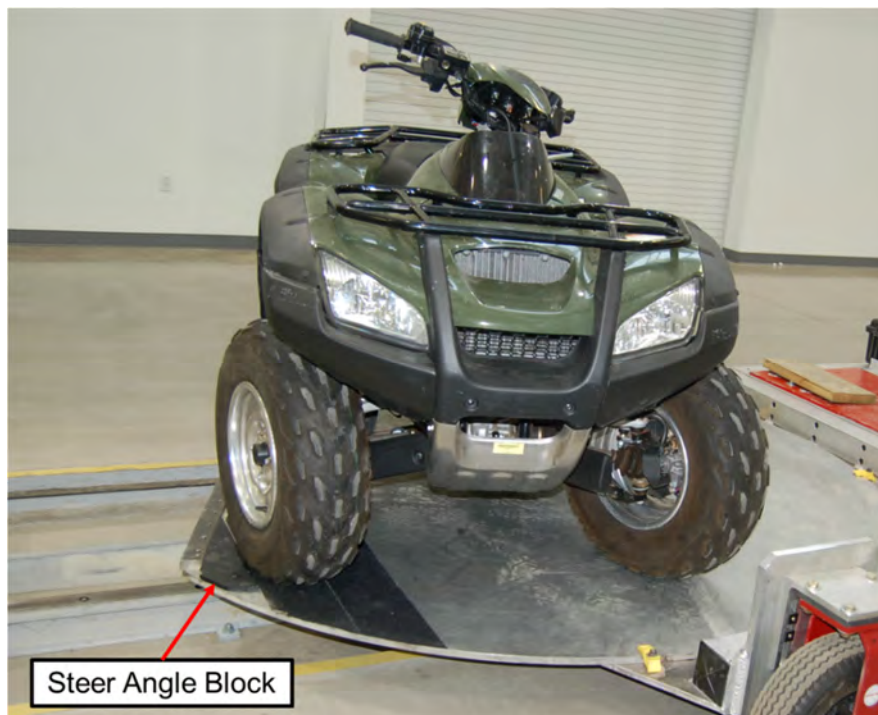
Figure F.5: Photo Showing Steer Angle Block
