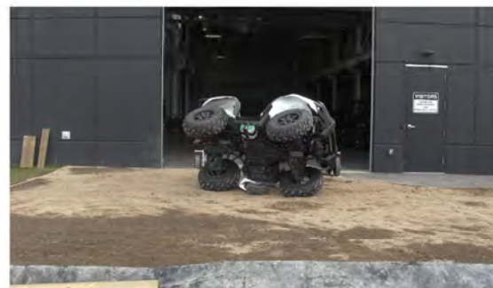
RT Camera 2 - Max Angle = 297.7° - Time = 2.56 sec
