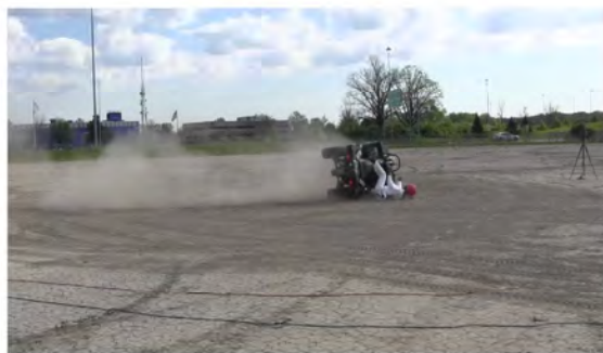
RT Camera 1 - Roll Angle = 90^{\circ} - Time = 2.8 sec
