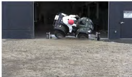
RT Camera 2 - Roll Angle = 45° - Time = 0.78 sec
