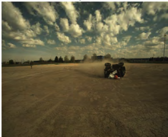
AOS Camera 1 - Max Angle = 114.2° - Time = 3.26 sec
