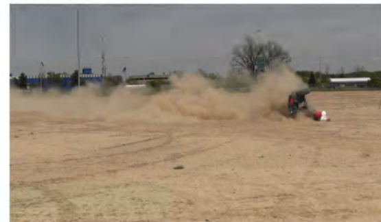
RT Camera 1 - Roll Angle = 270° - Time = 2.46 sec
