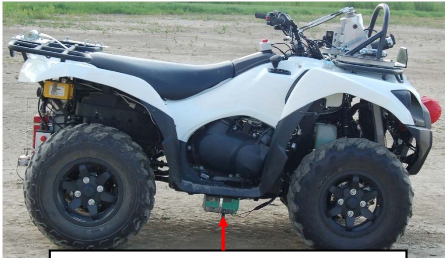
Two 12V Batteries Under Footwells
