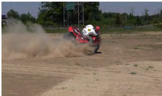
RT Camera 1 - Roll Angle = 45° - Time = 2.38 sec
