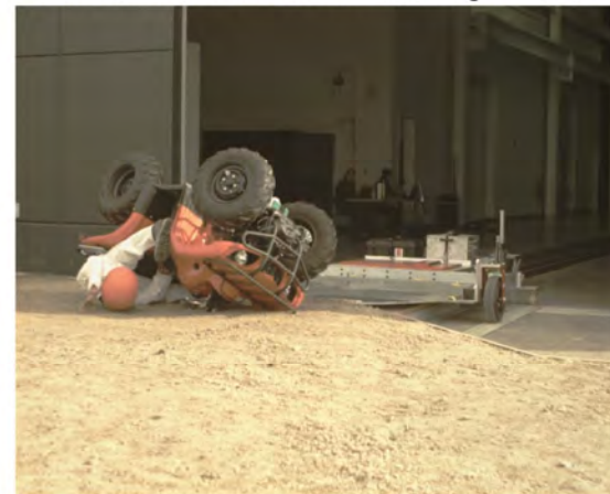
AOS Camera 2 - End of Run - Roll Angle = 144.4°
