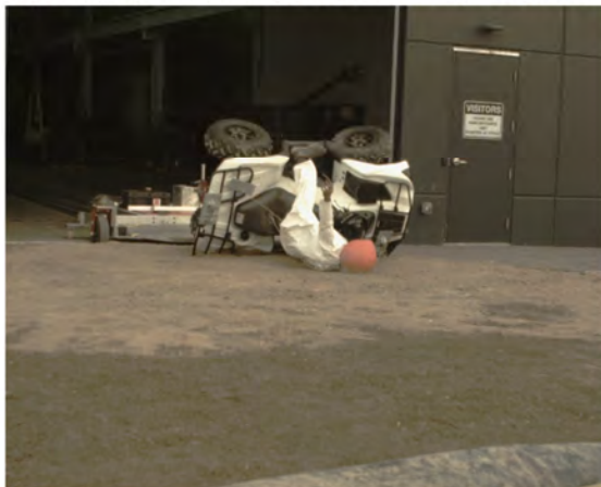
AOS Camera 1 - ATD Head Strike - Time = 0.88 sec
