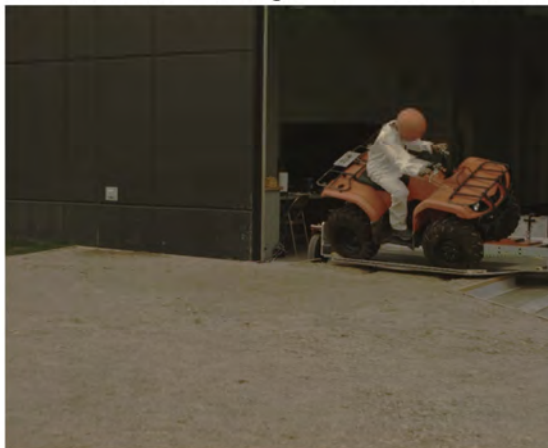
AOS Camera 2 - Roll Angle = 45° - Time = 0.62 sec
