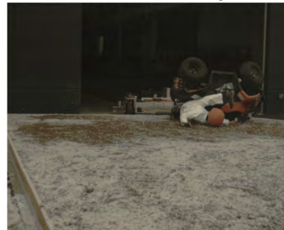
AOS Camera 1 - End of Run - Roll Angle = 141.8°
