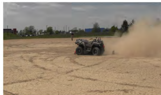
RT Camera 2 - End of Run - Roll Angle = 361.7^{\circ}
