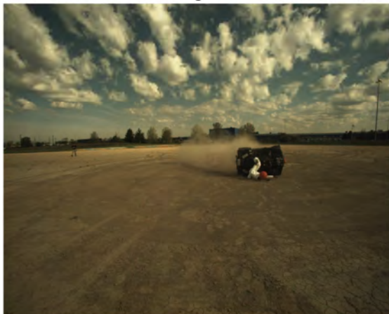
AOS Camera 1 - Roll Angle = 90° - Time = 2.8 sec
