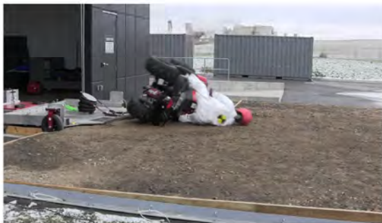
RT Camera 1 - ATD Head Strike - Time = 1.02 sec
