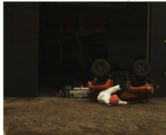
AOS Camera 1 - End of Run - Roll Angle = 151.9°
