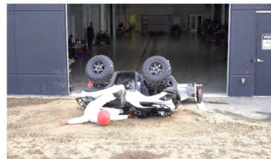
Drone Camera - End of Run - Roll Angle = 148.4°
