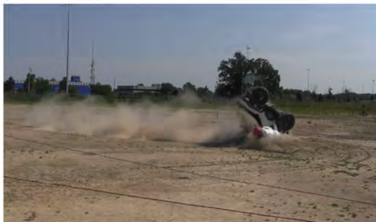
RT Camera 1 - Roll Angle = 180° - Time = 1.95 sec
