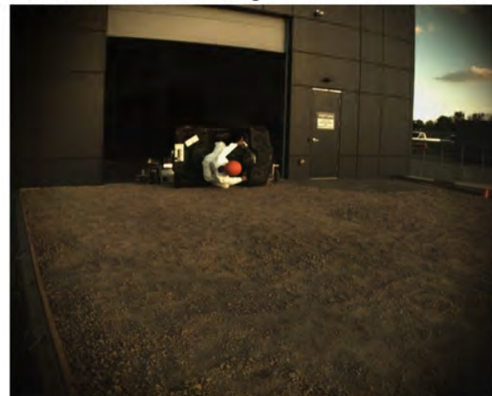
AOS Camera 1 - Roll Angle = 90° - Time = 1.2 sec
