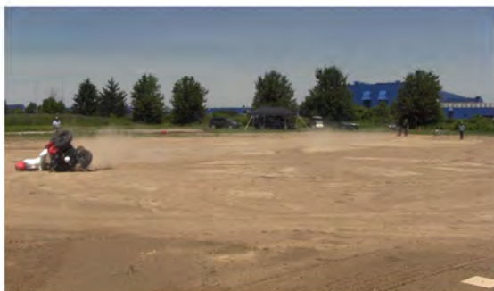
RT Camera 2 - ATD Head Strike - Time = 1.43 sec
