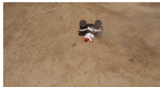
Drone Camera - End of Run - Roll Angle = 137.3°
