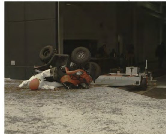
AOS Camera 2 - End of Run - Roll Angle = 141.8°
