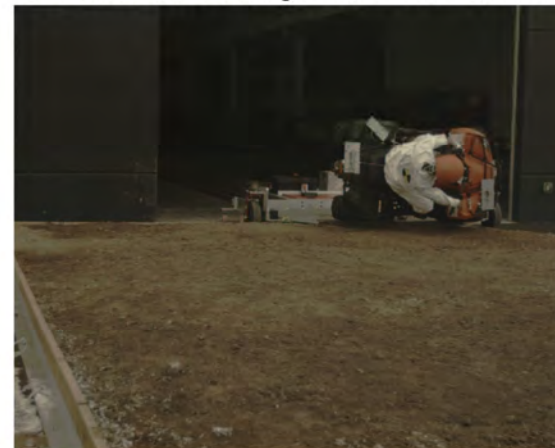
AOS Camera 1 - Roll Angle = 90° - Time = 0.86 sec
