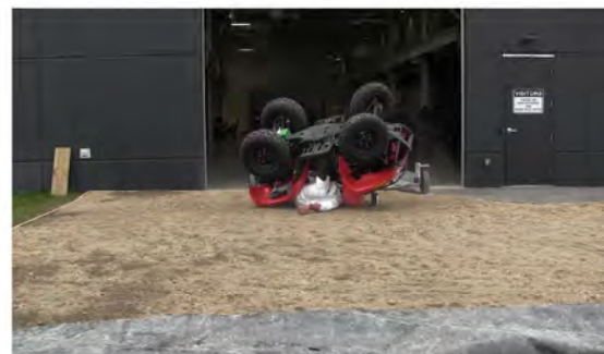
RT Camera 2 - Max Angle = 202.3° - Time = 2.16 sec
