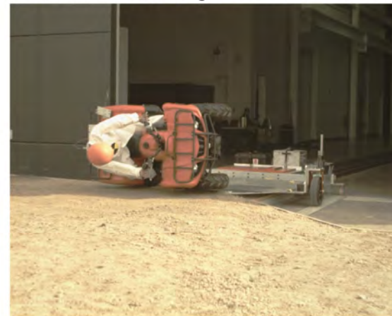
AOS Camera 2 - Roll Angle = 90° - Time = 1.07 sec
