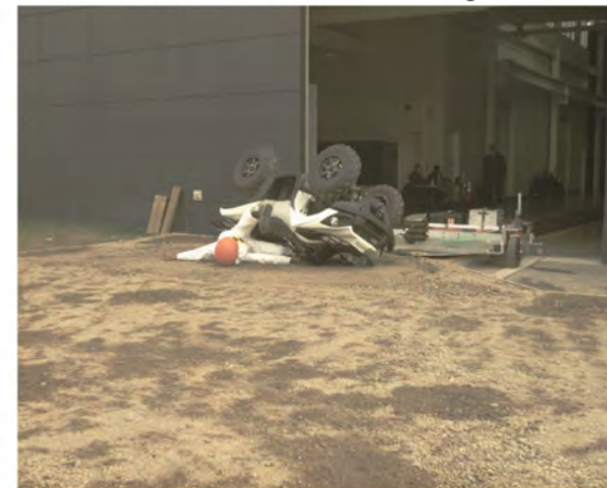
AOS Camera 2 - End of Run - Roll Angle = 148.4°
