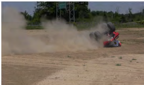
RT Camera 1 - Max Angle = 148.3° - Time = 3.44 sec
