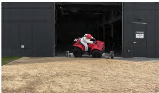
RT Camera 2 - Roll Angle = 30° - Time = 0.73 sec
