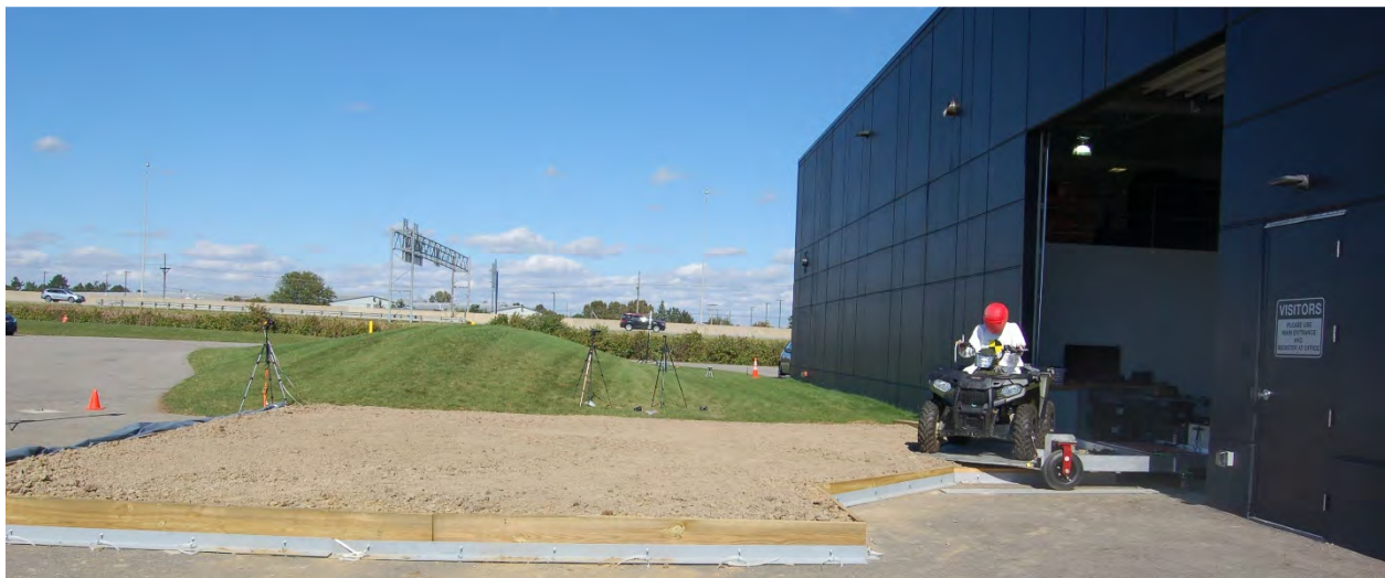
Figure F.2: View of ATV Rollover Simulator Landing Pit
