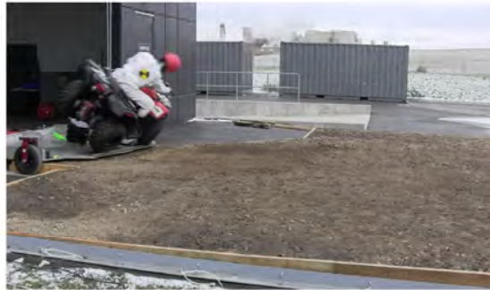
RT Camera 1 - Roll Angle = 45° - Time = 0.64 sec
