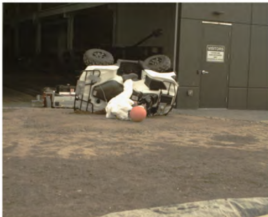
AOS Camera 1 - ATD Head Strike - Time = 1.08 sec
