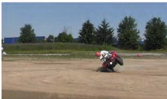
RT Camera 2 - Roll Angle = 45° - Time = 1.54 sec
