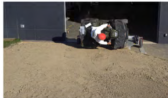
Drone Camera - Roll Angle = 90° - Time = 0.79 sec
