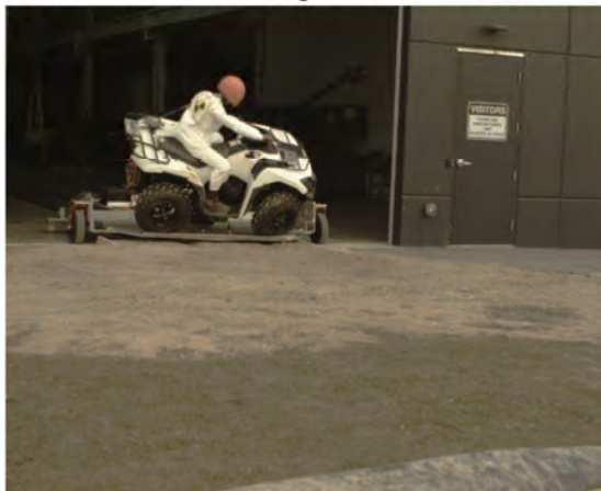
AOS Camera 1 - Roll Angle = 45° - Time = 0.53 sec
