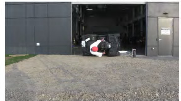
RT Camera 2 - Roll Angle = 90° - Time = 1.2 sec
