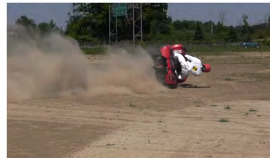
RT Camera 1 - Roll Angle = 90° - Time = 2.72 sec
