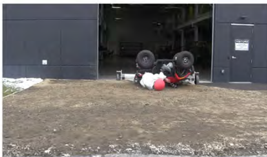
RT Camera 2 - Roll Angle = 180° - Time = 1.18 sec
