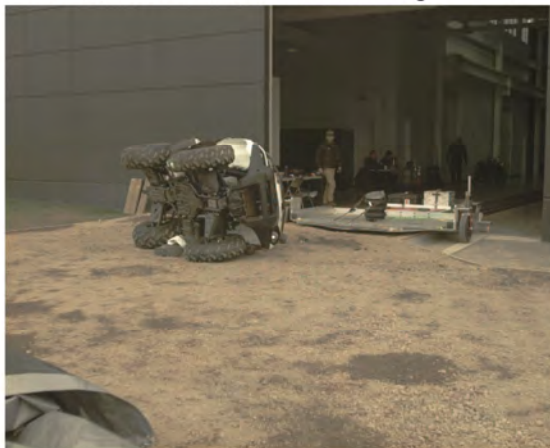
AOS Camera 2 - End of Run - Roll Angle = 277.1°
