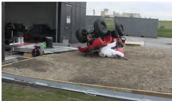
RT Camera 1 - Max Angle = 157.9° - Time = 1.7 sec
