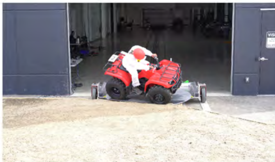
Drone Camera - Roll Angle = 45° - Time = 0.82 sec
