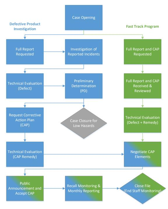
Note: This chart reflects a typical process flow in defective product investigations handled by Compliance Enforcement and Litigation, and Fast Track Program recalls. These processes may be adapted to the circumstances of a case, as necessary, to respond to specific product safety issues.
