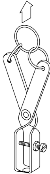
Figure 3 to paragraph (b)(3) — Tension Test Adapter Clamp
