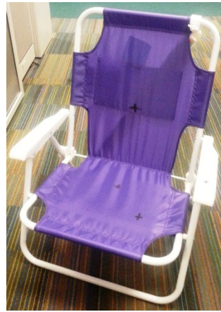
Figure 4. Examples of Children’s Folding Chairs that Failed Sideways Stability
