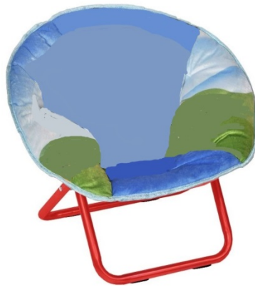
Figure 4. Examples of Children’s Folding Chairs that Failed Sideways Stability
