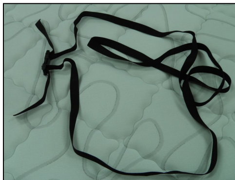
Figure 2: Example of a retention system that was not permanently attached to the product.
