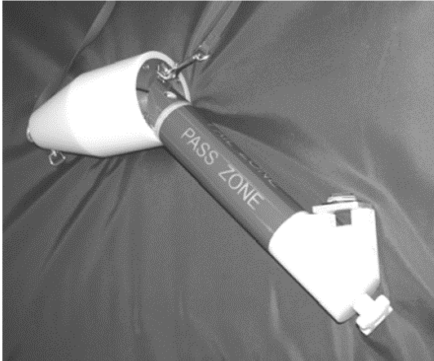
Figure 1: Entrapment Test Probe. From FDA (2006).
