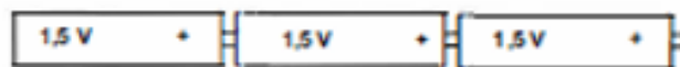
Figure 2A. Example of battery compartment (partial image from IEC 62115 Figure 1 section 7 Marking and instructions. )
