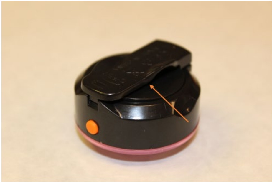
Figure 16. Single diagonal force to open battery compartment cover
