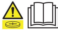
Figure 3A. Internationally recognized symbols "Warning: Contains coin battery," and "Read operator's manual," respectively.
