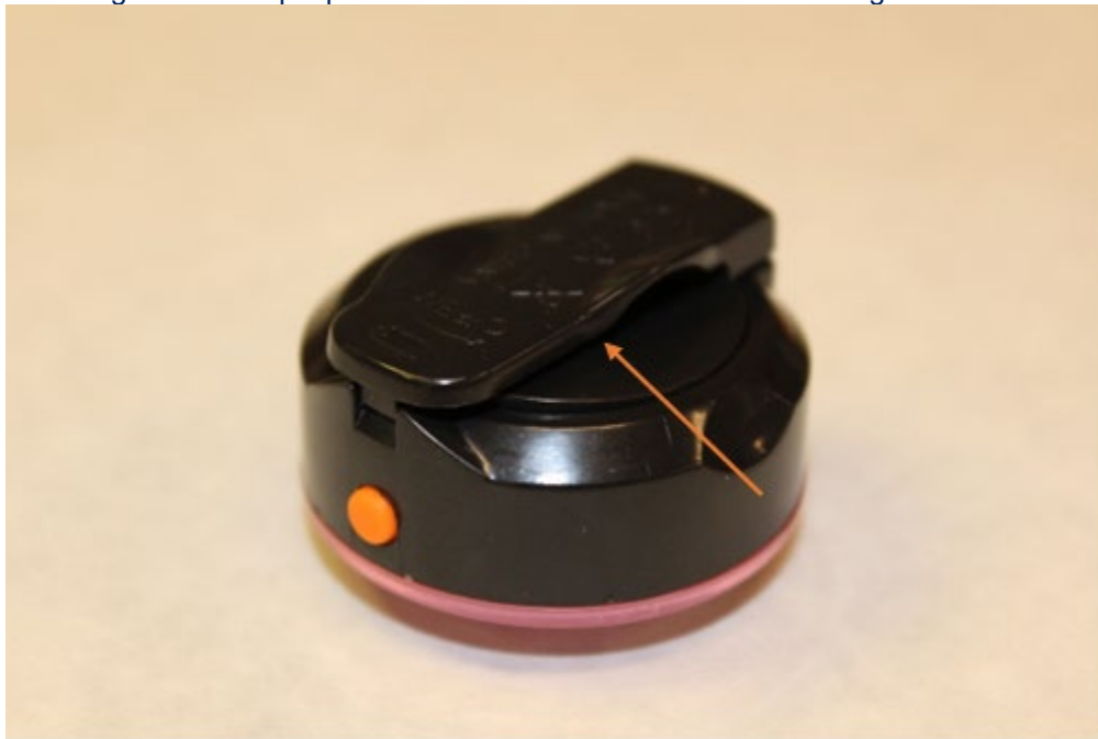
Figure 10. Single diagonal force to open battery compartment cover
