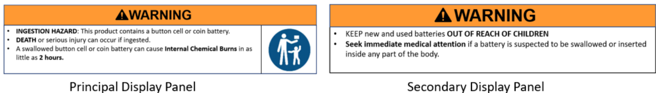
Figure 23. Example abbreviated warning, if the consumer product packaging does not have space for the full warning on the front. The icon must be at least 8 mm in diameter.
