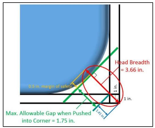
Figure 2, Detail View of Maximum Corner Gap Location and Measurement.
