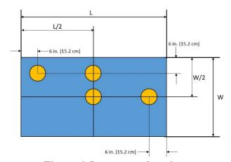
Figure 6. Impact test locations
