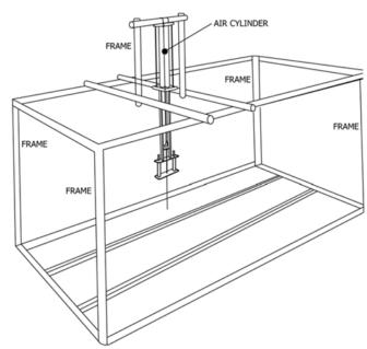
Figure 3. Typical free fall impacting system<sup>72</sup>
