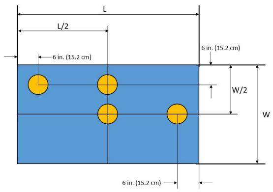
Figure 1. Impact test locations.
