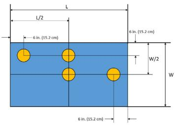
Figure 6. Impact test locations
