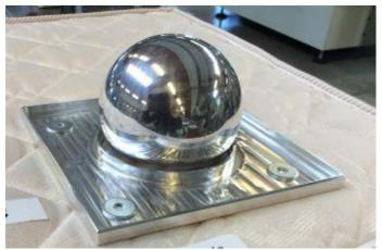
Photo 2. EN 16890 firmness test fixture.<sup>34</sup>
