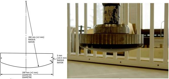
Figure 4. Profile of Impact mass<sup>51</sup>
