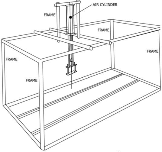
Figure 3. Typical free fall impacting system<sup>51</sup>
