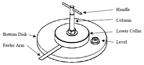
Figure 2. Firmness Test Fixture Adapted from Australian/New Zealand Standard 8811.1:2013 test apparatus
