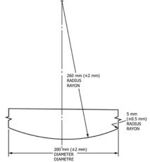
Figure 4. Profile of Impact mass<sup>72</sup>
