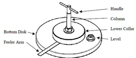
**Figure 2. Mattress Firmness Test Fixture**
