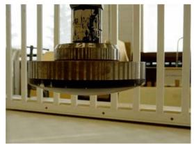
Figure 5. Photo of typical impact mass<sup>72</sup>
