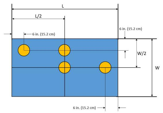
Figure 4. Impact test locations.
