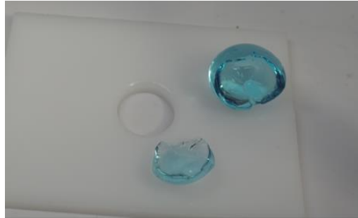
Figure 8: Expanded Water Bead After Being Fragmented by 10.0 mm Diameter Rod End.
