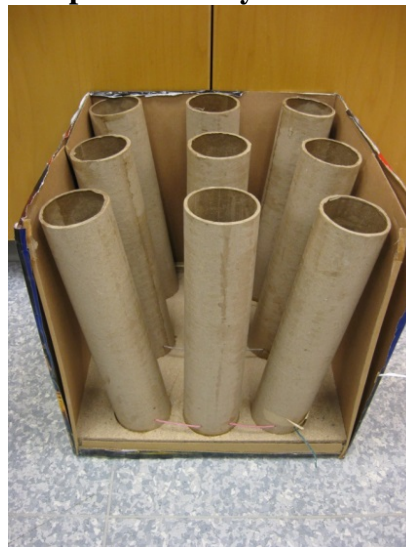
Figure 2: Example Cut Away of a Mine Shell Device
