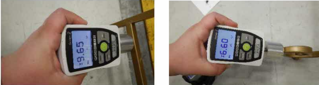
Figure 15. Testing of the sample in the direction of folding with the force gauge and 1.5-inch disk parallel to the surface.
