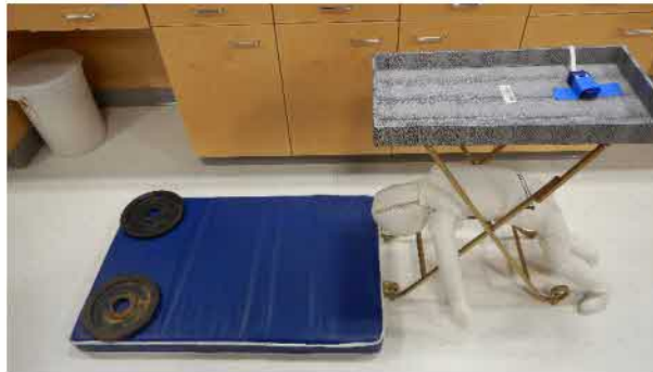
Figure 18. Test set up for measuring the forces exerted upon an entrapped child
