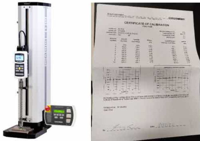
Figure 34. Calibrated MARK-10 Motorized Tension / Compression Test Stand and Certificate of Calibration
