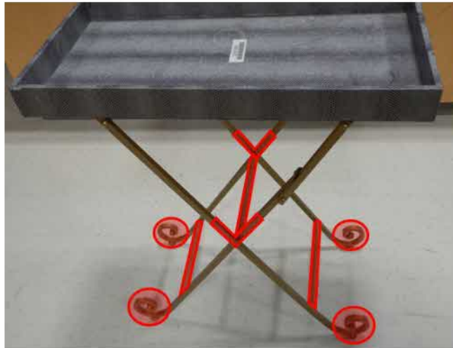
Figure 27. Footholds identified on the sample
