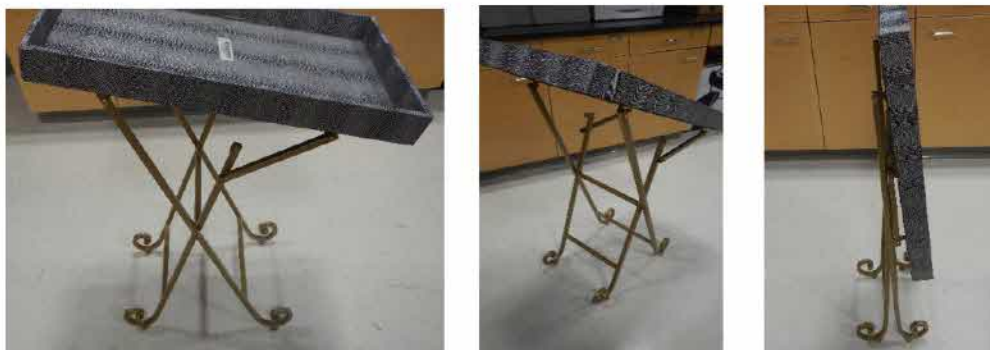
Figure 6. Various stable configurations where product is partially collapsed but still standing from LSM PSA (Figure 29)
