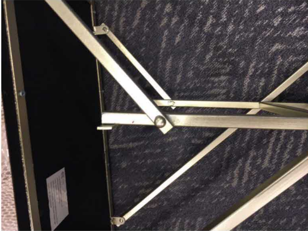
Photograph 2-11: Close up of the folding mechanism
