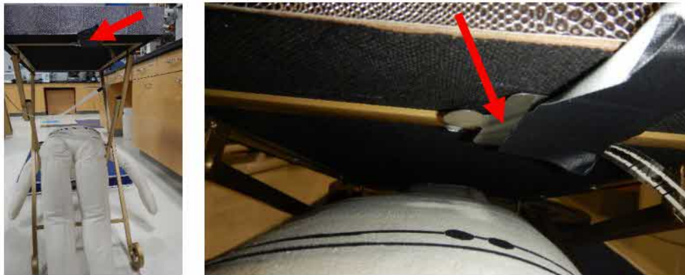
Figure 26. Compression force sensor on the bottom of the tray when the frame was fully engaged (left) and in contact with the CAMI dummy when the frame was collapsed (right)
