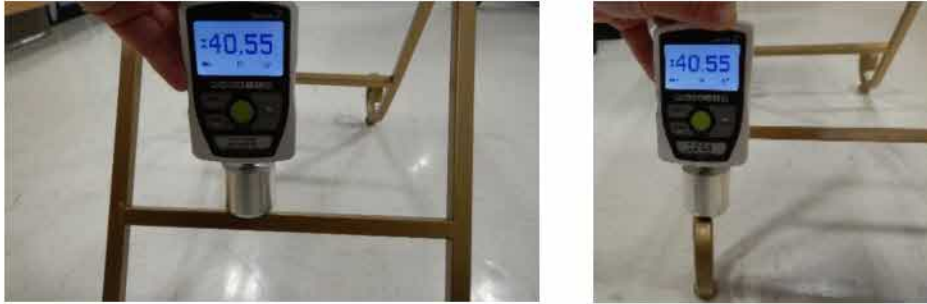
Figure 28. Force being applied vertically to the footholds
