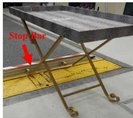
Figure 14. Test set up for measuring the forces that contribute to the sample folding.
