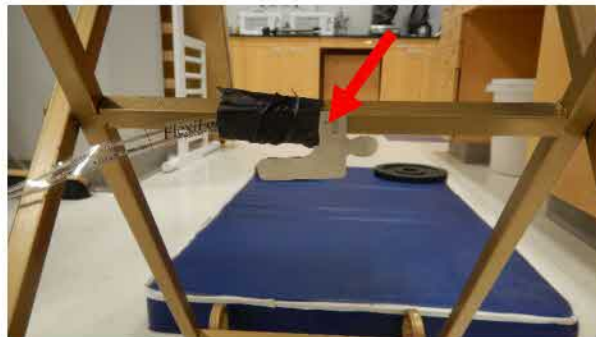
Figure 23. Placement of compression force sensor on the side of the middle horizontal bar
