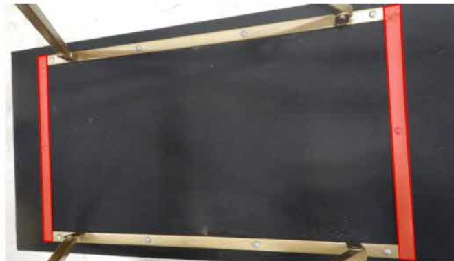
Figure 11. The sections highlighted in red corresponds with the location and size of the indentations found on the victim's back.
