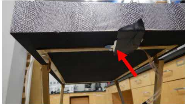
Figure 25. Placement of compression force sensor on the top of the frame connected to the bottom of the tray
