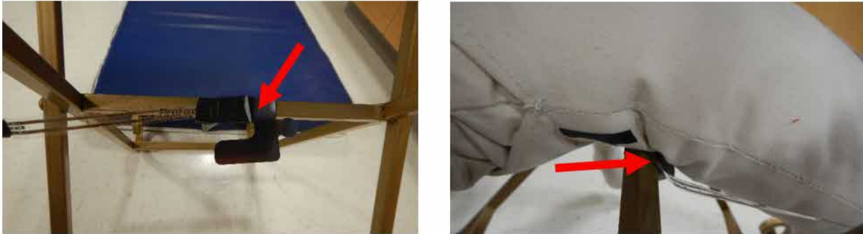
Figure 22. Placement of compression force sensor on the top of the middle horizontal bar and in contact with the CAMI dummy
