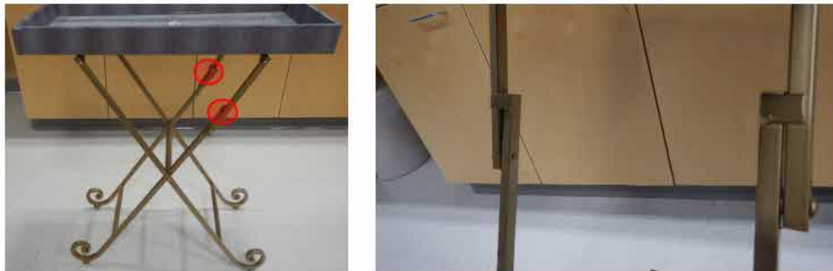
Figure 30. Tab stops on the exemplar samples.
