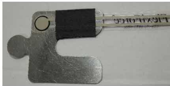
Figure 21. Compression force sensor taped to 0.20 in. shim
