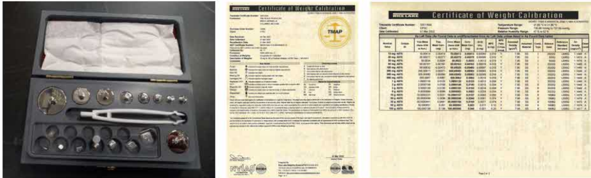
Figure 33. Calibrated Rice Lake Weighing Systems Calibration Weights and Certificate of Weight Calibration
