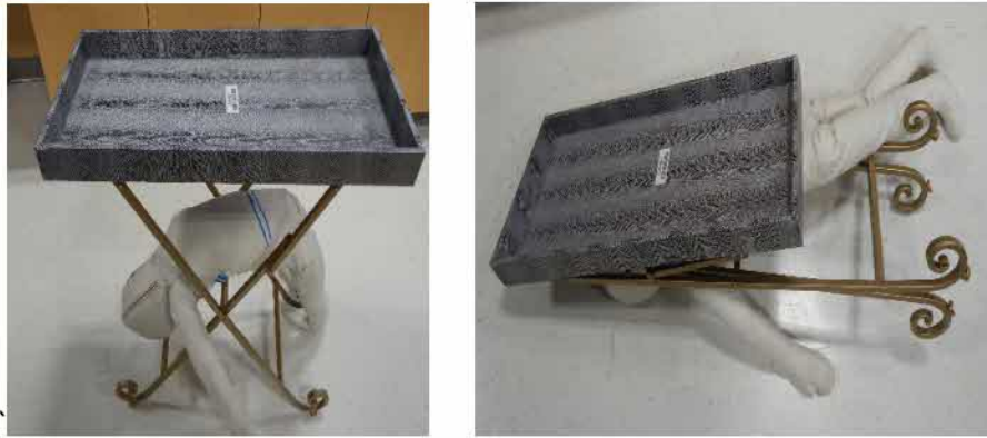
Figure 7. CAMI entered from the upper right side and the table fell to the left.
