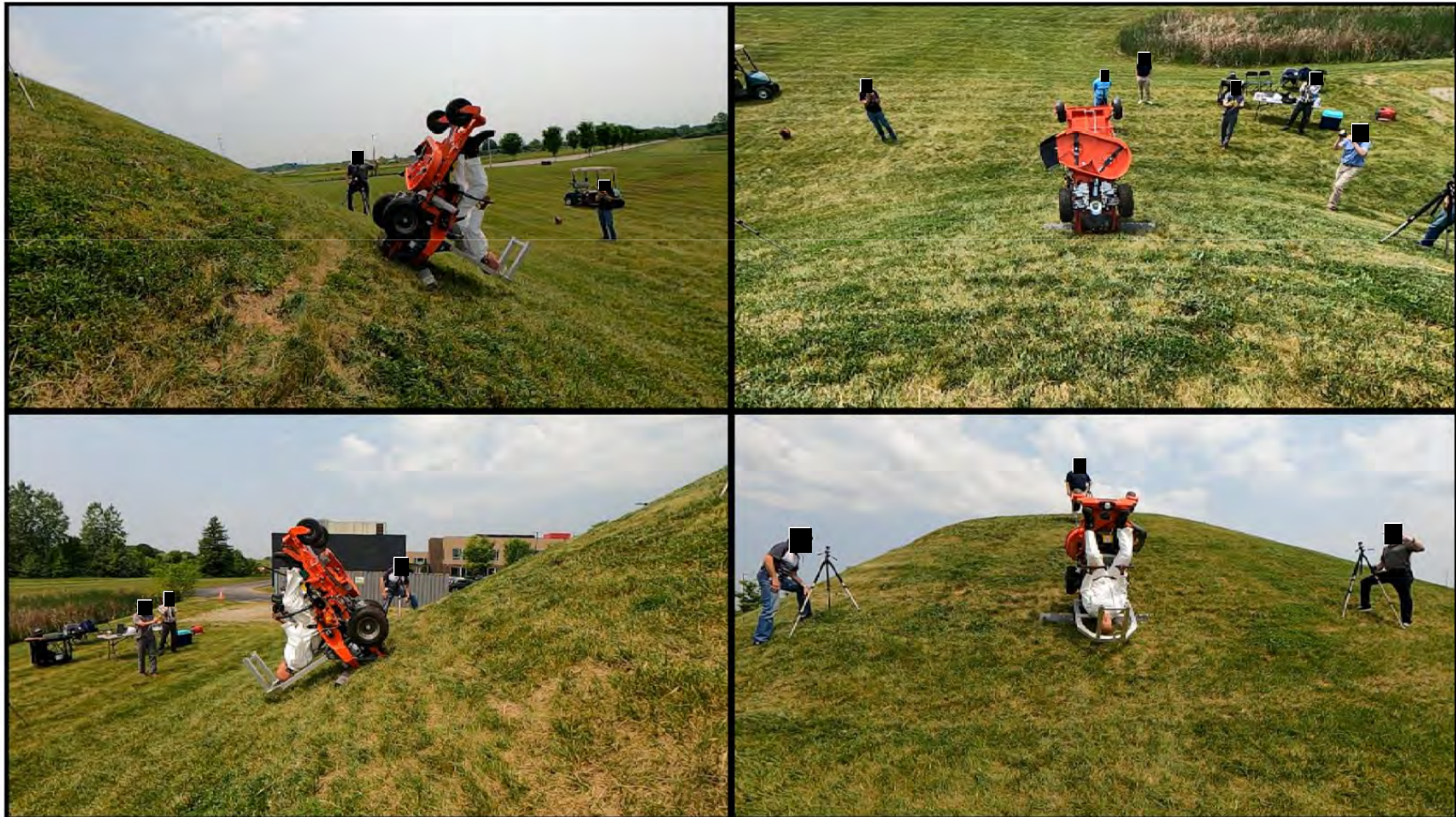
Zero-Turn Mower – Rearward Pitchover with ROPS
