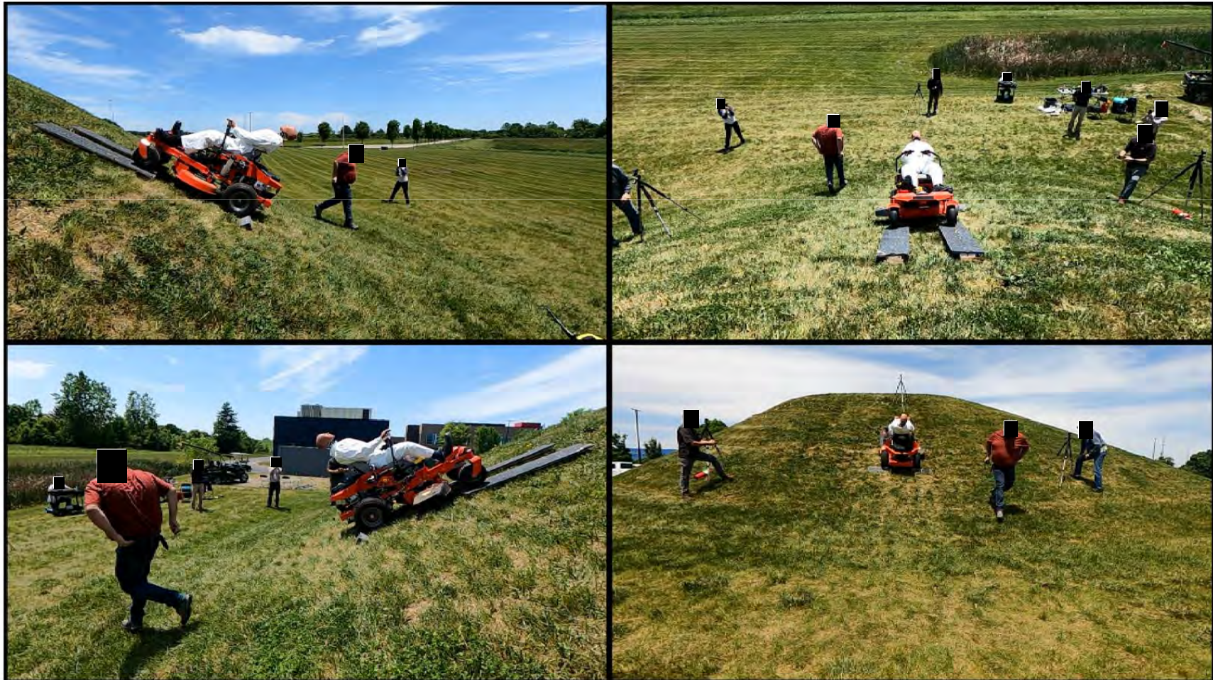
Zero-Turn Mower – Rearward Pitchover without ROPS
