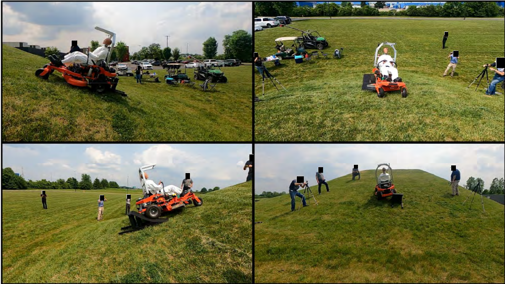
Zero-Turn Mower – Quasi-Lateral Rollover with ROPS
