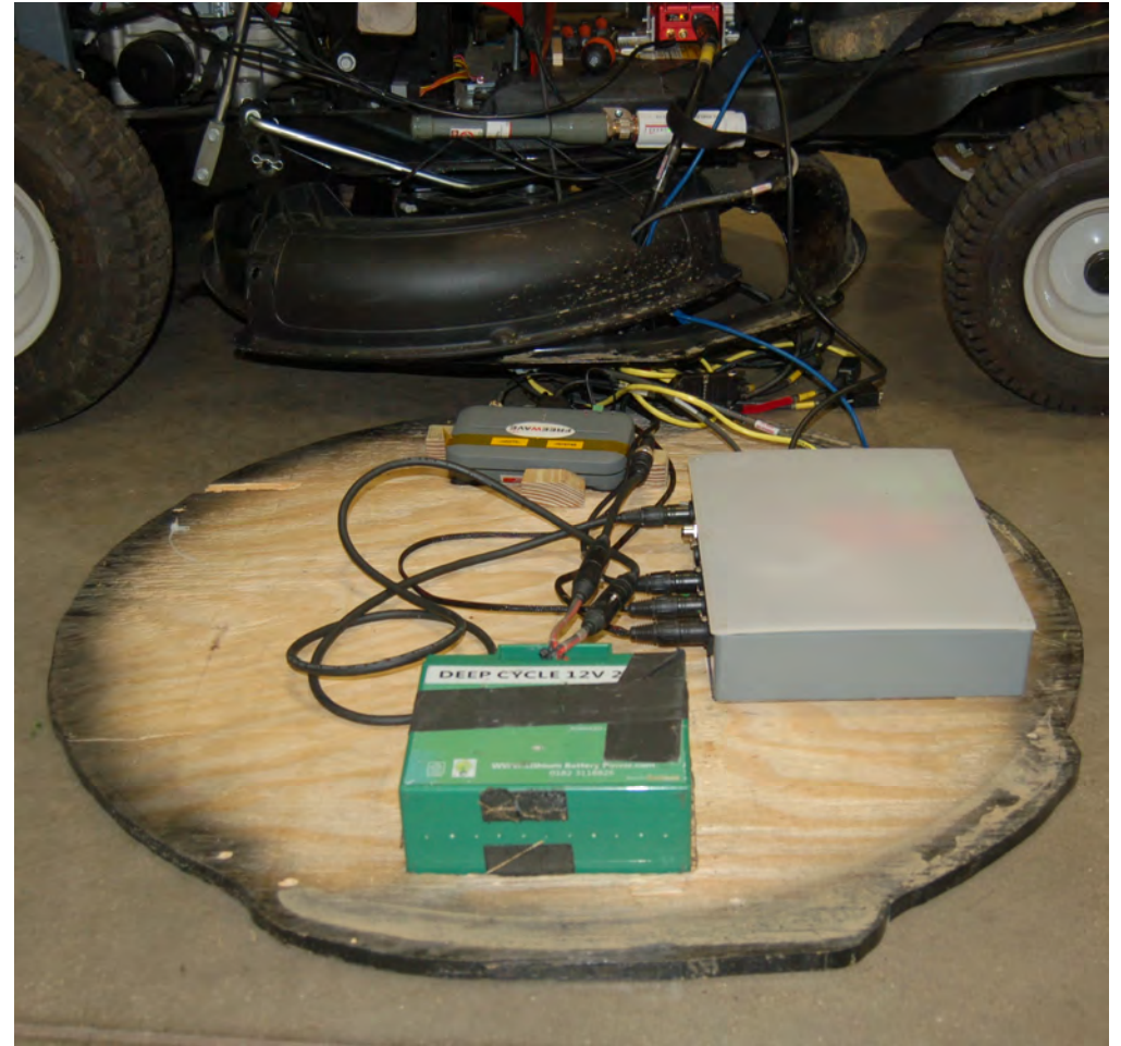
On-Vehicle Computer Box, 12V Battery, and Freewave Radio Mounted on Board Fixed Beneath Mower Deck
