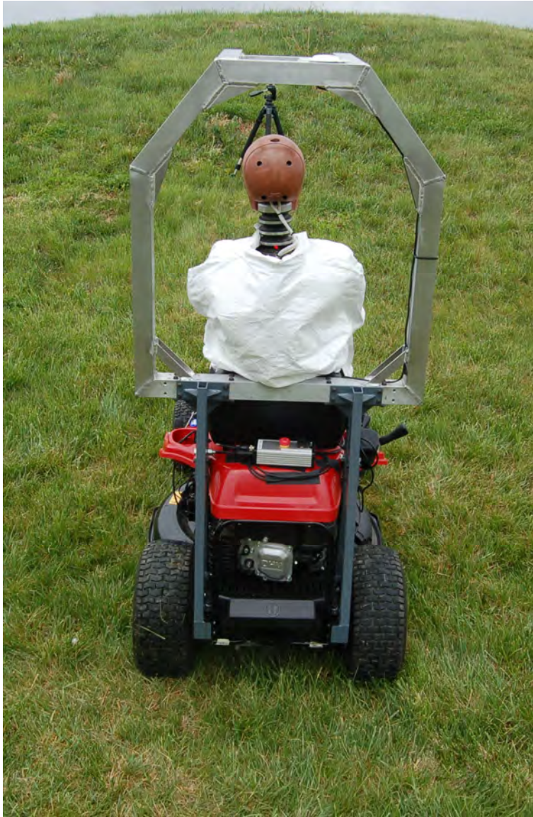
Rear View for Rearward Pitchover Test
