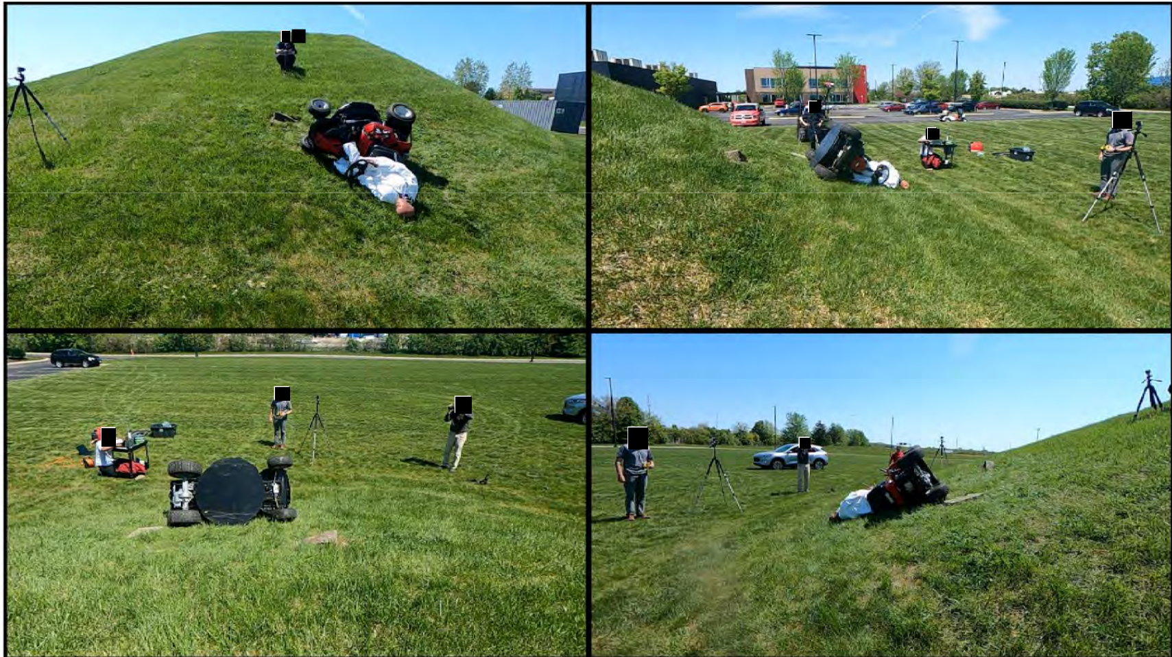
Tractor Style Mower – Lateral Rollover without ROPS
