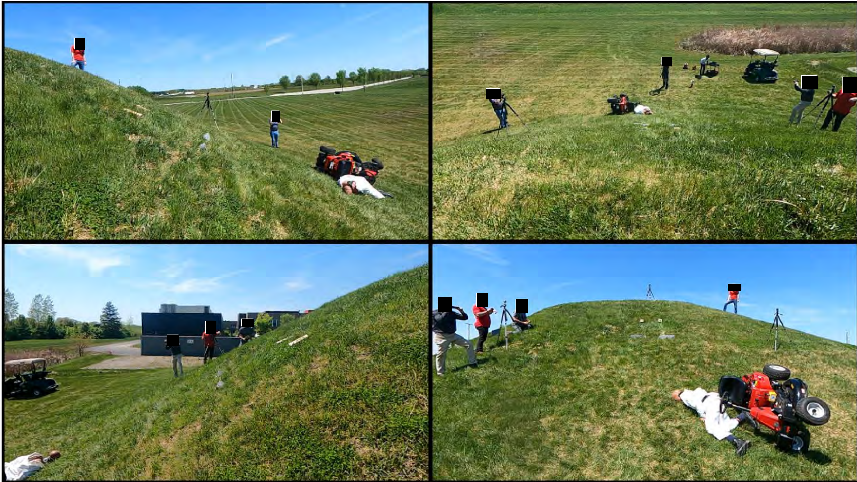
Tractor Style Mower – Rearward Pitchover without ROPS
