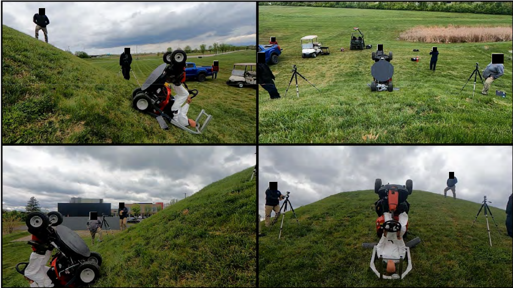
Tractor Style Mower – Rearward Pitchover with ROPS
