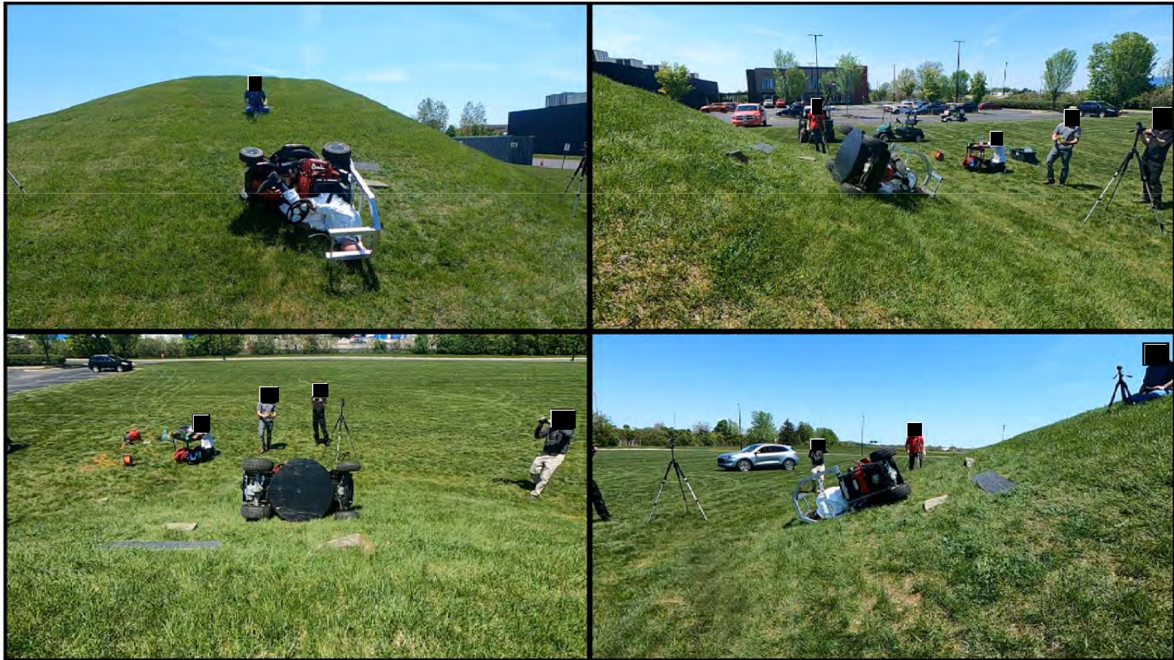
Tractor Style Mower – Lateral Rollover with ROPS
