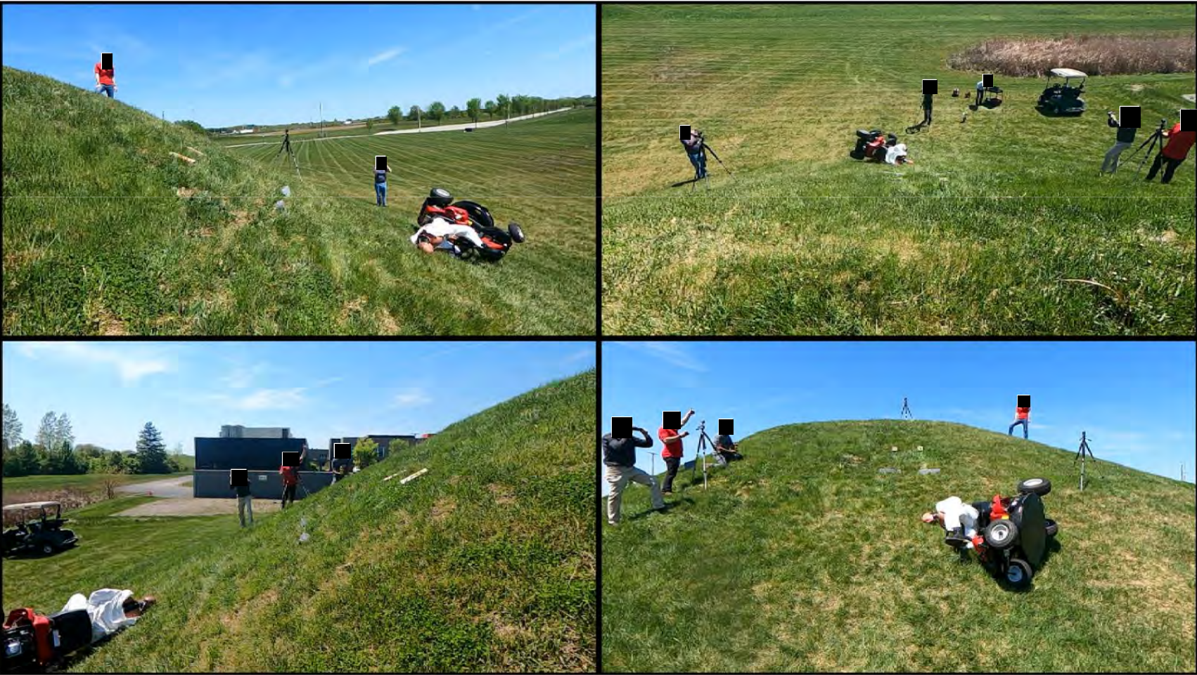
Tractor Style Mower – Rearward Pitchover without ROPS
