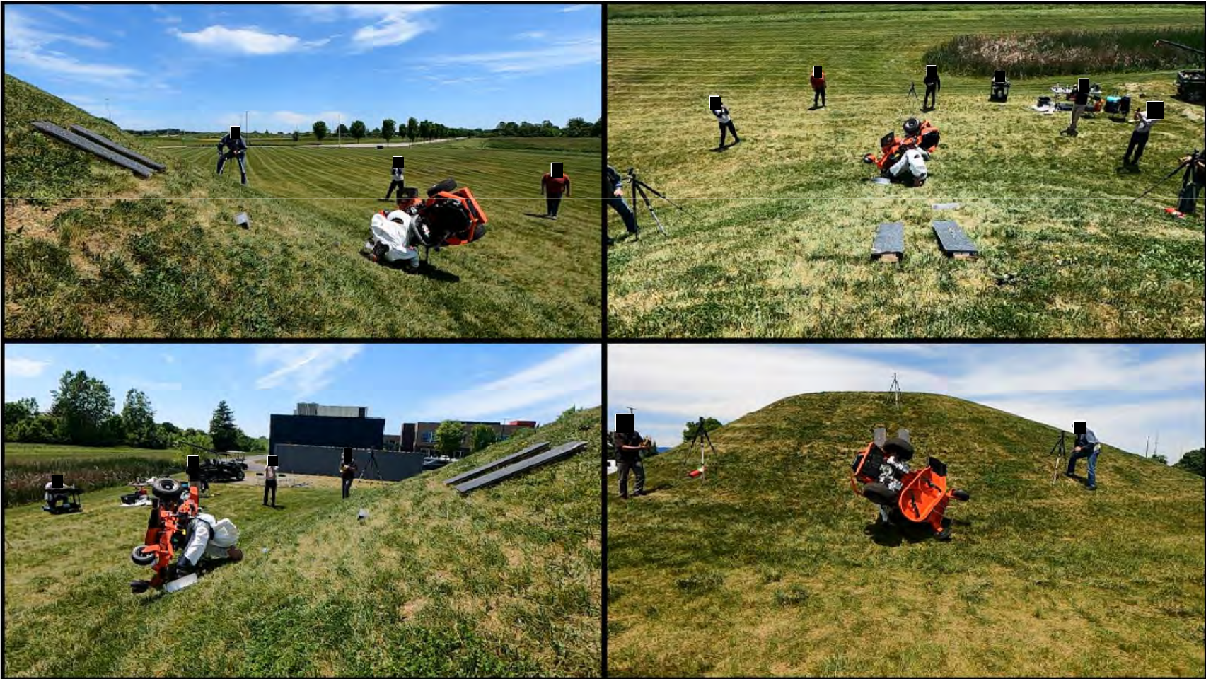
Zero-Turn Mower – Rearward Pitchover without ROPS
