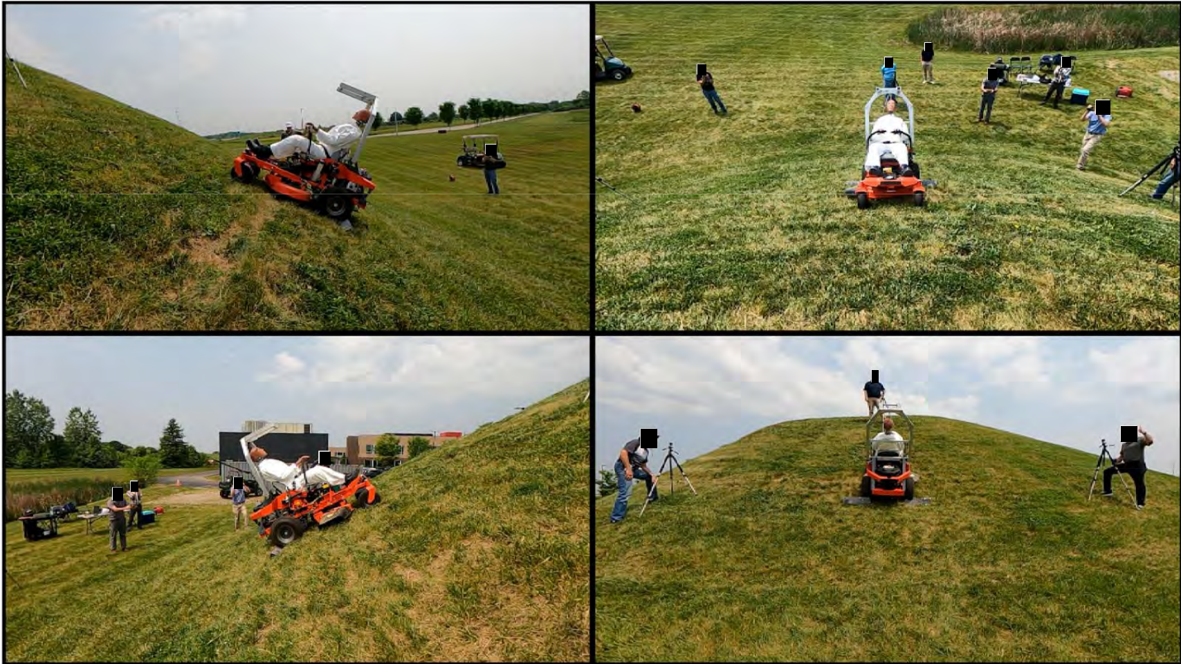
Zero-Turn Mower – Rearward Pitchover with ROPS
