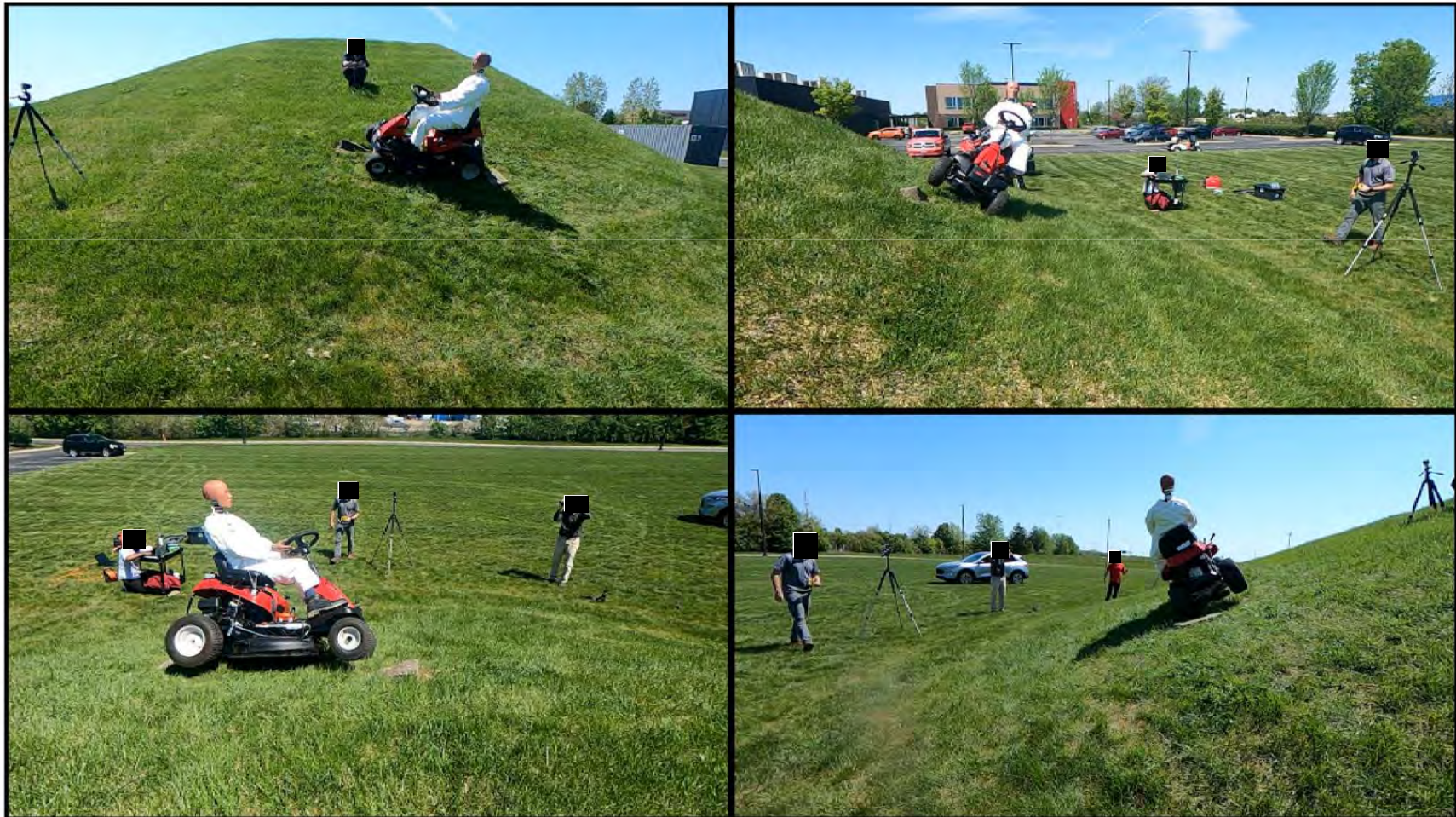
Tractor Style Mower – Lateral Rollover without ROPS
