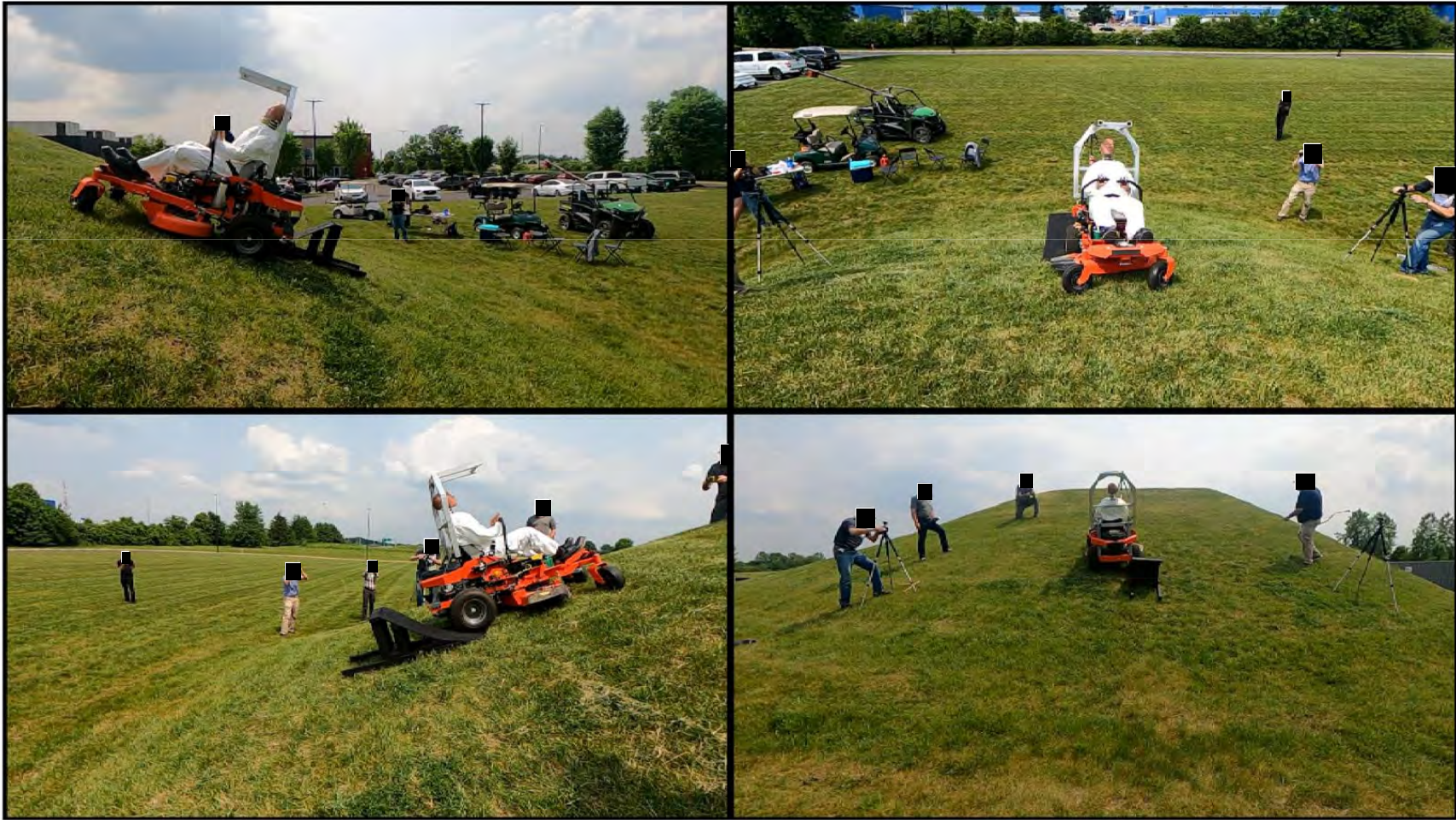
Zero-Turn Mower – Quasi-Lateral Rollover with ROPS
