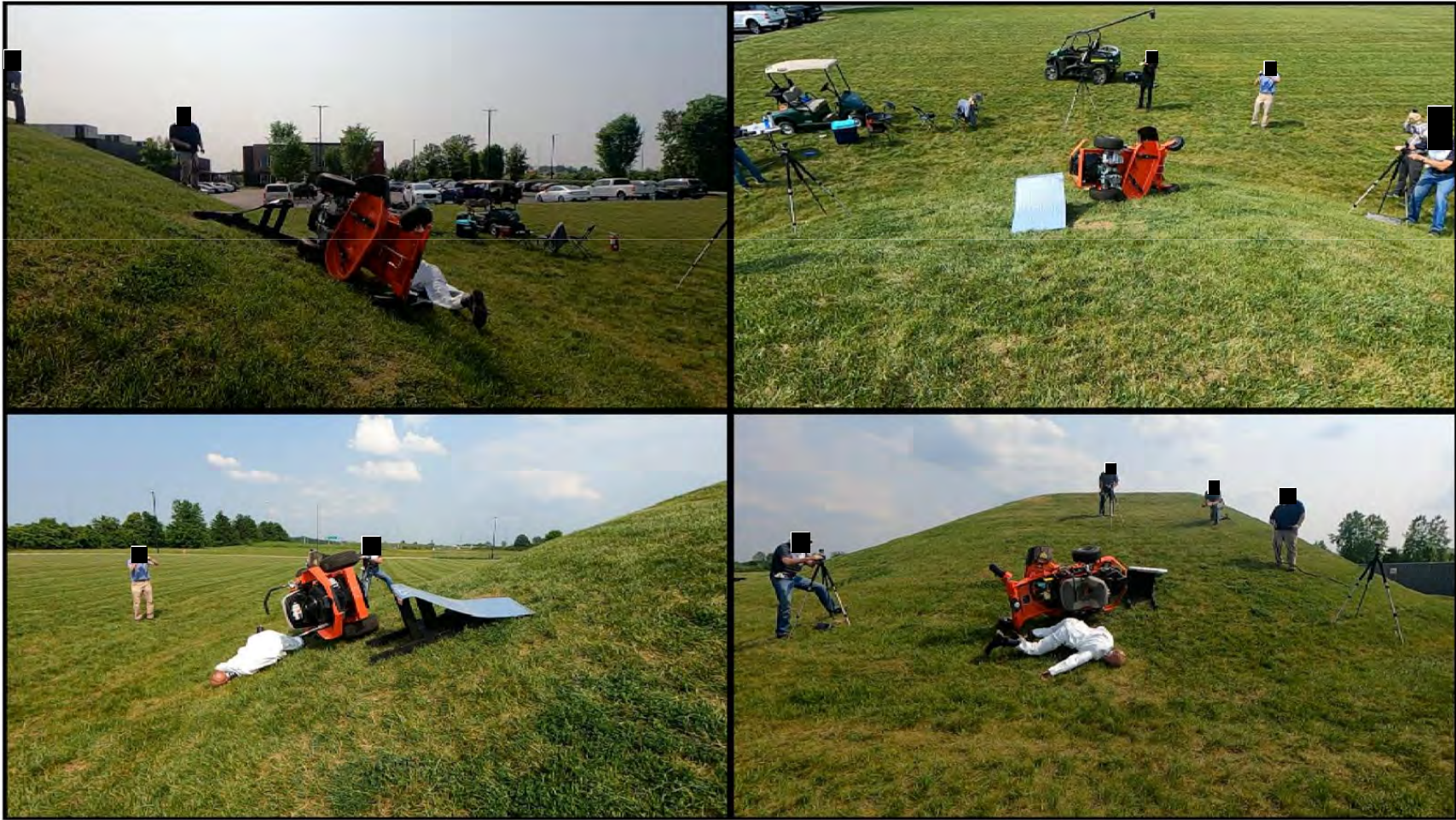
Zero-Turn Mower – Quasi-Lateral Rollover without ROPS
