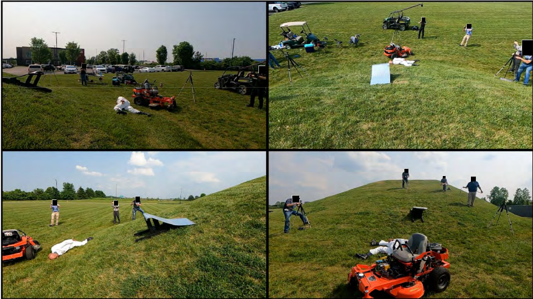
Zero-Turn Mower – Quasi-Lateral Rollover without ROPS
