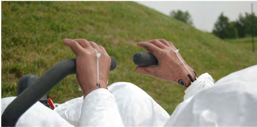
Cable Ties for Handhold to Control Levers
