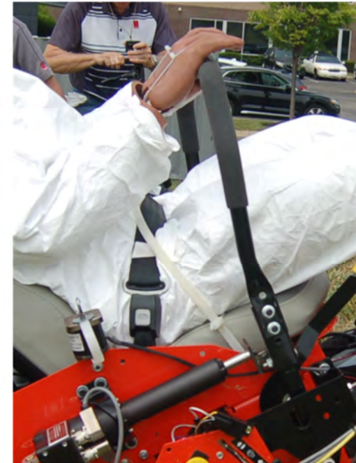
Cable Tie Loosely Connecting ATD Thigh to Seat Belt to Prevent Seat Belt from Sliding into Cavity Between ATD Pelvis and Chest
