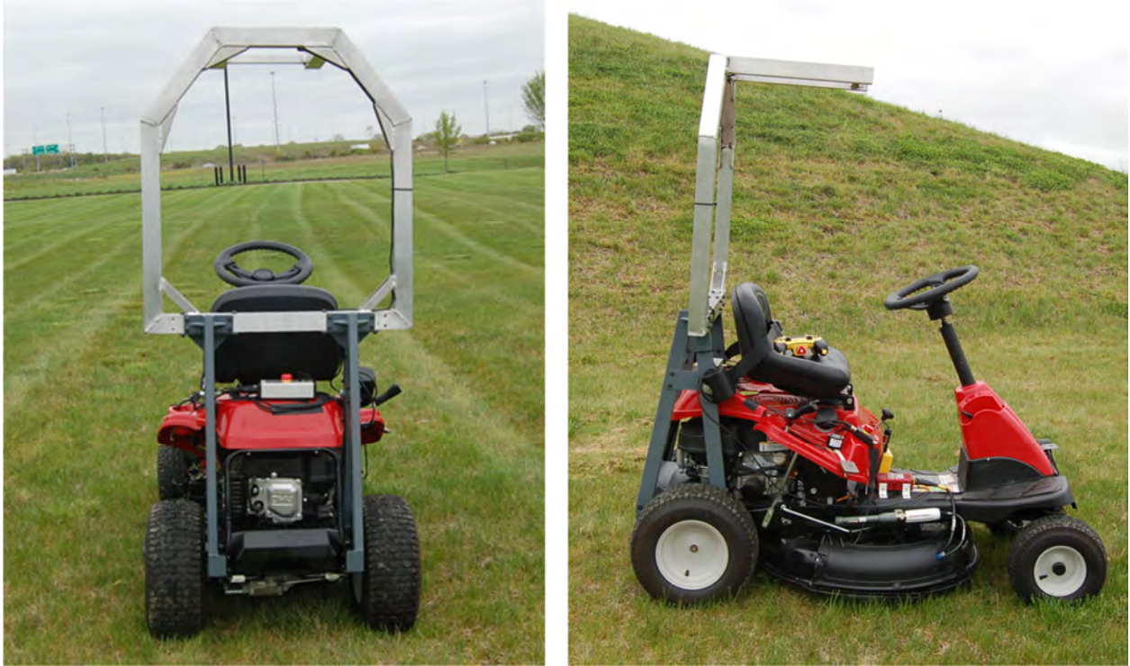
Figure 9: Rear and Side Views of Tractor Mower with ROPS
