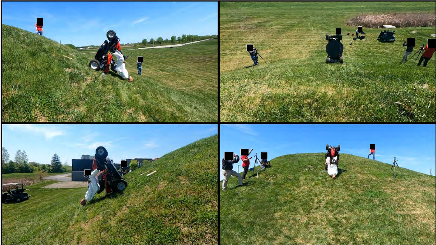
Tractor Style Mower – Rearward Pitchover without ROPS
