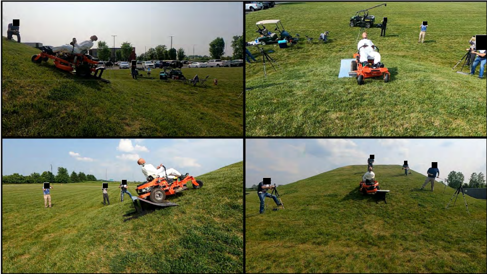
Zero-Turn Mower – Quasi-Lateral Rollover without ROPS
