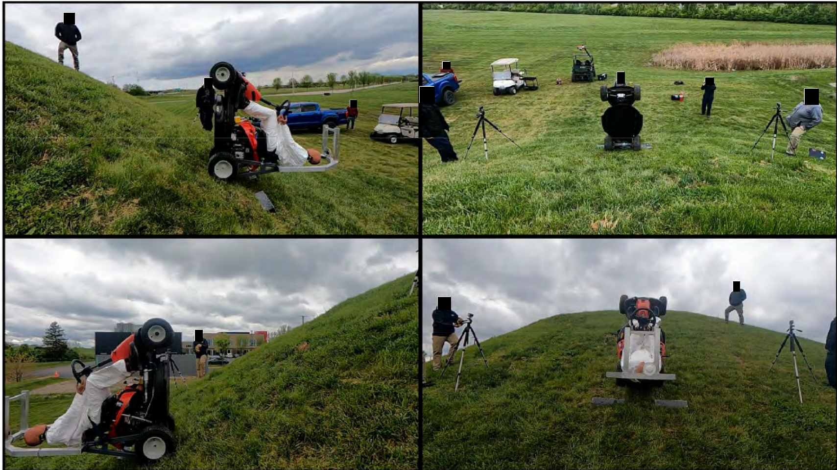
Tractor Style Mower – Rearward Pitchover with ROPS
