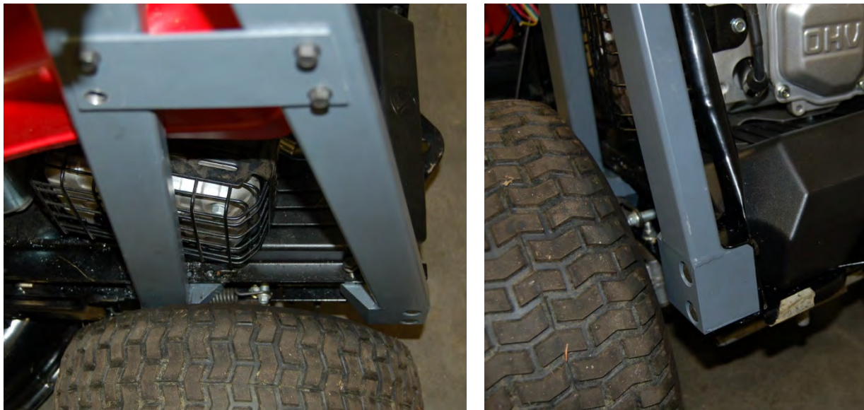
Figure 8: Left Photo: Side View of the Lower Section of ROPS for the Tractor Mower Right Photo: Oblique View of the Lower Section of ROPS for the Tractor Mower (As with the zero-turn mower, the lower ROPS pieces act as reinforcements for the mower frame, which was not designed for use with ROPS.)
