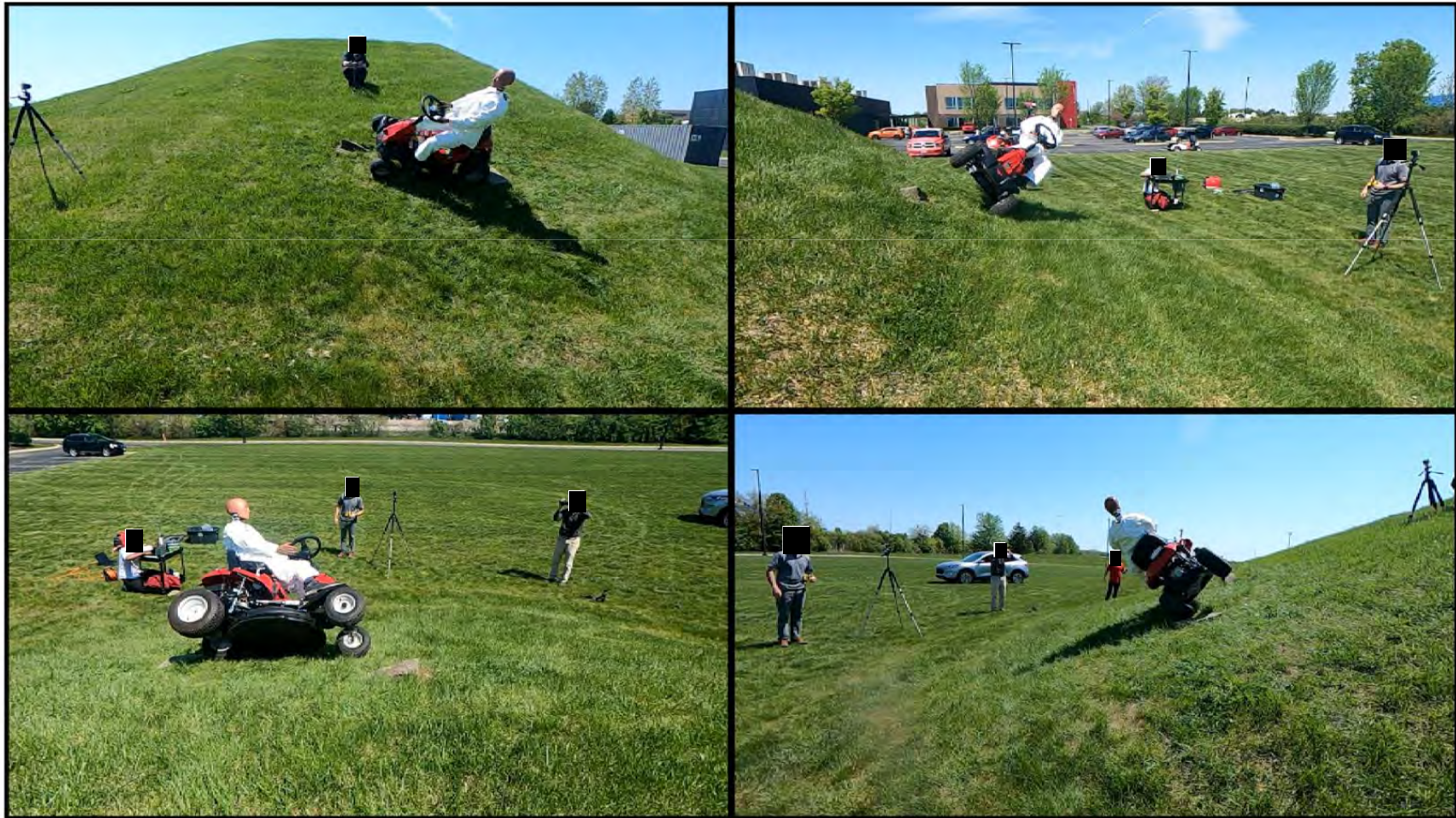
Tractor Style Mower – Lateral Rollover without ROPS
