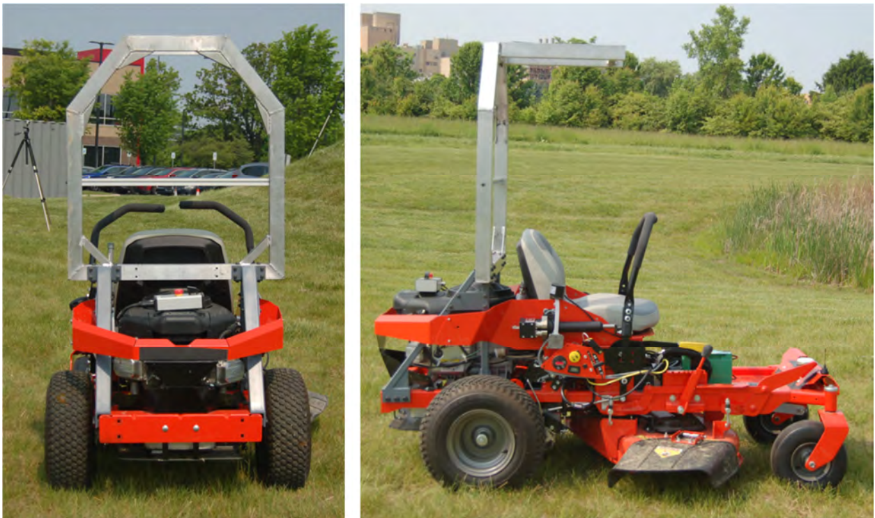
Figure 10: Rear and Side Views of Zero-Turn Mower with ROPS
