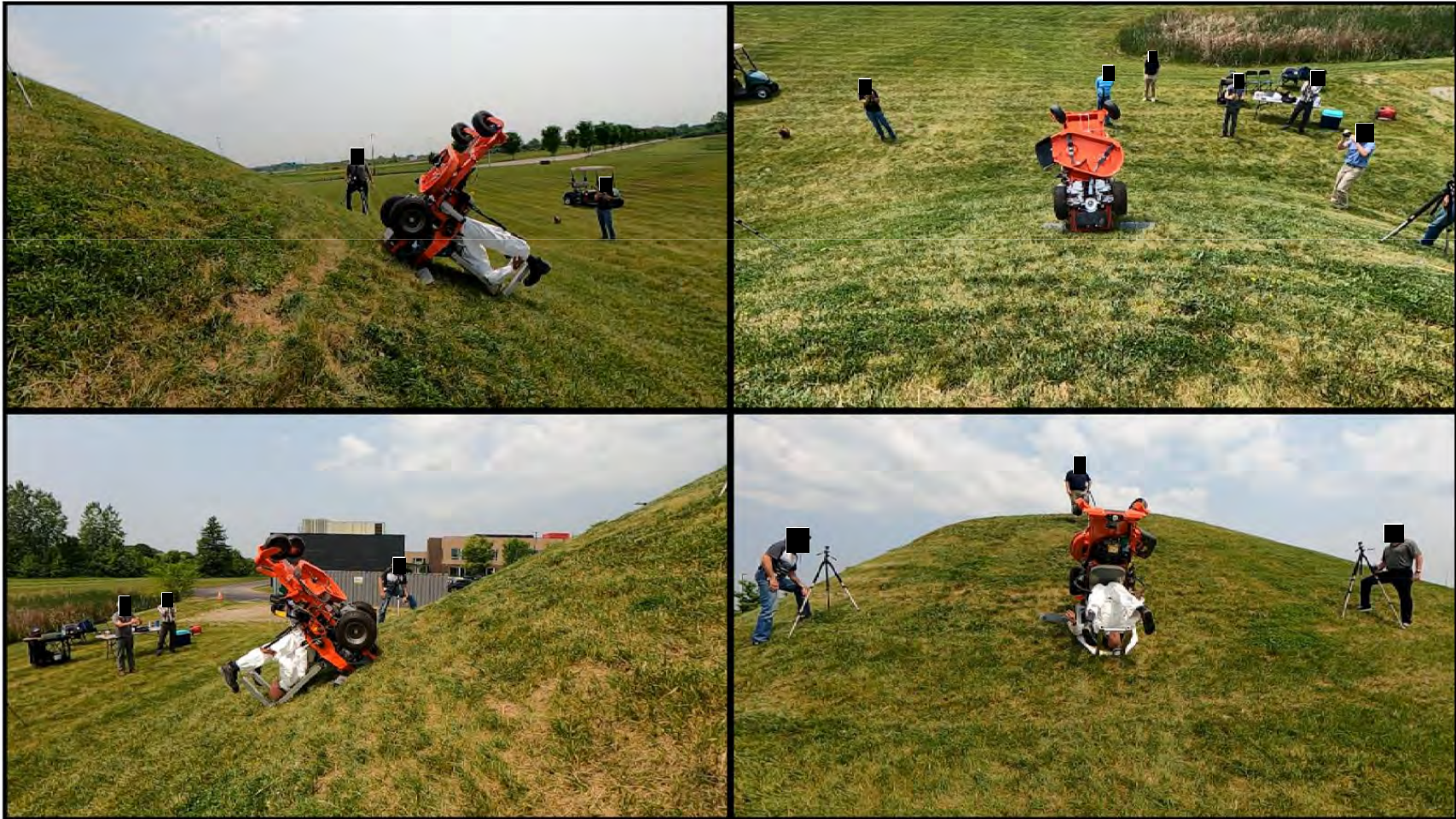
Zero-Turn Mower – Rearward Pitchover with ROPS
