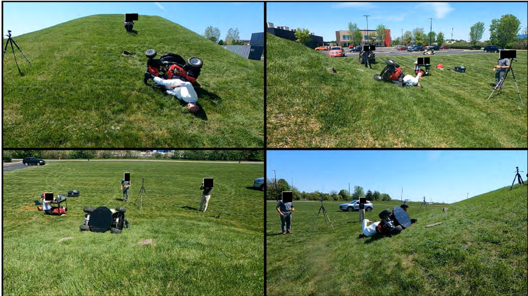
Tractor Style Mower – Lateral Rollover without ROPS
