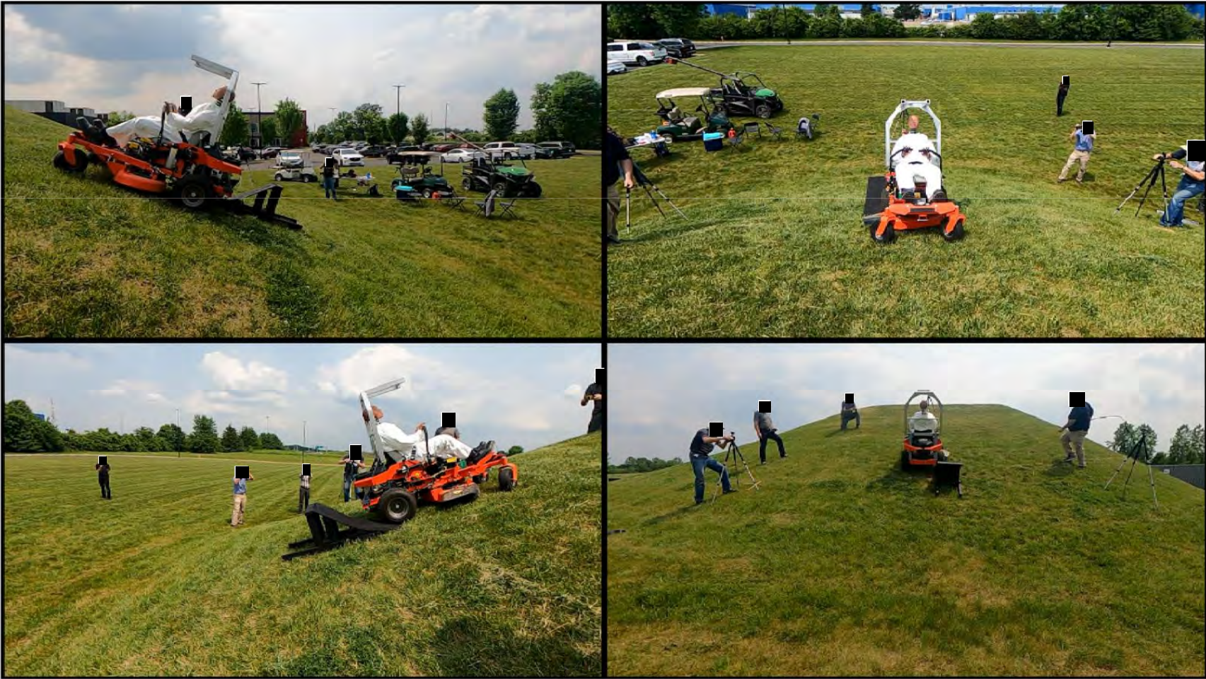
Zero-Turn Mower – Quasi-Lateral Rollover with ROPS
