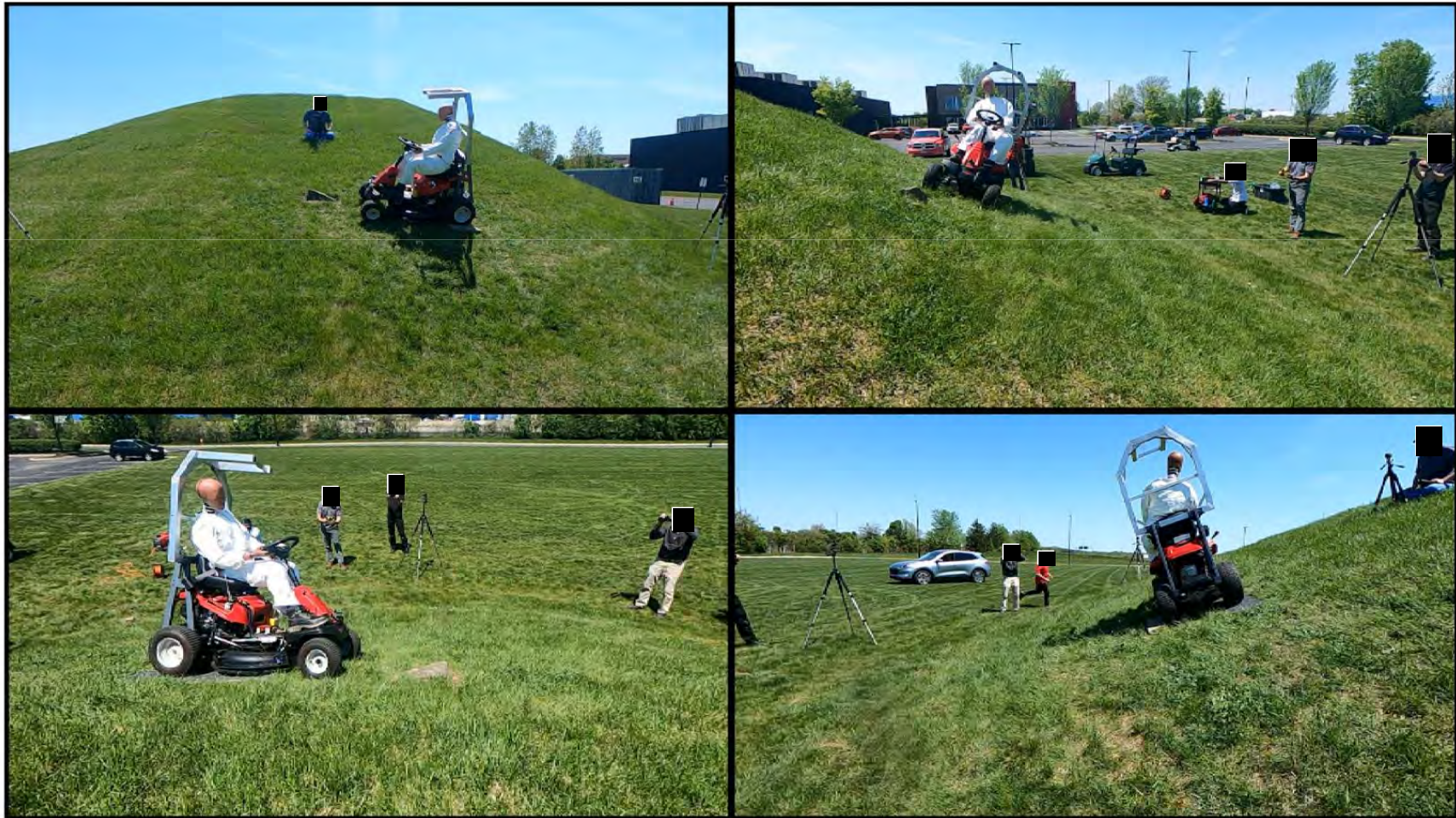
Tractor Style Mower – Lateral Rollover with ROPS
