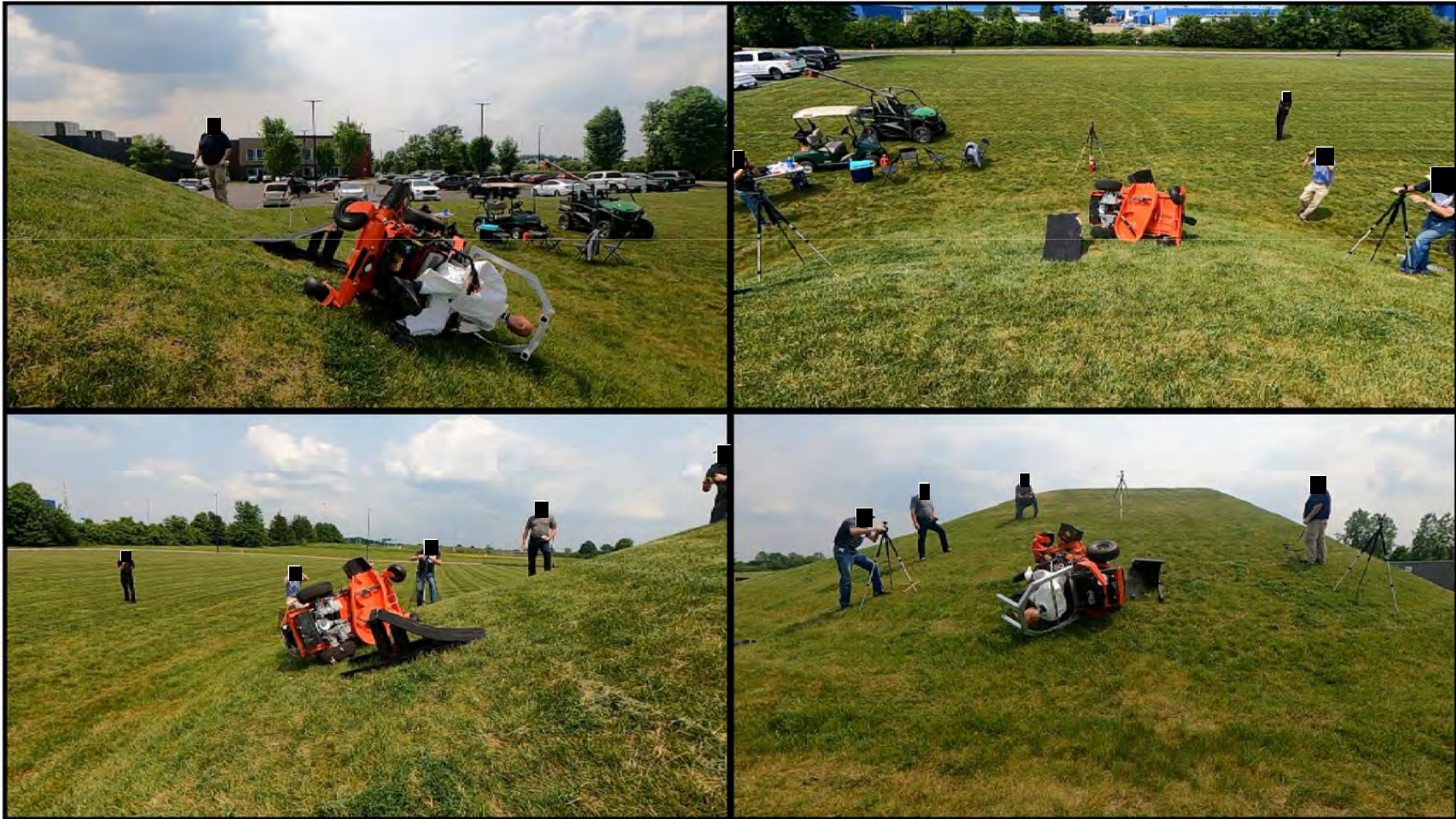
Zero-Turn Mower – Quasi-Lateral Rollover with ROPS
