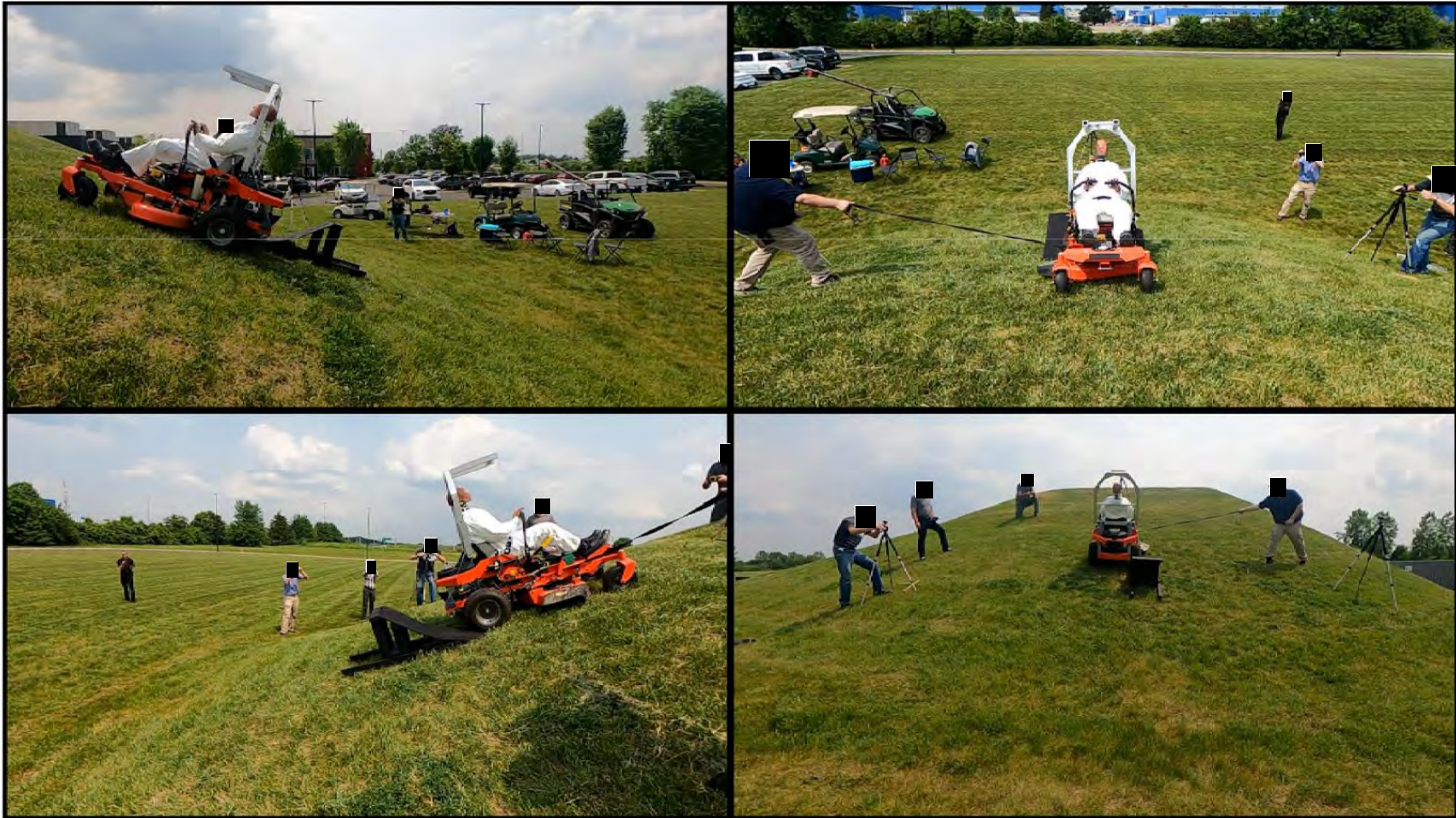
Zero-Turn Mower – Quasi-Lateral Rollover with ROPS
