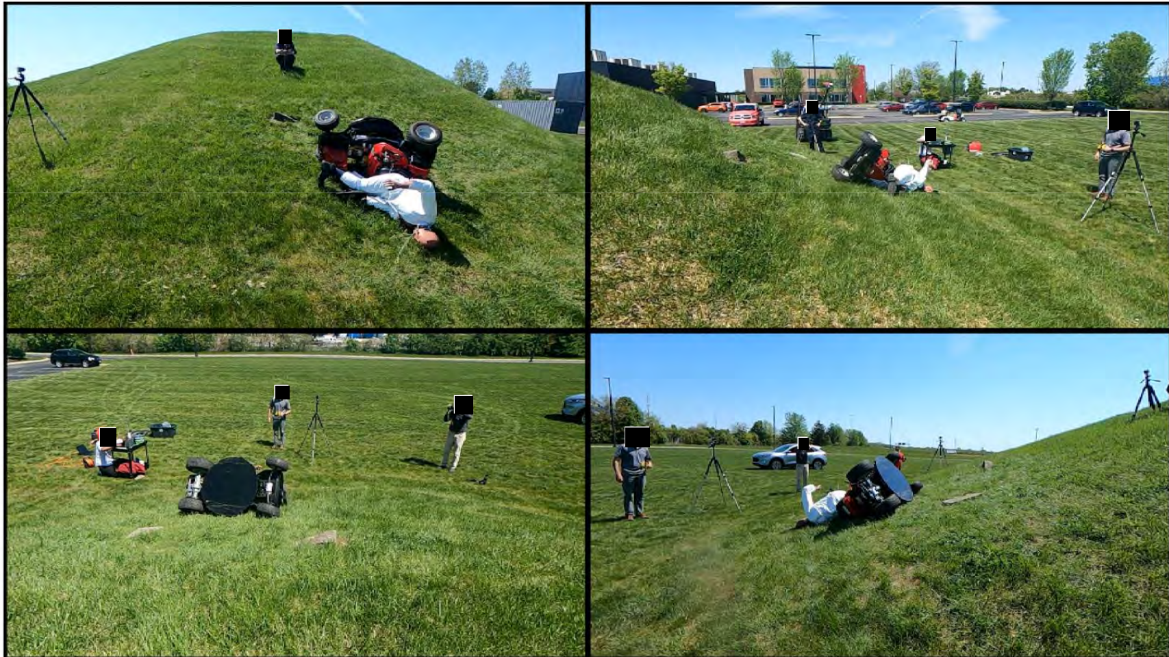
Tractor Style Mower – Lateral Rollover without ROPS
