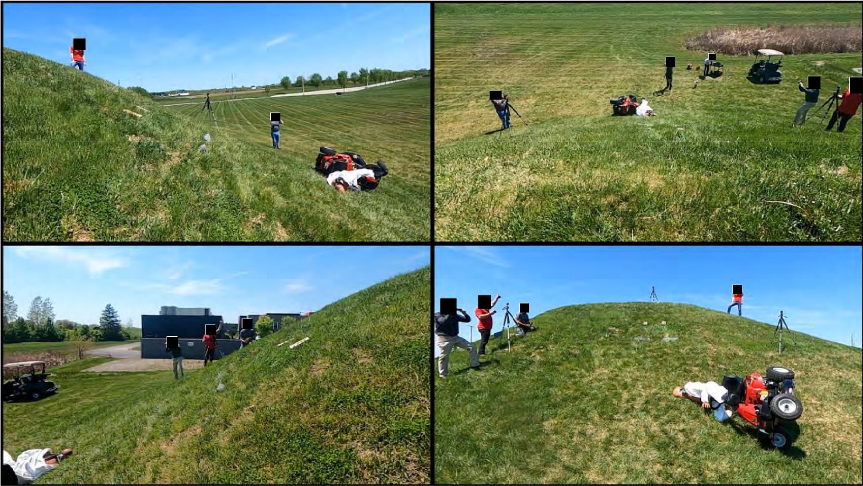
Tractor Style Mower – Rearward Pitchover without ROPS
