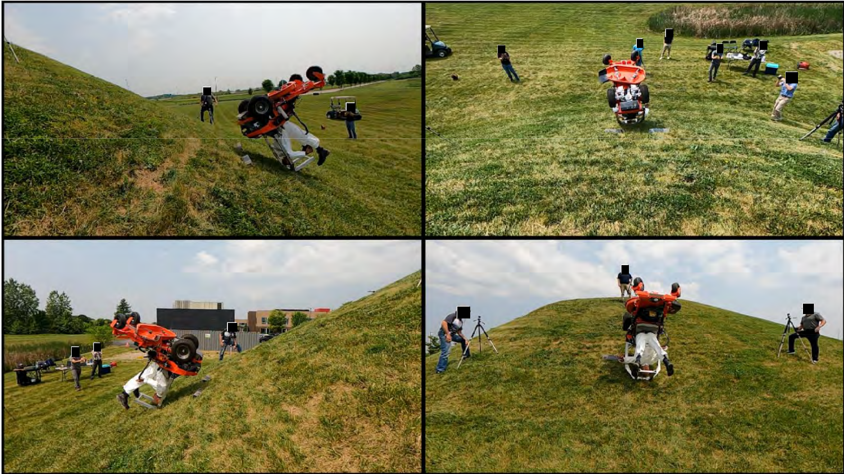
Zero-Turn Mower – Rearward Pitchover with ROPS
