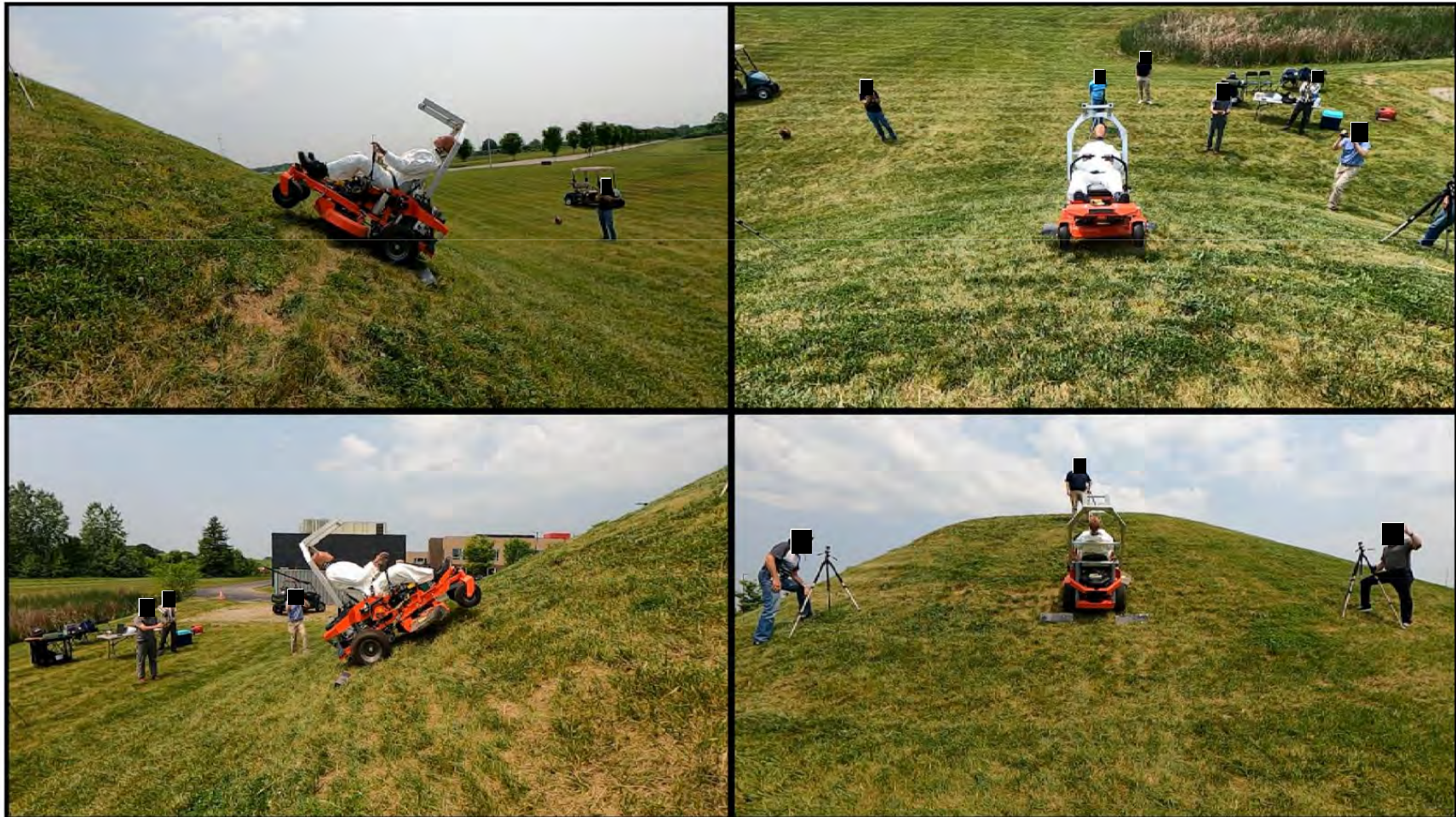
Zero-Turn Mower – Rearward Pitchover with ROPS
