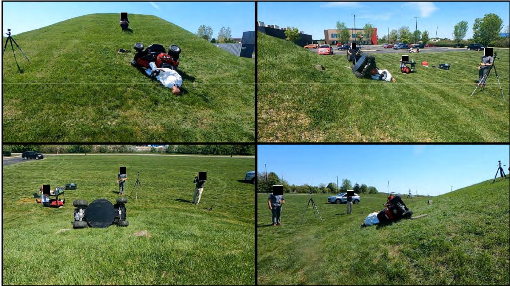
Tractor Style Mower – Lateral Rollover without ROPS
