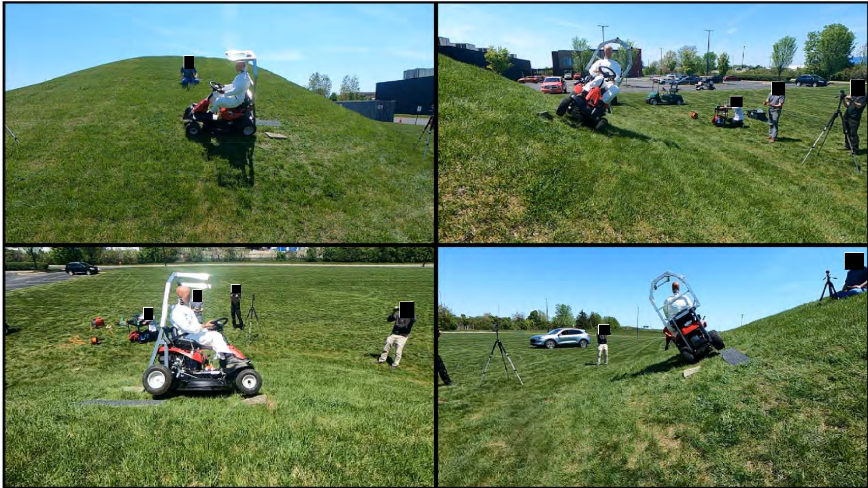
Tractor Style Mower – Lateral Rollover with ROPS
