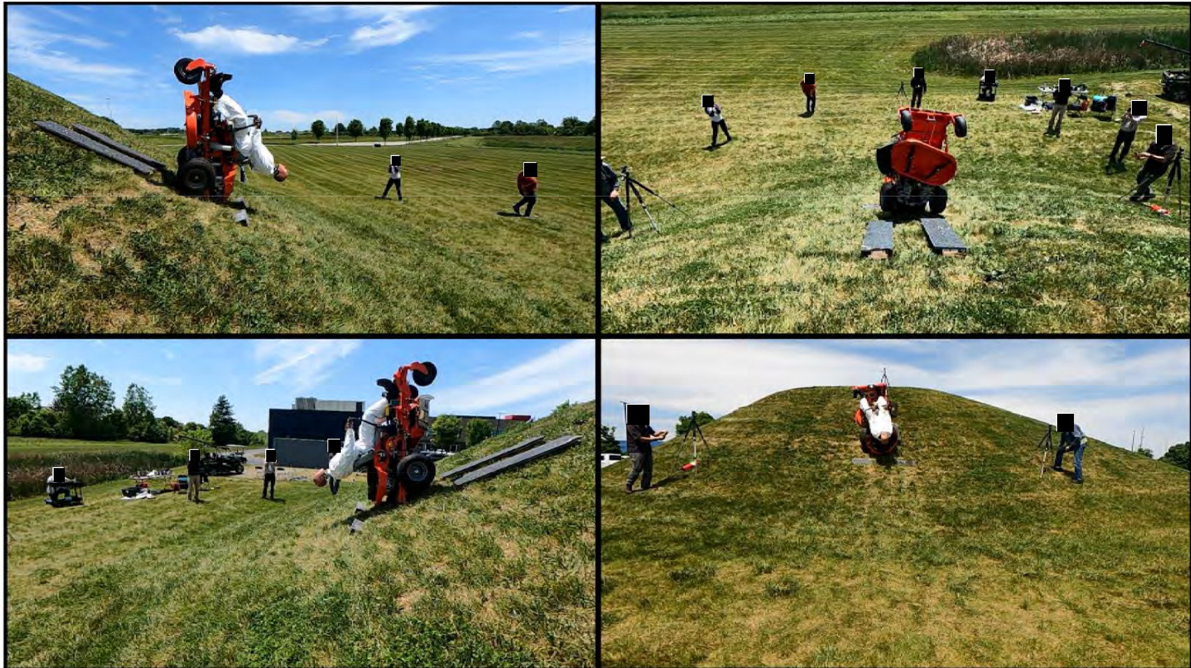
Zero-Turn Mower – Rearward Pitchover without ROPS
