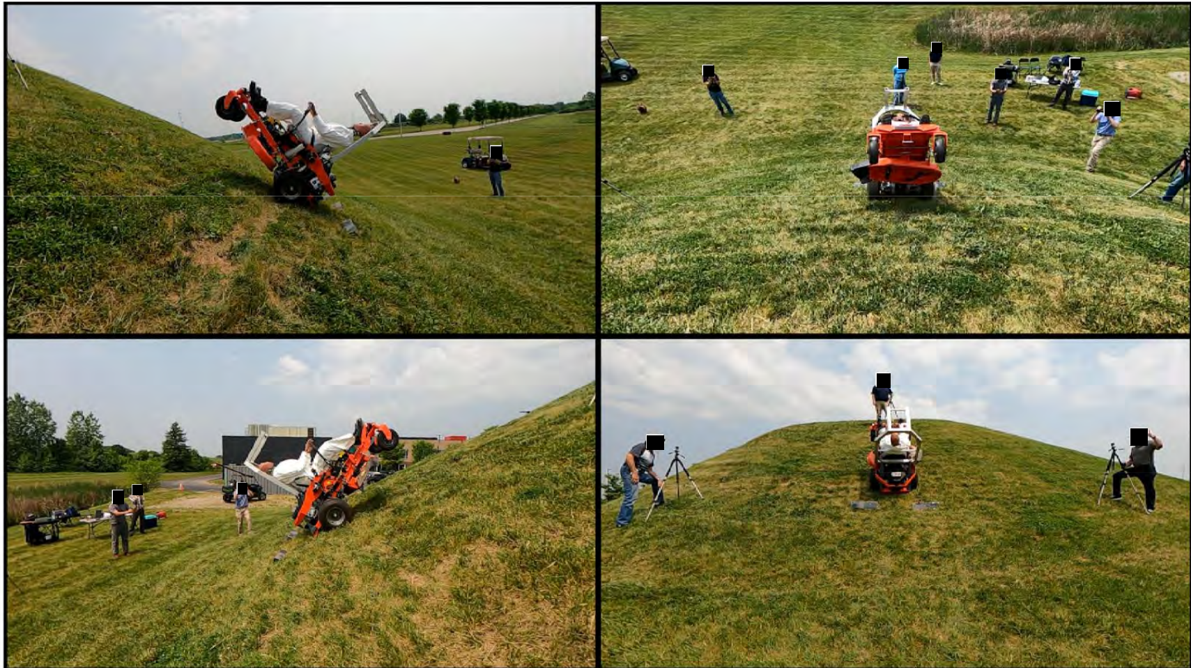
Zero-Turn Mower – Rearward Pitchover with ROPS
