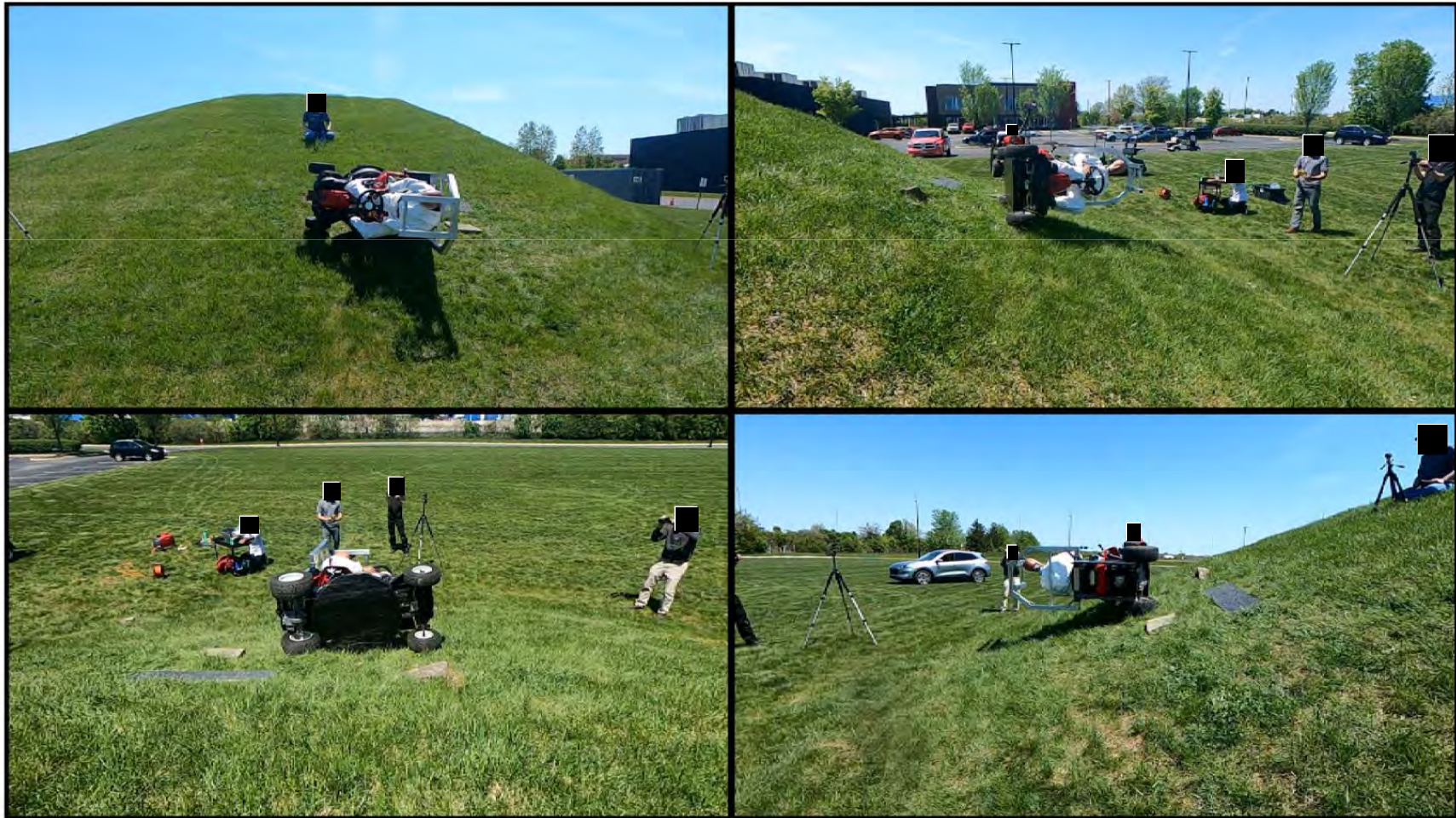
Tractor Style Mower – Lateral Rollover with ROPS
