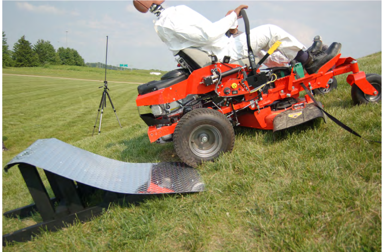
Side View for Quasi-Lateral Rollover Test
