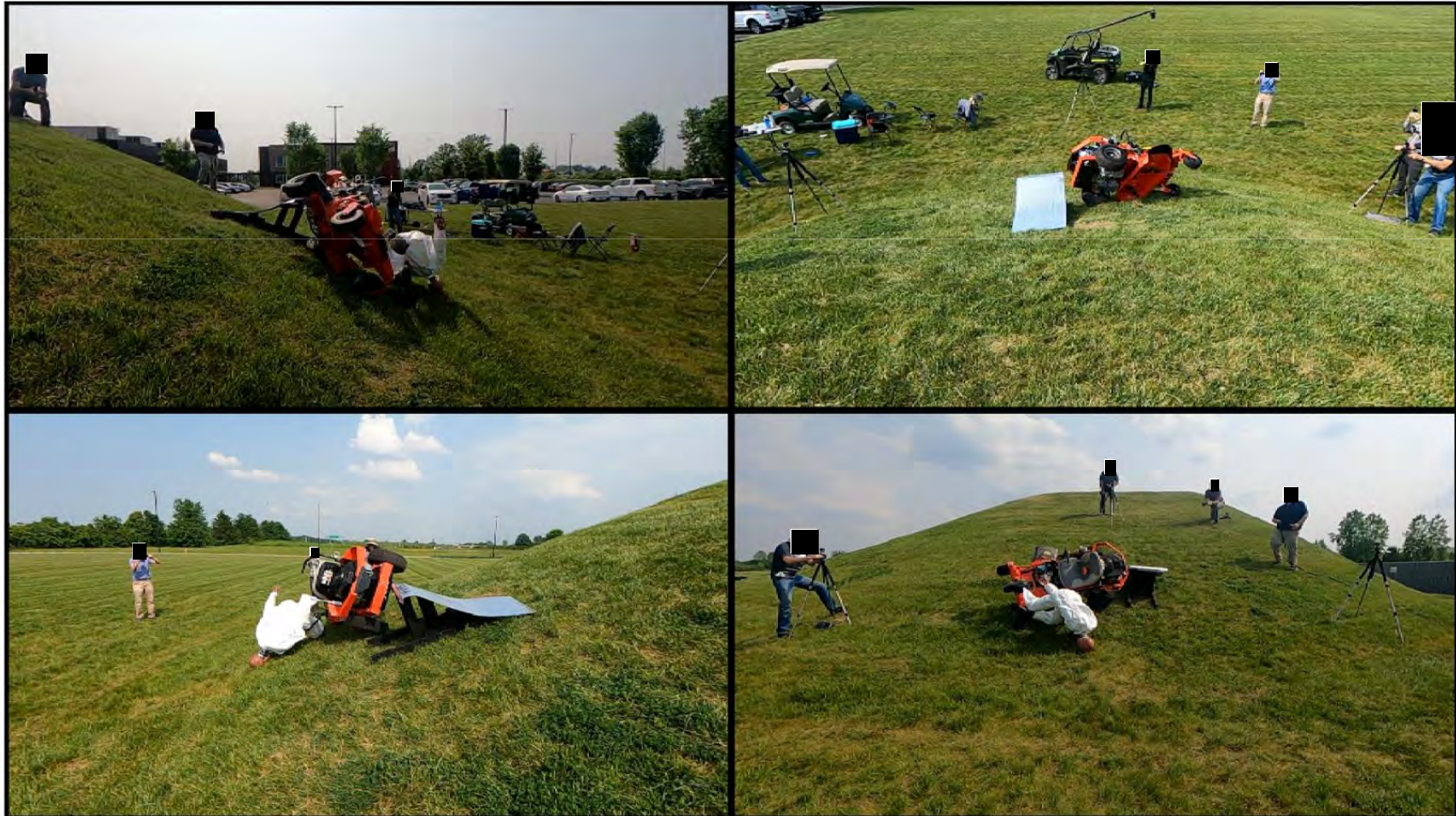
Zero-Turn Mower – Quasi-Lateral Rollover without ROPS
