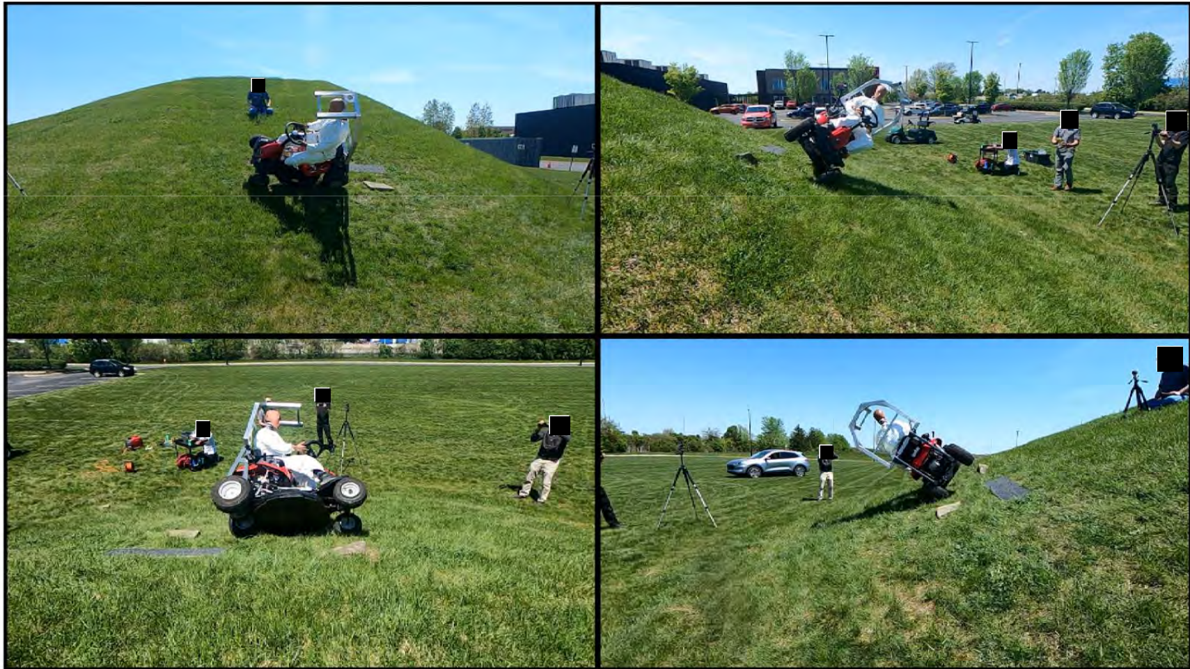
Tractor Style Mower – Lateral Rollover with ROPS
