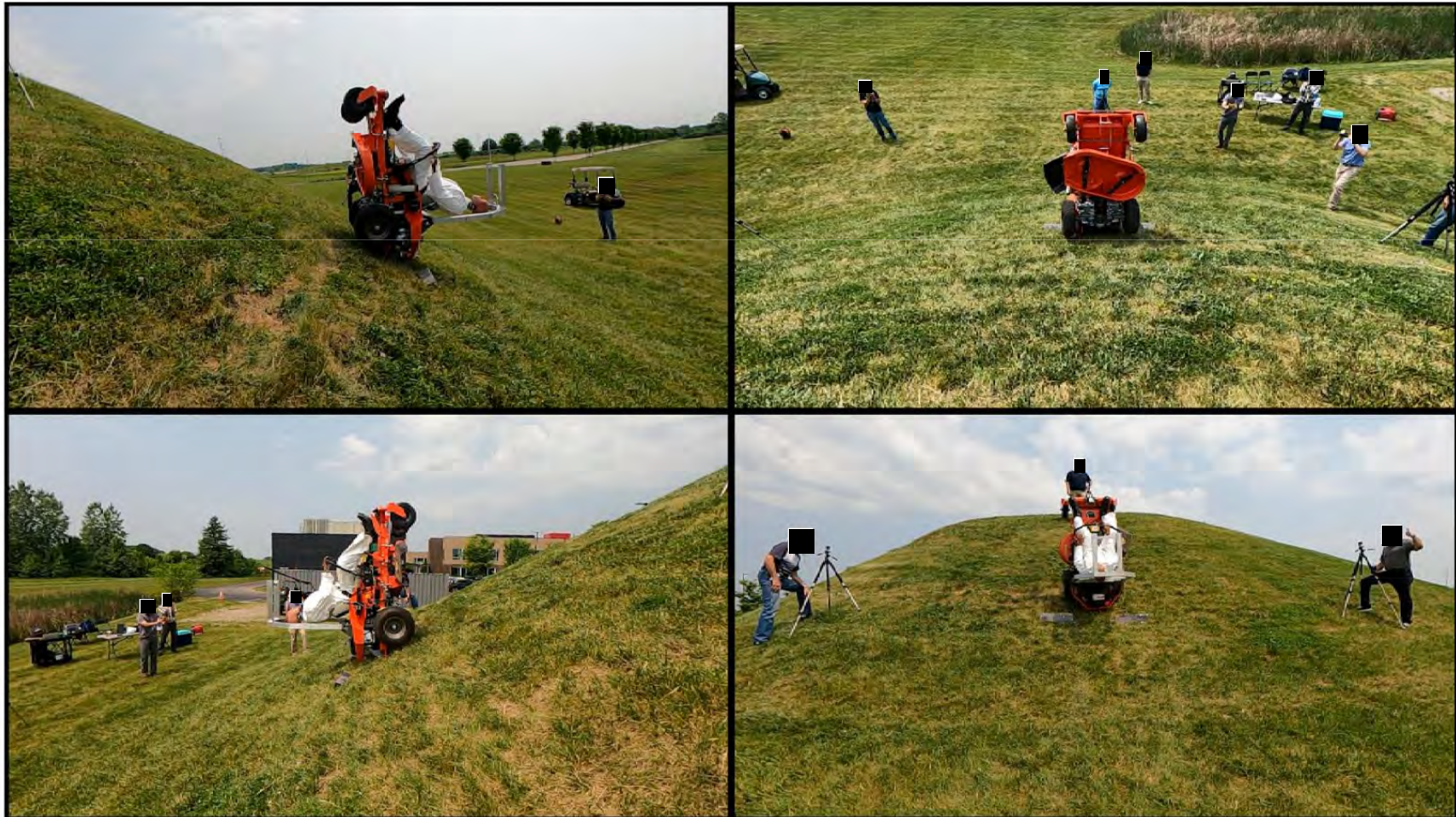
Zero-Turn Mower – Rearward Pitchover with ROPS
