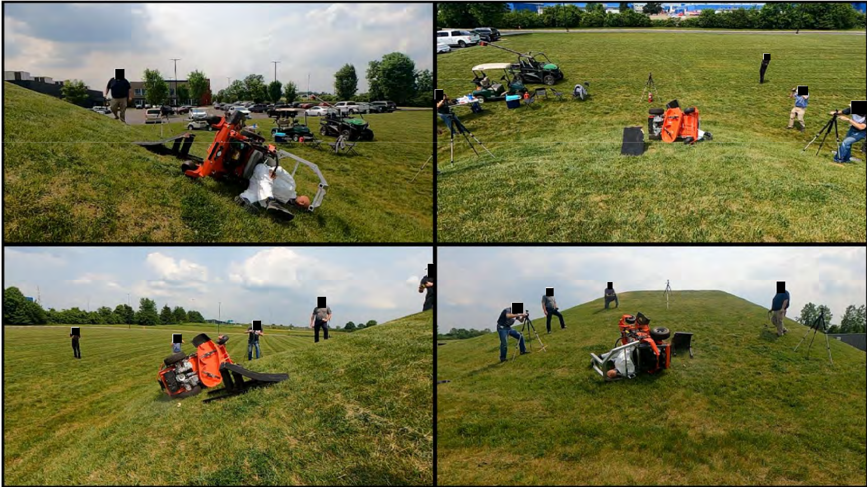
Zero-Turn Mower – Quasi-Lateral Rollover with ROPS
