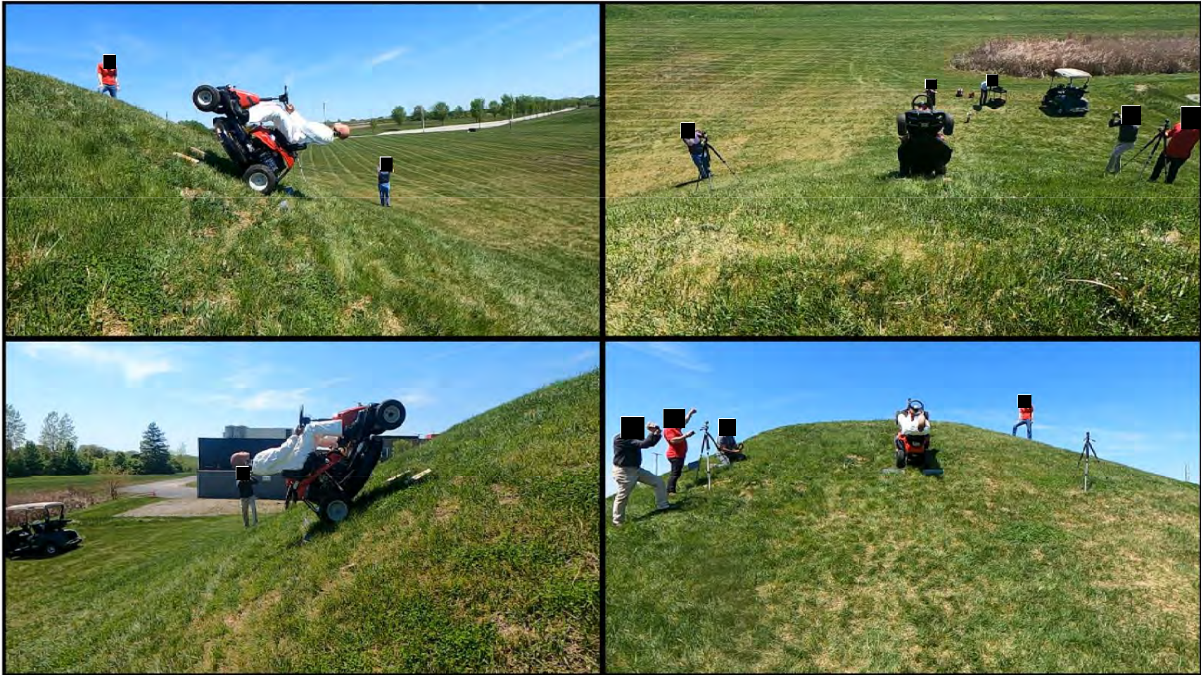
Tractor Style Mower – Rearward Pitchover without ROPS
