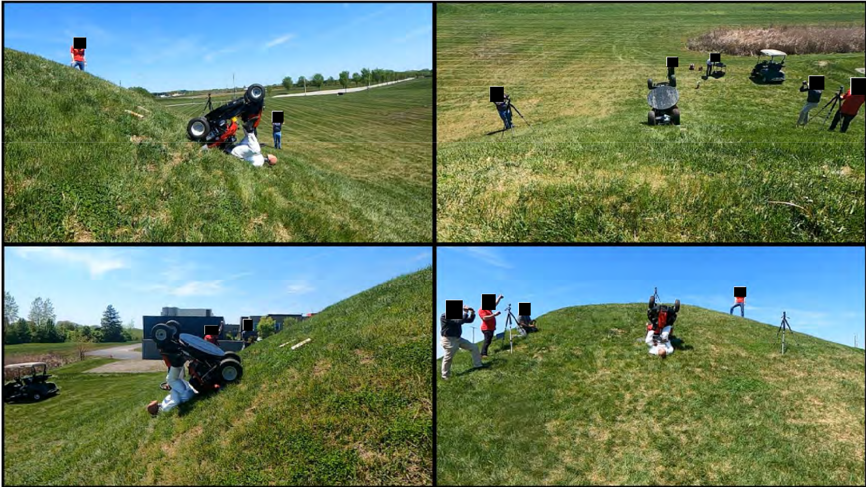
Tractor Style Mower – Rearward Pitchover without ROPS
