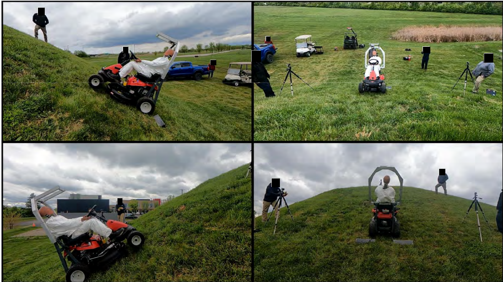
Tractor Style Mower – Rearward Pitchover with ROPS
