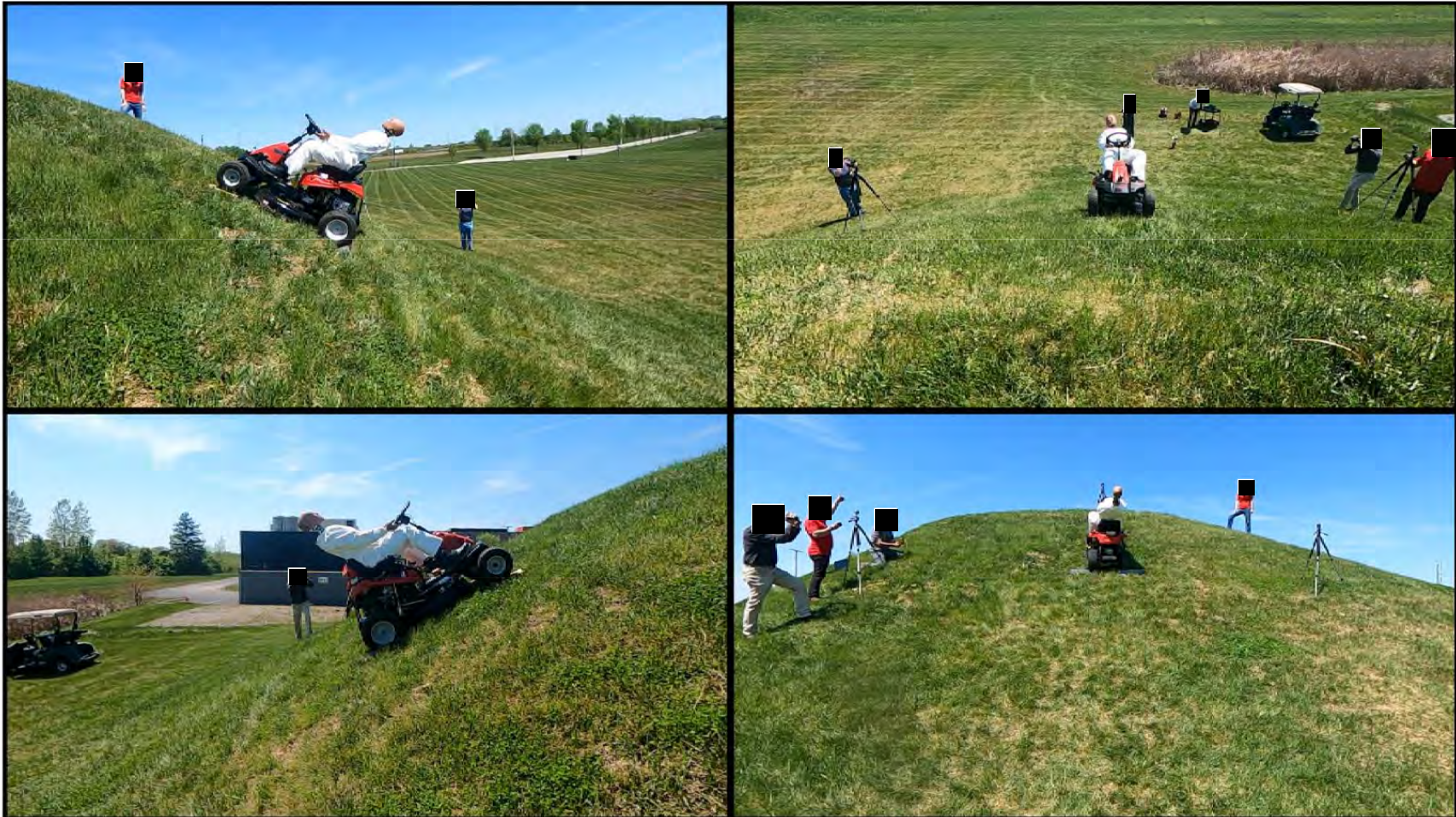
Tractor Style Mower – Rearward Pitchover without ROPS
