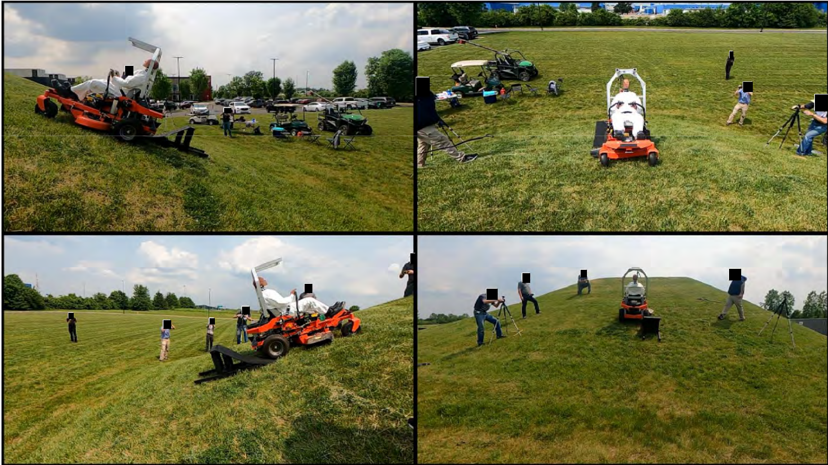
Zero-Turn Mower – Quasi-Lateral Rollover with ROPS
