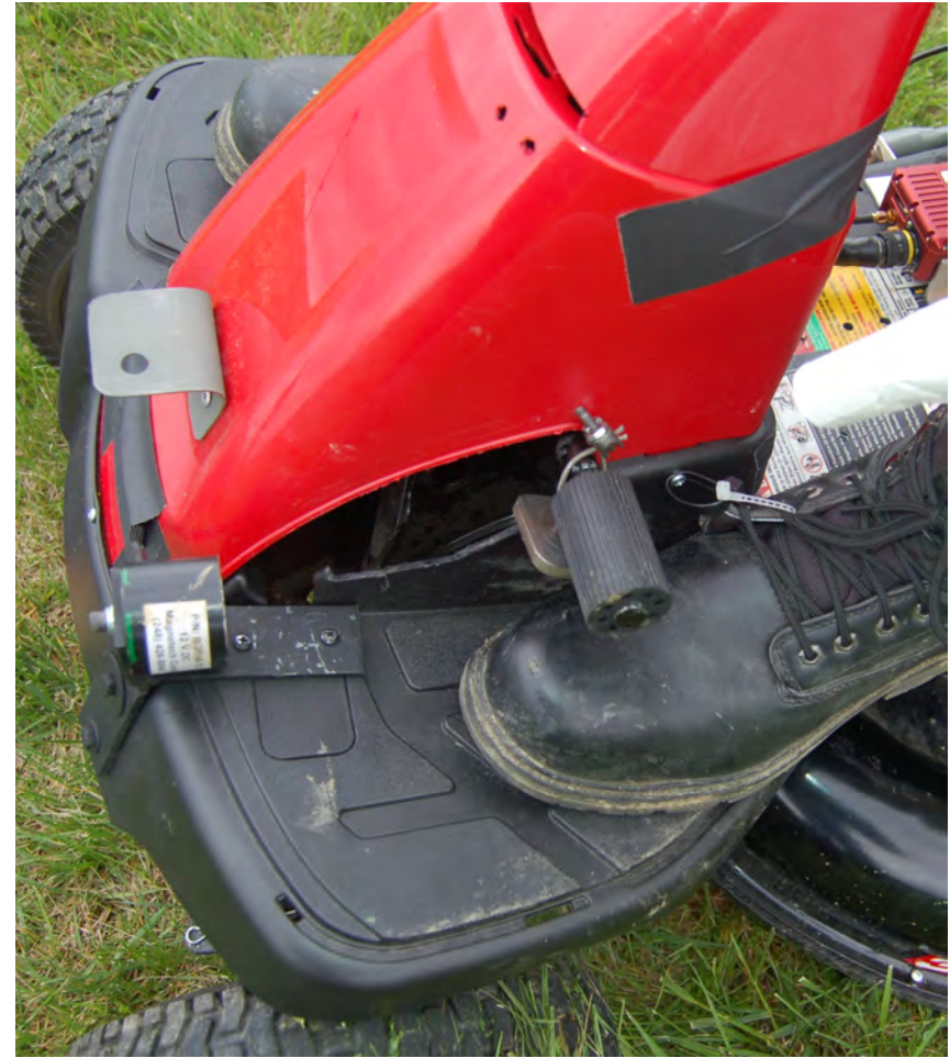
Vehicle Brake Off and Drive Engaged (Pedal Plate Released from Electromagnet)
