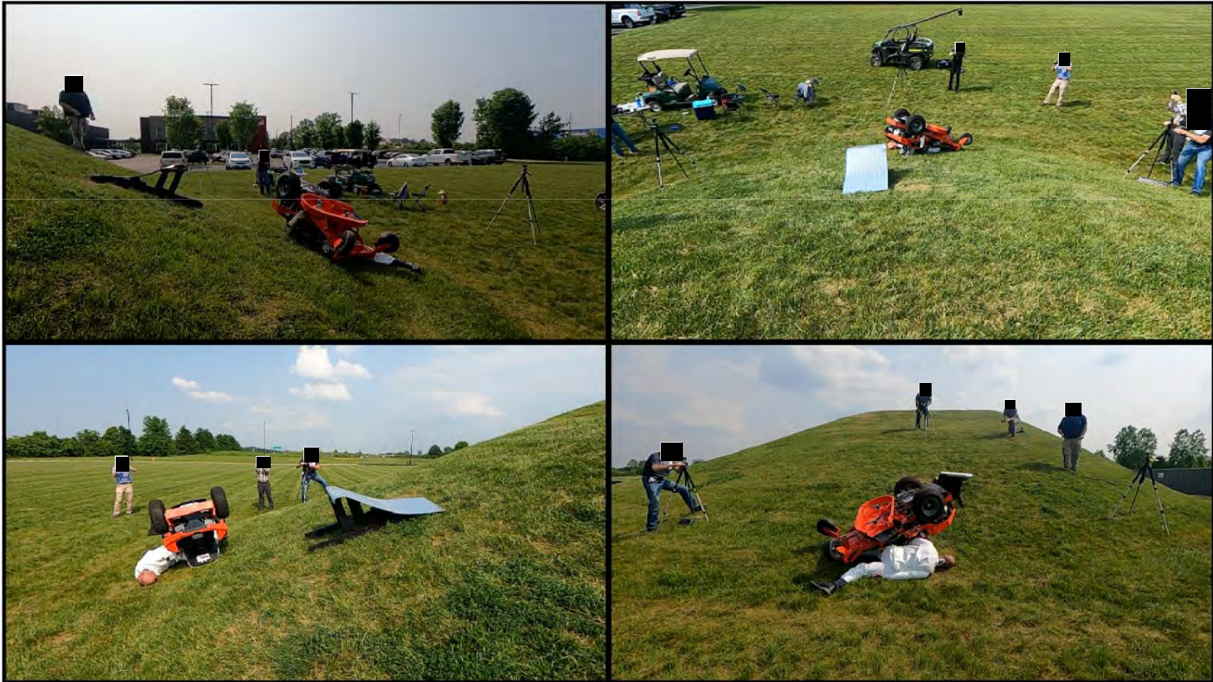
Zero-Turn Mower – Quasi-Lateral Rollover without ROPS
