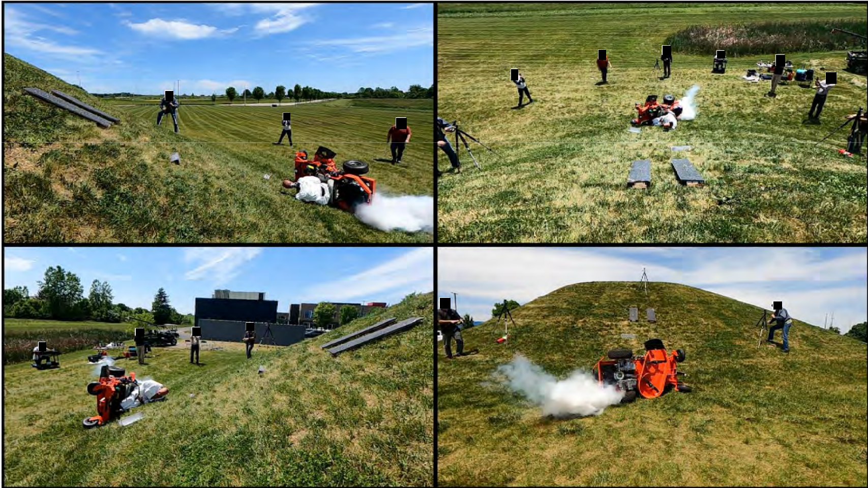
Zero-Turn Mower – Rearward Pitchover without ROPS
