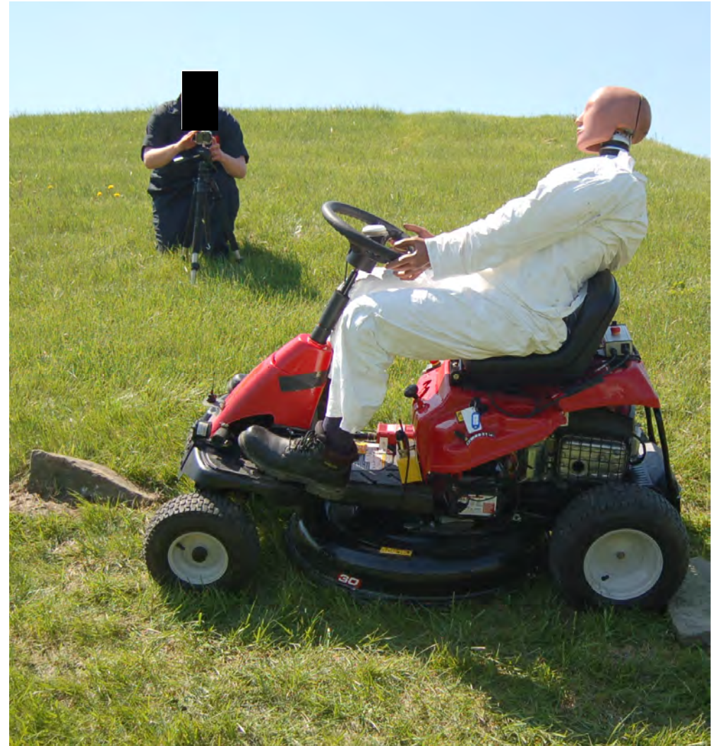
Side View for Lateral Rollover Test
