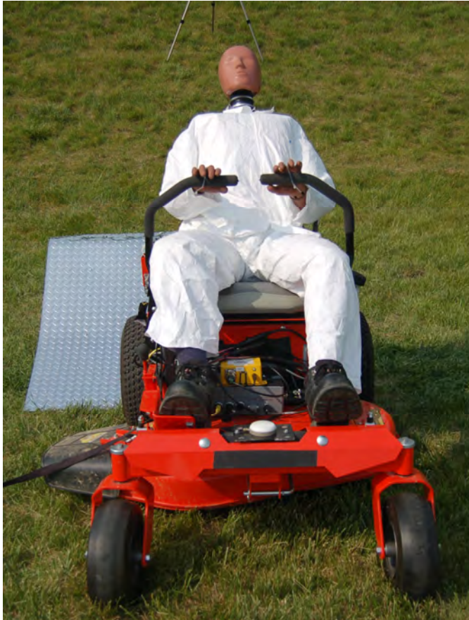
Front View for Quasi-Lateral Rollover Test
