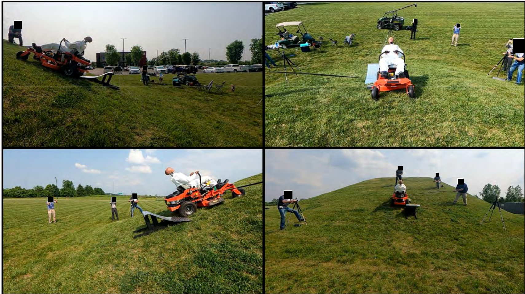
Zero-Turn Mower – Quasi-Lateral Rollover without ROPS
