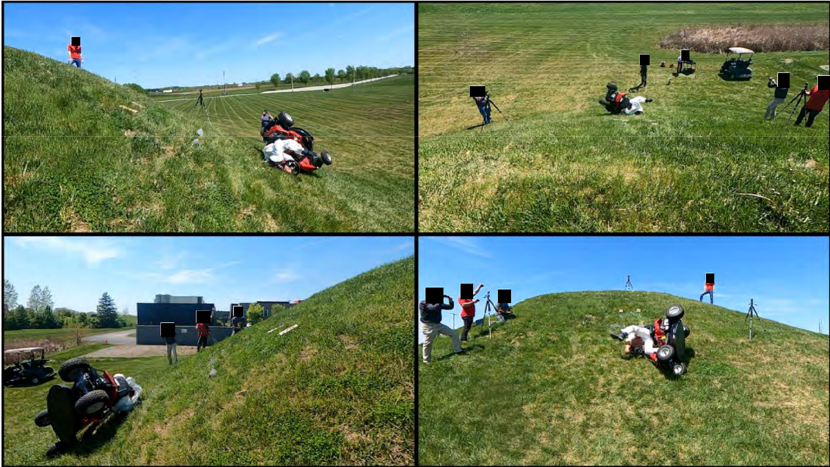
Tractor Style Mower – Rearward Pitchover without ROPS
