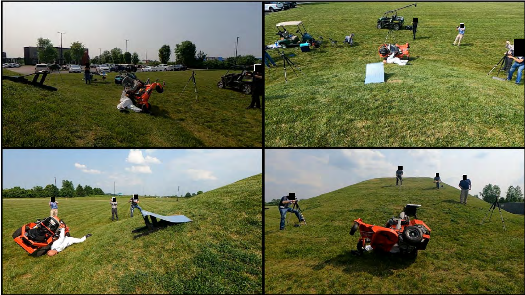
Zero-Turn Mower – Quasi-Lateral Rollover without ROPS
