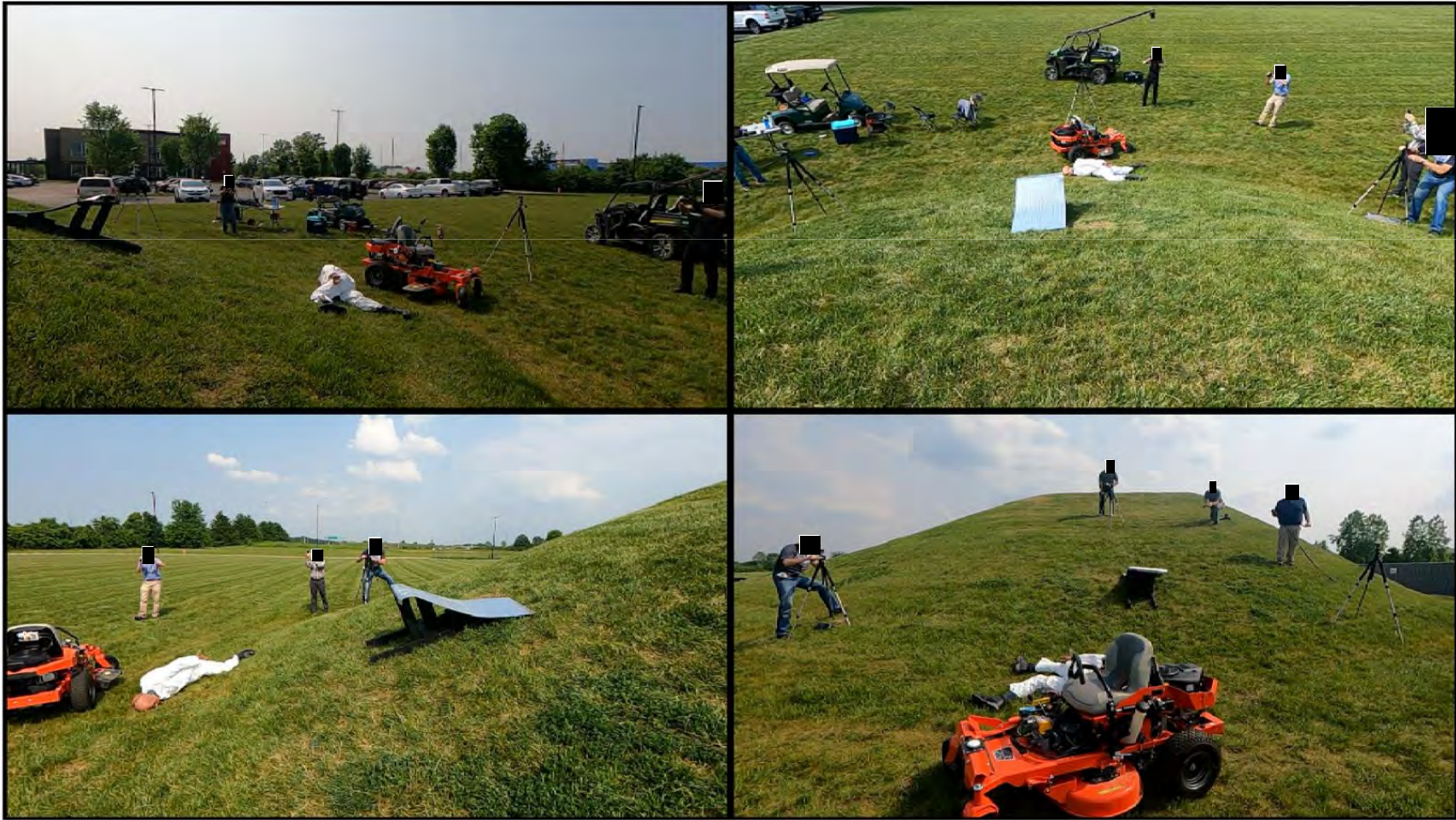
Zero-Turn Mower – Quasi-Lateral Rollover without ROPS
