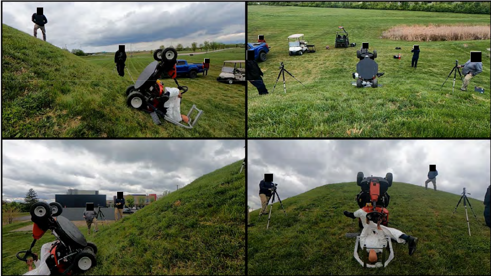
Tractor Style Mower – Rearward Pitchover with ROPS
