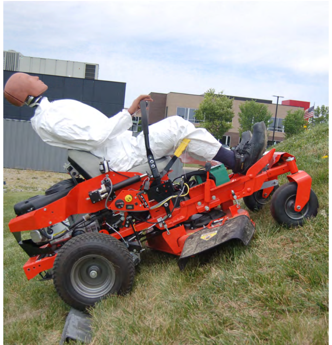
Side View for Rearward Pitchover Test
