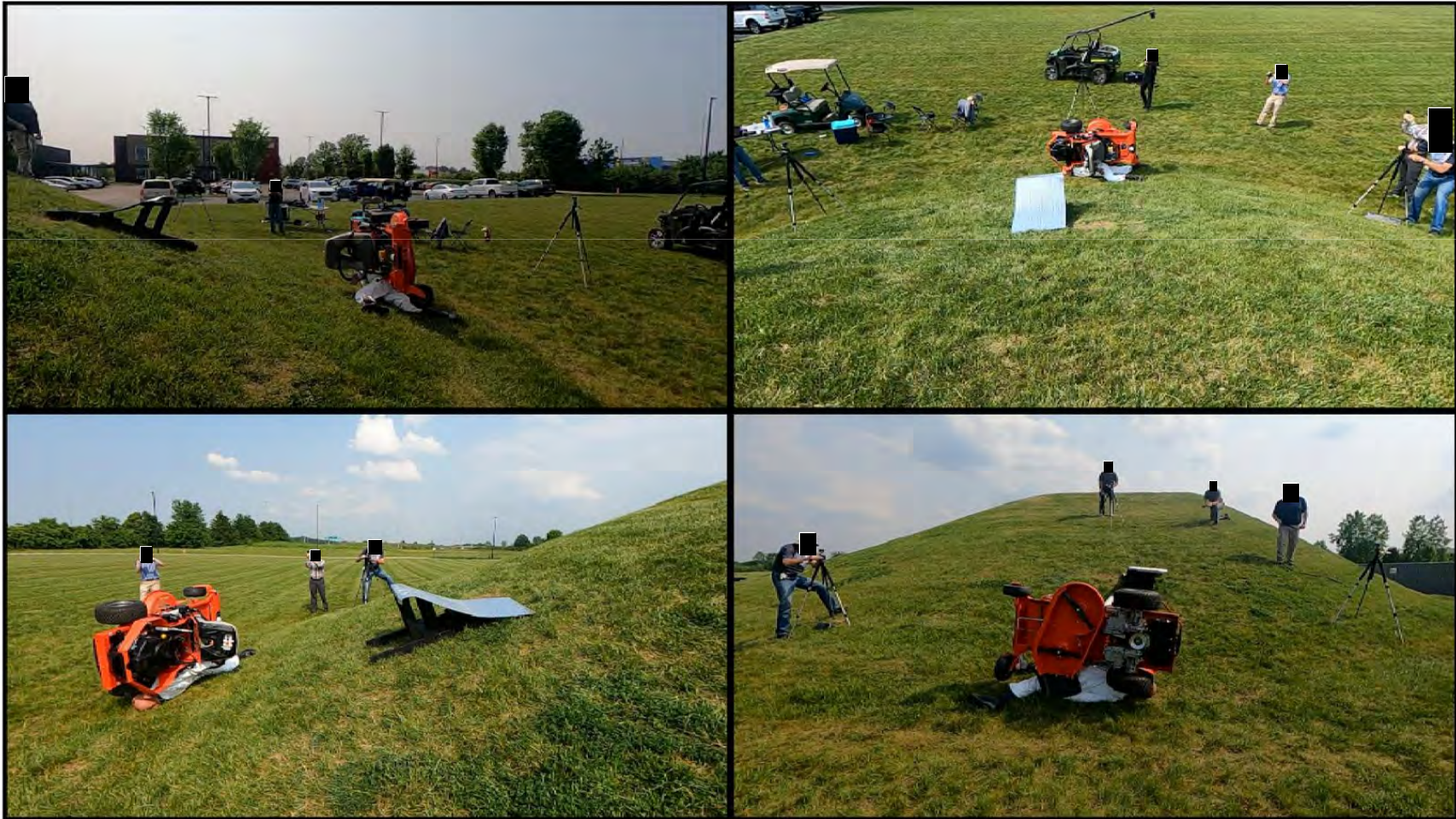
Zero-Turn Mower – Quasi-Lateral Rollover without ROPS
