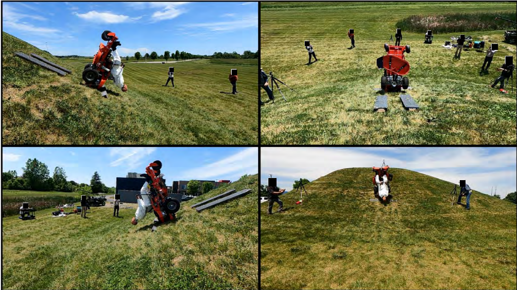
Zero-Turn Mower – Rearward Pitchover without ROPS
