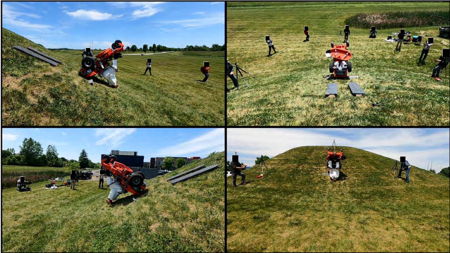
Zero-Turn Mower – Rearward Pitchover without ROPS
