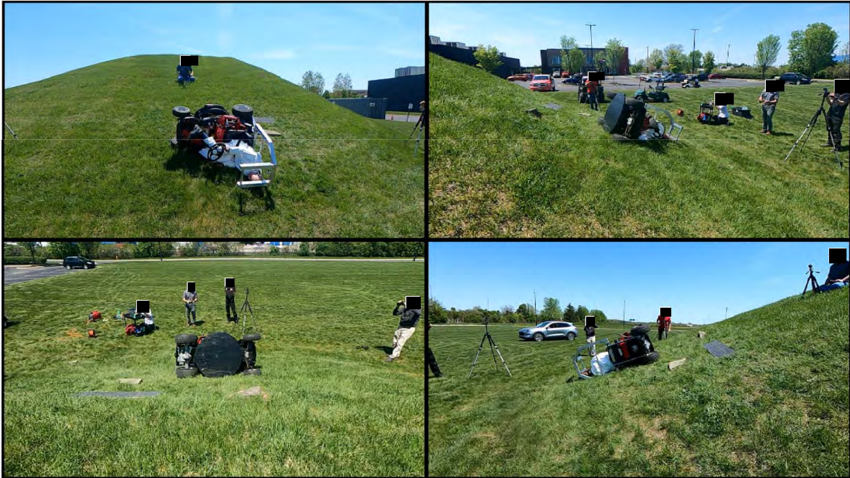
Tractor Style Mower – Lateral Rollover with ROPS
