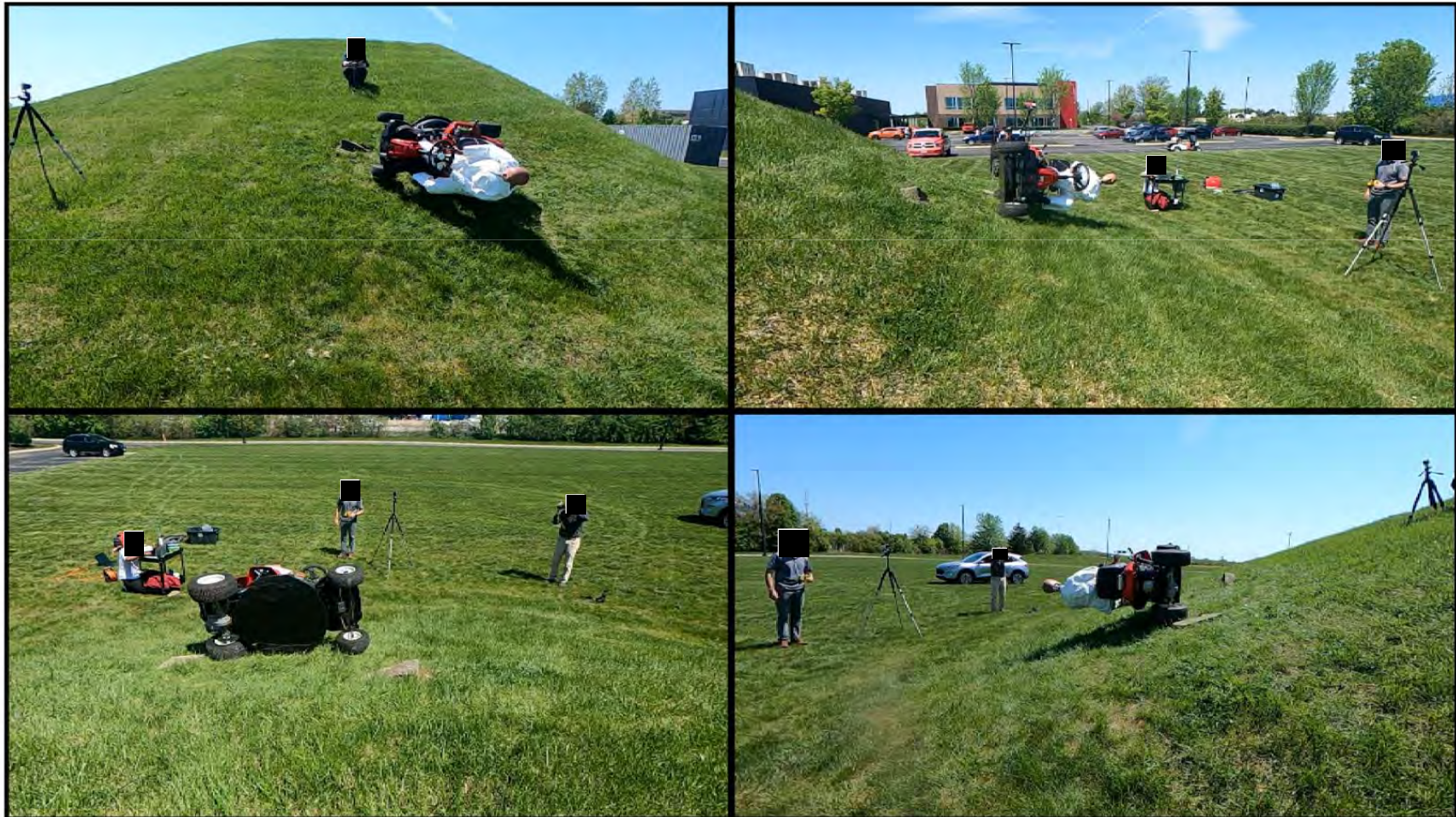
Tractor Style Mower – Lateral Rollover without ROPS
