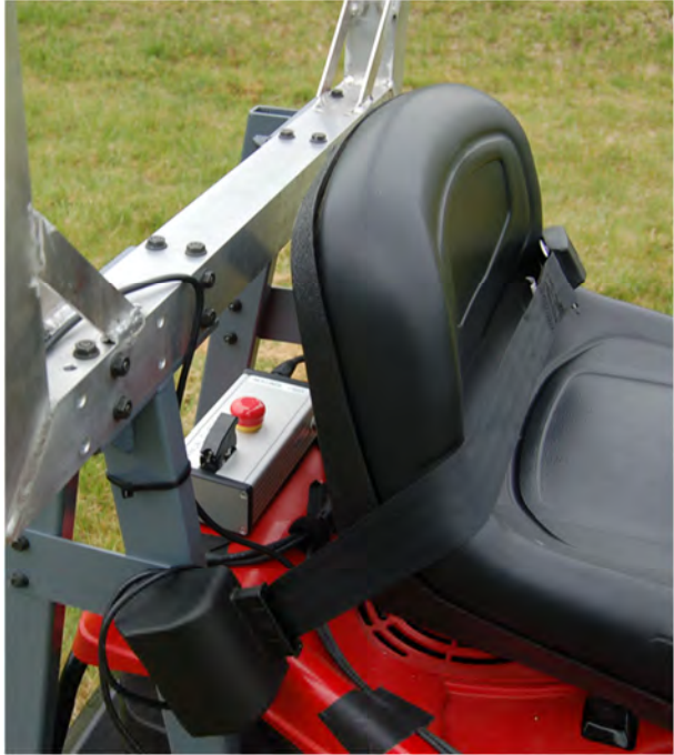
Seat Belt with Anchors Installed on ROPS Frame
