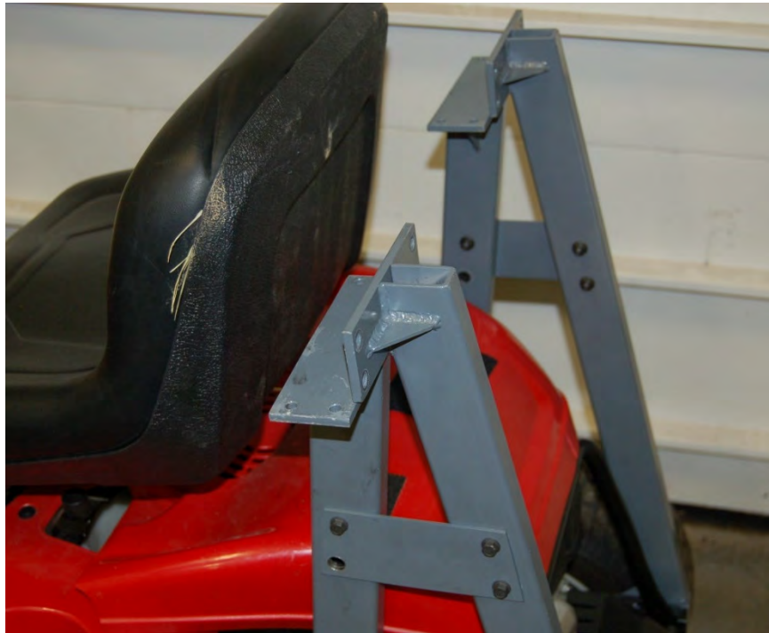
Figure 7: Photo Showing Top of the Lower ROPS Section for the Tractor Mower
