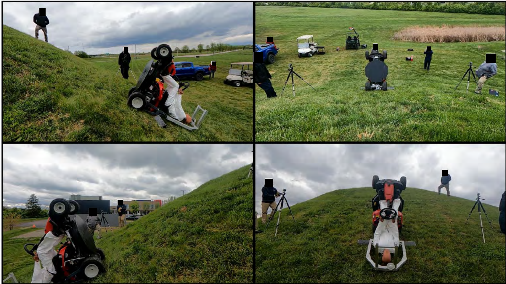
Tractor Style Mower – Rearward Pitchover with ROPS
