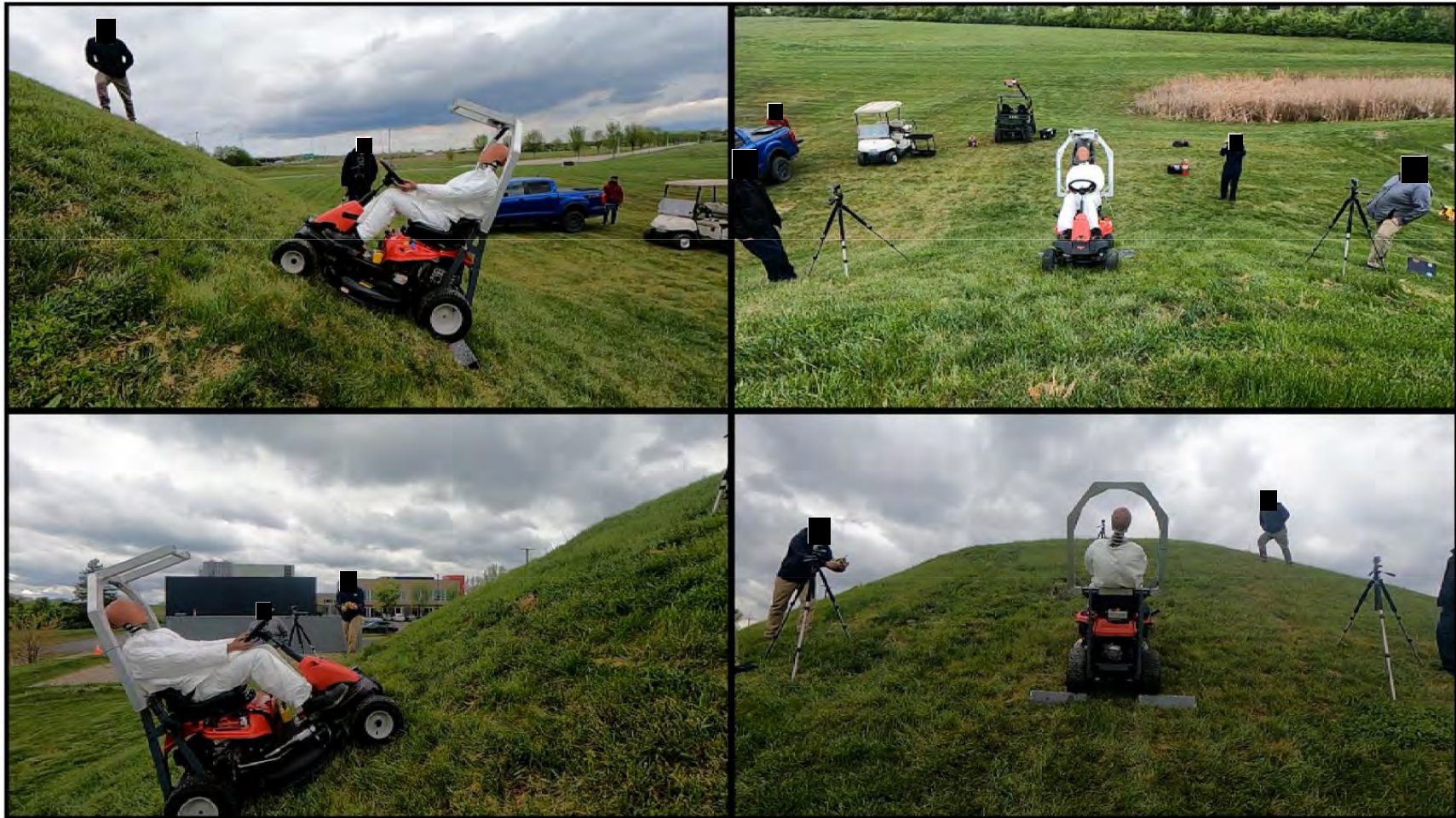
Tractor Style Mower – Rearward Pitchover with ROPS
