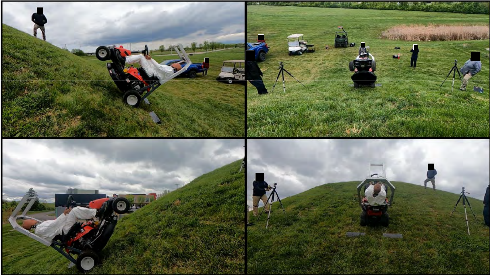
Tractor Style Mower – Rearward Pitchover with ROPS
