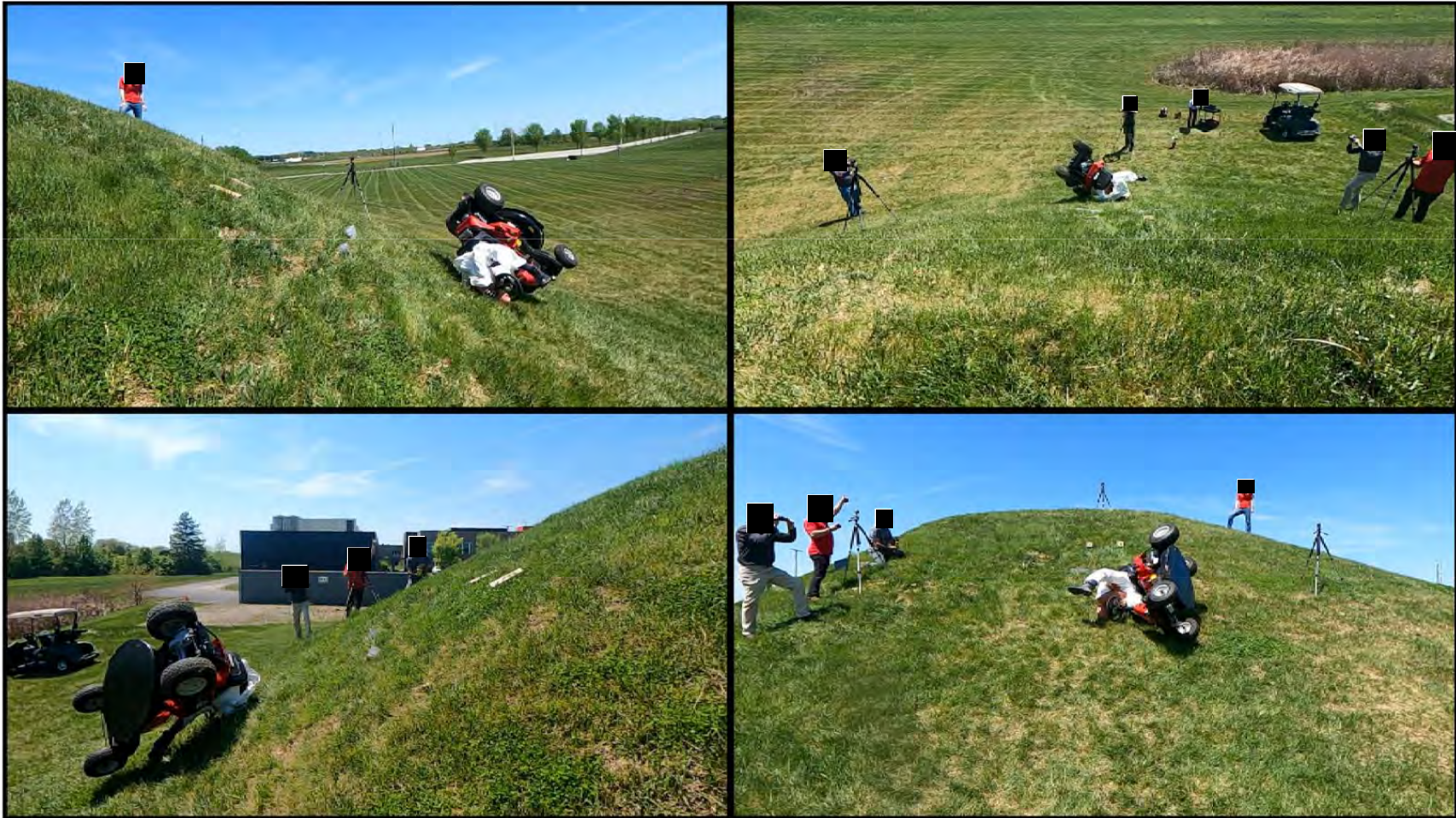
Tractor Style Mower – Rearward Pitchover without ROPS
