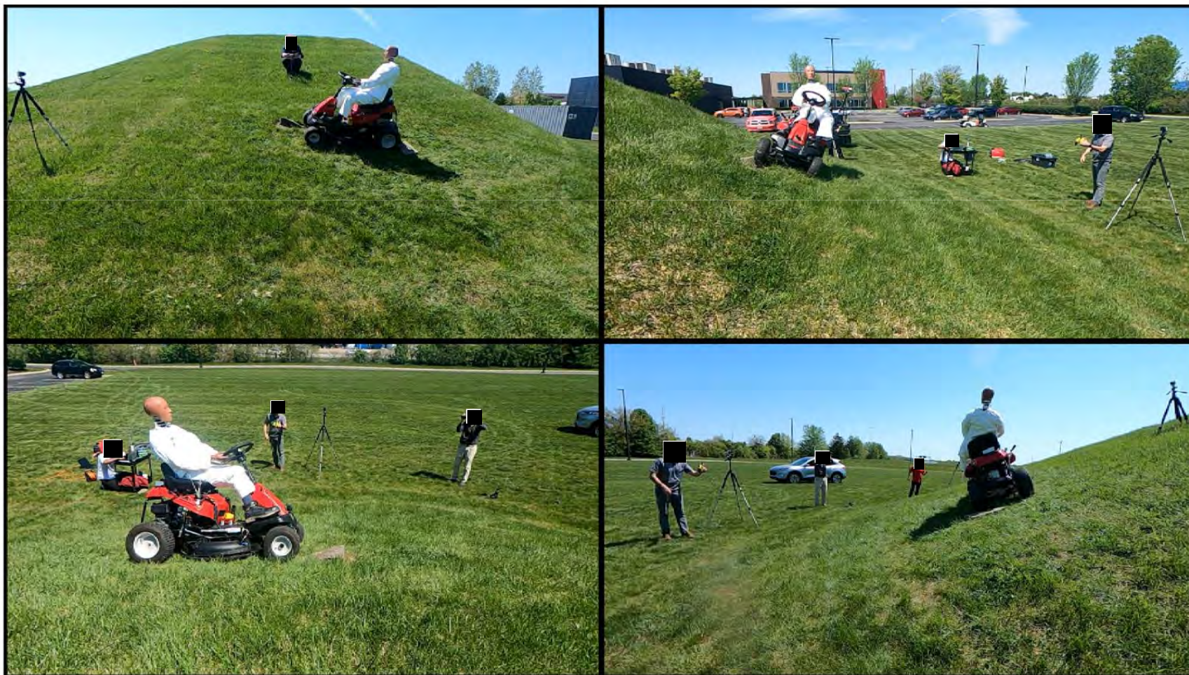
Tractor Style Mower – Lateral Rollover without ROPS
