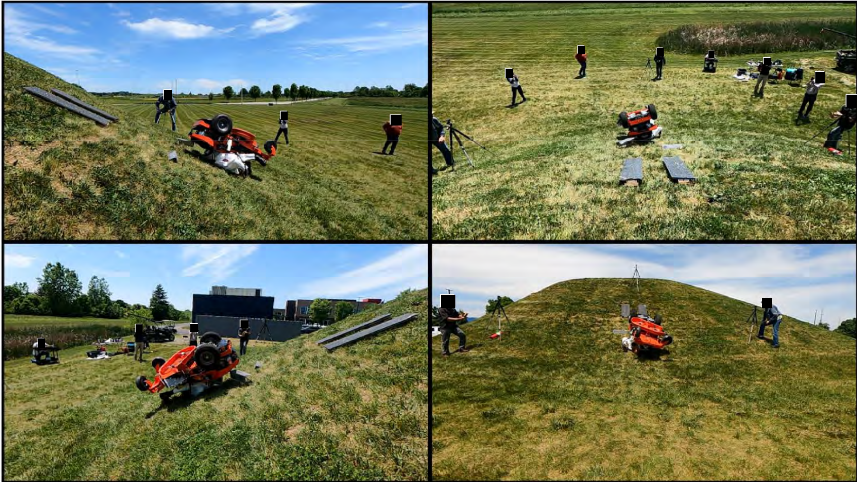
Zero-Turn Mower – Rearward Pitchover without ROPS
