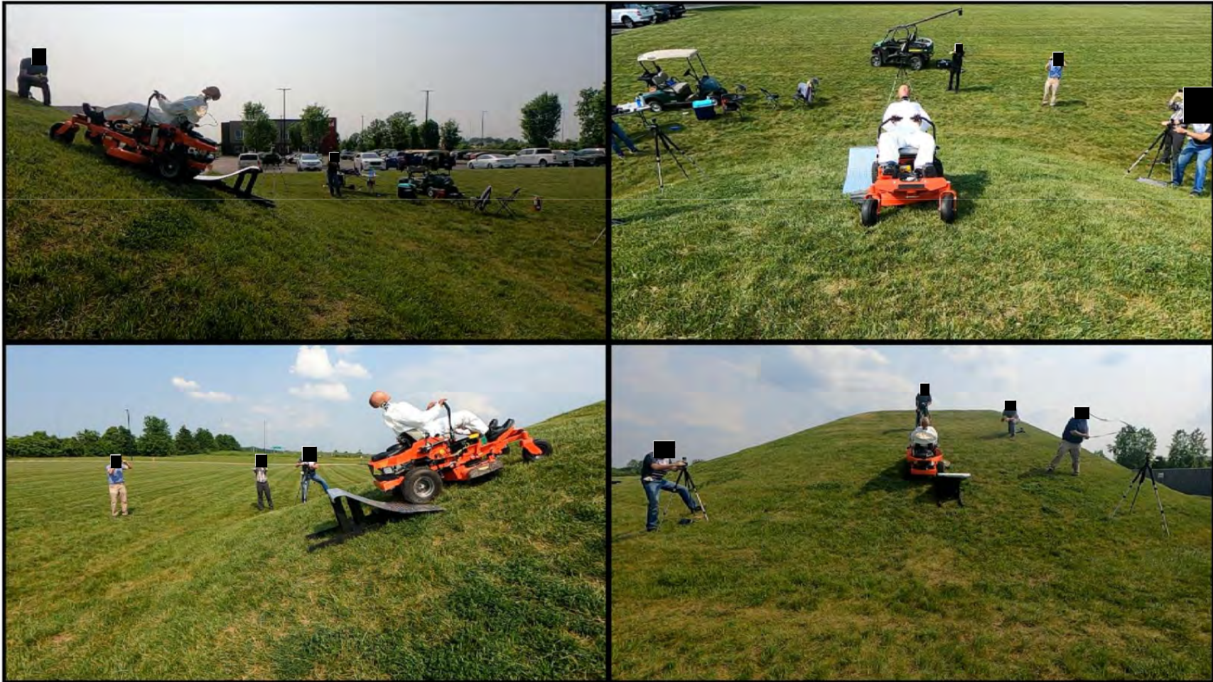
Zero-Turn Mower – Quasi-Lateral Rollover without ROPS
