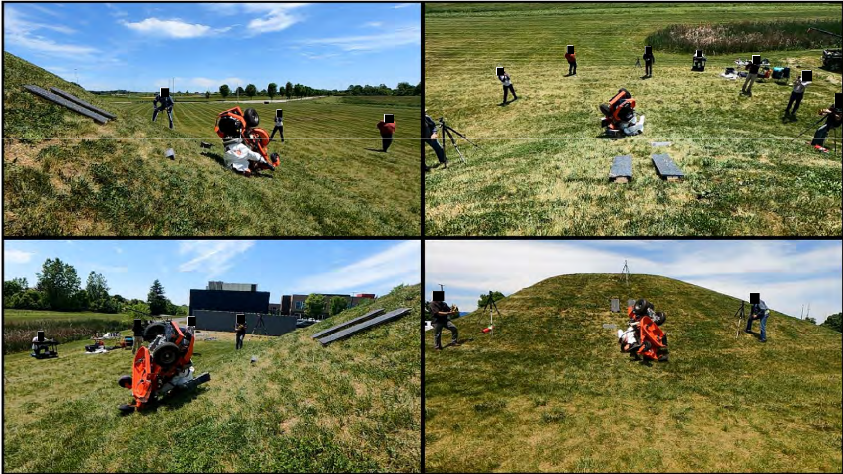
Zero-Turn Mower – Rearward Pitchover without ROPS
