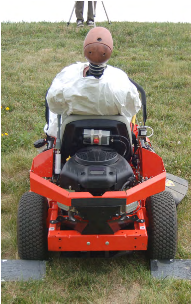
Rear View for Rearward Pitchover Test
