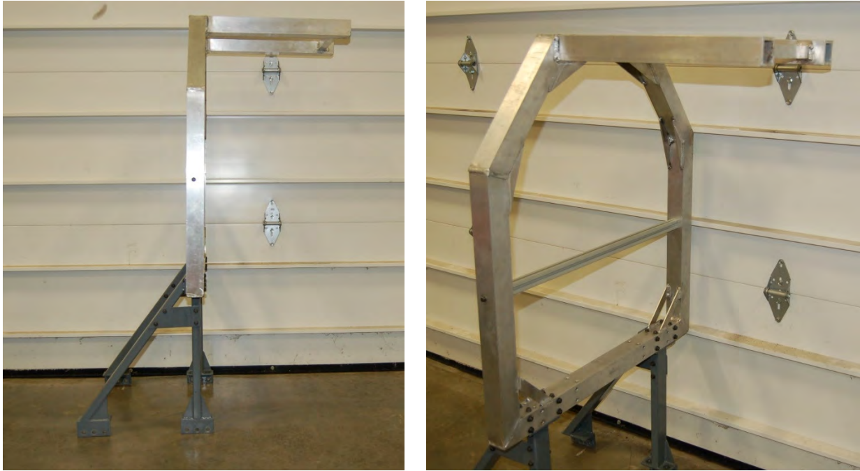
Figure 5: Left Photo: Overall View of Upper Section (Shiny Aluminum) and Lower Section (Steel Painted Gray) for the Zero-Turn Mower
