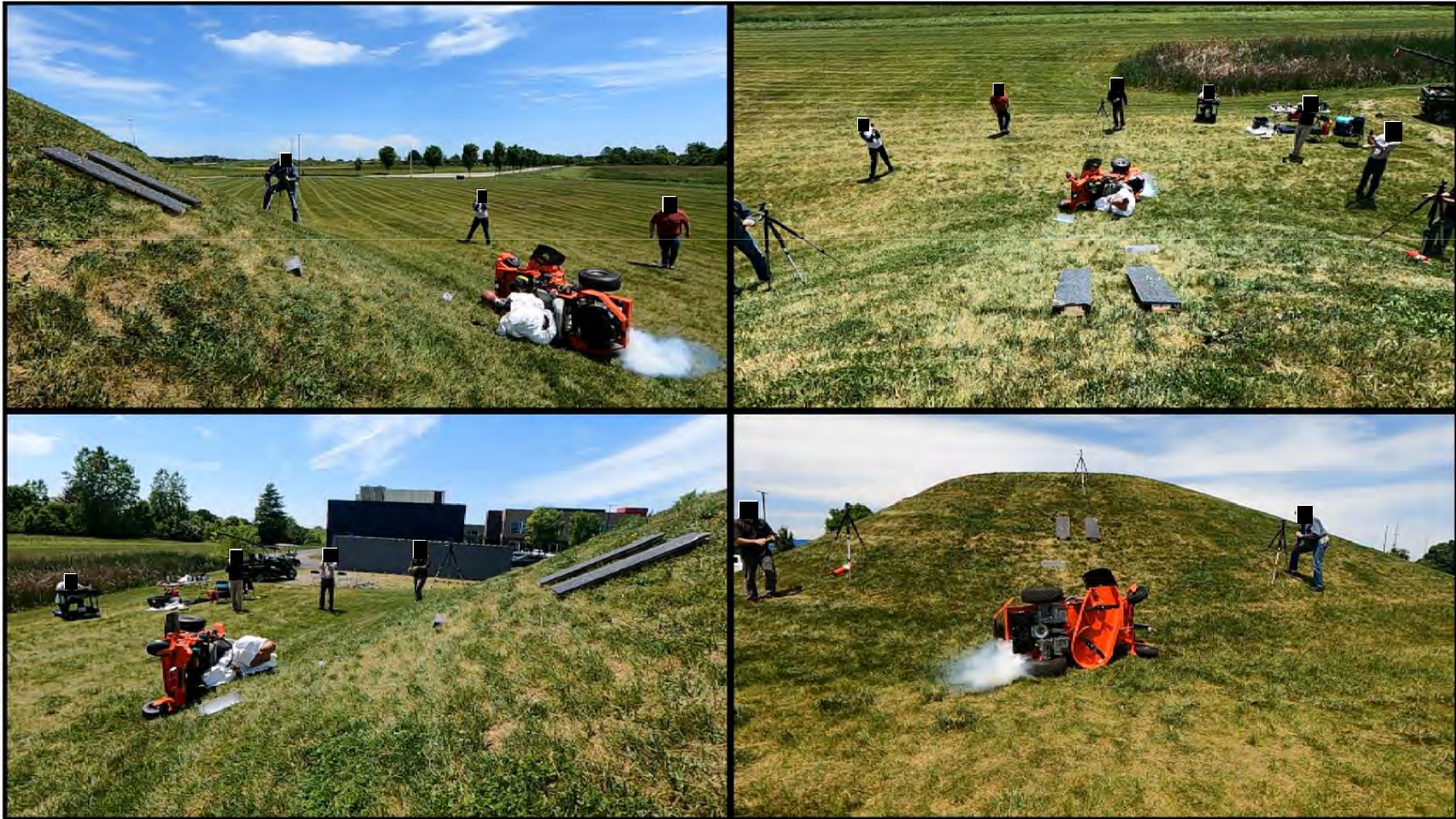
Zero-Turn Mower – Rearward Pitchover without ROPS
