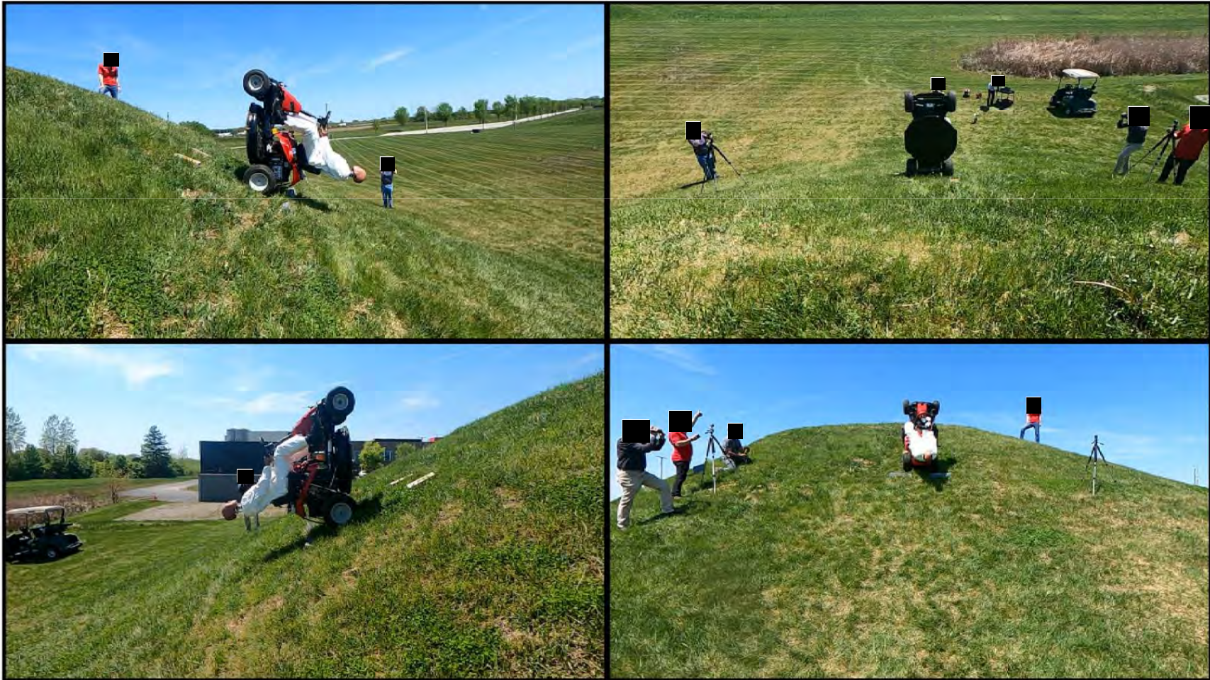
Tractor Style Mower – Rearward Pitchover without ROPS
