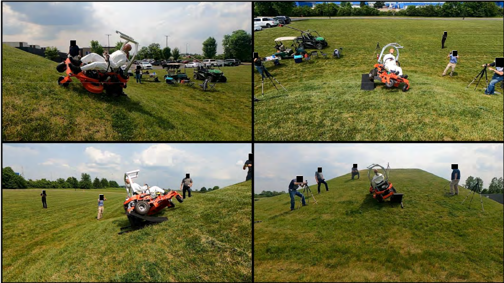
Zero-Turn Mower – Quasi-Lateral Rollover with ROPS
