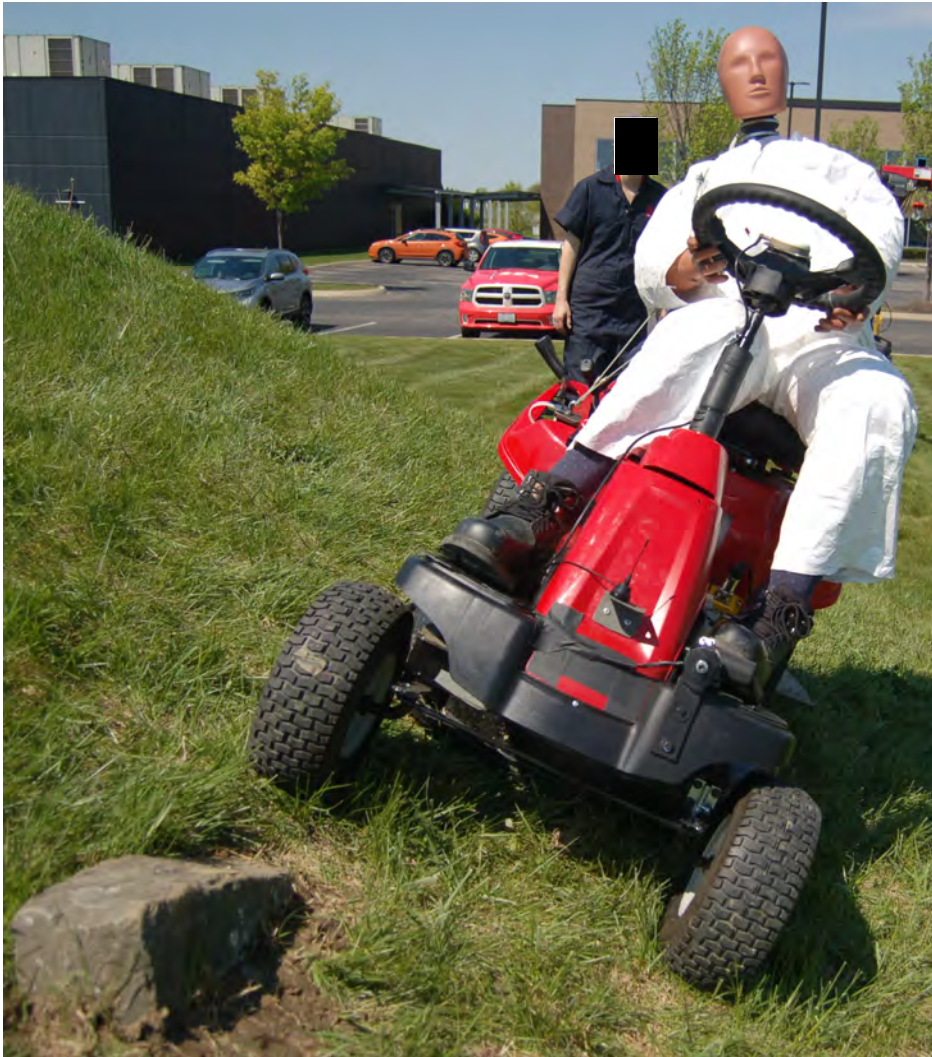
Front View for Lateral Rollover Test
