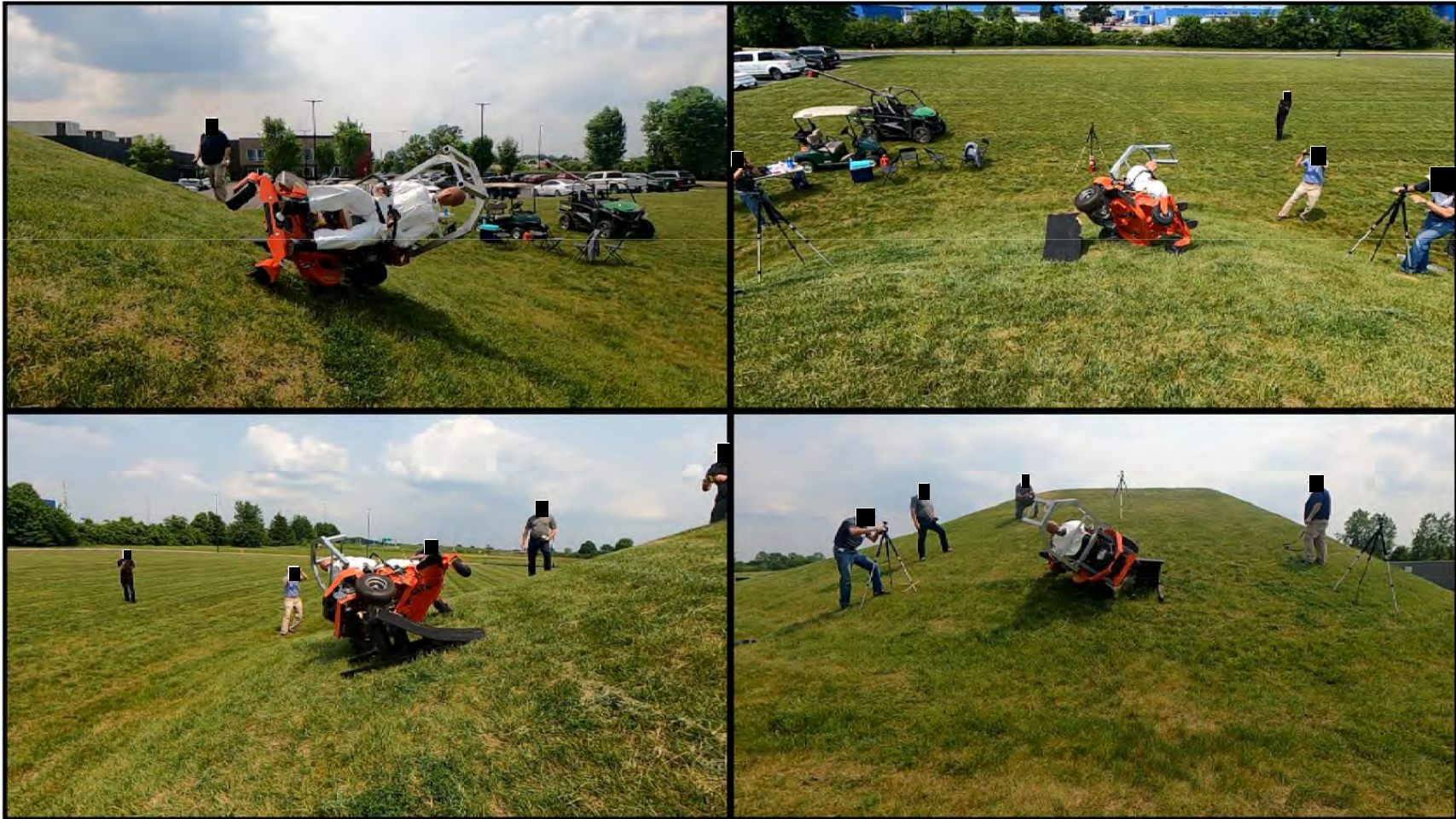
Zero-Turn Mower – Quasi-Lateral Rollover with ROPS
