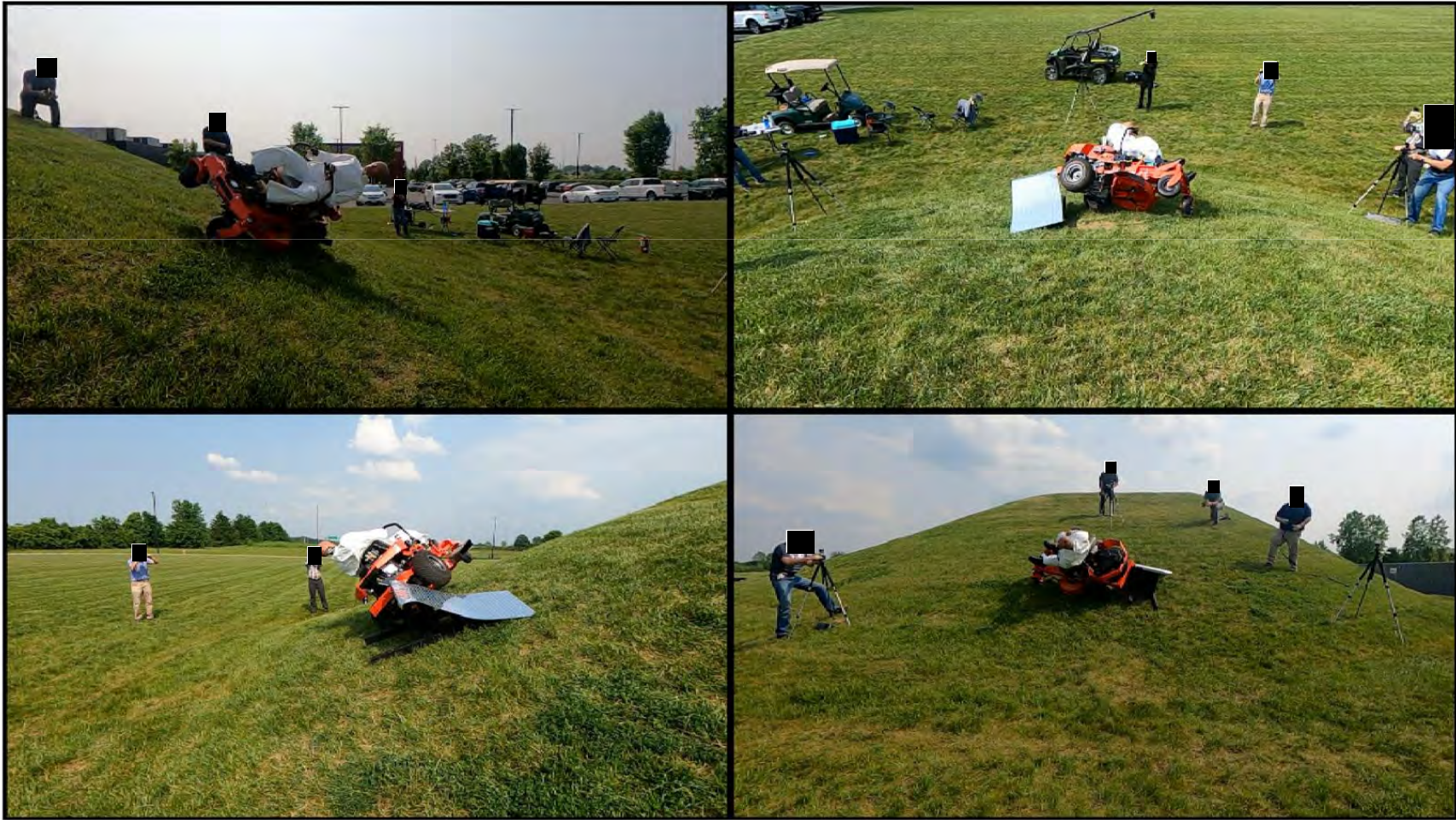
Zero-Turn Mower – Quasi-Lateral Rollover without ROPS
