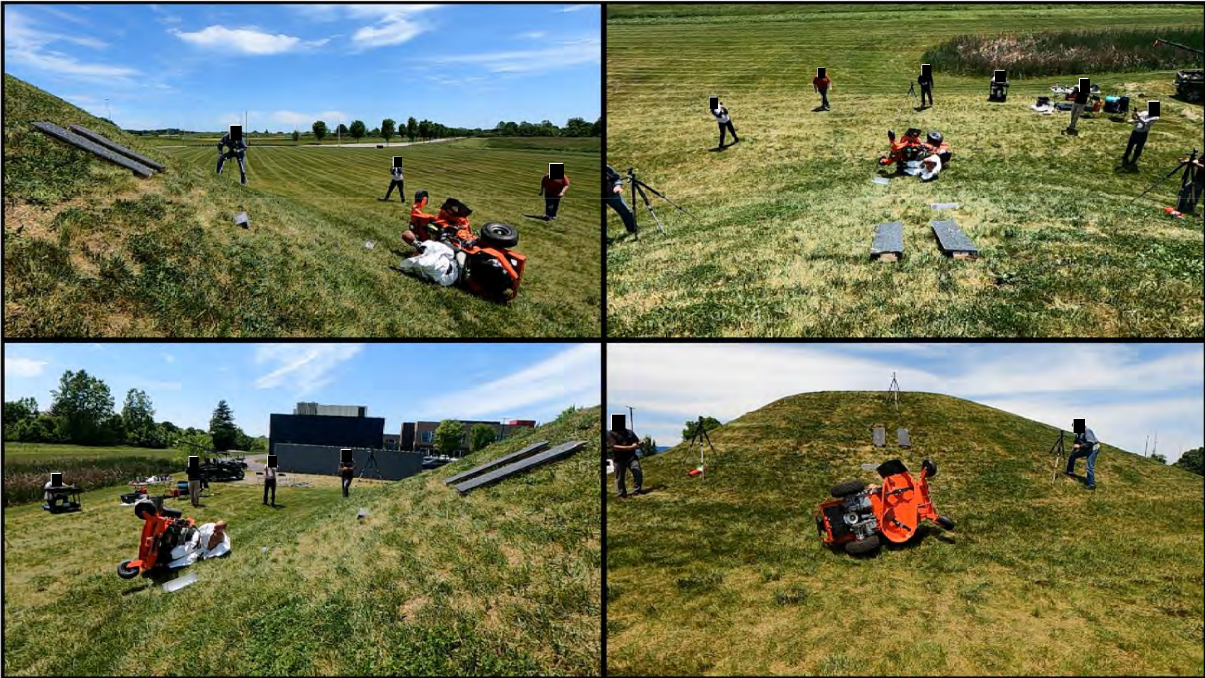
Zero-Turn Mower – Rearward Pitchover without ROPS
