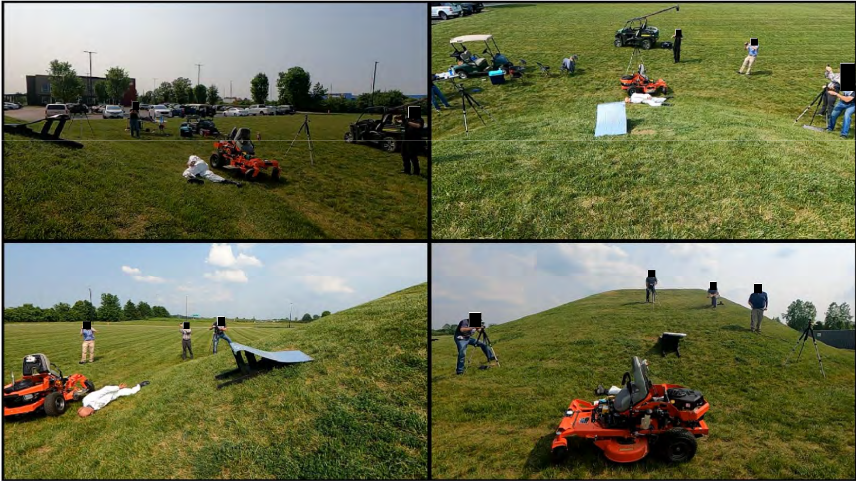
Zero-Turn Mower – Quasi-Lateral Rollover without ROPS
