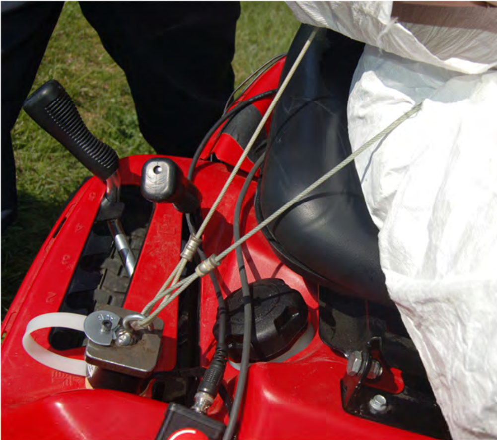
Restraint System Secure & Release Cables Connected to Electromagnet Plate
