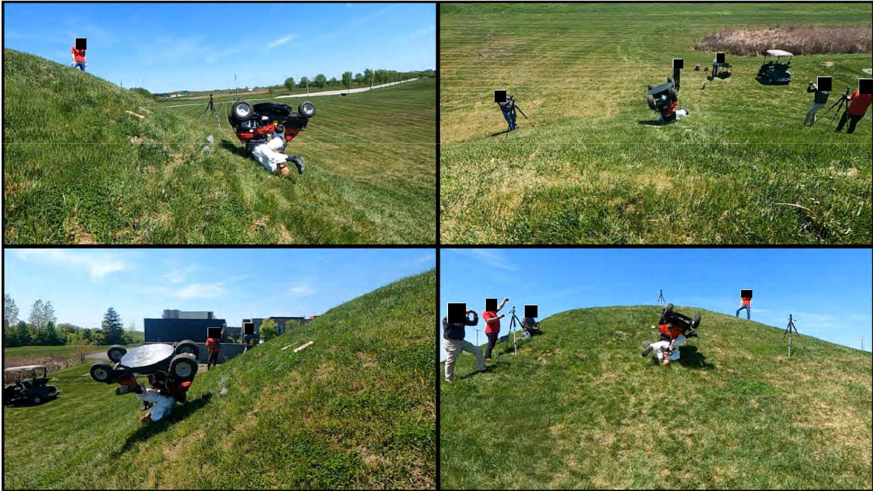
Tractor Style Mower – Rearward Pitchover without ROPS
