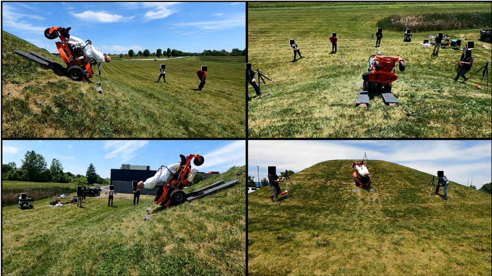
Zero-Turn Mower – Rearward Pitchover without ROPS
