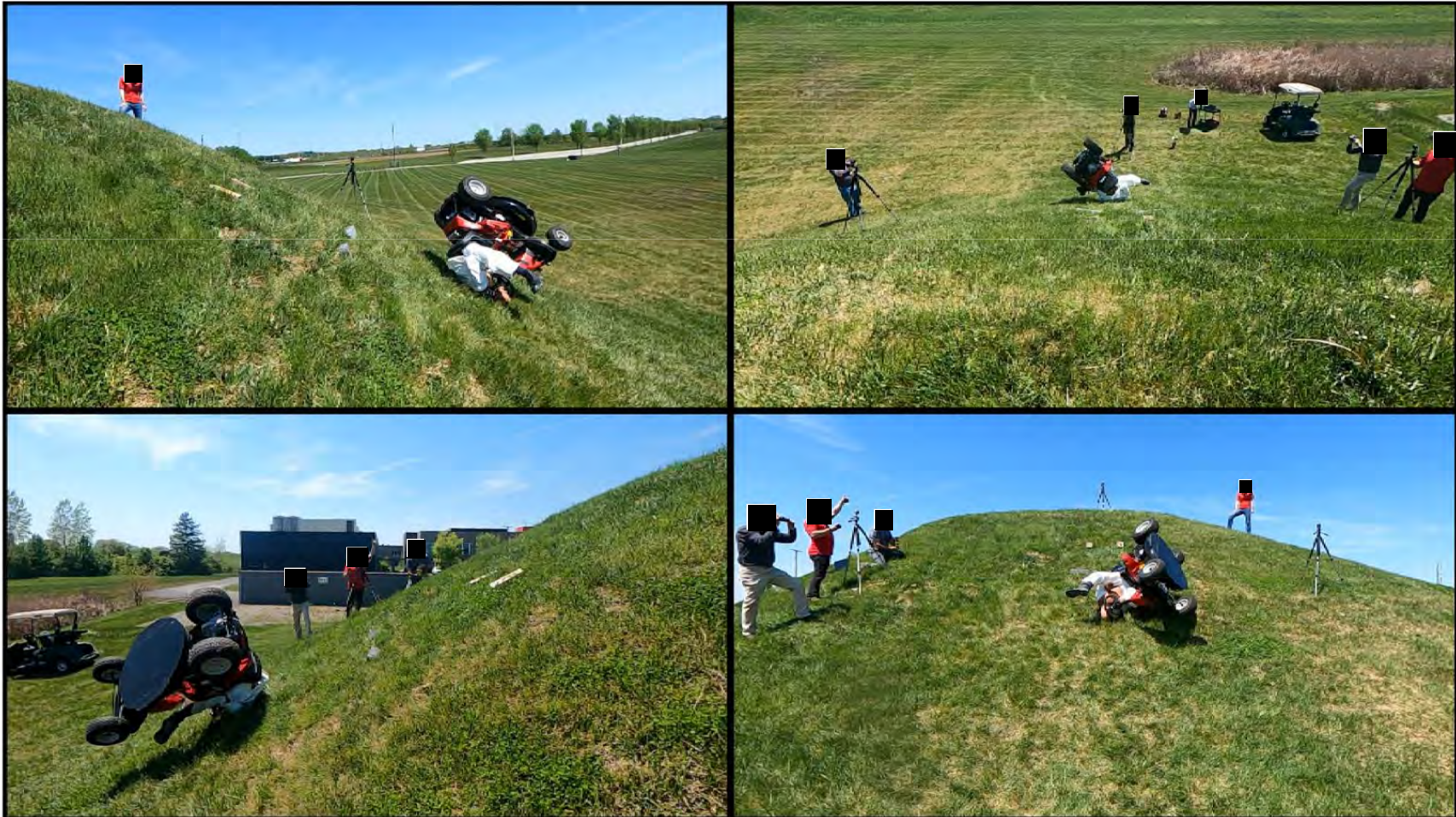
Tractor Style Mower – Rearward Pitchover without ROPS
