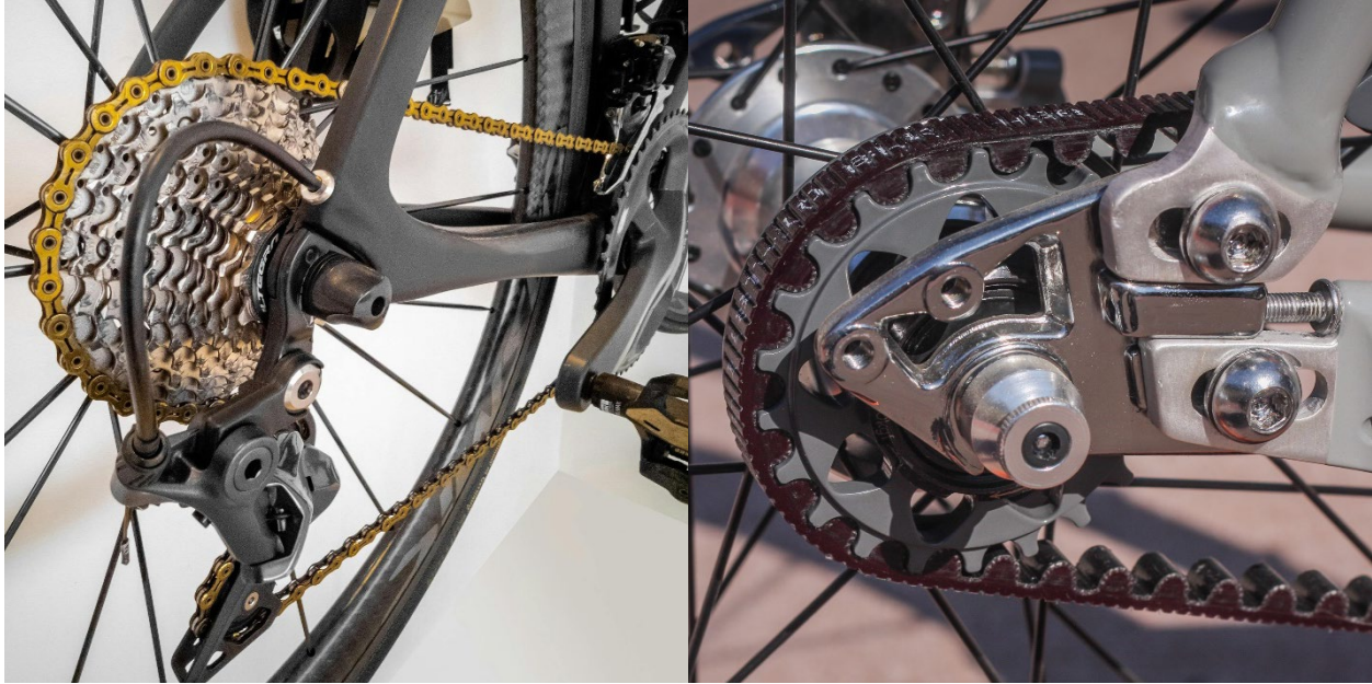
Figure 16. Drive systems: chain (left) and belt (right)
