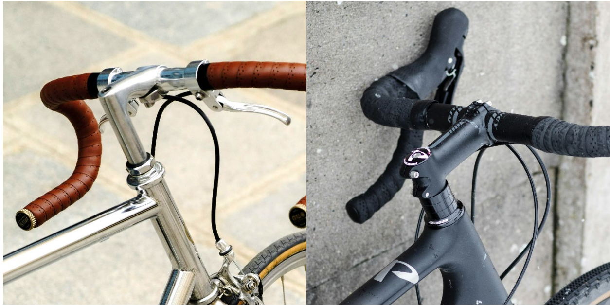
Figure 6. Types of handlebar stems: threaded (left) and threadless (right)
