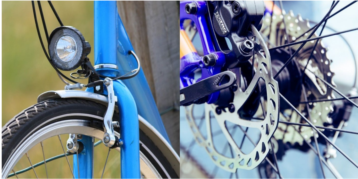
Figure 2. Common brake types: rim brake (left) and disc brake (right)
