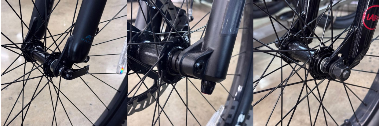
Figure 18. Bicycle hub types: quick-release (left), thru-axle (center), bolt-on (right)
