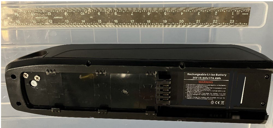
Figure 7 – User replaceable eBike battery pack, 10S4P, 36 V DC (nominal), 10.4 Ah, 374.4 Wh
