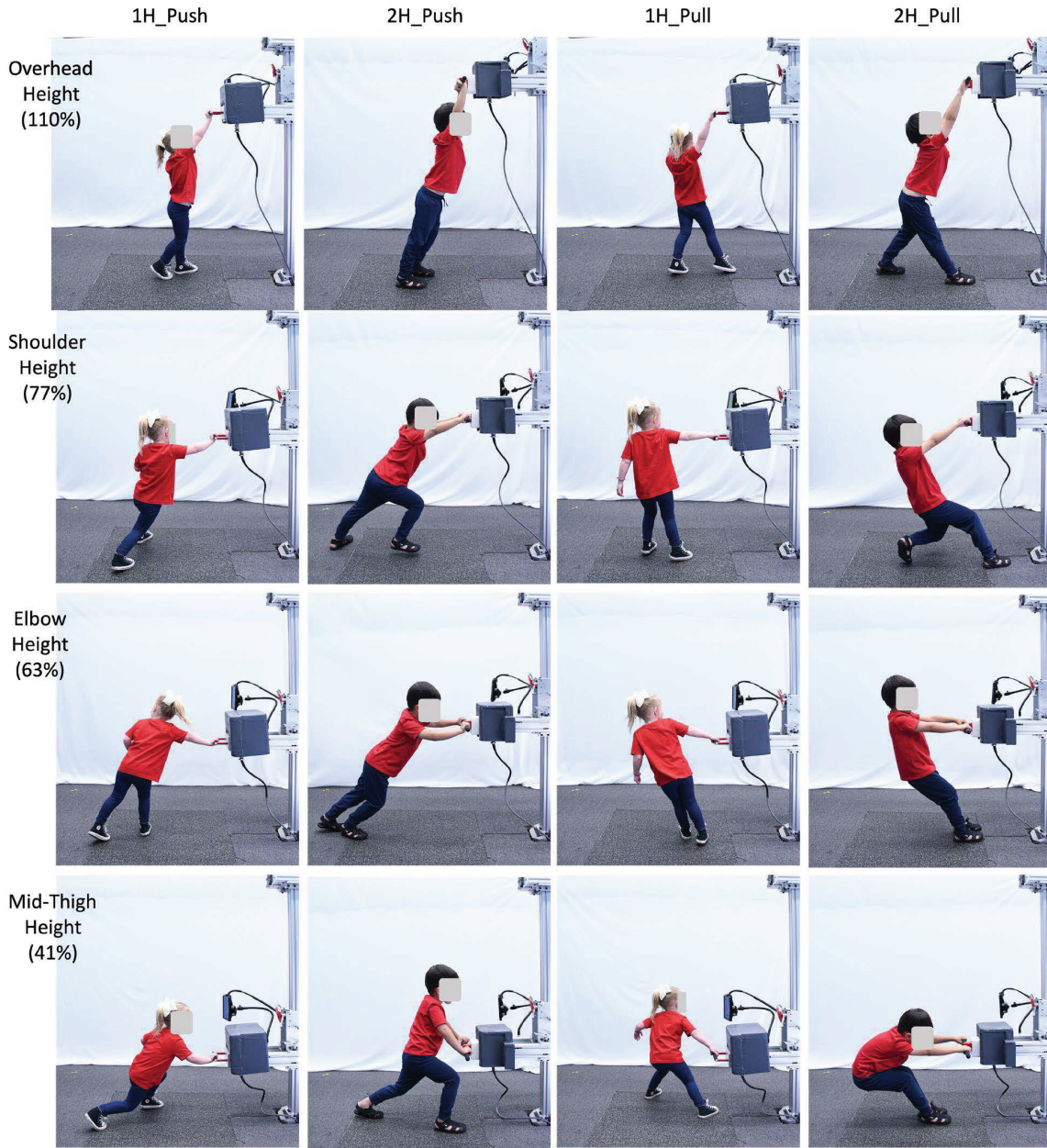
Figure 9. Illustration of one and two-hand standing push and pull exertions (1H_Overhead_Push, 1H_Shoulder_Push, 1H_Elbow_Push; 1H_Thigh_Push; 2H_Overhead_Push, 2H_Shoulder_Push, 2H_Elbow_Push; 2H_Thigh_Push; 1H_Overhead_Pull, 1H_Shoulder_Pull, 1H_Elbow_Pull; 1H_Thigh_Pull; 2H_Overhead_Pull, 2H_Shoulder_Pull, 2H_Elbow_Pull; 2H_Thigh_Pull). Note that the children depicted were not participating in the study; photos were staged for purposes of illustration.
