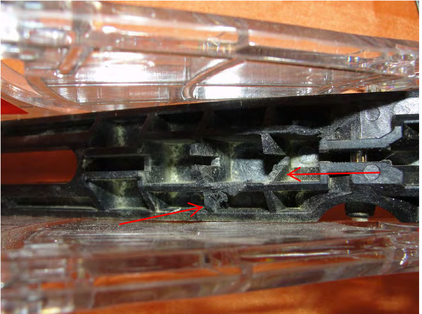
Photo 28: Underside of blade guard showing damage done as a result of the incident
