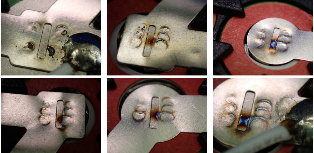
Figure B - 7. Signs of overheating observed on some tab welds on cell cans.
