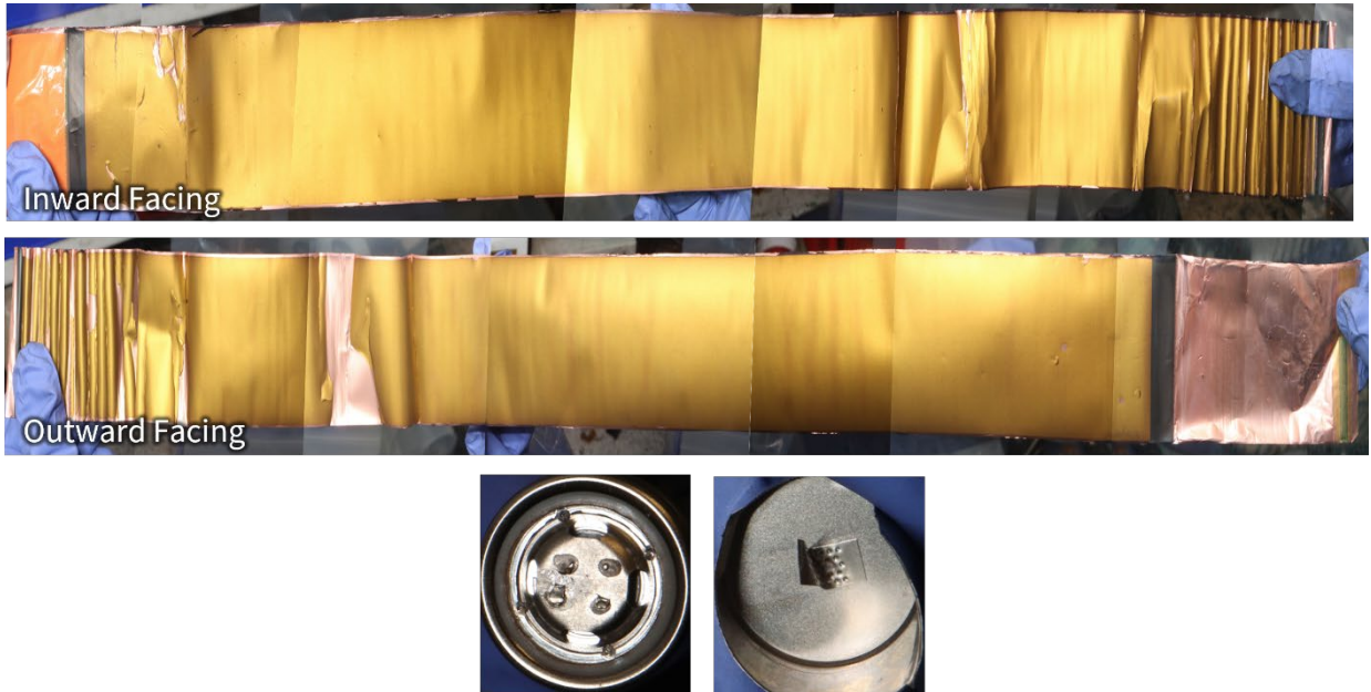
Figure B - 50. Pair 2 OEM – Pack disassembly at 100% SOC; Negative electrodes are shown.
