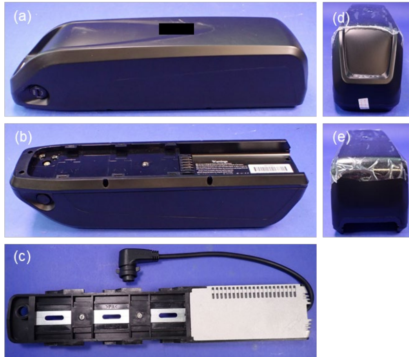
Figure A - 5 Pair 2 OEM – Pack as received; (a) and (b) outer enclosure; (c) adapter between stack and load; (d) and (e) end caps with indicators.
