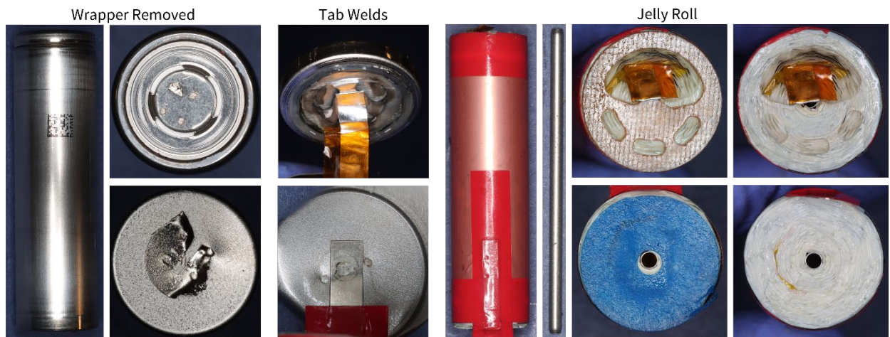
Figure B - 40. Pair 1 Rep – Pack disassembly and cell construction overview.
