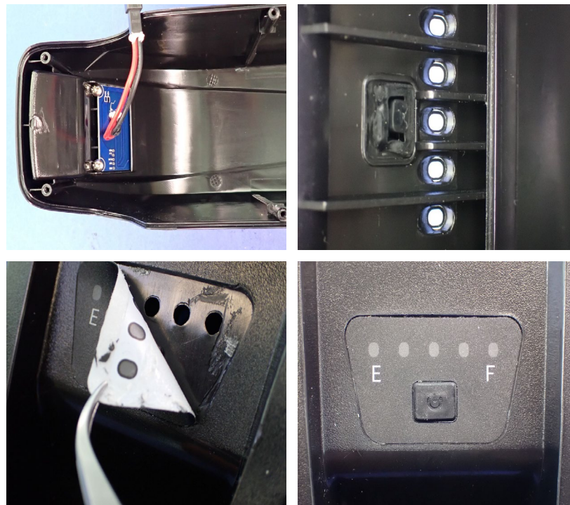
Figure B - 10. SOC indicator had openings that were covered only with a plastic sheet held in place with an adhesive. No gasket or seals were observed around this indicator making it prone to ingress.
