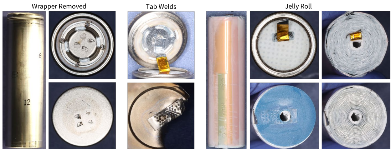
Figure B - 42. Pair 2 OEM – Pack disassembly and cell construction overview.
