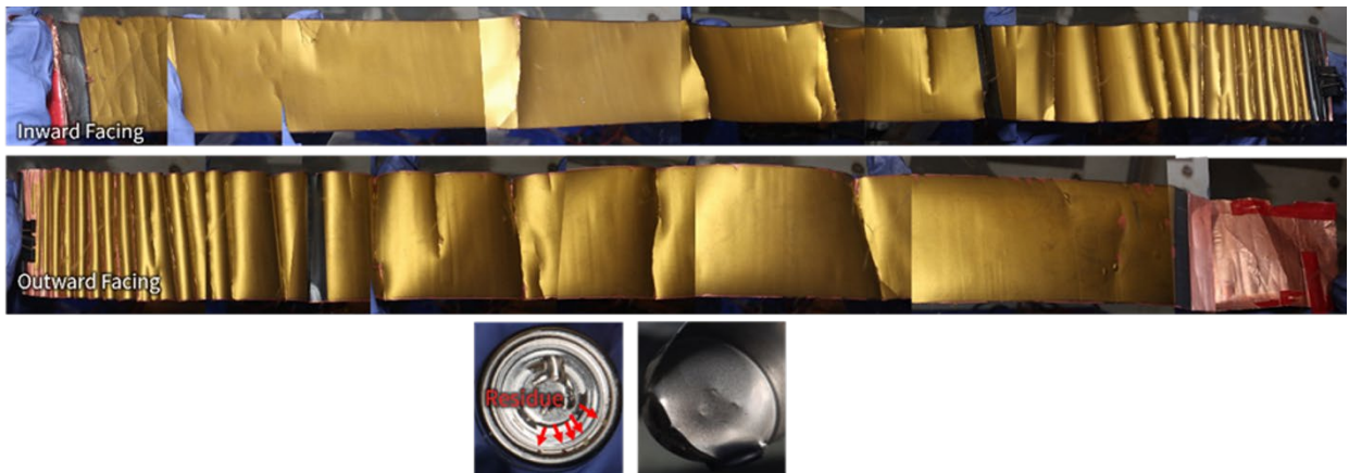
Figure F - 7. Pair 1 Rep – Pack disassembly at 100% SOC; negative electrodes are shown. A brown residue was observed on the edge of the outer can where the crimping occurs.
