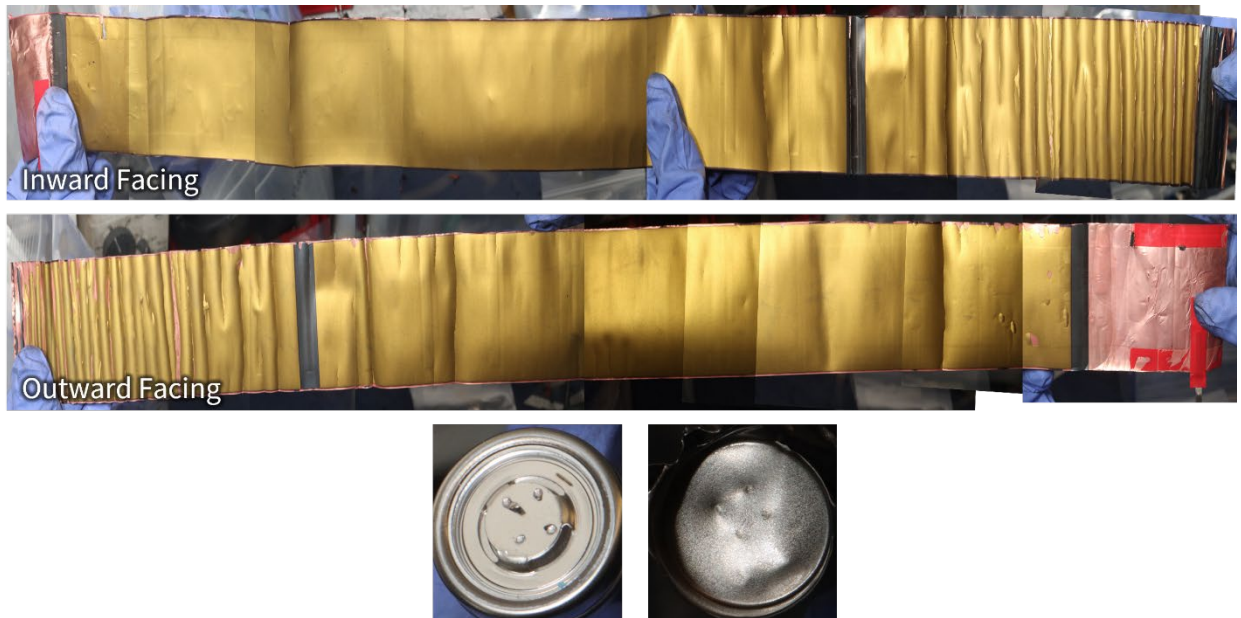
Figure B - 49. Pair 1 Rep – Pack disassembly at 100% SOC; negative electrodes are shown.
