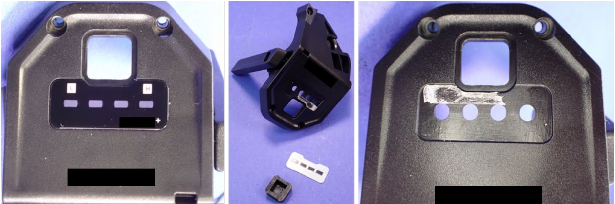
Figure B - 4. SOC indicator had openings that were covered only with a plastic sheet held in place with an adhesive. No gasket or seals were observed around this indicator making it prone to ingress.
