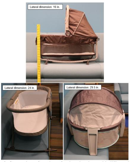
Figure 2: Comparison of overhang for three bassinets with different lateral dimensions on a sofa with a seat depth of approximately 20.25 inches
