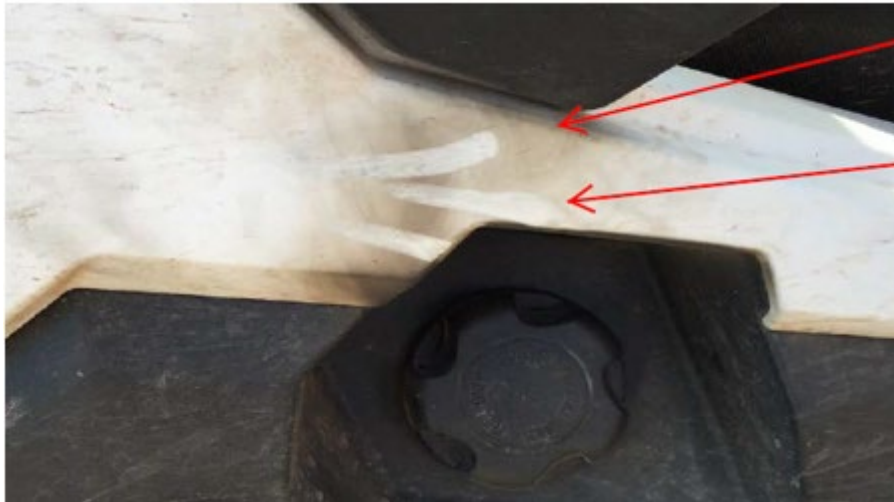
Figure 5 – Soot on the Frame of the ROV (Red Arrows) Resulted from Flames that Shot Out from the Fuel Tank When the Consumer Opened the Gas Cap
