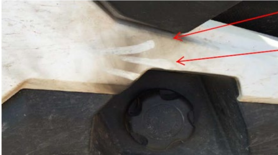
Figure 6 – Soot on the Frame of the ROV (Red Arrows) Resulted from Flames that Shot Out from the Fuel Tank When the Consumer Opened the Gas Cap
