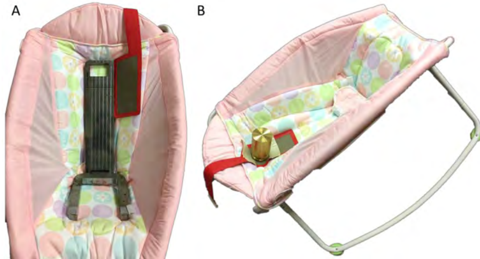
Figure 5. Hinged weight-gauge infant and pressure-mapping sensor location determination (A), and 2 kg weight on pressure-mapping sensor on tilted product (B).
