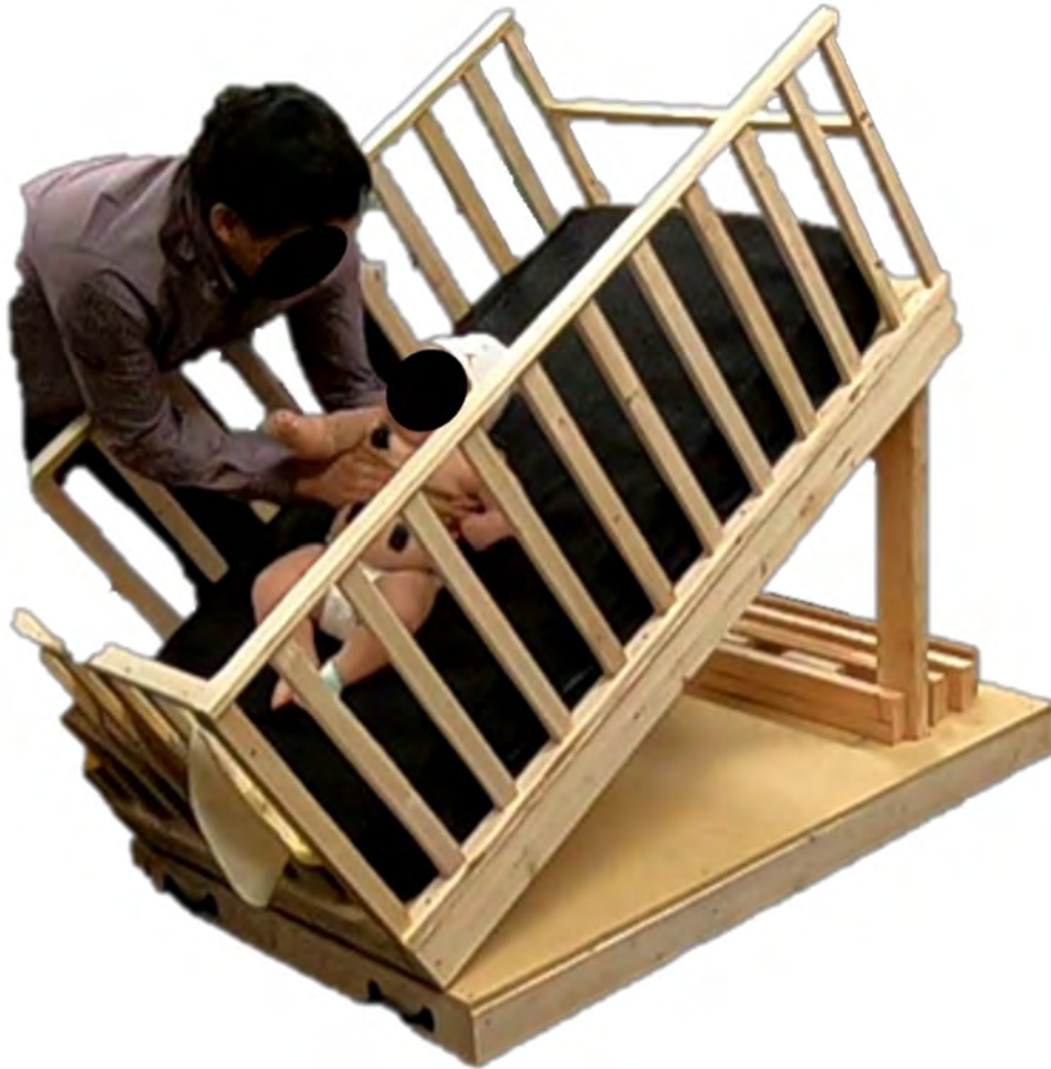
Figure 9. Infant slips downward at 30° incline, presenting a hazard. Therefore, 30° was not included in future testing.
