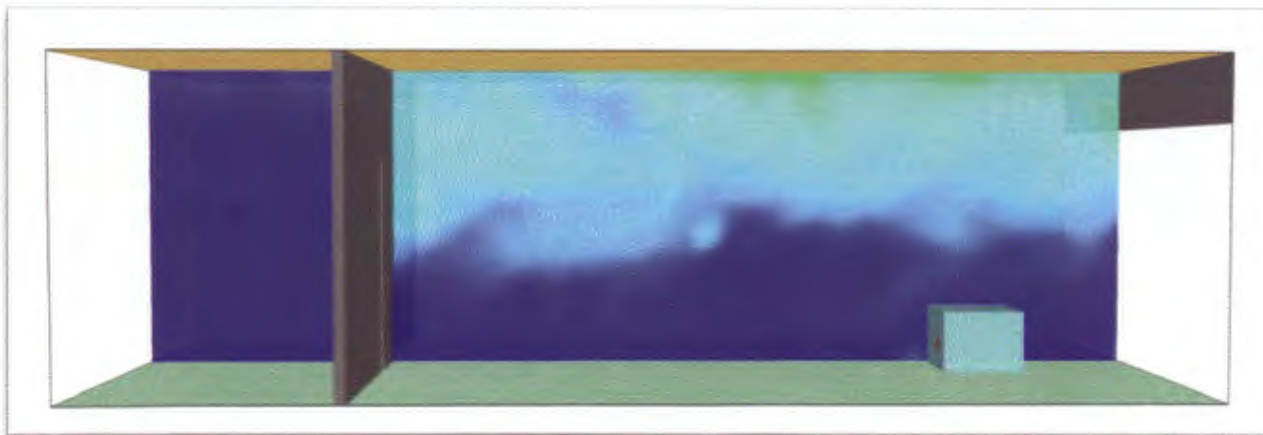
Exhaust volume fraction slice file 1 meter offset from exhaust plane.
