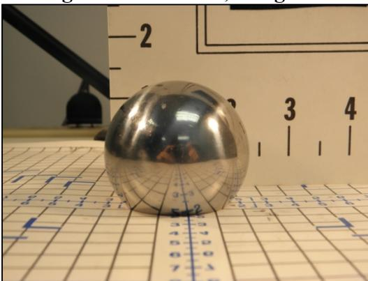
The maximum height of the ball is measured to evaluate against a pass or fail threshold (currently 2.2 meters, as set by AFSL<sup>5</sup>). During FY 2012, staff tested the AFSL’s proposed method to determine if it could be a viable substitute for the current test methods. Photographs of the plastic tubes affixed with an electronic match, as well as the electronic ignition device used in the testing are shown in Figures 3 and 4.
