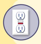
Use ground-fault circuit-interrupters (GFCI) – inside and OUTSIDE the house.
