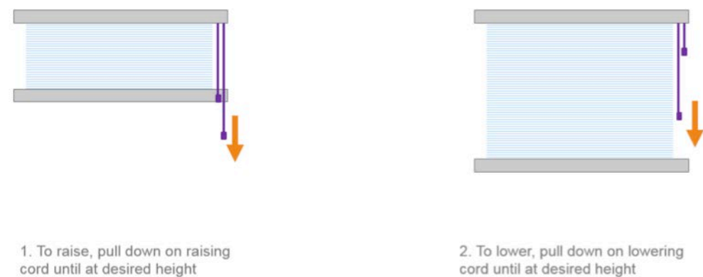
Figure 39. Mechanism 5 Raising and Lowering Operations
