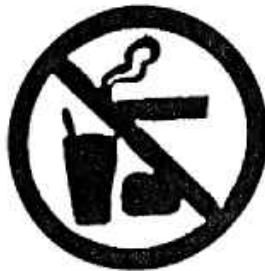
Figure 7.4 Example of a nearly illegible pictorial symbol. It is supposed to mean 'no eating, drinking or smoking'.
