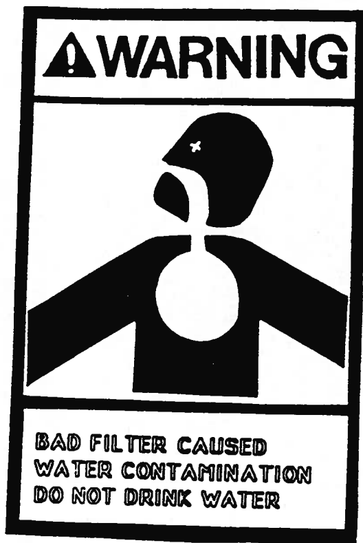
Figure 1. Enhanced warning on water fountain. Note that the top panel that serves as a background to the word WARNING was orange.
