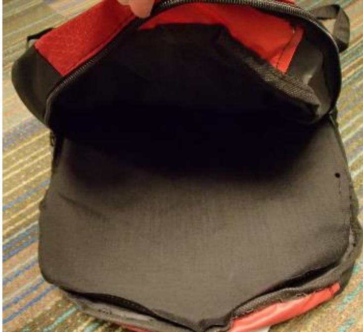
Figure 6. Consumer view when opening main section of backpack. Stitching has been removed in order to access ballistic panel.
