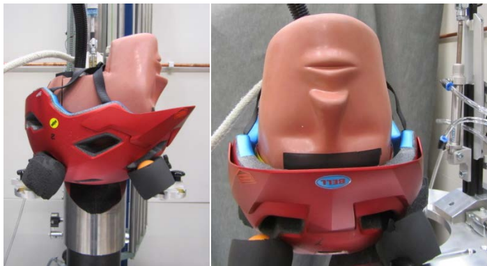
Figure 5. Oblique test with rotation around the x-axis.
