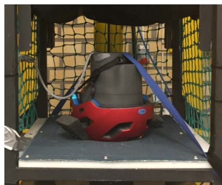
Figure 2. The method used in shock absorption test
