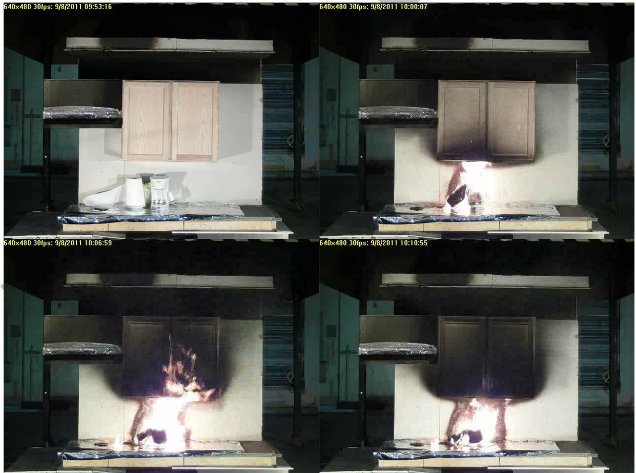
Figure 28. Photo sequence for Test A1B - Oak/pressboard with barrier exposed to ignition scenario
