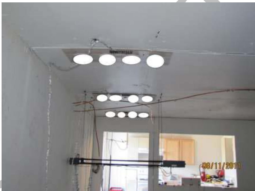
Figure 13. Picture showing alarm placements, extinction meter, sampling tubes, and window and door openings.
