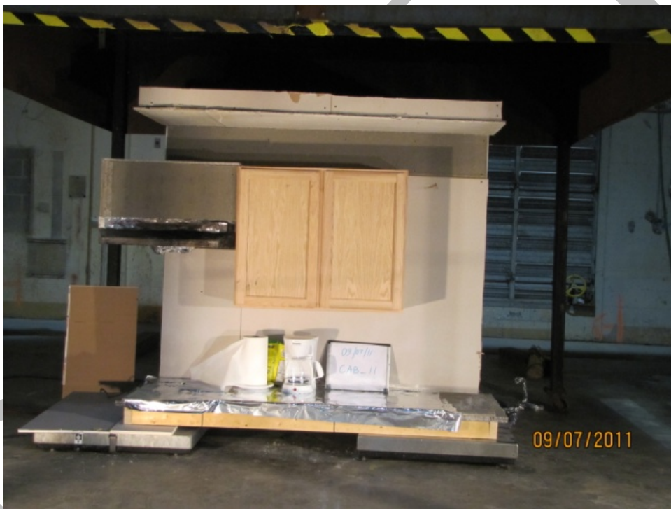
Figure 9. Kitchen counter and cabinet mock-up. The counter level rests on load cells, and the entire mock-up fits under the furniture calorimeter hood.
