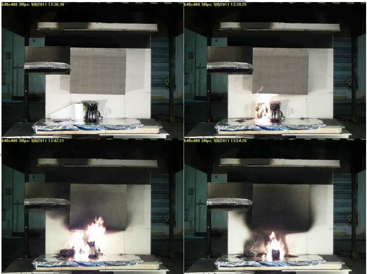
Figure 36. Photo sequence for Test CB1 – Cement board exposed to ignition scenario 1.
