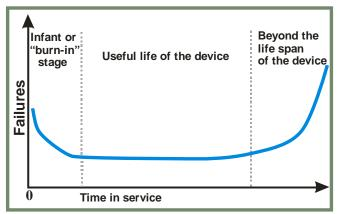
Figure 1. Typical failure rate plot for devices
