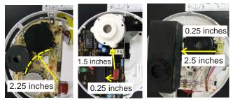
Figure 6. Varied distance between critical components
