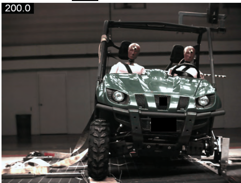
Figure 4.7 Sled Test at time = 200 msec
