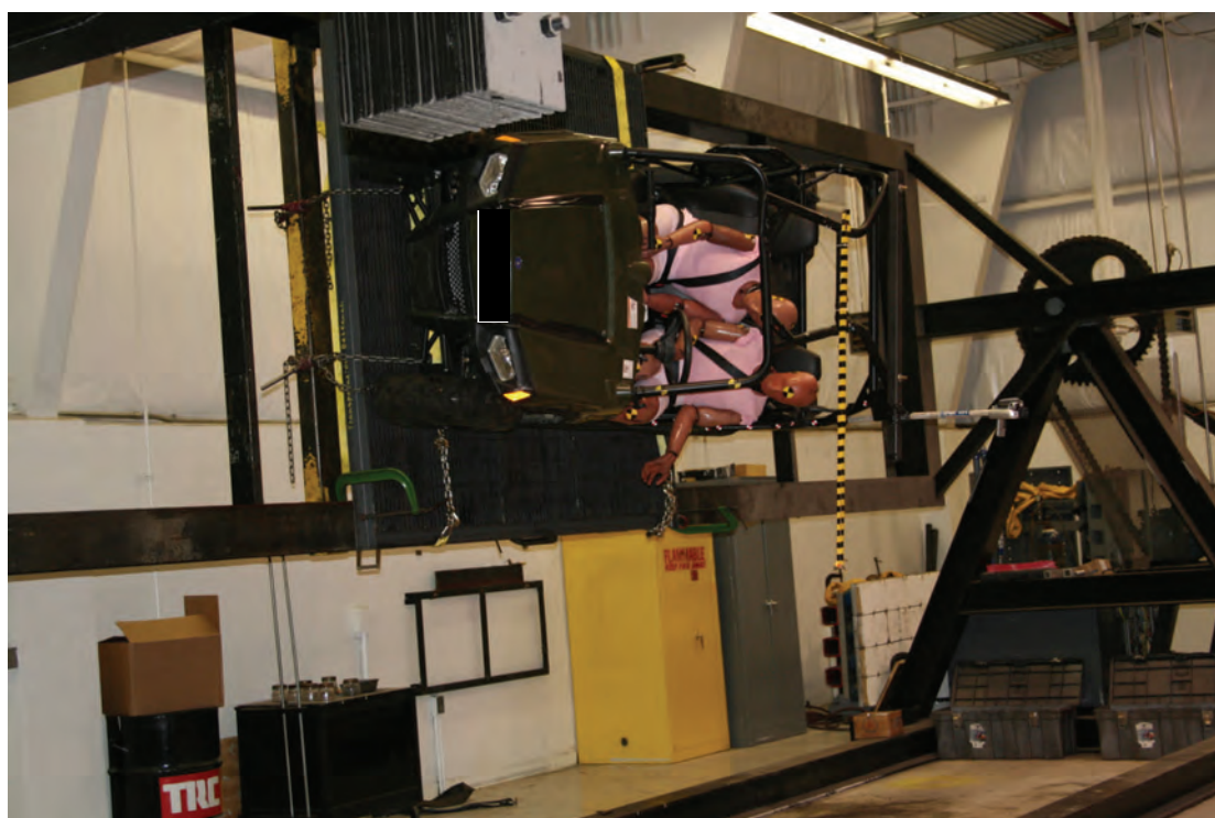
Figure 3.8 Vehicle at 90 degrees Static Roll
