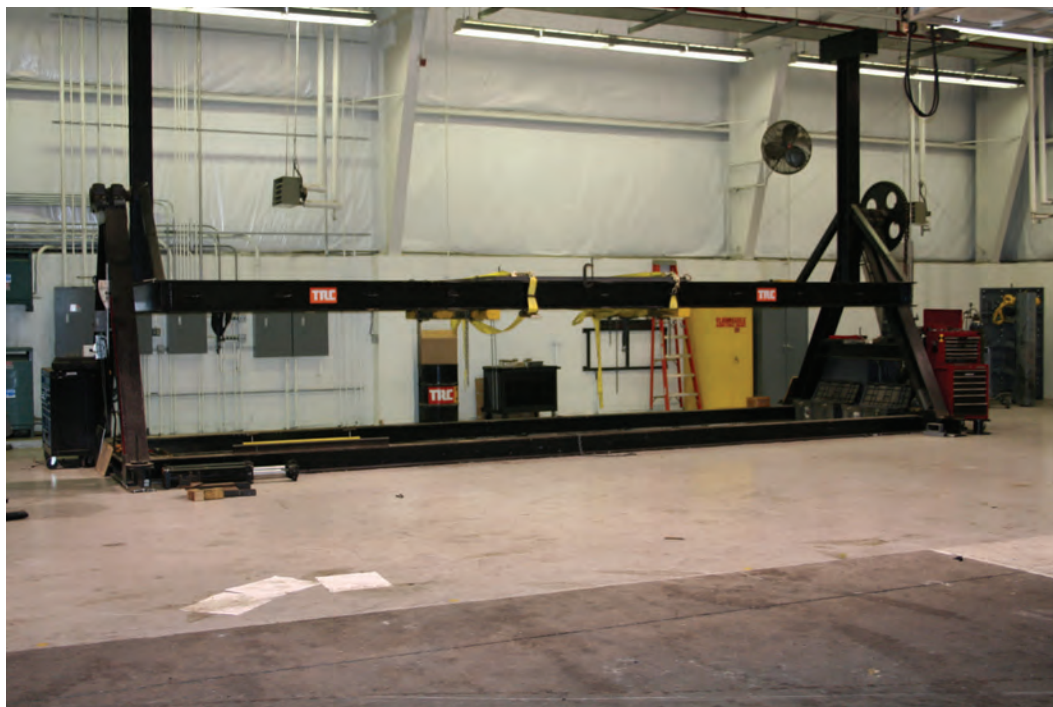
Figure 3.1 FMVSS 301 Static Roll Test Fixture
