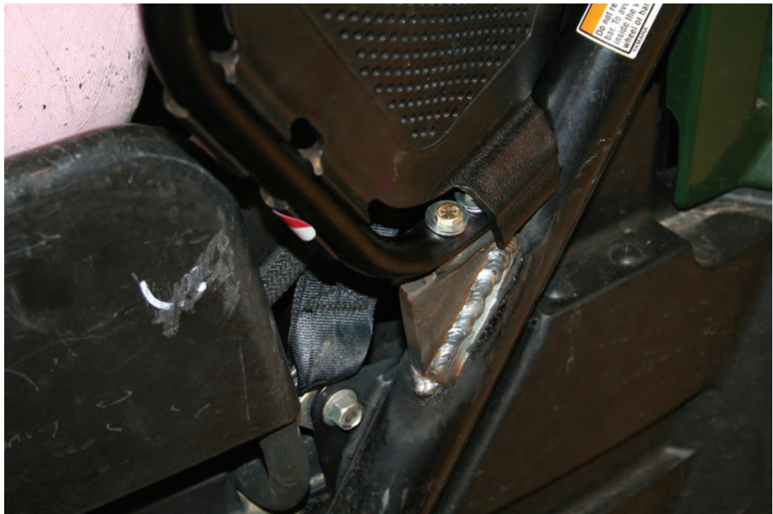
Figure 3.14 Lower Mounting of Enhanced Restraint in [REDACTED]
