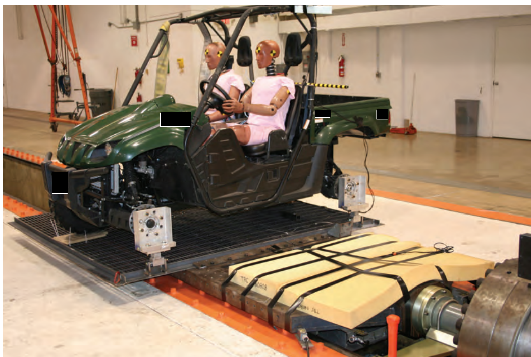
Figure 3.15 Padding Added for Unbelted Dummy Tests
