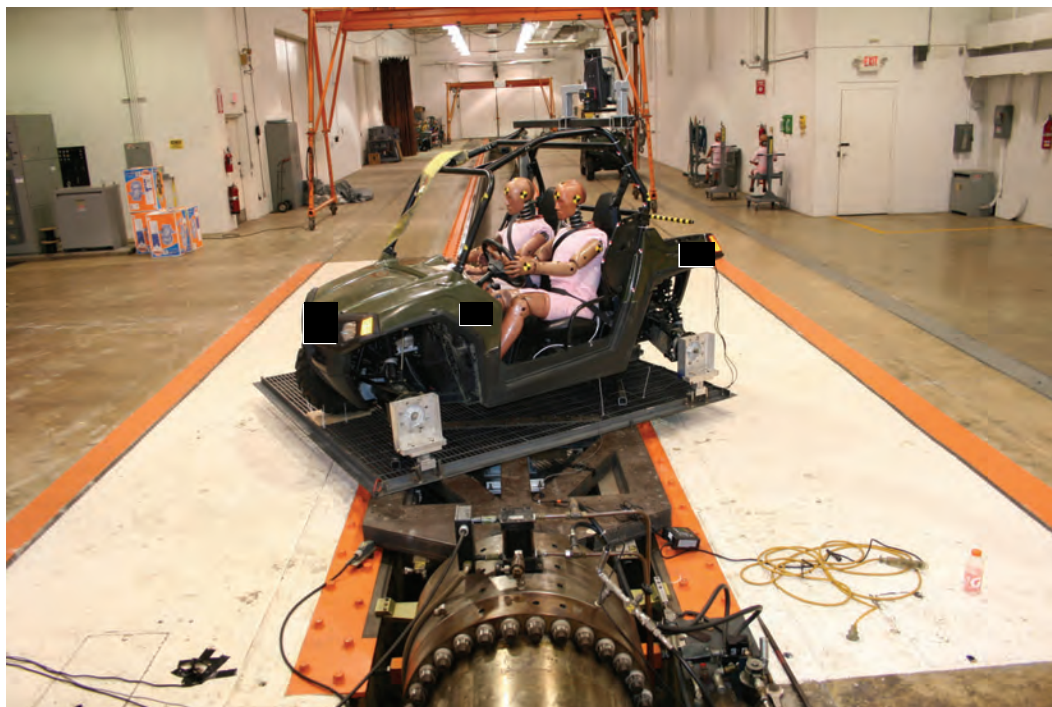
Figure 3.9 Vehicle Mounting Hinges on Sled
