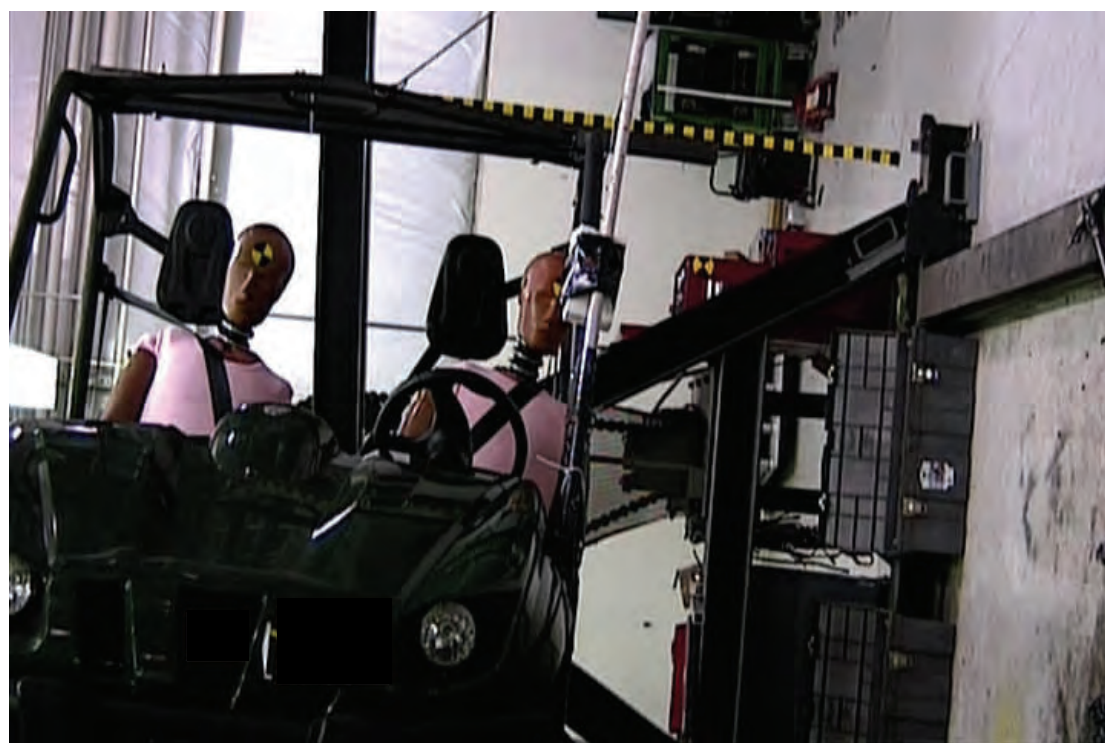
Figure 4.5 Static Test of [REDACTED] with Enhanced Restraint at 90 degrees
