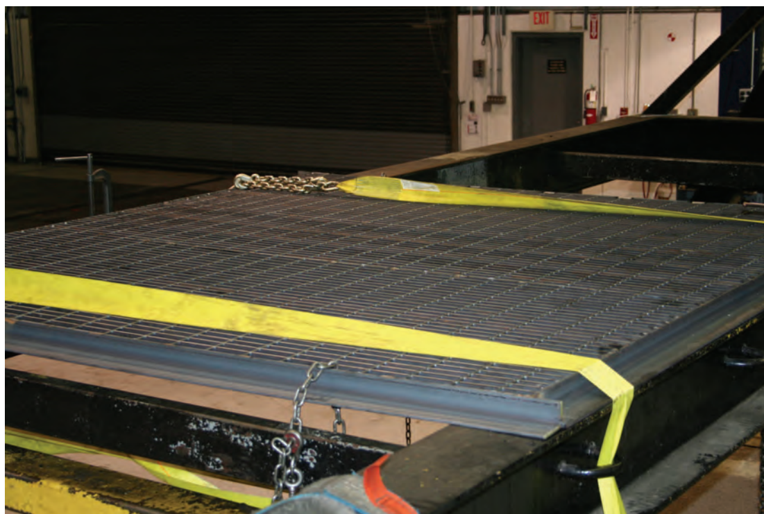
Figure 3.2 Grating on 301 Test Fixture
