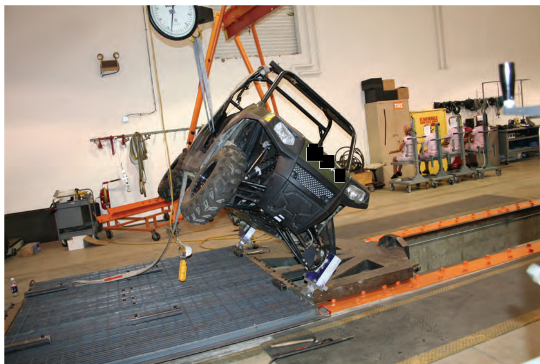
Figure 3.10 Vehicle Rotated for Tether Adjustment
