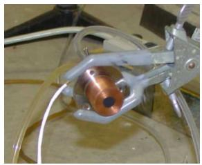
Figure 1: Radiant Flux Sensor
