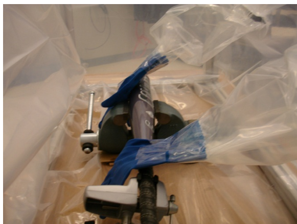
Figure 2: Temporary glove box constructed with a large plastic bag, plastic gloves and 80-20 framing. This photo illustrates how the bat was held in place during the cutting process.
