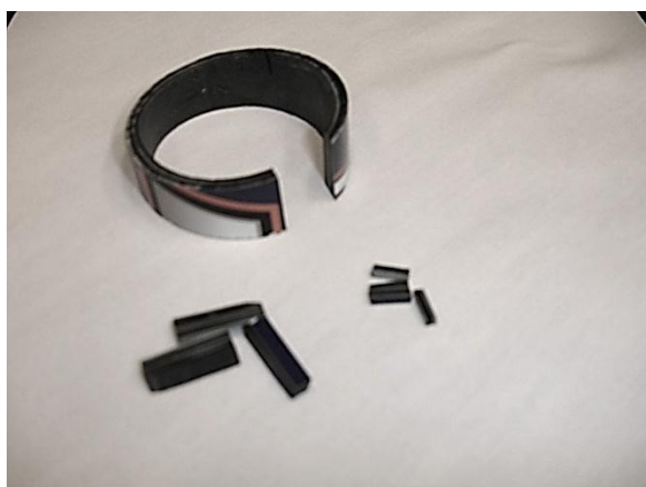
Figure 3: Larger open ring shaped piece is from the original hack saw cut in the glove bag. Smaller pieces were obtained from the ring shaped piece using a wet band saw.
