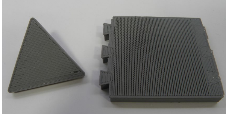
Figure 7: An example of different bottom layer finishes based on the structure's printing location on the flexible bed.
