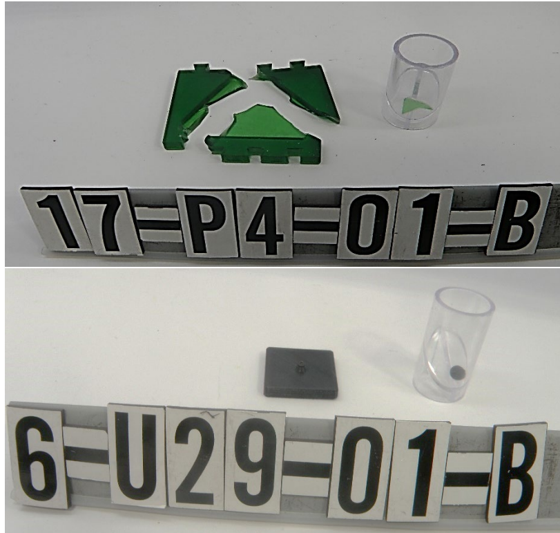
Figure 15: Examples of First Puzzle System sets which liberated small parts that did not meet the requirements of ASTM F963-17. Top; A Printer D resin sample with spider cracks originating from the center of its thinnest wall. Bottom; Printer A filament sample which fractured at the knob-peg connection point.
