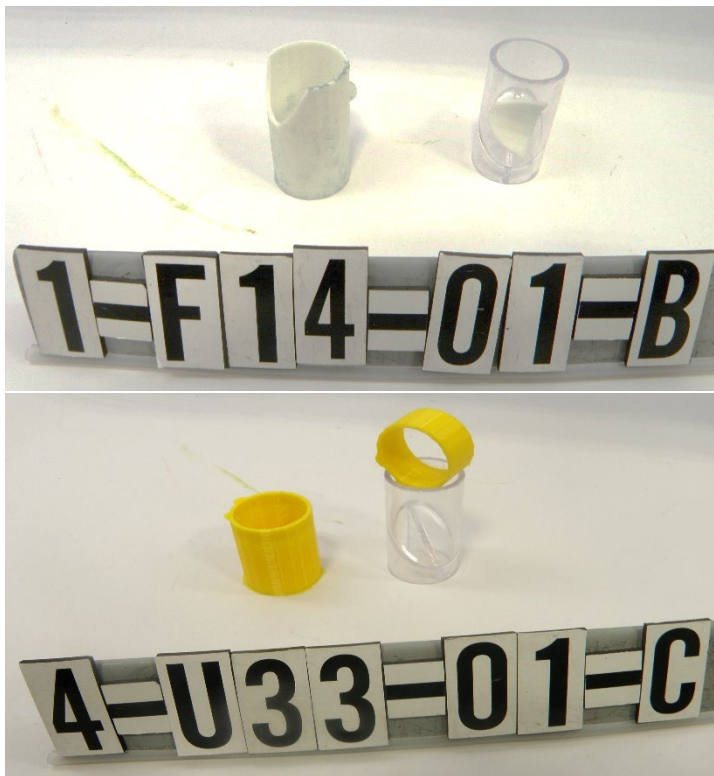
Figure 12: Example of Bubble Toy sets which fractured. Top; A Printer C resin sample which liberated a part that did not meet the requirements of ASTM F963-17. Bottom; Printer A filament sample which fractured at approximately the same point but distributed the force such that the split portion still met the same requirements.
