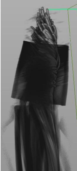
(a) CT image of butt connection (b) CT cross section of butt connector
