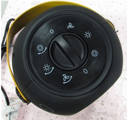
Mechanical heat selector switch (S24)
