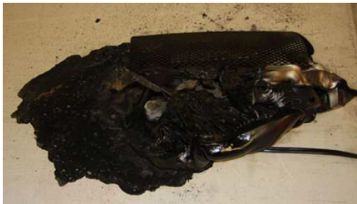
Heater sample in open room after test
