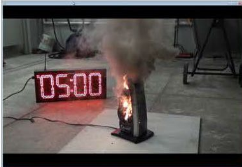
5 minutes after exposed to source flame
