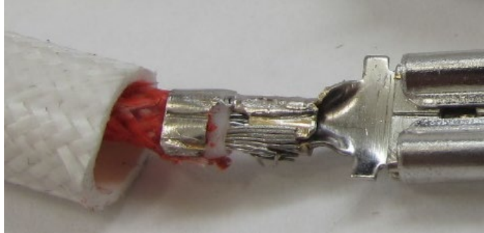
Figure 7-29. Poor crimp connection
