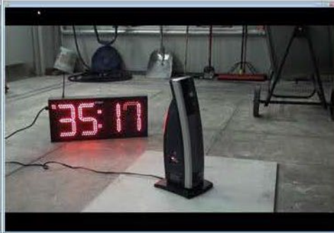
Time 35.17 seconds after exposed to flame 5.17 seconds after source flame removed
