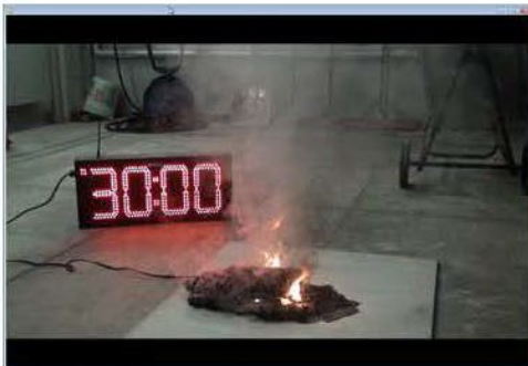
30 minutes after exposed to source flame Ignition of the fan housing in an open room
